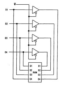
Figure 5. Separate I/O Buffer
