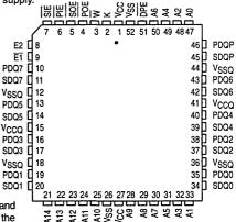
All power supply and ground pins must be connected for proper operation of the device.  $V_{CC} \ge V_{CCQ}$  at all times including power up.
