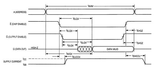
NOTE: Addresses valid prior to or coincident with  $\overline{E}$  going low/  $\overline{E}$  going high.
