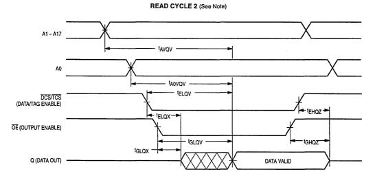
NOTE: Address valid prior to or coincident with  $\overline{\text{DCS}}$  or  $\overline{\text{TCS}}$  going low.
