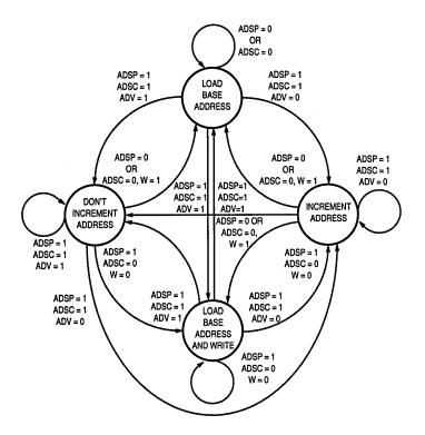
Figure 2. State Diagram for Address Determination on the MCM62486A BurstRAM
