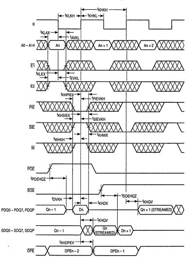
NOTE: DPE is valid exactly one clock cycle after the output data is valid.
