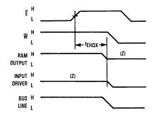
Figure 2c. Using E to Avoid Bus Contention
