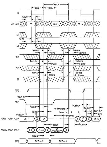
NOTE: DPE is valid exactly one clock cycle after the output data is written.
