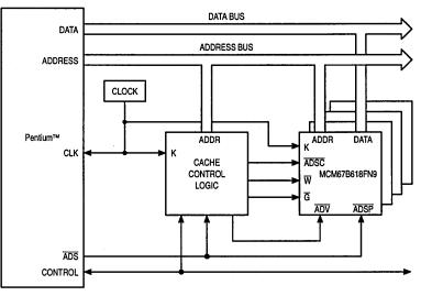
512K Byte Burstable, Secondary Cache Using Four MCM67B618FN9s with a 66 MHz Pentium
