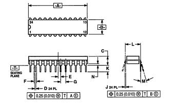
NOTES: 1. DIMENSIONING AND TOLERANCING PER ANSI Y14.5M, 1982. 2. CONTROLLING DIMENSION: NCH. 3. DIMENSIONL TO CENTER OF LEAD WHEN FORMED PARALLEL. 4. DIMENSION A AND B DOLES NOT INCLUDE MOLD FLASH. MAXIMUM MOLD FLASH 0.25 (0.010).
