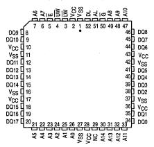
All power supply and ground pins must be connected for proper operation of the device.
