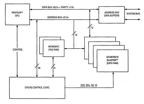
Configuration A Secondary Cache Solution for Pentium --- 512KByte
