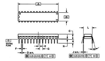
NOTES: 1. DIMENSIONING AND TOLERANCING PER ANSI Y14.5M, 1982. 2. CONTROLLING DIMENSION: NCH. 3. DIMENSIONL TO CENTER OF LEAD WHEN FORMED PARALLEL 4. DIMENSION A AND B DOES NOT INCLUDE MOLD FLASH. MAXIMUM MOLD FLASH 0.25 (0.010).
