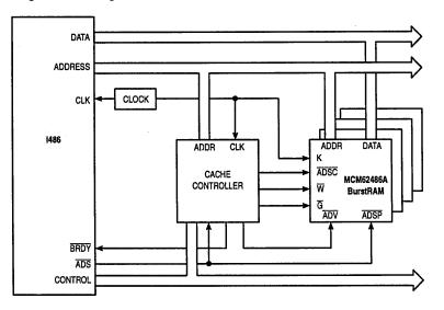
Figure 3. i486 128K Byte Burstable Cache Memory Block Diagram
