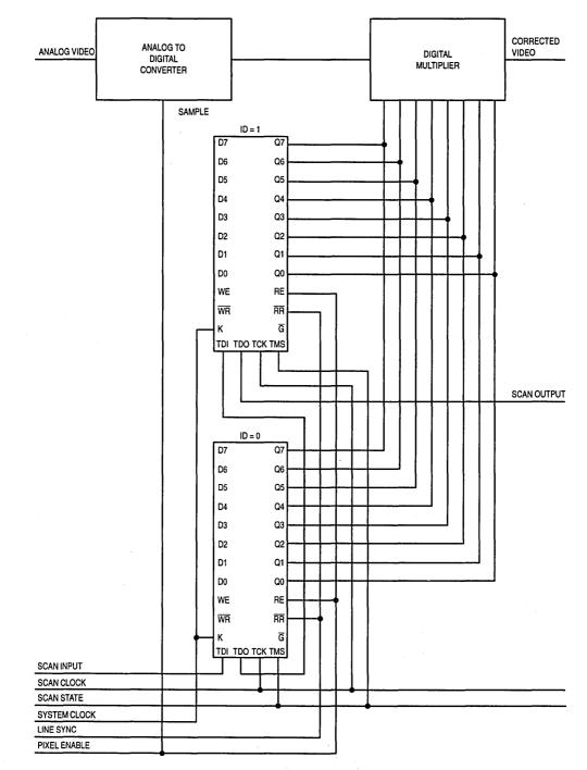
Figure 9. CCD Gain Correction, Buffer Written From Scan Input (16384 Pixels Maximum)
