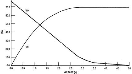
Figure 5. IOL/IOH Output Buffer Characteristics (Iout vs Vout) for MCM6205C, MCM6206C, MCM6264C, MCM6265C, MCM56824A, MCM56824AZP
