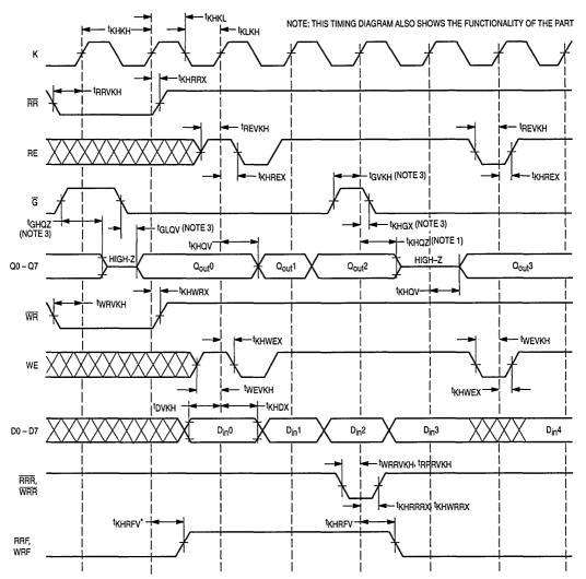
\*Roll-Over Outputs assert high when counters reach their initial value. This timing diagram shows the relationship between the roll-over output and reset pin only.
