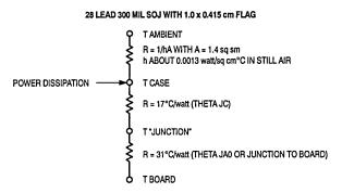
NOTE: Theta JA simulated in Natural Convection 77°C/watt.
