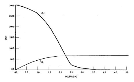
Figure 3. IOL/IOH Output Buffer Characteristics (I<sub>OUt</sub> vs V<sub>Out</sub>) for MCM6705A, MCM6706A, MCM6708A, MCM6709A
