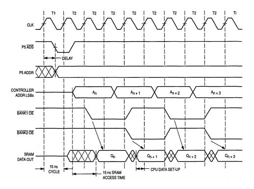
Figure 1. Two Bank Asynchronous SRAMs Performing 3-2-2-2 Burst READ
