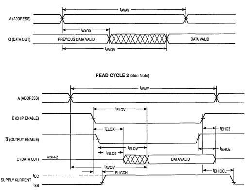
NOTE: Addresses valid prior to or coincident with  $\overline{E}$  going low/ $\overline{E}$  going high.
