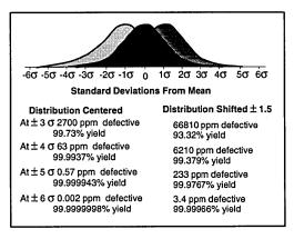
Figure 2. Percent Defective and Yield from a Normal Distribution of Product with 6σ Capability
