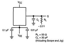
Figure 2. AC Test Circuit
