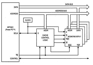
256K Byte Burstable, Secondary Cache Using Four MCM67M518FN11s with a 66 MHz MPC601 Power PC™
