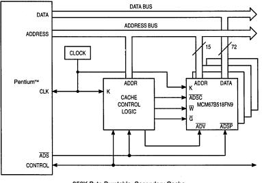
256K Byte Burstable, Secondary Cache Using Four MCM67B518FN9s with a 66 MHz Pentium
