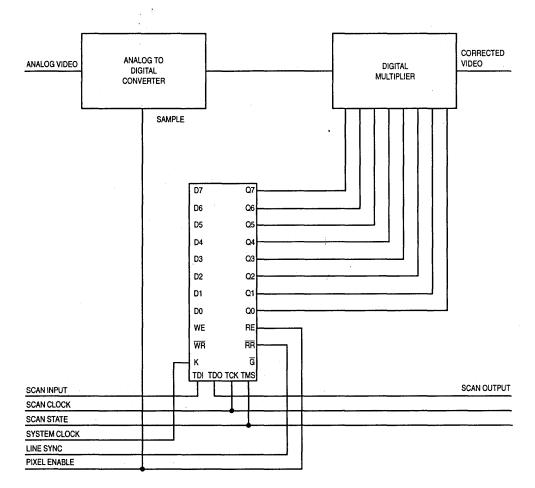
Figure 10. CCD Gain Correction, Buffer Written From Scan Input (8192 Pixels Maximum)
