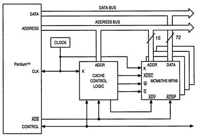
256K Byte Burstable, Secondary Cache Using Four MCM67H518FN9s with a 66 MHz Pentium
