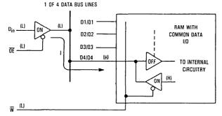
Figure 1. Common I/O Bus Contention
