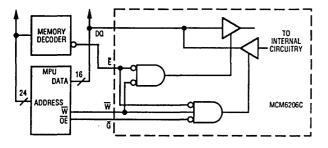
Figure 4a. Using G to Avoid Bus Contention
