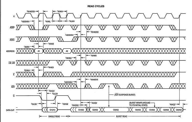
NOTE: Q1(A2) represents the first output data from the base address A2; Q2(A2) represents the next output data in the burst sequence with A2 as the base address.
