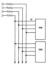
Figure 6. Using Series Terminating Resistors
