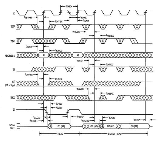
NOTE: Q1(A2) represents the first output from the external address A2; Q2(A2) represents the next output data in the burst sequence with A2 as the base address.
