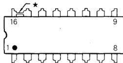
★ External lead connection (shorting bar) between Pins 15 and 16.
