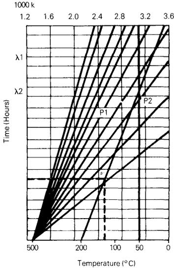
For increased flexibility in working with a broad range of device hours, the time-temperature regression lines have been normalized to 500°C and the time scale omitted, permitting the user to define the scale based on his own requirements.
