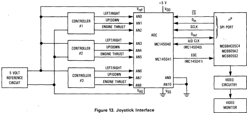
Figure 13. Joystick Interface
