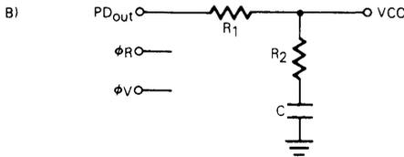
$$\omega_n = \sqrt{\frac{K_\phi K_{VCO}}{NC(R_1 + R_2)}}$$
