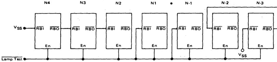
FIGURE 3 – LEADING AND TRAILING ZERO SUPPRESSION WITH PWM INTENSITY BLANKING AND NO LAMP TEST
