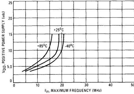
FIGURE 2 – MAXIMUM OSCILLATOR INPUT FREQUENCY versus SUPPLY VOLTAGE
