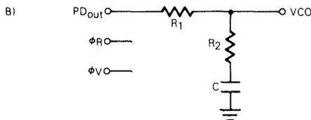
$$\omega_n = \sqrt{\frac{K_\phi K_{VCO}}{NC(R_1 + R_2)}}$$
