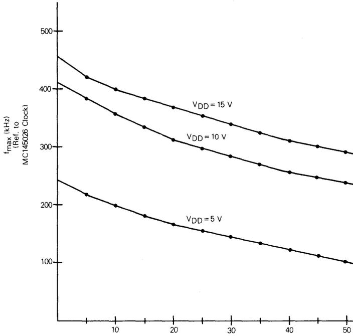
$C_{layout}$  (pF) on Pins 1-5 (MC145027); Pins 1-5 and 12-15 (MC145028);
