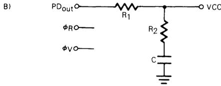
$$\omega_n = \sqrt{\frac{K_\phi K_{VCO}}{NC(R_1 + R_2)}}$$
