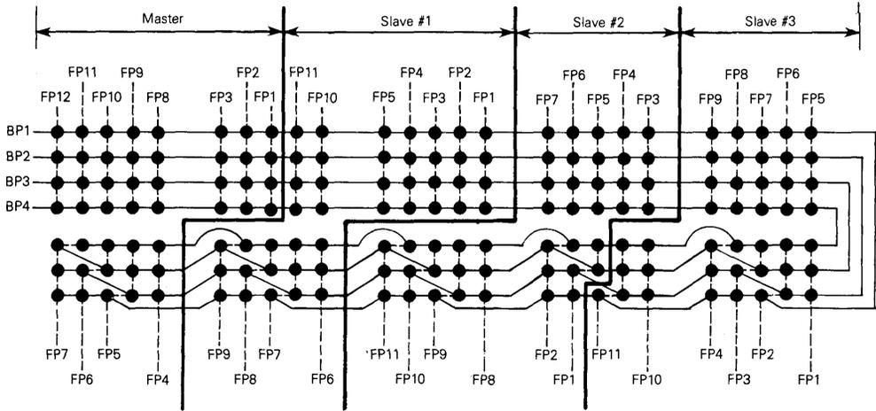
FIGURE 9 — EXAMPLE OF A 5x7 DOT MATRIX DISPLAY SYSTEM CONTROLLED BY TWO MASTER AND TWO SLAVE UNITS
