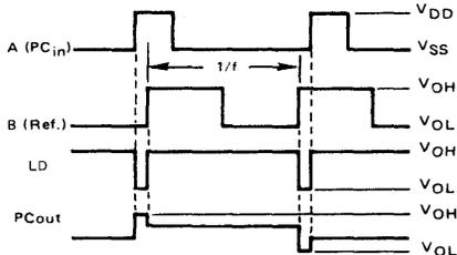
FIGURE 5 - PHASE COMPARATOR STATE DIAGRAM
