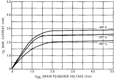
FIGURE 4 – TYPICAL P-CHANNEL SOURCE CURRENT AT VDD-VSS = 5 VOLTS
