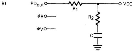
$$\omega_n = \sqrt{\frac{K_\phi K_{VCO}}{NCR_1 + R_2}}$$
