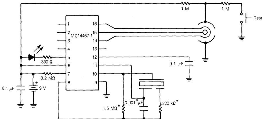
\*NOTE: Component values may change depending on type of piezoelectric horn used.
