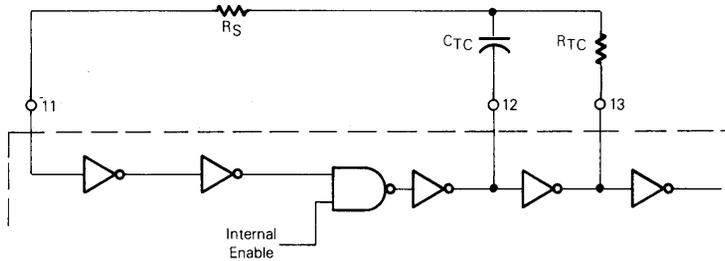
This oscillator will operate at a frequency determined by the external RC network; i.e.,
