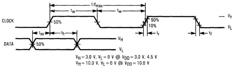
Figure 1. Switching Waveforms
