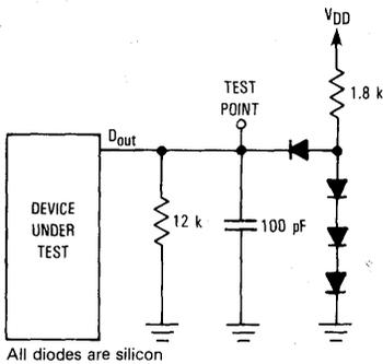
Figure 7. Test Circuit
