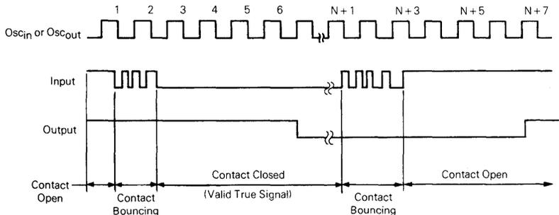
FIGURE 4 – TYPICAL "FORM A" CONTACT DEBOUNCE CIRCUIT
