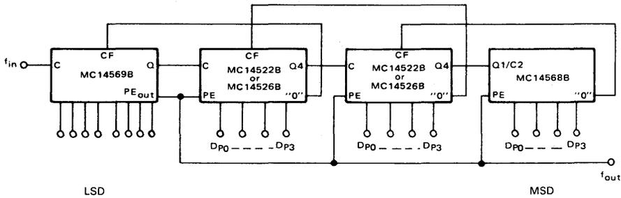
FIGURE 7 – FREQUENCY SYNTHESIZER WITH MC14568B and MC14569B USING A MIXER
