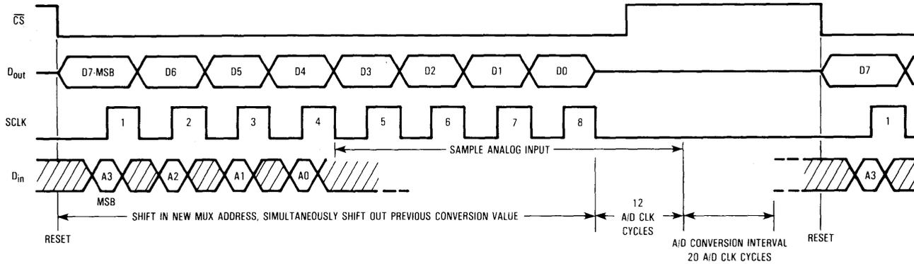
Figure 9. MC145040 Timing Diagram Utilizing  $\overline{CS}$  to Three-State  $D_{out}$
