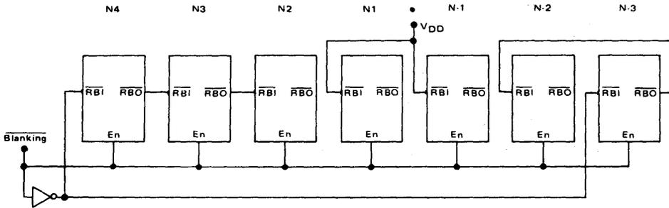
FIGURE 4 – ZERO SUPPRESSION WITH LAMP TEST AND INTENSITY BLANKING
