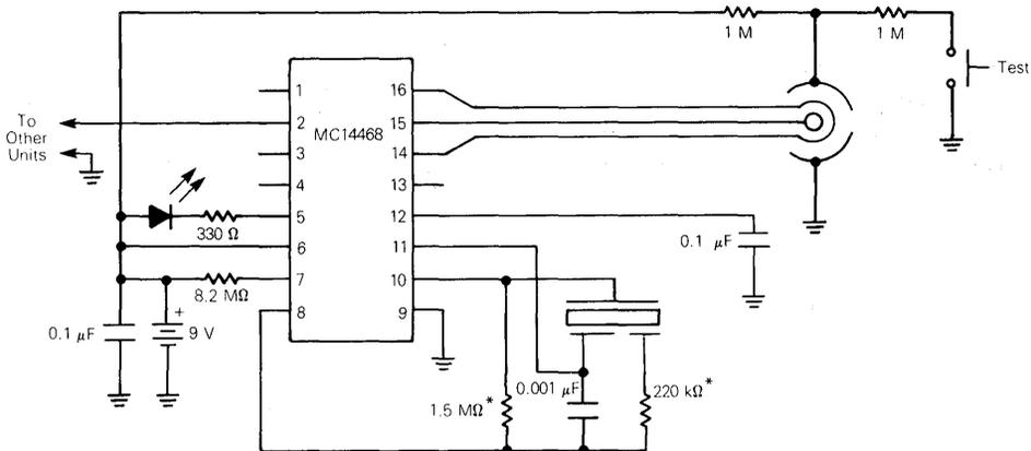
\*NOTE: Component values may change depending on type of piezoelectric horn used.
