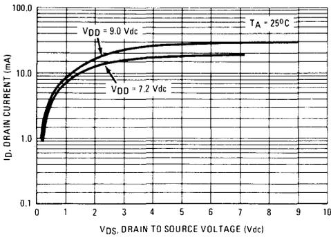
FIGURE 2 — TYPICAL COMPARATOR OUTPUT I-V CHARACTERISTIC
