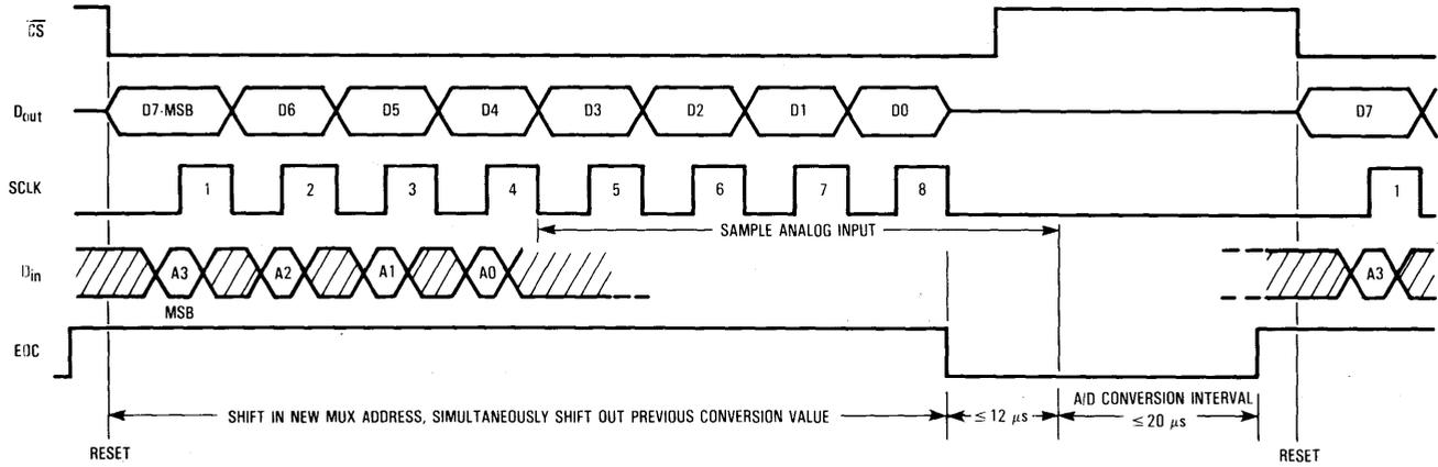
Figure 11. MC145041 Timing Diagram Utilizing CS to Three-State D<sub>out</sub>
