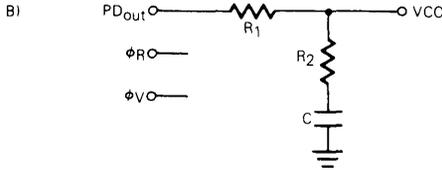
$$\omega_n = \sqrt{\frac{K_\phi K_{VCO}}{N C (R_1 + R_2)}}$$
