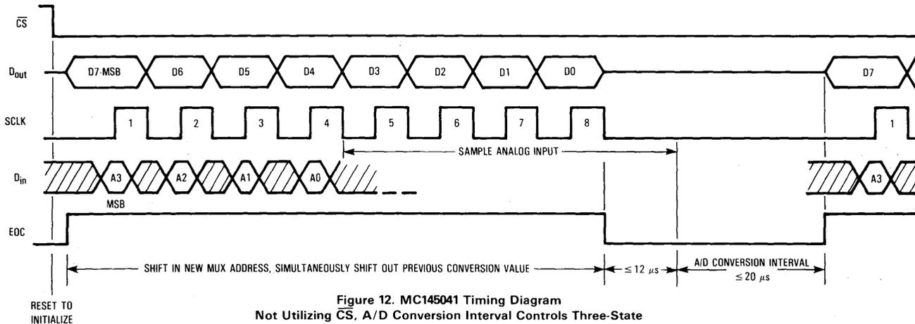
Figure 12. MC145041 Timing Diagram Not Utilizing CS, A/D Conversion Interval Controls Three-State
