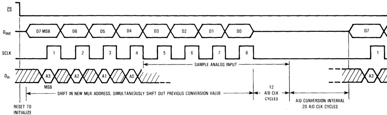
Figure 10. MC145040 Timing Diagram Not Utilizing  $\overline{CS}$ , A/D Conversion Interval Controls Three-State
