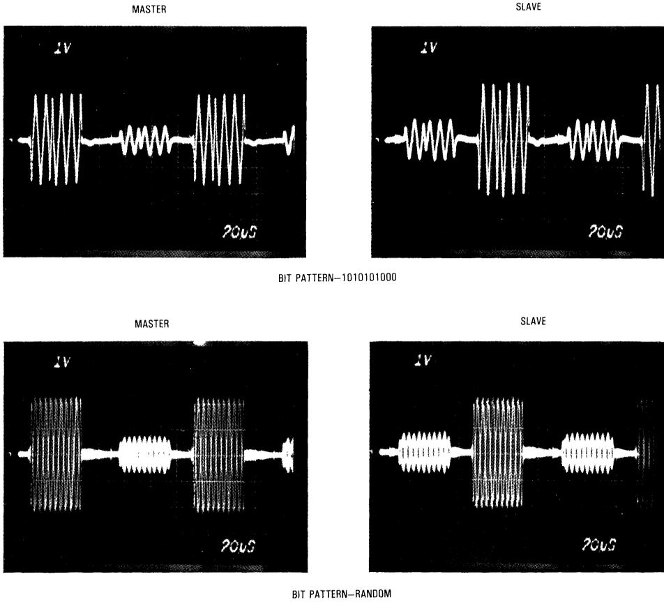
Figure 14. Typical Signal Waveforms at Demodulator
