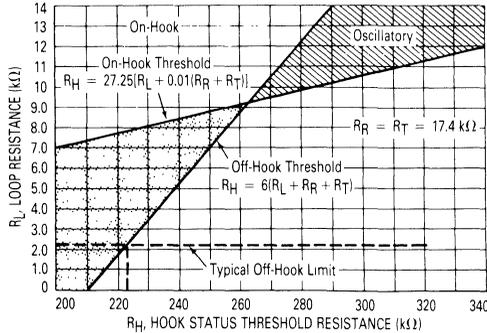
Figure 11 shows such a graph using 17.4 kΩ as the values for  $R_R$  and  $R_T$ . Note the oscillatory condition to the right of the crossing point. Selection of  $R_H$  in this region is usually not a problem since the majority of telephone lines do not fall into this resistance range.  $R_H$  always ties to  $V_{QB}$  and HST and will give reliable hook status information regardless of power supply voltages and  $\overline{PDI}$ .
