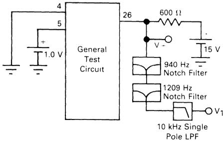
Note: The notch filters must have 50 dB attenuation at their respective center frequencies.
