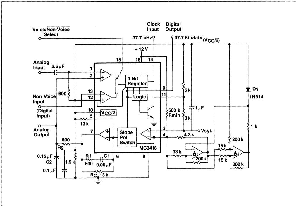
FIGURE 5 — TELEPHONE QUALITY DELTA MODULATOR CODEC
