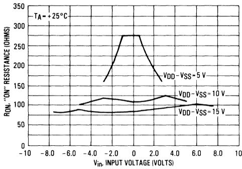
FIGURE 8 —  $V_{DD} = 2.5\text{ V}$ ,  $V_{SS} = -2.5\text{ V}$
