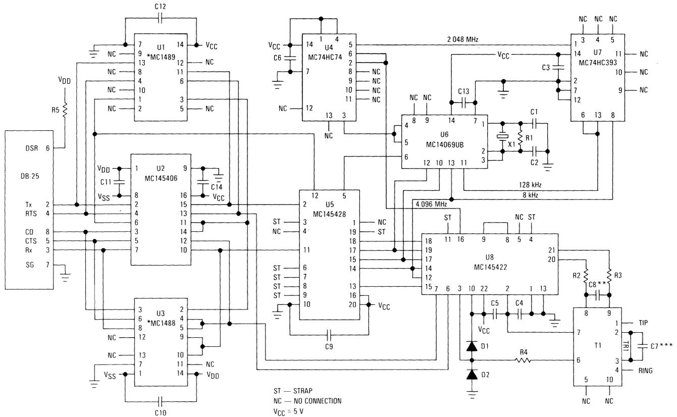
Figure 5. Master Limited Distance Modem
