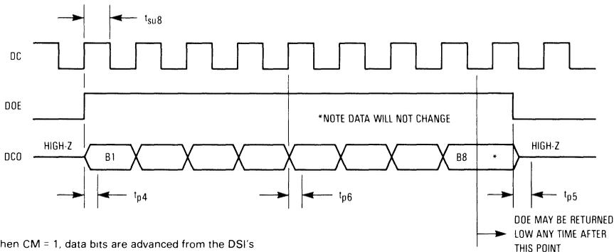
NOTE When CM = 1, data bits are advanced from the DSI's SYNCHRONOUS CHANNEL TRANSMITTER at the DCO pin on the rising edge of the signal formed by the LOGICAL AND of DC and DOE (DC • DOE)
