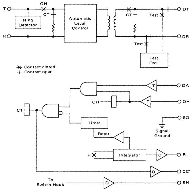
FIGURE 14 – Block Diagram of CBT Data Coupler
