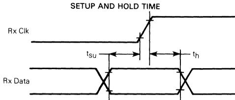
Note: Timing measurements are referenced to and from a low voltage of 0.8 volts and a high voltage of 2.0 volts, unless otherwise noted.
