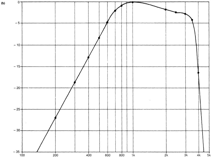
**Telephony signal conditioning** is a snap with this switched-capacitor filter IC (a). Meeting C Message standards, the circuit allows you to measure a voice channel's signal-to-noise ratio, harmonic distortion and idle-channel noise. A 5-pole elliptic characteristic (b) rolls off sharply above 4 kHz.
