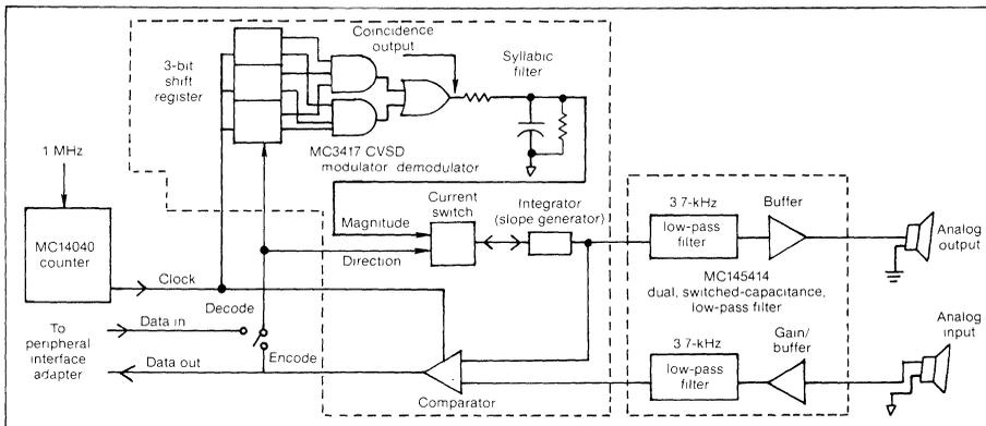
**1. At the heart of a three-chip speech peripheral is an MC3417 continuously variable-slope delta modulator-demodulator, which converts an audio waveform into a serial bit stream. The second and newest of the three is an MC145414 dual switched-capacitor low-pass filter with on-board operational amplifiers. An MC14040 12-bit binary counter completes the trio.**
