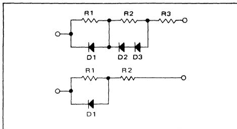
If the performance of more complex diode networks is desired, the circuit in Figure 18 should be used. It simulates the companding characteristics of nonlinear  $R_x$  elements in a different manner.
