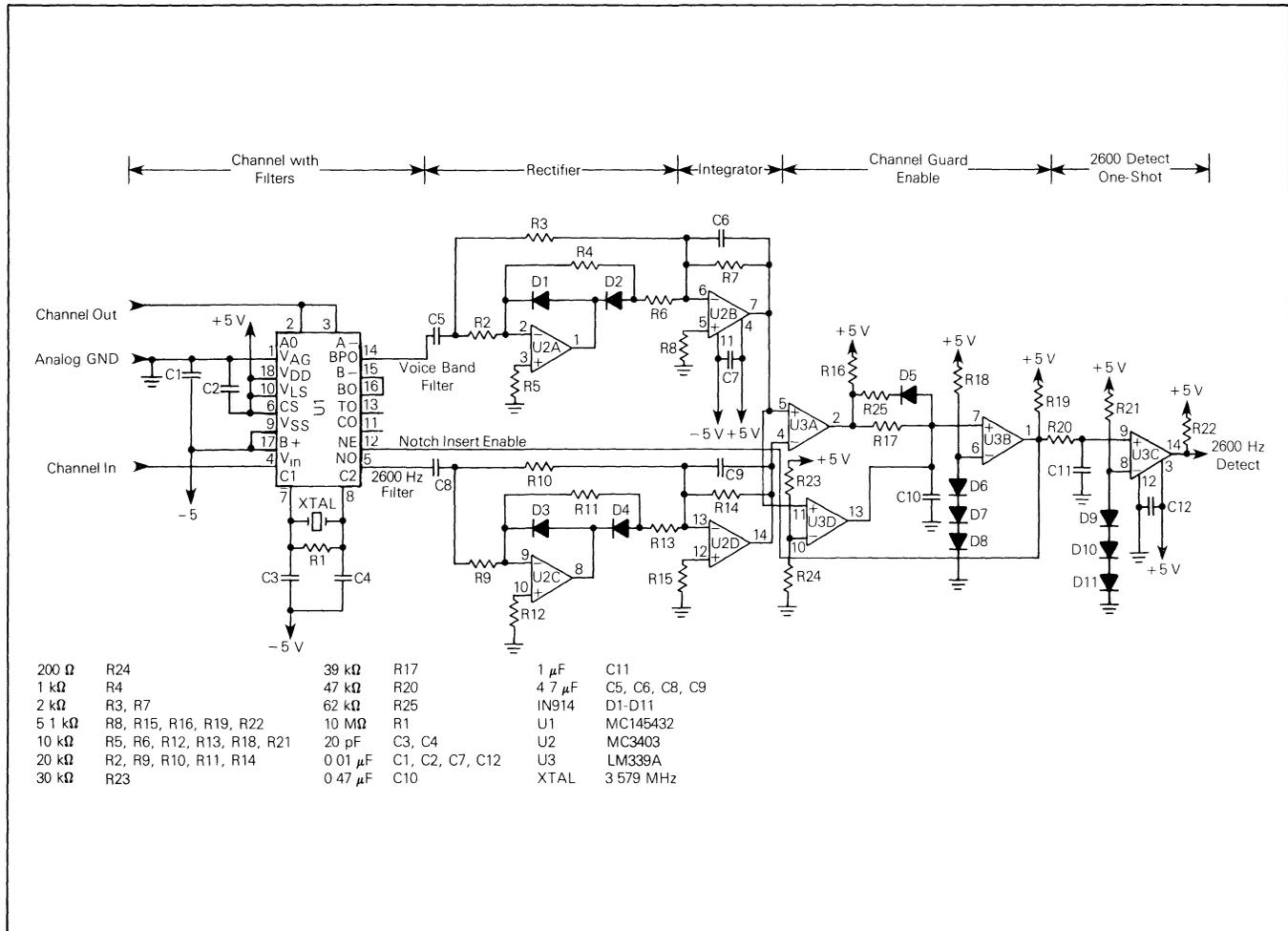
FIGURE 1 — 2600 Hz Guard and Channel Circuit
