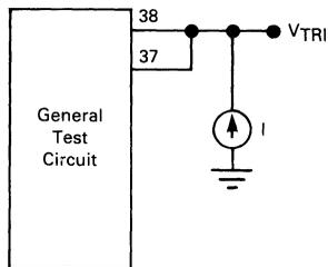
Set  $I = 1.0 \text{ mA}$  and measure  $V_{TRI}$ .
