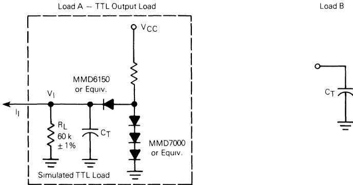
$C_T = 20 \text{ pF}$  = total parasitic capacitance, which includes probe, wiring, and load capacitances
