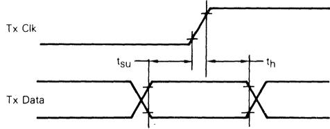
Note: Timing measurements are referenced to and from a low voltage of 0.8 volts and a high voltage of 2.0 volts, unless otherwise noted.
