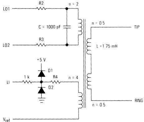
Figure 8. Transformer Configuration Used in LDM Schematic
