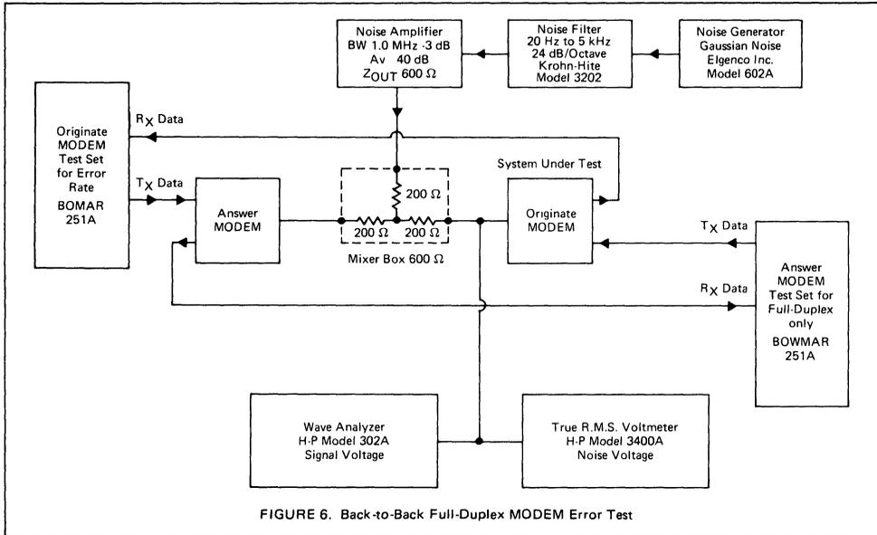
FIGURE 6. Back-to-Back Full-Duplex MODEM Error Test
