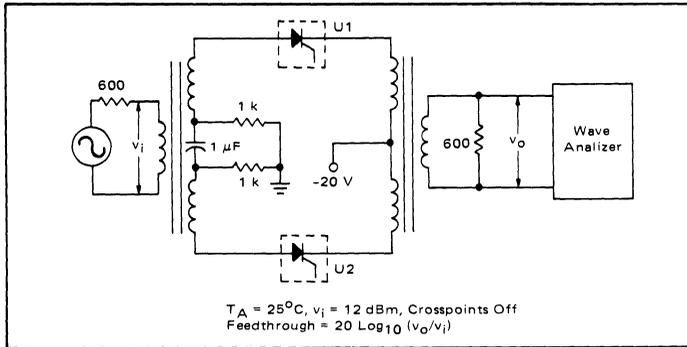
FIGURE 19 – TEST CIRCUIT FOR CROSSTALK versus FREQUENCY
