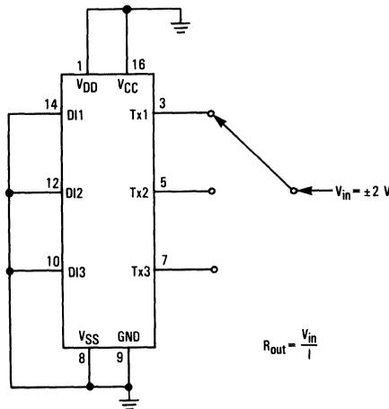
Figure 1. Power-Off Source Resistance (Drivers)
