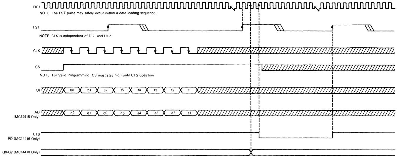
NOTE For the MC14416, the CTS line is pulled low by the device selected by the CS pin
