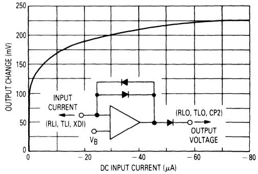
FIGURE 8 — LOG AMP TRANSFER CHARACTERISTICS
