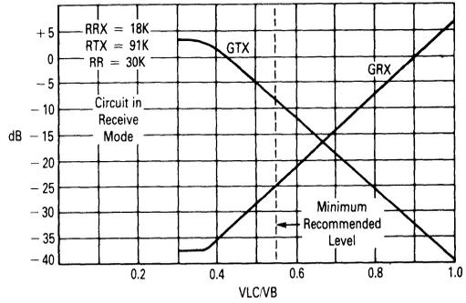
FIGURE 6 — ATTENUATOR GAIN versus ΔVacf
