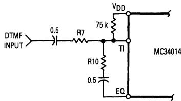
Figure 5. Alternate Biasing
