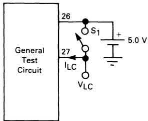
With  $S_1$  open measure  $V_{LC}$ .
