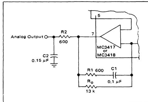
These component values are for the telephone channel circuit poles described in the text. The  $R_2, C_2$  product can be provided with different values of  $R$  and  $C$ .  $R_2$  should be chosen to be equal to the termination resistor on pin 1.
