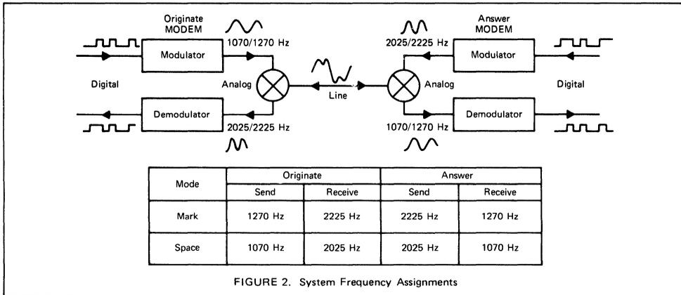
FIGURE 2. System Frequency Assignments
