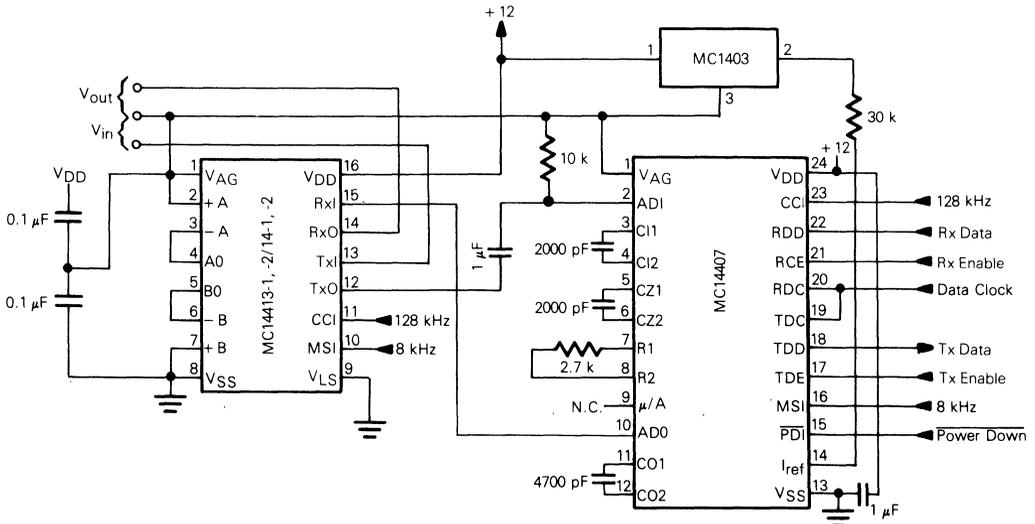
\*Keep all capacitors as near to device pins as possible.
