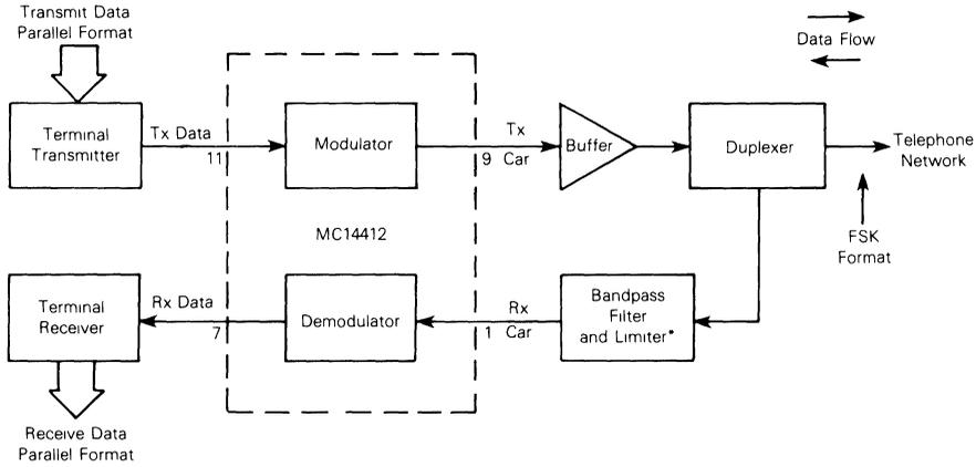
Since the modulator and demodulator sections of the MC14412 are functionally equivalent to those of the MC6860, additional application information can be obtained from the following Motorola publications:
