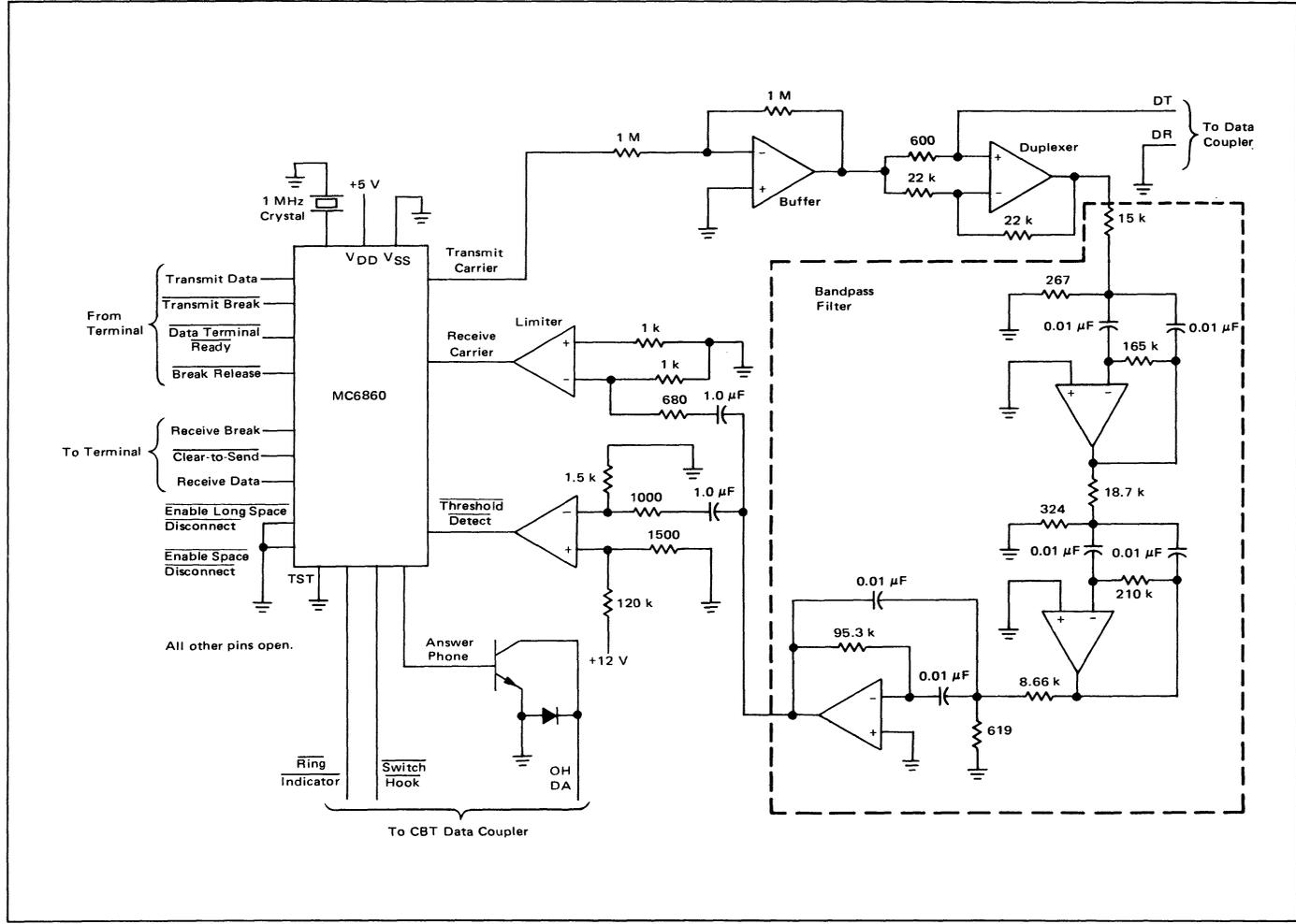
FIGURE 9 - Originate Modem
