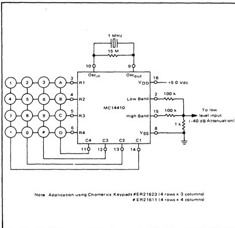
FIGURE 6 – BATTERY POWERED OPERATION (Driving Audio Speaker)
