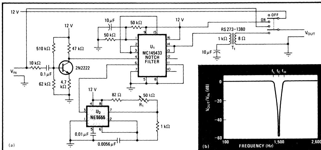
**Filtering.** Motorola's switched-capacitor notch filter MC145433 is switched by adjustable clock  $U_2$  to provide a tunable audio notch filter (a). This notch filter has a frequency response of about 100 Hz to 2.6 kHz (b) and can operate with voltages from +10 to +15 V dc. Transistor  $Q_1$  improves the circuit's signal-to-noise ratio, while audio transformer  $T_1$  drives an 8-ohm load.
