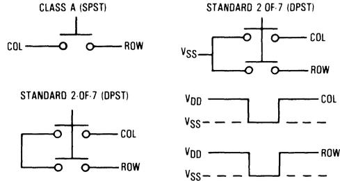
Figure 1. Keyboard Configurations
