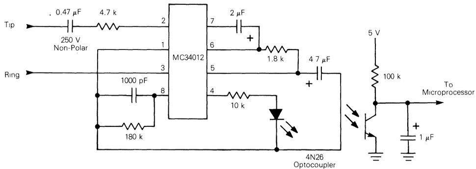
FIGURE 1 — Ring Detector Schematic
