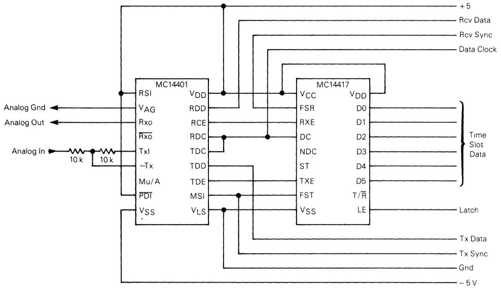
The MC14417 TSAC offers simple flexible time slot assignment for the PCM mono-circuit. Assignments are wired or latched into the data port. The MC14401 offers supply flexibility of  $\pm 5$ ,  $\pm 6$ ,  $+12$ , or  $+10$  V with 18 pin packages and TTL compatibility.
