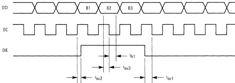
NOTE When  $CM = 0$ , data bits are read into the DSI's SYNCHRONOUS CHANNEL RECEIVER at the DCI pin on the falling edge of the signal formed by the LOGICAL NAND of  $\overline{DC}$  and DIE
