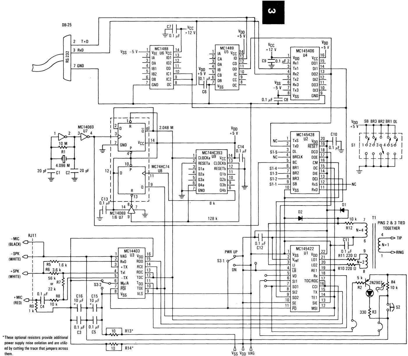
\*These optional resistors provide additional power supply noise isolation and are utilized by cutting the trace that jumpers across them.
