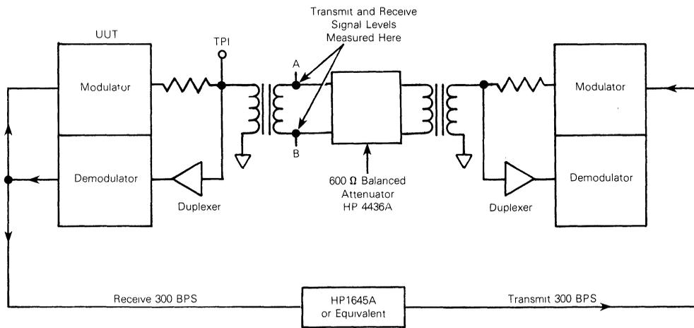
FIGURE 7 — Test Set-Up
