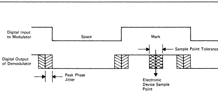
FIGURE 5. Demodulator Data Bit Output
