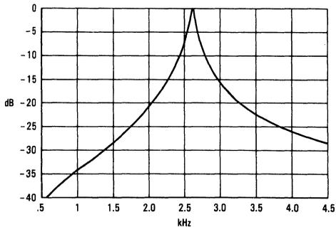
FIGURE 4 — Notch Frequency Response
