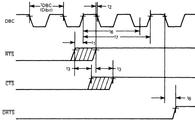
A positive transition of  $\overline{\text{RTS}}$  after  $\overline{\text{CTS}}$  has become active can result in different functional characteristics of the  $\overline{\text{CTS}}$  and  $\overline{\text{DRTS}}$  output signals, depending on the time duration that  $\overline{\text{RTS}}$  remains inactive.
