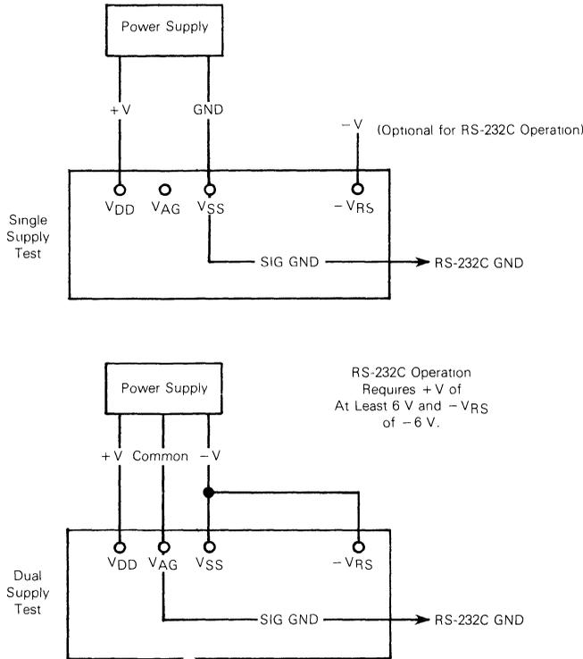
FIGURE 5 — Power Supply Set-Up
