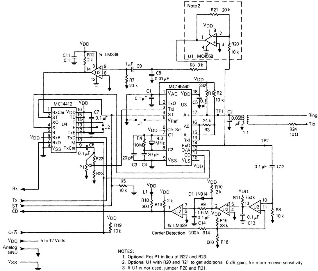
FIGURE 8 — Modem 1 Board MC145440/MC14412
