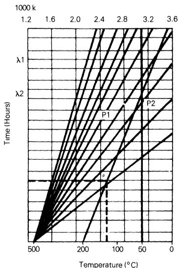
For increased flexibility in working with a broad range of device hours, the time-temperature regression lines have been normalized to 500°C and the time scale omitted, permitting the user to define the scale based on his own requirements.
