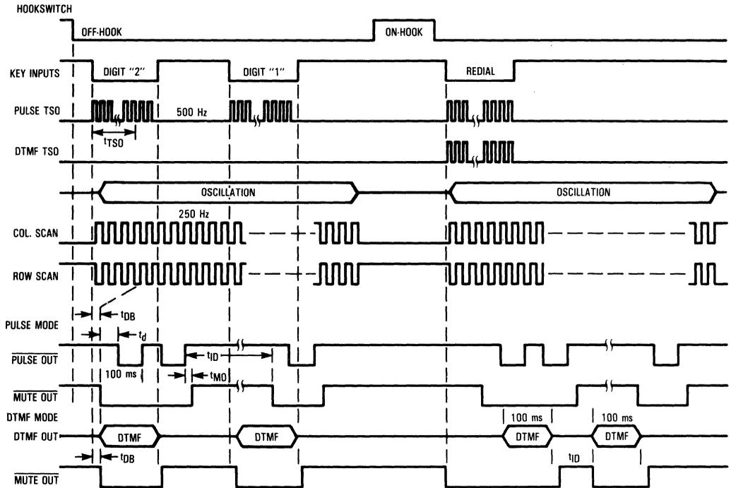
Figure 2. Timing Diagram
