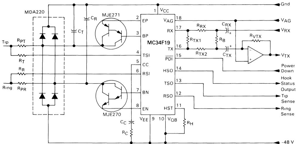
The line-feed current flows between ground and  $V_{EE}$ ; however, the control electronics is referenced to  $V_{QB}$  and ground. Therefore, the dc feed resistance appears to be referenced to  $V_{QB}$  and ground.
