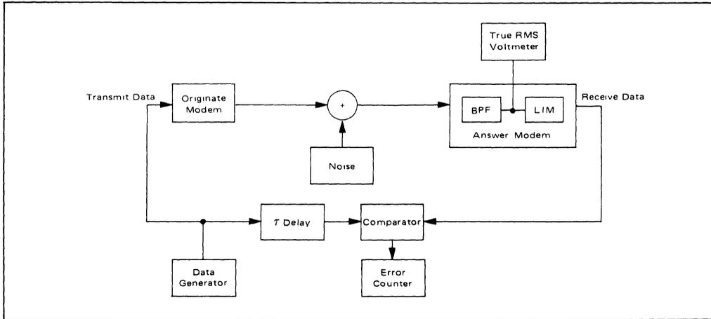
FIGURE 16 – Modem Test Equipment Configuration
