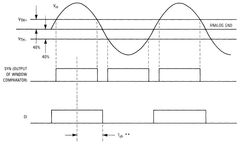
\*\* $T_{sh}$  - SYN should be high a minimum of three 4 096 MHz clock periods before the first zero crossing as indicated by DI state change
