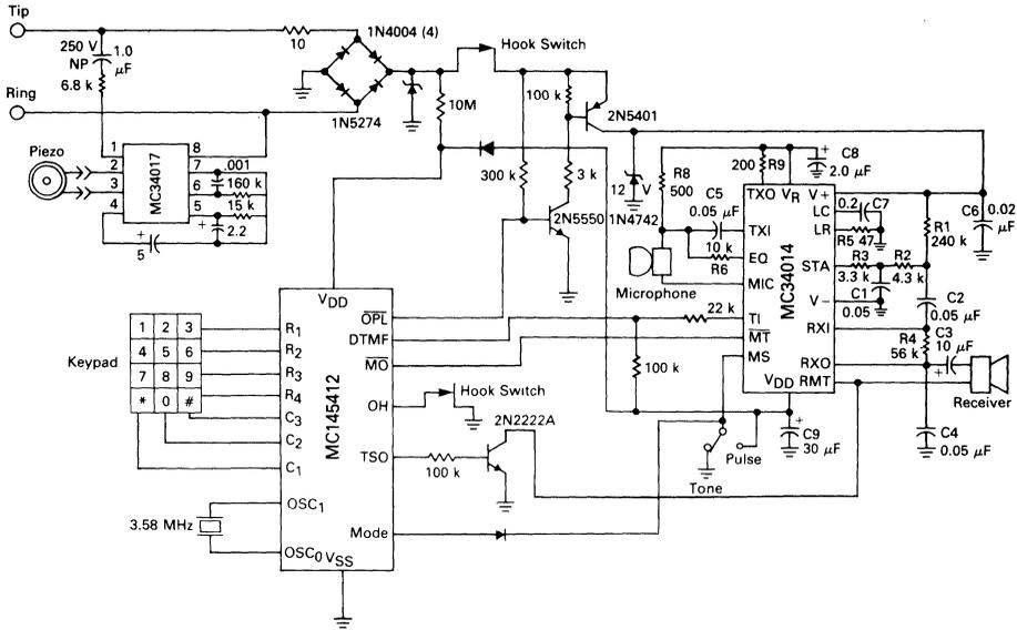
FIGURE 22 — COMPLETE TELEPHONE WITH PULSE DIALING
