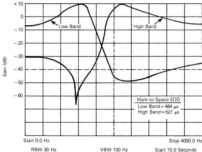
FIGURE 2 — Frequency Response of High Band and Low Band of MC145440
