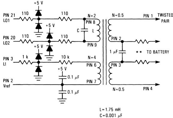
\*\* Battery Feed limiting resistors. (optional)
