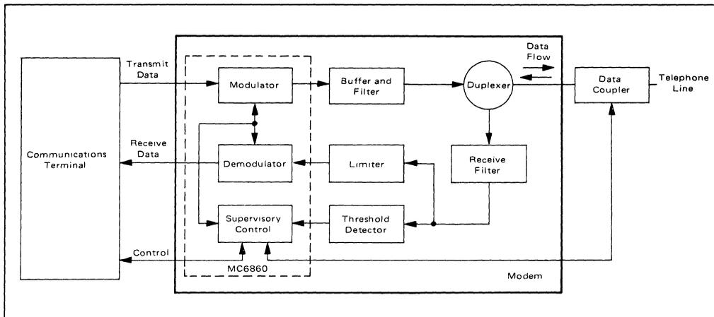
FIGURE 1 – Low-Speed Modem and Interconnections
