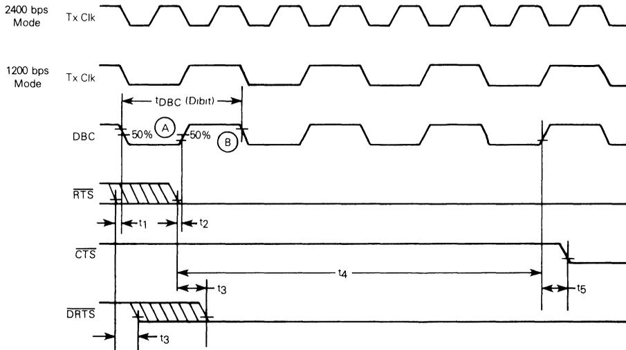
$\overline{\text{RTS}}$ -CTS delay options are selected by the CTS1 and CTS2 inputs, and are stated as time delay interval  $t_4$ . An RTS input signal synchronized about point A will synchronize CTS with the positive transition of DBC (Dibit Clock). Delay  $t_4$  is measured with respect to the negative transition of RTS.
