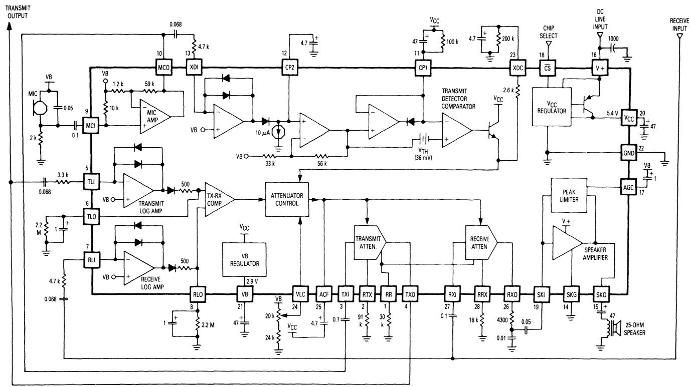
Figure 2. MC34018 Speakerphone Circuit
