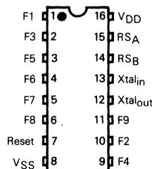
This device contains circuitry to protect the inputs against damage due to high static voltages or electric fields; however, it is advised that normal precautions be taken to avoid application of any voltage higher than maximum rated voltages to this high impedance circuit. For proper operation it is recommended that  $V_{in}$  and  $V_{out}$  be constrained to the range  $V_{SS} \leq (V_{in} \text{ or } V_{out}) \leq V_{DD}$ .
