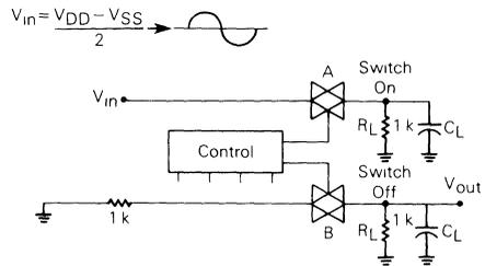
FIGURE 5 — CROSSTALK CONTROL TO OUTPUT
