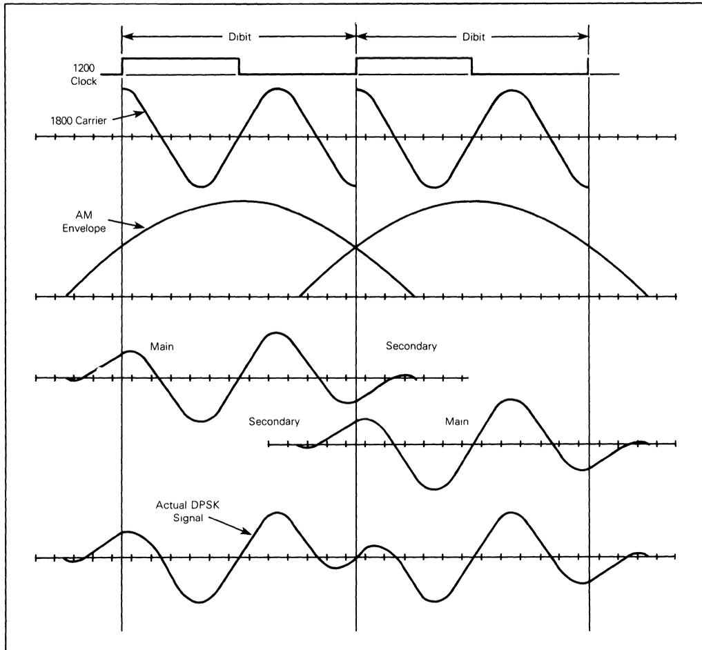
FIGURE 2—DPSK Waveforms
