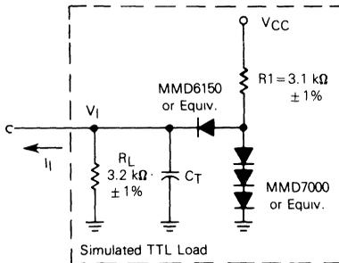
$C_T = 20$  pF = total parasitic capacitance, which includes probe, wiring, and load capacitances.
