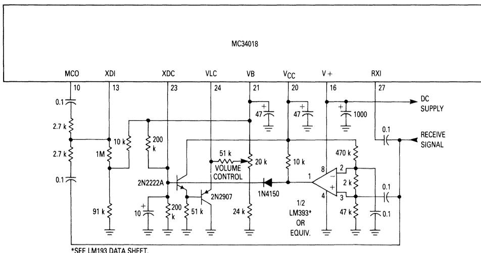
Figure 1. Receive-Idle Circuit
