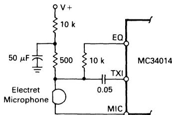
The overall gain from the microphone to  $V+$  will vary with loop current due to the influence of the equalization amplifier on TXI. The signal at EQ is out of phase with that at TXI, therefore the signal at  $V+$  decreases as loop current (and the EQ signal) increases. Variations are typically 2.0 to 5.0 dB and depend largely on the impedance characteristics of the microphone.
