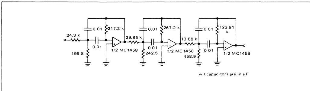
FIGURE 14a – Originate Filter Component Values
