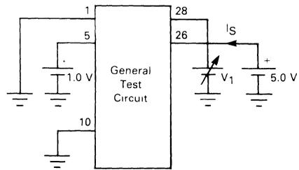
Measure  $I_S$  at  $V_1 = 1.8 \text{ V}$  and  $V_1 = 2.8 \text{ V}$ .
