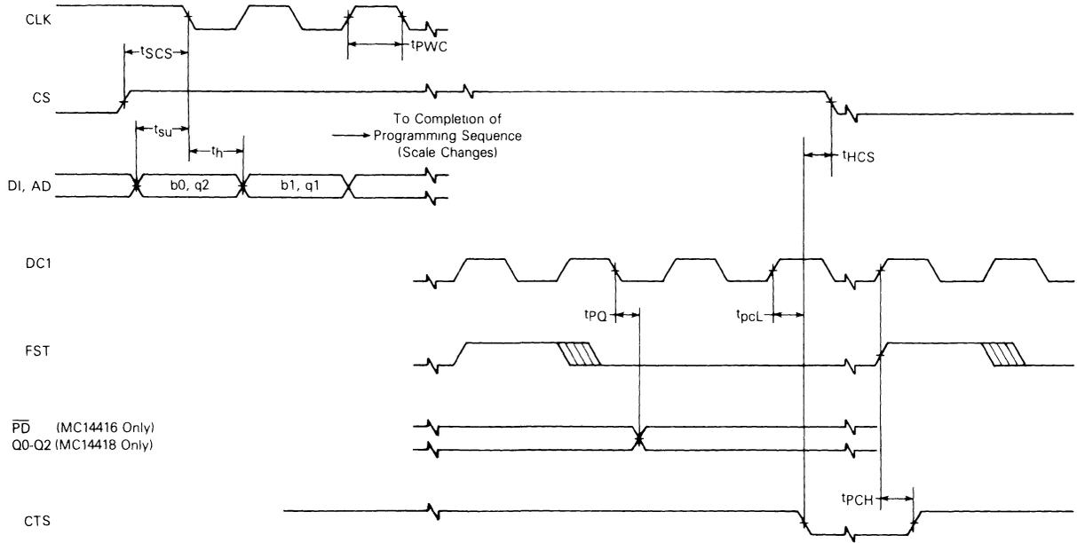
NOTE:  $t_{PCH}$  is measured from the rising edge of the latter of FST or DC1.
