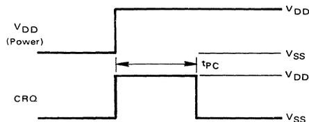
If power is turned off after each call, CRQ must stay high after power is applied (for a duration of t<sub>PC</sub>) to ensure no spurious outputting. For this use the redial function is invalid.
