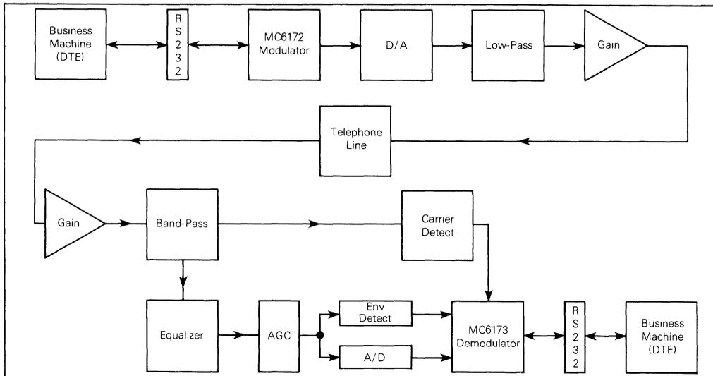
FIGURE 3—MC6172/6173 Modem Block Diagram
