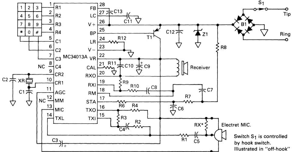
Switch  $S_1$  is controlled by hook switch. Illustrated in "off-hook" condition
