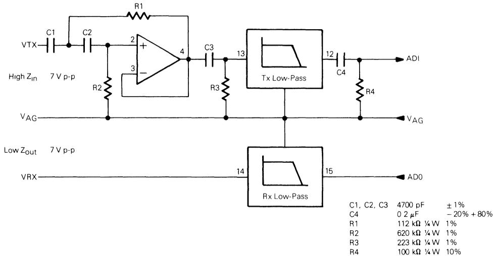
\*In noisy environments, R1-R4 should be 10 k $\Omega$  or less to minimize pickup
