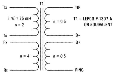
Figure 3. DLT Coupling Transformer
