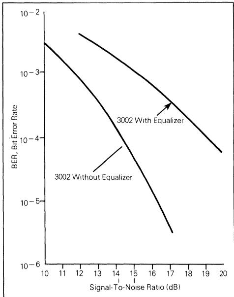
FIGURE 13 — B Mod 2400 BPS 3002 Simulator 511 Test Pattern
