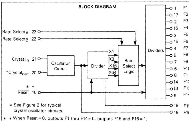
This device contains circuitry to protect the inputs against damage due to high static voltages or electric fields; however, it is advised that normal precautions be taken to avoid application of any voltage higher than maximum rated voltages to this high impedance circuit. For proper operation it is recommended that  $V_{in}$  and  $V_{out}$  be constrained to the range  $V_{SS} \leq (V_{in} \text{ or } V_{out}) \leq V_{DD}$ .
