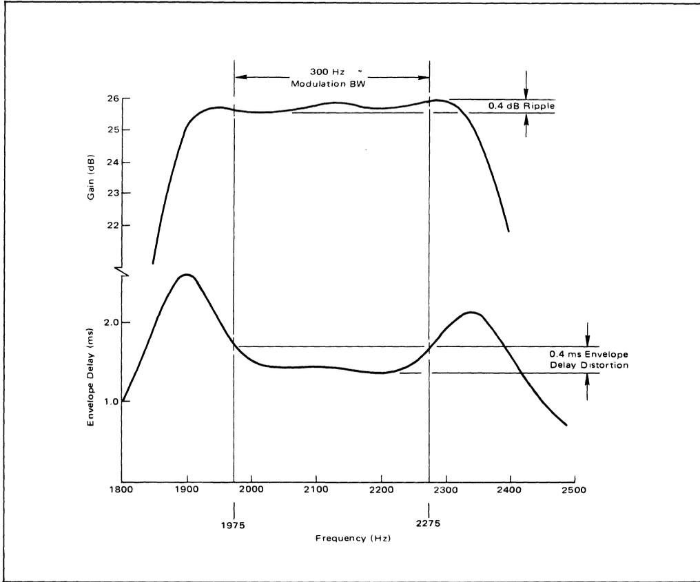
FIGURE 10 – Originate Bandpass Filter Characteristics
