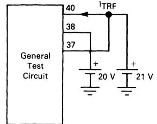
Measure  $I_{TRF}$ . Calculate:  $R_{TRF} = 1.0 \div I_{TRF}$ .
