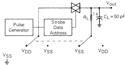
FIGURE 3 — BANDWIDTH AND FEEDTHROUGH ATTENUATION
