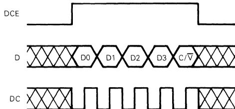
When C/V is "1", D0-D3 are loaded into the configuration register. The four configuration register bits then address a ROM which has outputs to control the analog subsystem elements, enable the appropriate volume register, select the appropriate volume register for the speaker/ringer volume control, and provide the SAE output.
