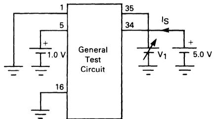
Measure  $I_S$  at  $V_1 = 1.8 \text{ V}$  and  $V_1 = 2.8 \text{ V}$ .
