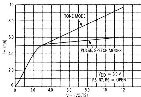
FIGURE 7 — CIRCUIT VOLTAGE versus LOOP CURRENT
