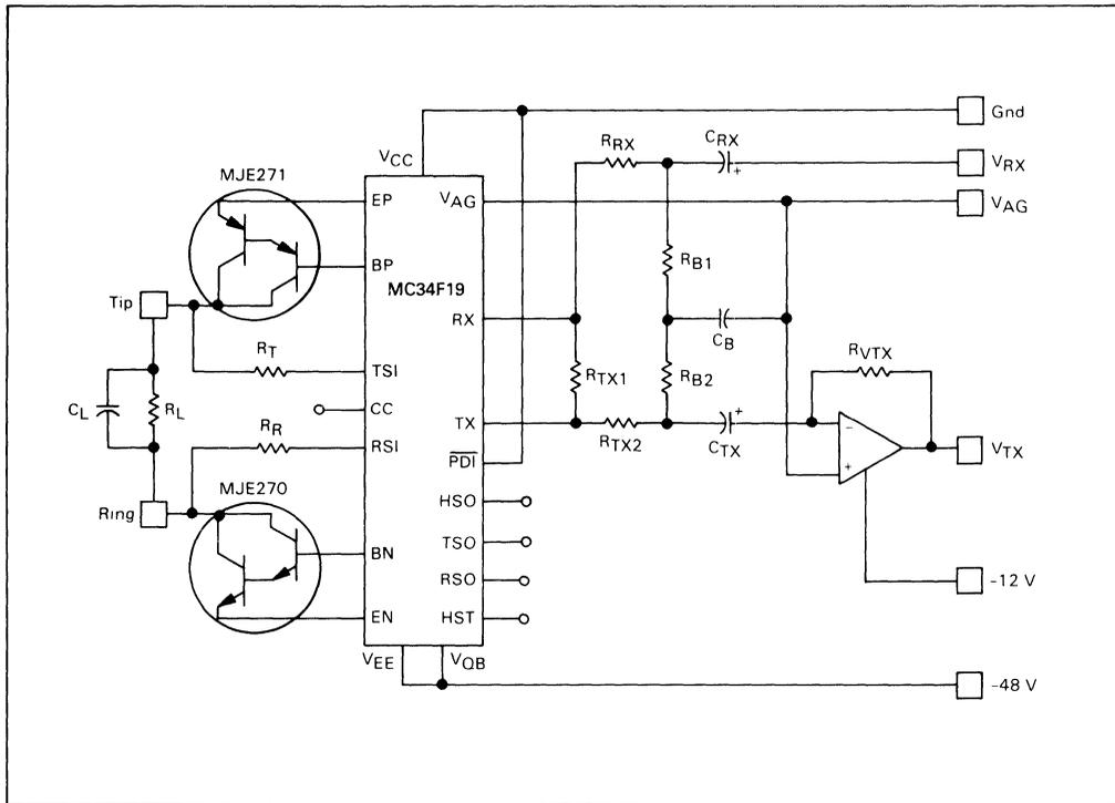
The  $\overline{\text{PDI}}$  pin is designed to be TTL compatible if the logic power supplies are 0 V and -5.0 V. It is also compatible with CMOS powered from 0 V and -12 V supplies, otherwise a level-shifter is required. If the power-down feature is not desired, this pin can be tied to  $V_{CC}$ .
