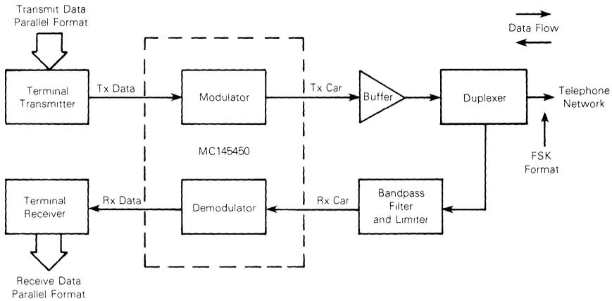
FIGURE 6 — TYPICAL 1200 BAUD 4 WIRE MODEM APPLICATION
