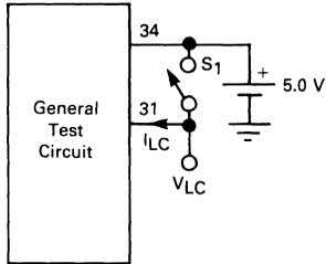
With  $S_1$  open measure  $V_{LC}$ .
