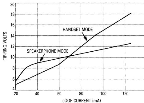
Figure 5. Tip-Ring Voltage versus Loop Current
