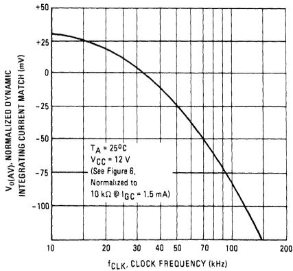
FIGURE 10 – DYNAMIC TOTAL LOOP OFFSET versus CLOCK FREQUENCY
