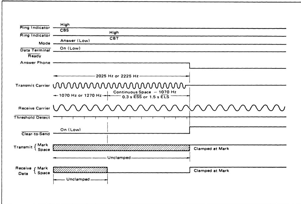
FIGURE 4 - Automatic Disconnect - Long or Short Space
