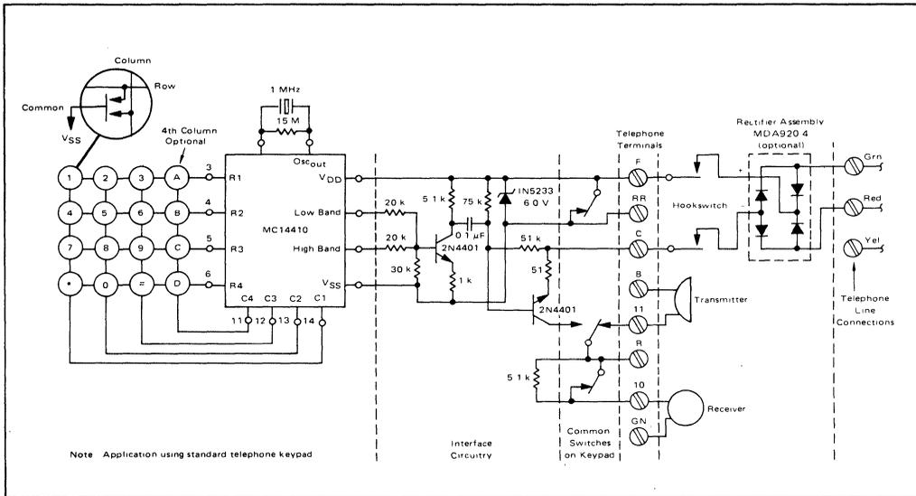
FIGURE 5 – LOW LEVEL OUTPUT TONE GENERATOR APPLICATION
