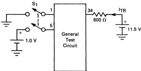
With  $S_1$  open measure  $I_{TR}$ . Close  $S_1$  and again measure  $I_{TR}$ . Calculate:
