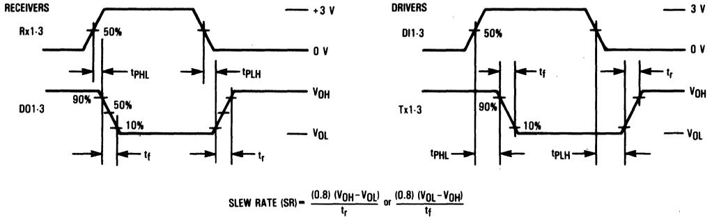
Figure 2. Switching Characteristics
