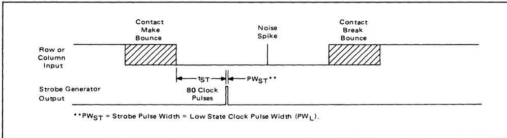
\*\* $PW_{ST}$  = Strobe Pulse Width = Low State Clock Pulse Width ( $PW_L$ ).
