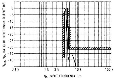
FIGURE 3 — FILTER A AND B LOWPASS CHARACTERISTICS WITH CLOCK 1 AND 2 AT 256 kHz
