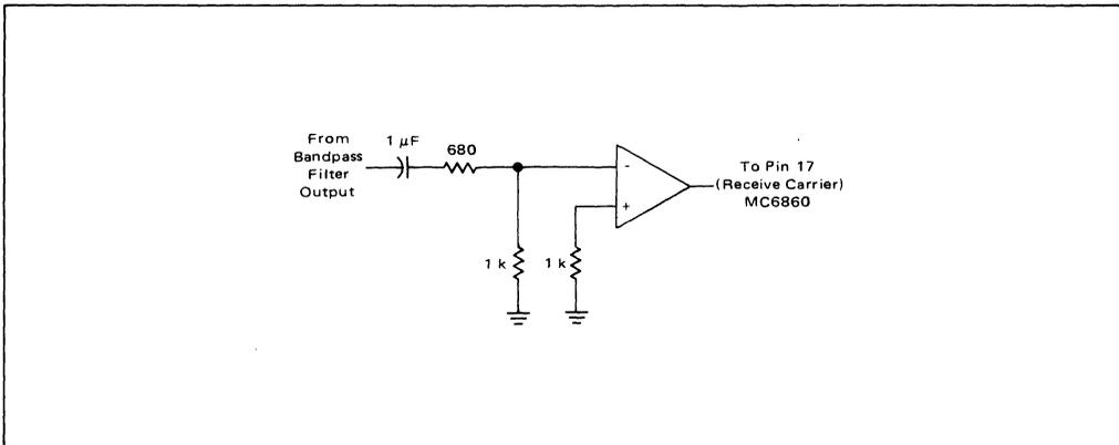
FIGURE 11 – Limiter Schematic
