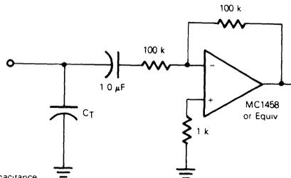
$C_T = 20$  pF = total parasitic capacitance, which includes probe, wiring, and load capacitance
