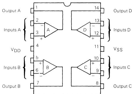
This device contains circuitry to protect the inputs against damage due to high static voltages or electric fields, however, it is advised that normal precautions be taken to avoid application of any voltage higher than maximum rated voltages to this high-impedance circuit. For proper operation it is recommended that  $V_{IN}$  and  $V_{OUT}$  be constrained to the range  $V_{SS} \leq (V_{IN} \text{ or } V_{OUT}) \leq V_{DD}$ .
