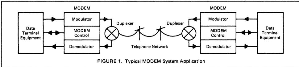
FIGURE 1. Typical MODEM System Application
