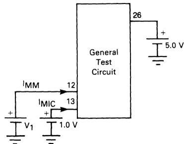
a. Set  $V_1 = 2.0 \text{ V}$  and measure  $I_{MIC}$ .
