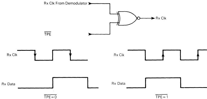
FIGURE 11 — PHASE-SHIFT SELECT DEMULTIPLEXER FOR TEST PATTERN ENABLE
