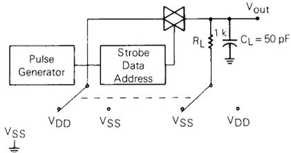
FIGURE 3 – BANDWIDTH AND FEEDTHROUGH ATTENUATION
