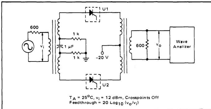
FIGURE 19 – TEST CIRCUIT FOR CROSSTALK versus FREQUENCY
