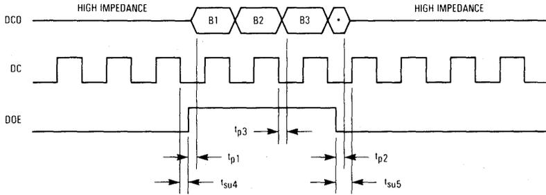
\*This bit will be output in the B1 position on the next cycle of DOE.
