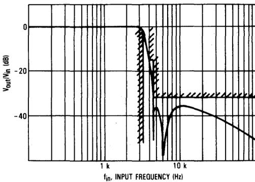
FIGURE 6 — TRANSMIT FILTER TYPICAL AND GUARANTEED PERFORMANCE (MC14414-1, -2)
