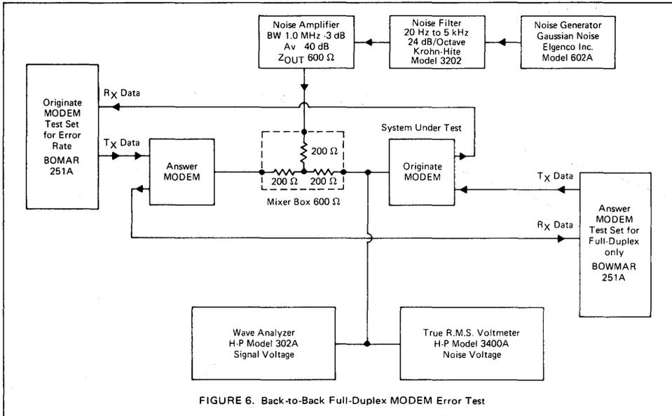
FIGURE 6. Back-to-Back Full-Duplex MODEM Error Test
