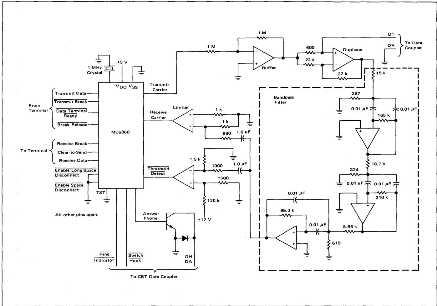
FIGURE 9 - Originate Modem
