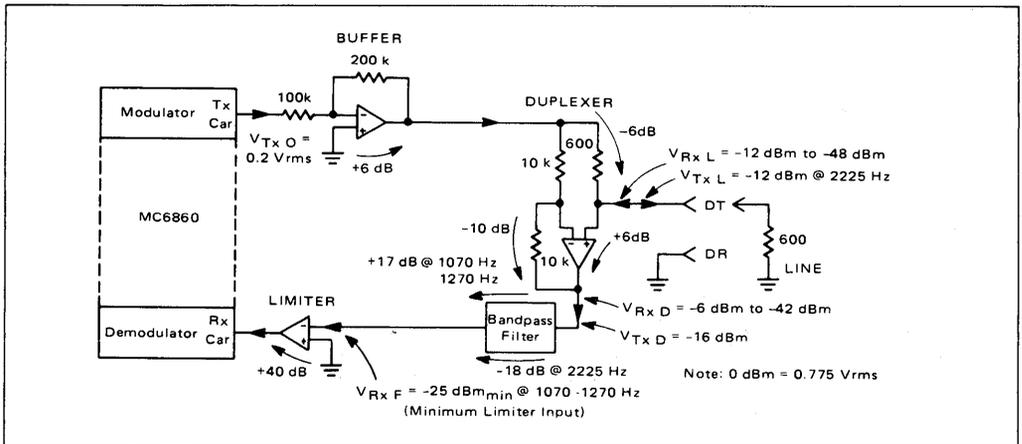
FIGURE 12 – System Level Constraints
