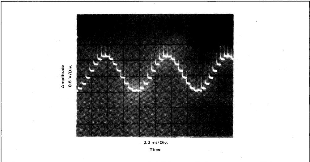
FIGURE 2 – MOS Synthesized 1270-Hz Sine Wave
