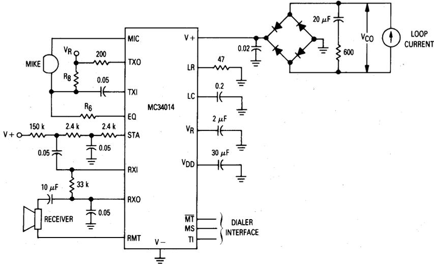
For Primo EM-95A microphone  $R_8 = 500 \Omega$ ,  $R_6 = 10 \text{ k}$
