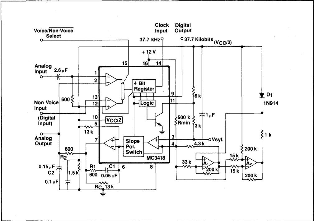
FIGURE 5 — TELEPHONE QUALITY DELTA MODULATOR CODER
