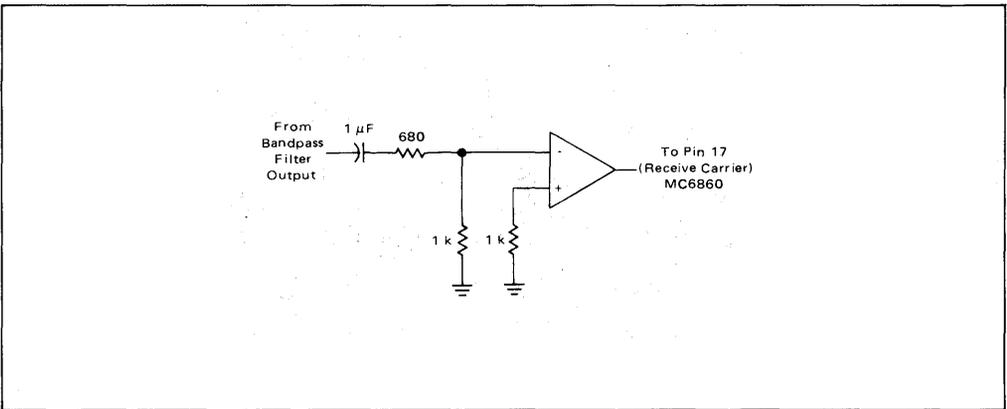
FIGURE 11 – Limiter Schematic
