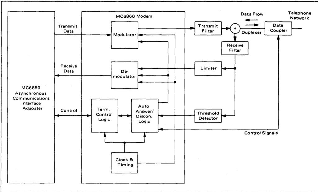
FIGURE 8 – Typical MC6860 Modem System
