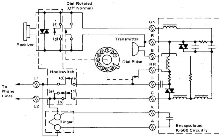
FIGURE 11 — MODIFIED K-500 TELEPHONE
