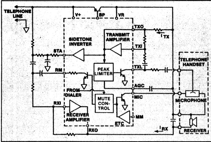
Fig. 4 Speech network block diagram.
