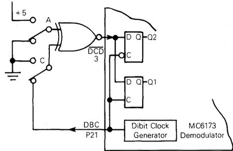
FIGURE 6 — ENVELOPE CLOCK TIMING DIAGRAM
