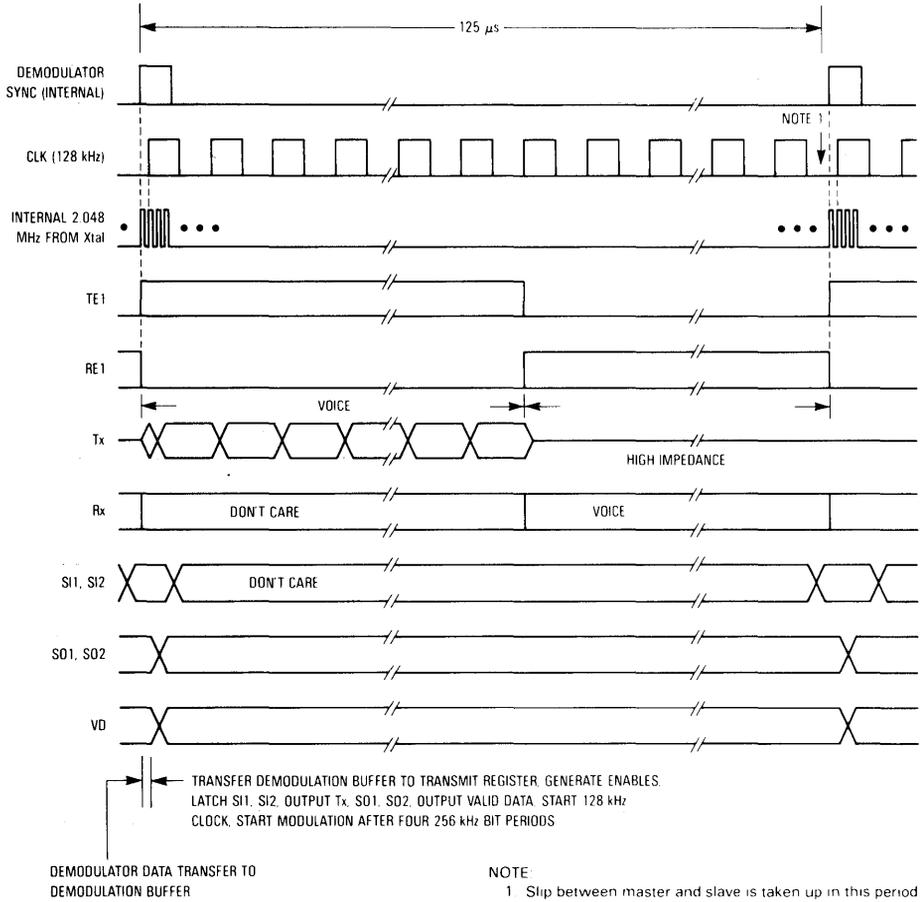
Figure 13. Slave DLT Timing
