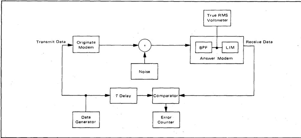
FIGURE 16 – Modem Test Equipment Configuration
