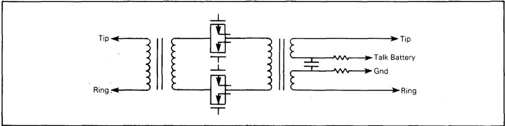
FIGURE 3A — Trunk-to-Station Loop
