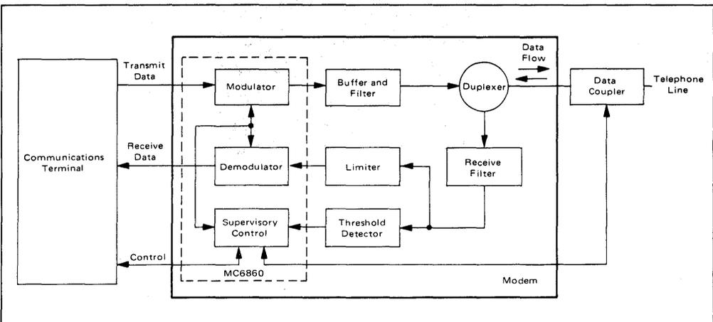
FIGURE 1 - Low-Speed Modem and Interconnections
