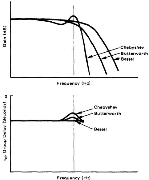
FIGURE 10 – Filter Approximation Characteristics
