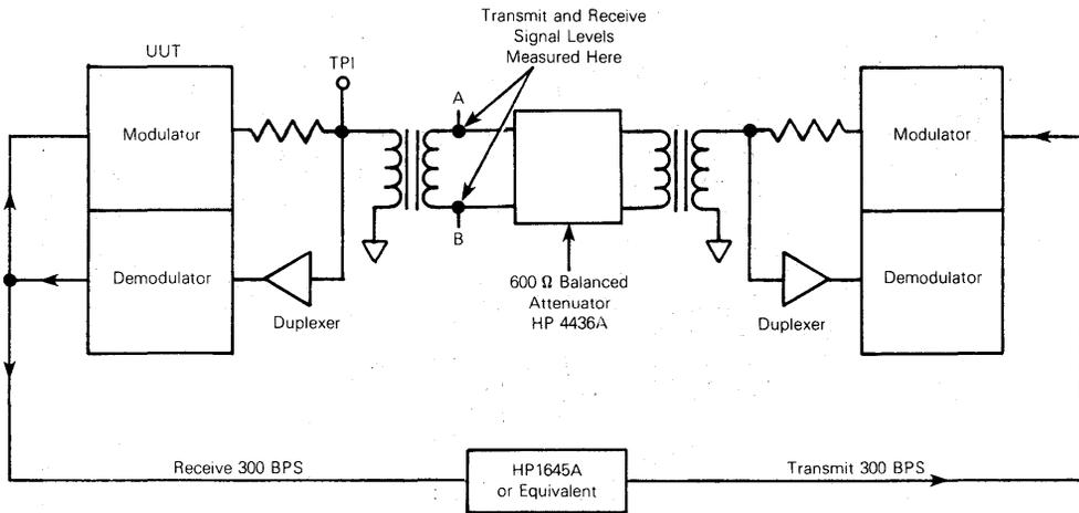
FIGURE 7 — Test Set-Up
