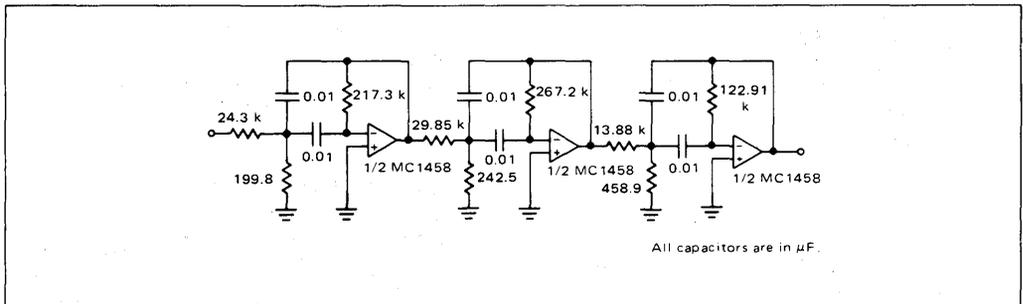
FIGURE 14a – Originate Filter Component Values
