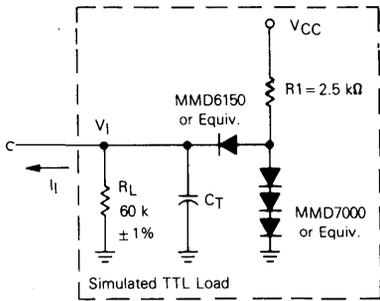
$C_T = 20 \text{ pF}$  = total parasitic capacitance, which includes probe, wiring, and load capacitances.
