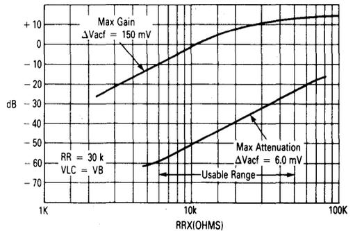
FIGURE 4 — GAIN AND ATTENUATION versus RESISTOR RATIOS
