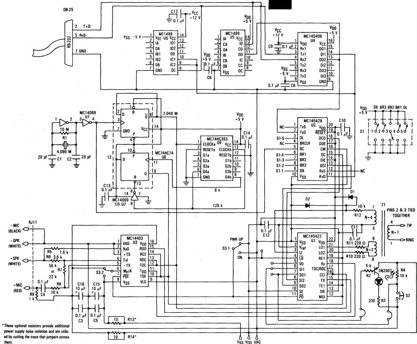
\*These optional resistors provide additional power supply noise isolation and are utilized by cutting the trace that jumpers across them.
