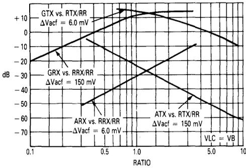
FIGURE 5 — ATTENUATOR GAIN versus VLC/VB
