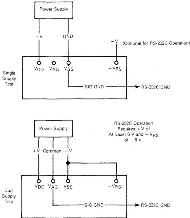
FIGURE 5 — Power Supply Set-Up
