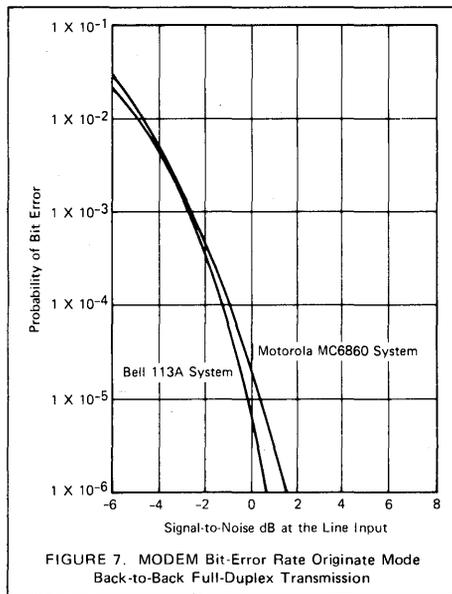
FIGURE 7. MODEM Bit-Error Rate Originate Mode Back-to-Back Full-Duplex Transmission
