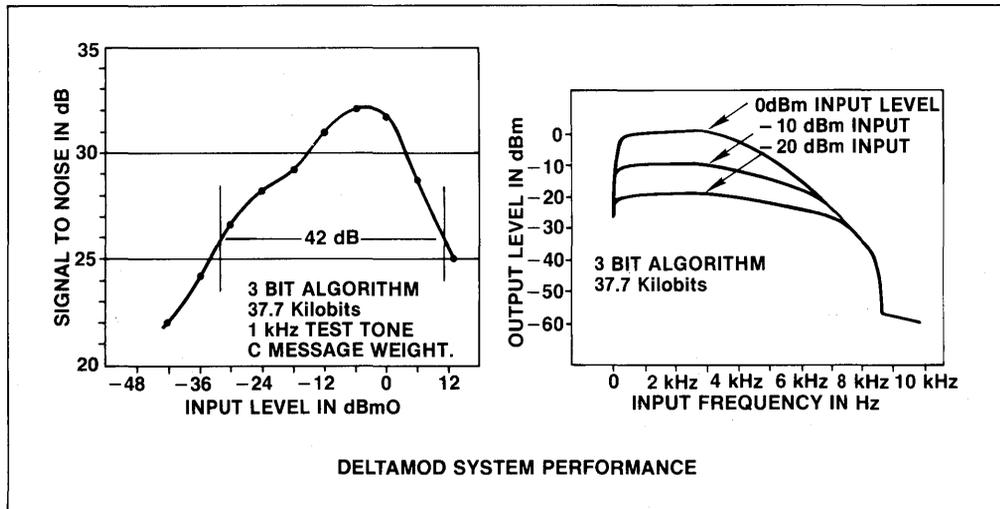
FIGURE 4 — SIGNAL TO NOISE PERFORMANCE AND FREQUENCY RESPONSE
