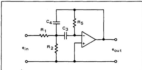
FIGURE 9 – Multiple Feedback Bandpass Filter Element
