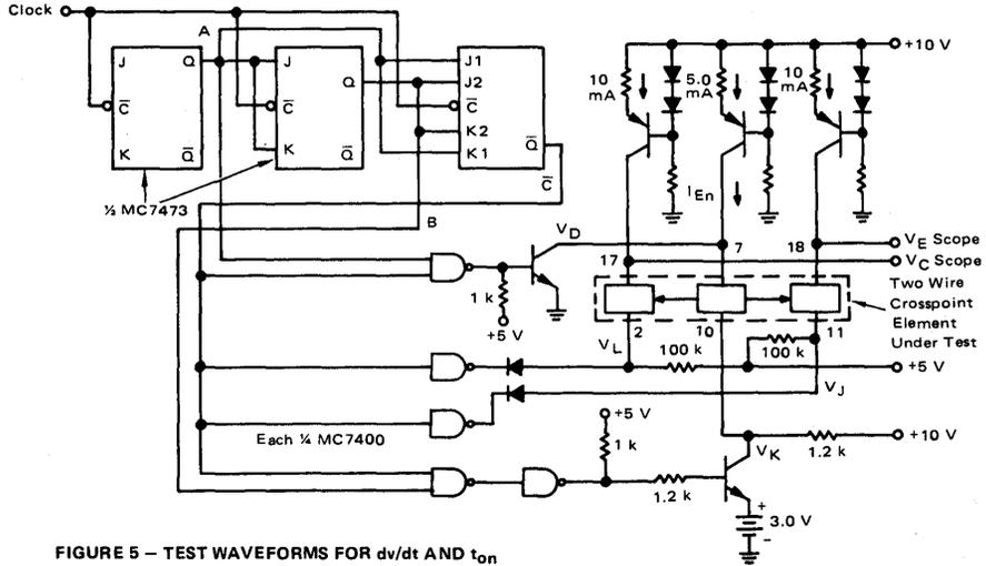
FIGURE 5 – TEST WAVEFORMS FOR  $dv/dt$  AND  $t_{on}$
