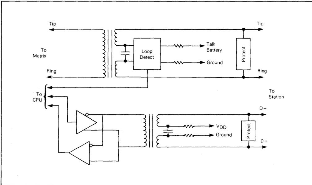
FIGURE 5 — Station Interface (Without Ring Generator)
