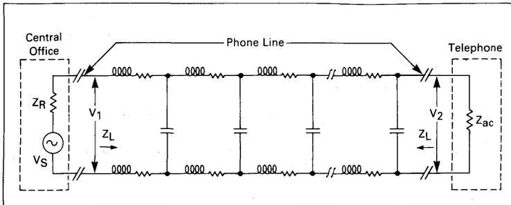
Figure 16 depicts the situation in the transmit mode. In this mode, the MC34014 is an ac current source, with a finite output impedance, modulating the loop current. The voltage signal  $V_1$  is therefore equal to the ac signal current acting on  $Z_{ac}$  in parallel with the characteristic
