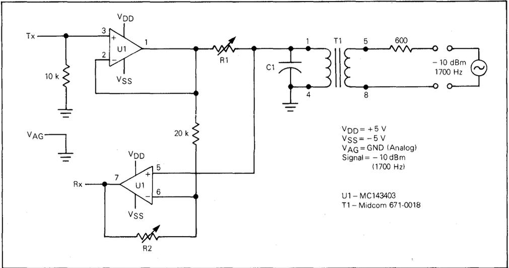
FIGURE 1 — Duplexer Circuit
