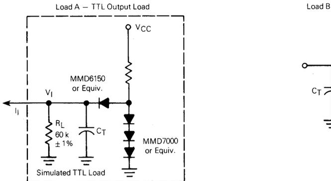
C<sub>T</sub> = 20 pF = total parasitic capacitance, which includes probe, wiring, and load capacitances
