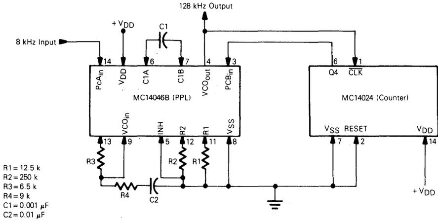
FIGURE 16 — GENERATION OF 128 kHz IN SYSTEM USING 1.544 MHz CLOCK
