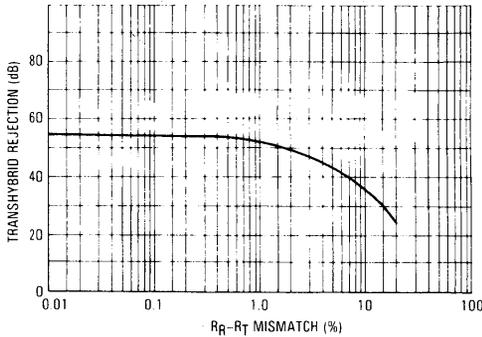
**FIGURE 10 — IMPEDANCE BALANCE versus TIP/RING RESISTOR MISMATCH**
