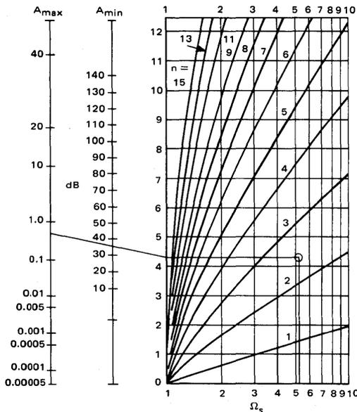
ripple ( $A_{max}$ ), and stopband attenuation ( $A_{min}$ ), to determine the order of the prototype lowpass filter.
