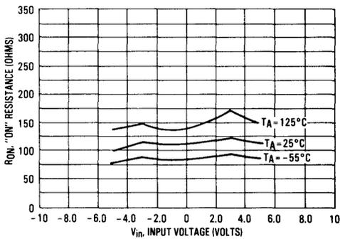
FIGURE 10 —  $V_{DD}=7.5\text{ V}$ ,  $V_{SS}=-7.5\text{ V}$
