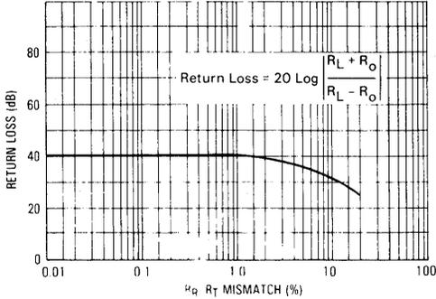
**FIGURE 9 — TRANSHYBRID REJECTION versus TIP/RING RESISTOR MISMATCH**
