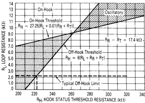
Figure 11 shows such a graph using 17.4 kΩ as the values for  $R_R$  and  $R_T$ . Note the oscillatory condition to the right of the crossing point. Selection of  $R_H$  in this region is usually not a problem since the majority of telephone lines do not fall into this resistance range.  $R_H$  always ties to  $V_{QB}$  and HST and will give reliable hook status information regardless of power supply voltages and PDI.
