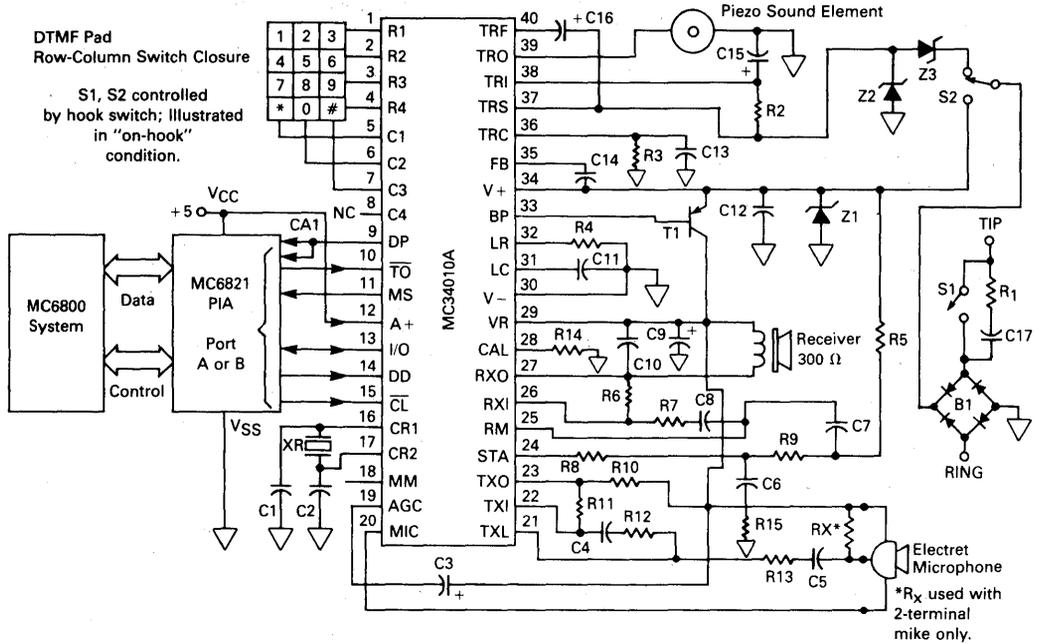
FIGURE 48 — MC34011A ELECTRONIC TELEPHONE APPLICATION CIRCUIT
