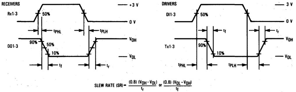
Figure 2. Switching Characteristics
