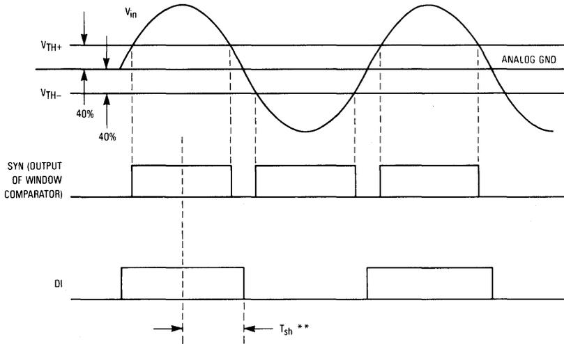
\*\*T<sub>sh</sub> - SYN should be high a minimum of three 4.096 MHz clock periods before the first zero crossing as indicated by DI state change.
