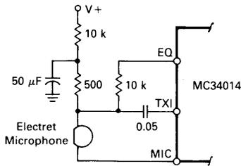
The overall gain from the microphone to  $V+$  will vary with loop current due to the influence of the equalization amplifier on TXI. The signal at EQ is out of phase with that at TXI, therefore the signal at  $V+$  decreases as loop current (and the EQ signal) increases. Variations are typically 2.0 to 5.0 dB and depend largely on the impedance characteristics of the microphone.
