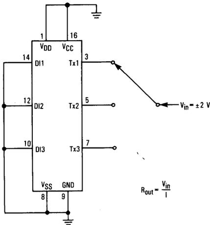
Figure 1. Power-Off Source Resistance (Drivers)
