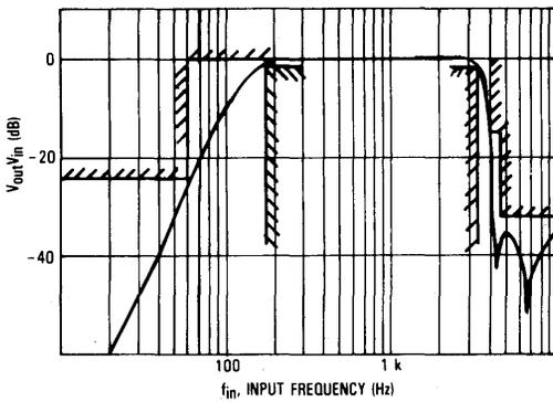
FIGURE 4 — TRANSMIT FILTER TYPICAL AND GUARANTEED PASS-BAND PERFORMANCE (MC14413-1, -2 AND MC14414-1, -2 USING FIGURES 10 AND 11)
