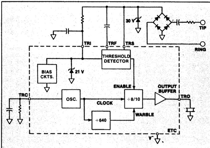
Fig. 5 Tone ringer block diagram.
