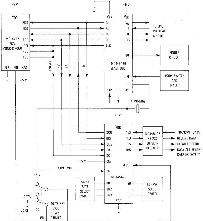
NOTE: Some pin connections on the MC145426 and MC14402 have been omitted. Consult MC145426 and MC14402 data sheets for more details.
