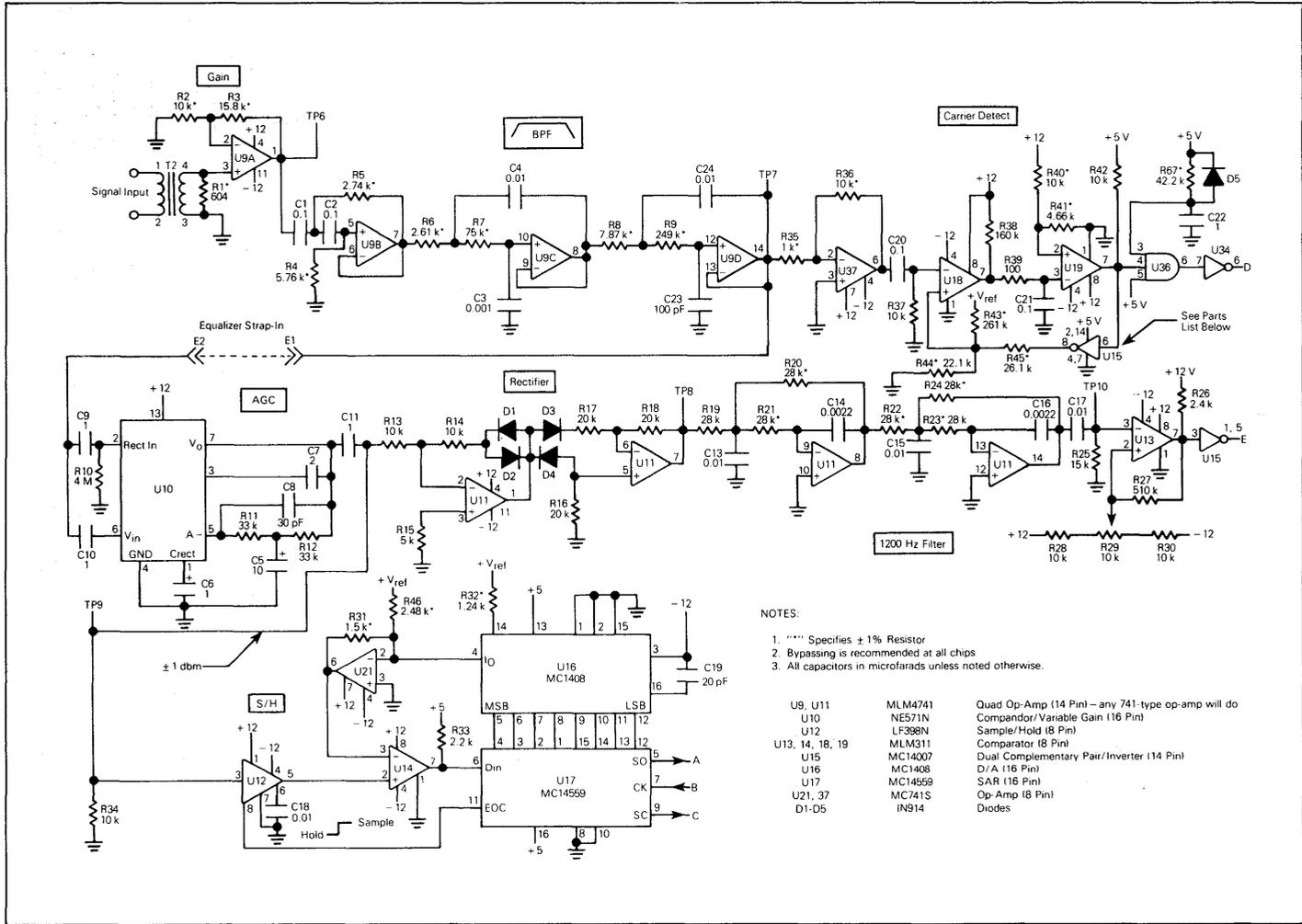
FIGURE 5 — 2400 BPS DPSK Demodulator (1 of 2)
