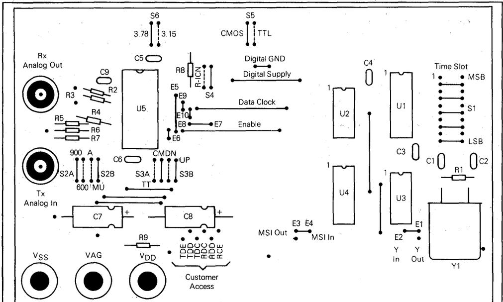
NOTE: Solid line indicates normal strapping as shipped from factory; dashed lines indicate optional straps as described below in the Strapping Information Chart.
