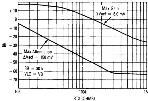
FIGURE 3 — RECEIVE ATTENUATOR versus RRX
