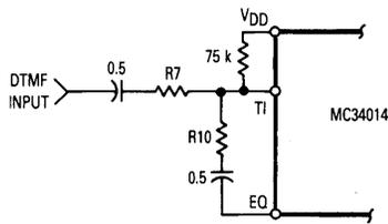
Figure 5. Alternate Biasing
