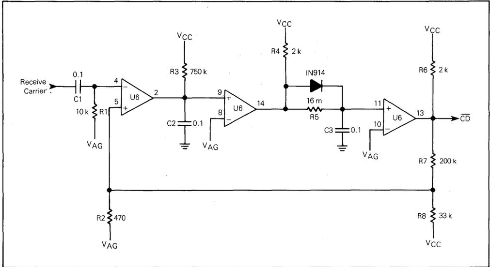
FIGURE 2 — CARRIER DETECT
