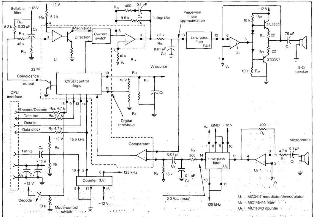
**3. A continuously variable slope gives the MC3417 the accuracy to reproduce analog signals. When necessary, the syllabic filter varies the rate of integration and with it the slope. The three basic chips, a simple audio amplifier, and a microprocessor interface complete the speech peripheral circuit.**
