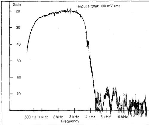
**2. The switched-capacitor low-pass filter limits both input and output frequencies to about 3.7 kHz, as reflected by the system frequency response curve. Input frequencies are limited to prevent aliasing; filtering the output smooths it out. Bandwidth for the circuit ranges from 500 Hz to 3.7 kHz.**
