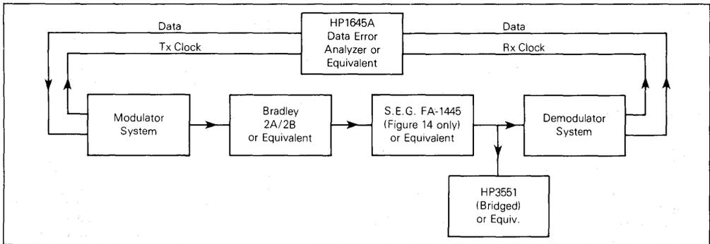
FIGURE 9 — Equipment Setup
