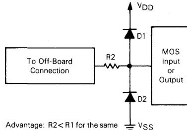
Advantage: R<sub>2</sub> < R<sub>1</sub> for the same level of protection. Impact on ac and dc characteristics is minimized.
