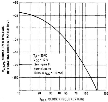
FIGURE 10 – DYNAMIC TOTAL LOOP OFFSET versus CLOCK FREQUENCY
