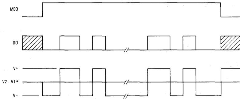
\*See Figure 14 for voltages V2, V1. |V+| must equal |V-| within 5%.
