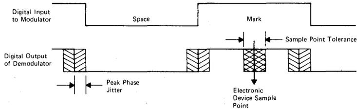
FIGURE 5. Demodulator Data Bit Output
