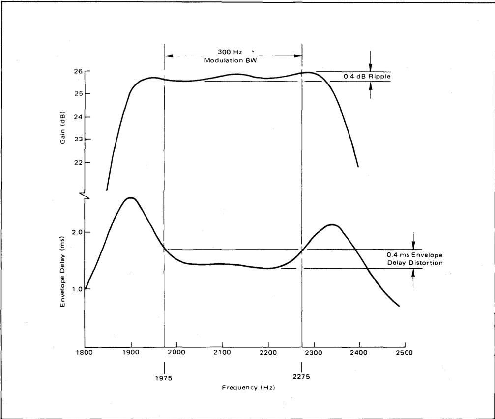
FIGURE 10 – Originate Bandpass Filter Characteristics
