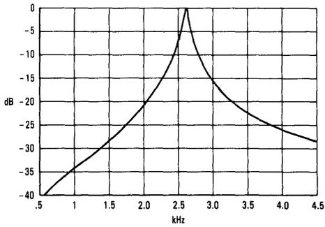
FIGURE 4 — Notch Frequency Response
