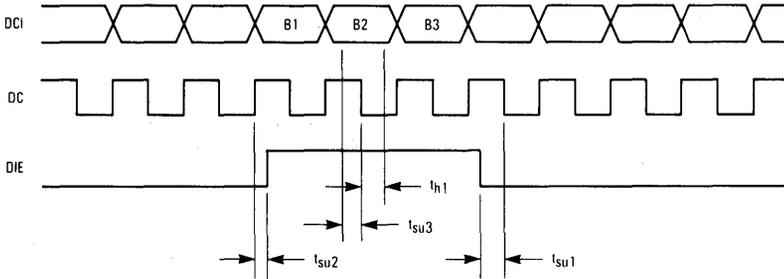
NOTE: When  $CM = 0$ , data bits are read into the DSI's SYNCHRONOUS CHANNEL RECEIVER at the DCI pin on the falling edge of the signal formed by the LOGICAL NAND of  $\overline{DC}$  and DIE, i.e.  $\psi$  of  $\overline{DC} \bullet DIE$ .
