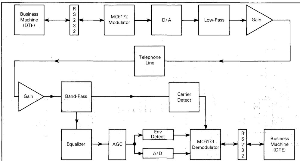
FIGURE 3—MC6172/6173 Modem Block Diagram
