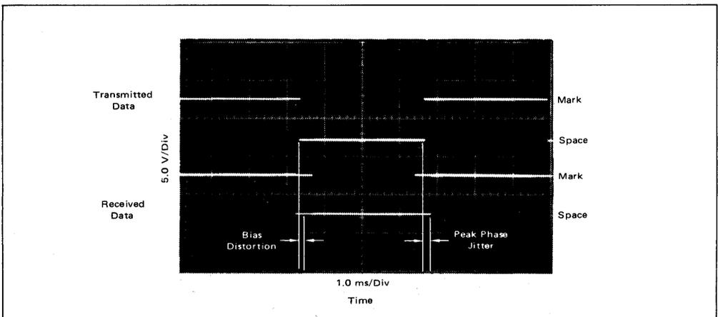
FIGURE 12 – Bias Distortion and Phase Jitter at Demodulator Output
