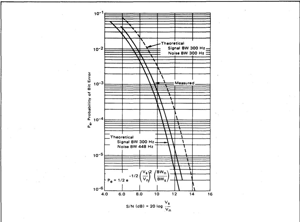
FIGURE 18 – System Performance with Gaussian Noise
