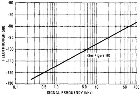
FIGURE 17 – CROSSTALK versus SIGNAL FREQUENCY
