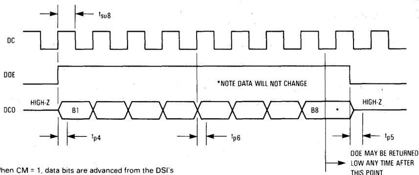
NOTE: When CM = 1, data bits are advanced from the DSI's SYNCHRONOUS CHANNEL TRANSMITTER at the DCO pin on the rising edge of the signal formed by the LOGICAL AND of DC and DOE. (DC • DOE)
