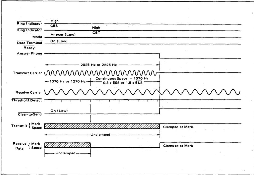
FIGURE 4 - Automatic Disconnect - Long or Short Space
