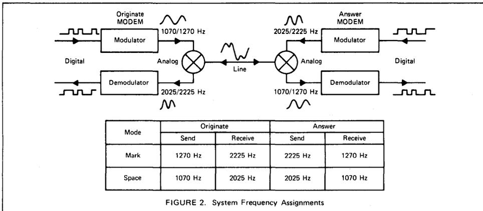
FIGURE 2. System Frequency Assignments
