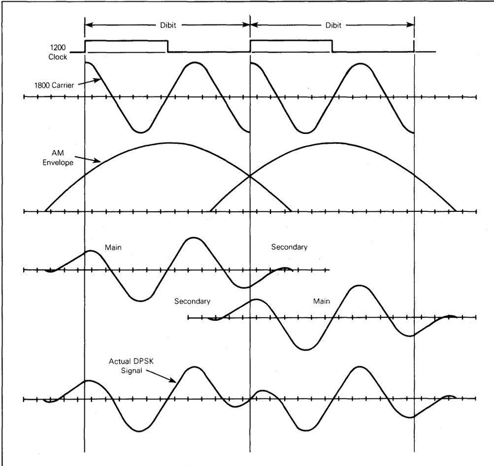
FIGURE 2—DPSK Waveforms
