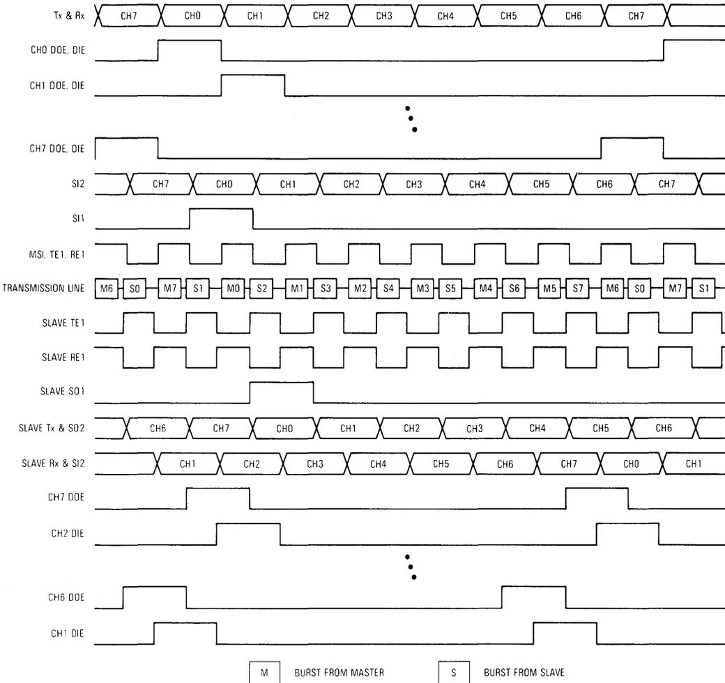
Figure 9. System Timing
