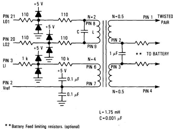
Figure 4. Application Circuit For the Transformer Interface
