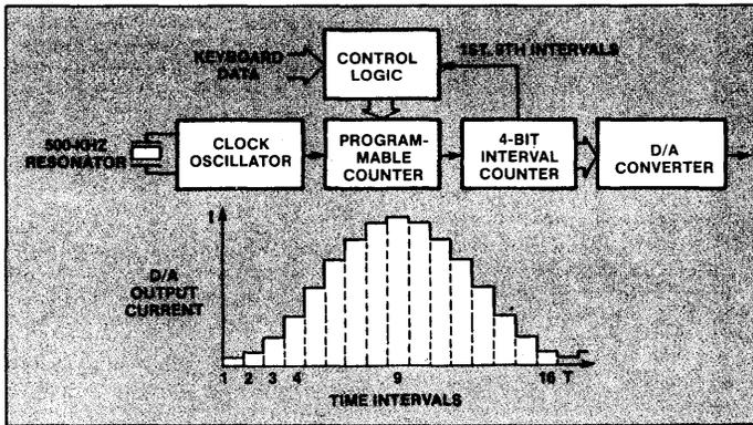
Fig. 2 The DTMF frequency synthesis technique.
