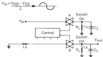
FIGURE 5 – CROSSTALK CONTROL TO OUTPUT
