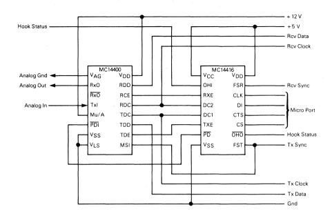
FIGURE 12 - TYPICAL CIRCUIT CONFIGURATION USING MC14416 IN CONJUNCTION WITH MC14400
