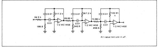
FIGURE 14a - Originate Filter Component Values
