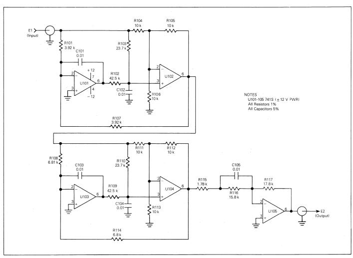
FIGURE 6 - 2400 BPS Modem System Equalizer Sub-Board
