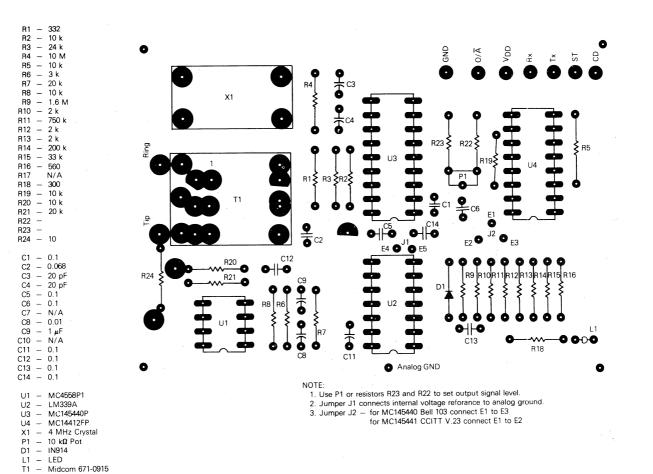
FIGURE 9 - Modem 1 Board MC145440/MC14412
