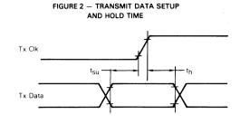
Note: Timing measurements are referenced to and from a low voltage of 0.8 volts and a high voltage of 2.0 volts, unless otherwise noted.
