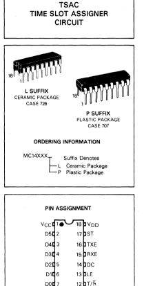
This device contains circuitry to protect the inputs against damage due to high static voltages or electric fields; however, it is advised that normal precautions be taken to avoid application of any voltage higher than maximum rated voltages to this high-impedance circuit. For proper operation it is recommended that V<sub>in</sub> and V<sub>out</sub> be constrained to the range V<sub>SS</sub>  $\leq$  (V<sub>in</sub> or V<sub>out</sub>) $\leq$  V<sub>DD</sub>.
