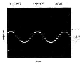
FIGURE 4 - TRANSMIT CARRIER SINEWAVE
