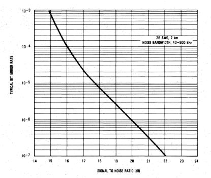
FIGURE 4 - TYPICAL BIT ERROR RATE PERFORMANCE vs SIGNAL-TO-NOISE RATIO FOR GAUSSIAN NOISE FIGURE 5 — TYPICAL MULTICHANNEL DIGITAL LINE CARD
