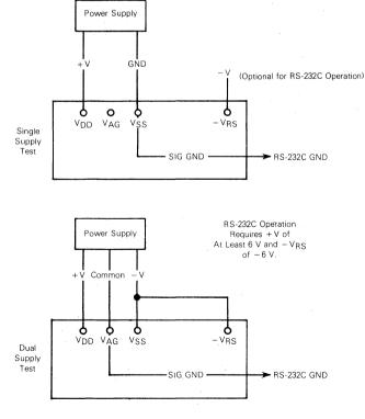
FIGURE 5 - Power Supply Set-Up
