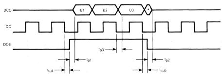
FIGURE 1B - CM = LOW, SYNCHRONOUS OUTPUT SWITCHING CHARACTERISTICS
