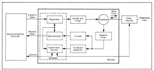
FIGURE 1 - Low-Speed Modem and Interconnections
