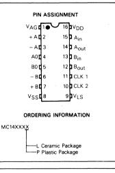
This device contains circuitry to protect the inputs against damage due to high static voltages or electric fields; however, it is advised that normal precautions be taken to avoid application of any voltage higher than maximum rated voltages to this high impedance circuit. For proper operation it is recommended that  $V_{in}$  and  $V_{OSS} \leq (V_{in} \text{ or } V_{OL}) \leq V_{DD}$ .
