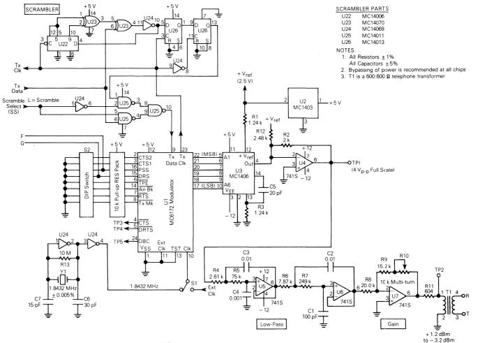
FIGURE 17 - 2400 BPS DPSK MODULATOR SYSTEM
