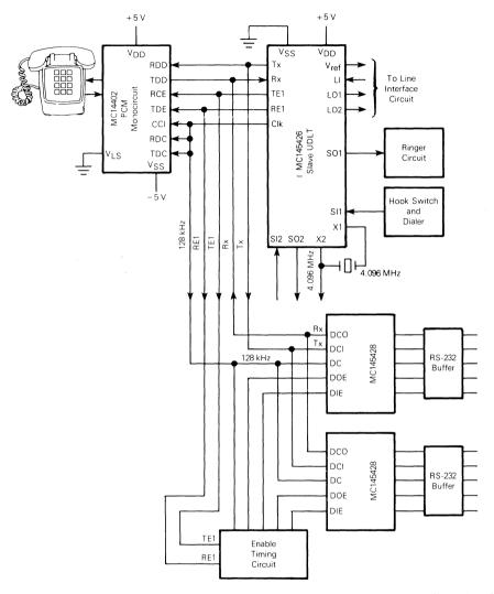
FIGURE 6 - MULTIPLEXING MULTIPLE RS-232 TELSET PORTS INTO 64 KILOBITS/SECOND CHANNEL OF MC145426
