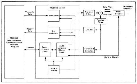
FIGURE 8 - Typical MC6860 Modem System
