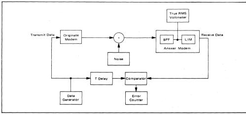
FIGURE 16 - Modem Test Equipment Configuration
