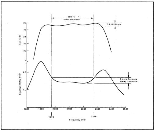
FIGURE 10 - Originate Bandpass Filter Characteristics
