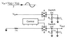
FIGURE 5 — CROSSTALK CONTROL TO OUTPUT
