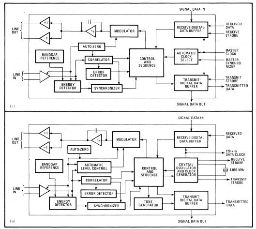
3. Obey. The universal digital-loop transceiver chip is designed in both master (a) and slave (b) versions. The 24-pin master takes care of four-wire PBXs, and the 22-pin master handles two-wire systems. The companion slave chips both have 22 pins.
