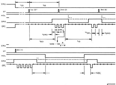
FIGURE 3 - PHONE DIALER SYSTEM TIMING DIAGRAM
