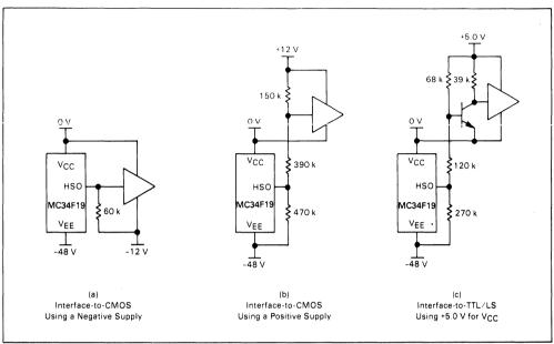
FIGURE 18 - INTERFACE-TO-DIGITAL LOGIC
