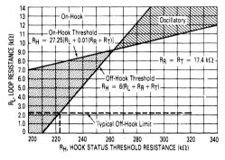
Figure 11 shows such a graph using 17.4  $k\Omega$  as the values for  $R_{R}$  and  $R_{T}$ . Note the oscillatory condition to the right of the crossing point. Selection of  $R_{H}$  in this region is usually not a problem since the majority of telephone lines do not fall into this resistance range.  $R_{H}$  always ties to  $V_{OB}$  and HST and will give reliable hook status information regardless of power supply voltages and PDI.
