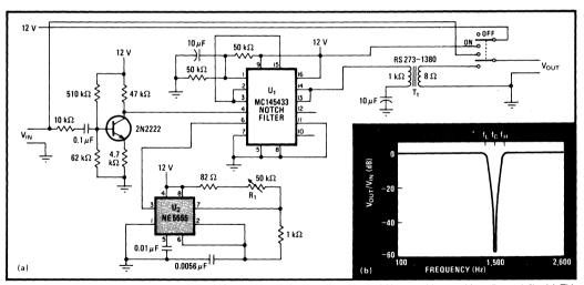
Filtering. Motorola's switched-capacitor notch filter MC145433 is switched by adjustable clock U<sub>2</sub> to provide a tunable audio notch filer (a). This notch filter has a frequency response of about 100 Hz to 2.6 kHz (b) and can operate with voltages from + 10 to + 15 V dc. Transistor Q<sub>1</sub> improves the circuit's signal-to-noise ratio, while audio transformer T<sub>1</sub> drives an 8-ohm load.
