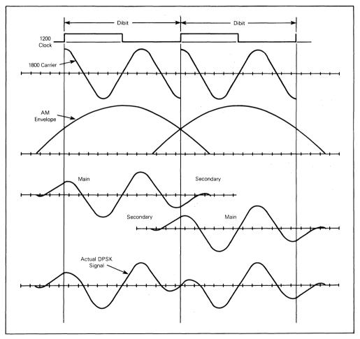
FIGURE 2-DPSK Waveforms
