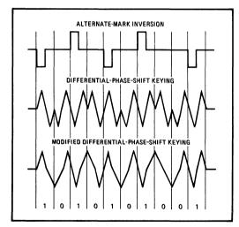
Better yet. For purposes of transmitting 256-kb/s data bursts on twisted pairs up to 2 kilometers in length, a modified differential phase-shift-keyed signal has better electrical properties than either alternate-mark-inversion or unmodified DPSK methods.
