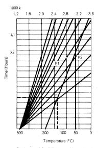
mechanisms: electromigration of circuit metallization, electrolytic corrosion in plastic devices and metal fatigue for Power devices.
