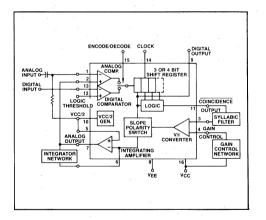
FIGURE 2 — CVSD BLOCK DIAGRAM A Detta Modulator Is Enclosed in a Digitally Controlled Gain Loop and Composes a Continuously Variable Slope Delta Modulator. A Bipolar/I<sup>2</sup>L Integrated Circuit Has Been Designed to Provide All the Active Circuitry Required.
