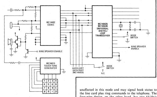
4. Basic. The universal digital-loop transceiver chip combines with other chips to form a digital voice and data telephone that is compatible upward and downward with existing and future private branch exchanges and central-office switches.
