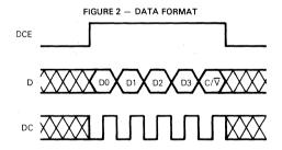
When  $C/\overline{V}$  is "1", D0-D3 are loaded into the configuration register. The four configuration register bits then address a ROM which has outputs to control the analog subsystem elements, enable the appropriate volume register, select the appropriate volume register for the speaker/ringer volume control, and provide the SAE output.
