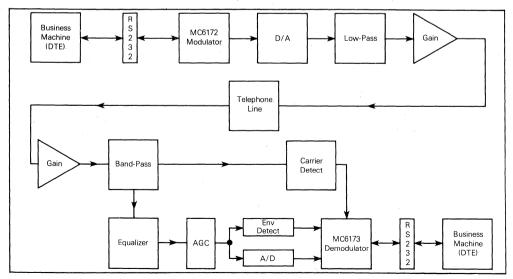
FIGURE 3-MC6172/6173 Modem Block Diagram
