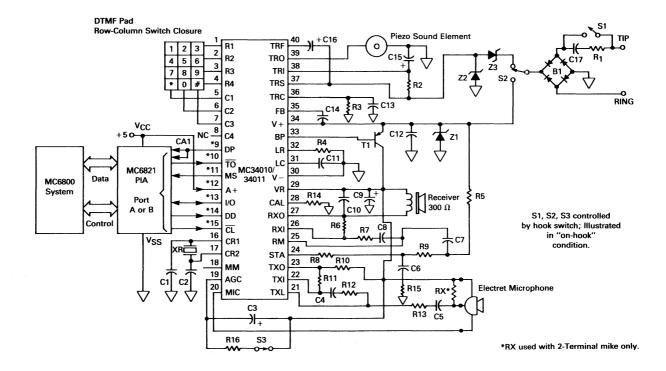
\* Pins 9 through 15 are for MC34010 only; corresponding pins on MC34011 should be connected to V-.
