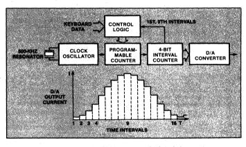
Fig. 2 The DTMF frequency synthesis technique.
