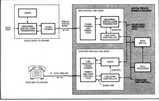
1. Versatile. Motorola's universal digital-loop transceivers bring the 64-kilobit-per-second data-handling power of the private branch exchange to the voice and data telephone or work station over existing twisted pairs, mounting a challenge to Ethernet-like local networks.
