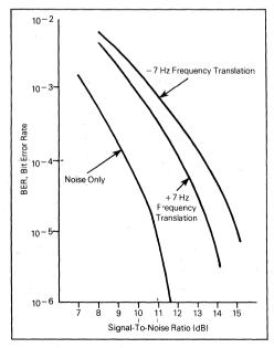
FIGURE 12 — B Mod 2400 BPS Frequency Translation 511 Test Pattern
