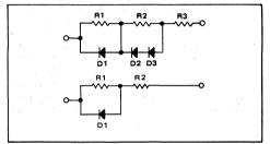
If the performance of more complex diode networks is desired, the circuit in Figure 18 should be used. It simulates the companding characteristics of nonlinear  $R_x$  elements in a different manner.
