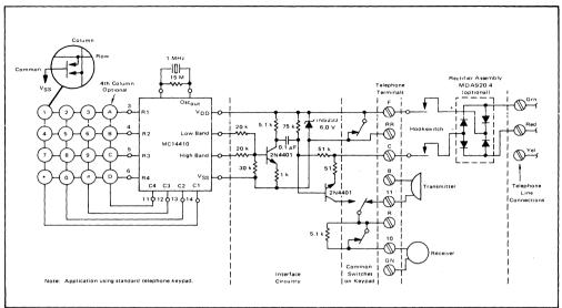
FIGURE 4 - TYPICAL TELEPHONE INTERFACE APPLICATION
