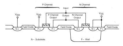
FIGURE 4 - LATCH UP CIRCUIT SCHEMATIC
