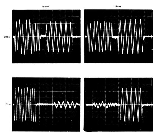
FIGURE 3 - TYPICAL SIGNAL WAVEFORMS AT DEMODULATOR
