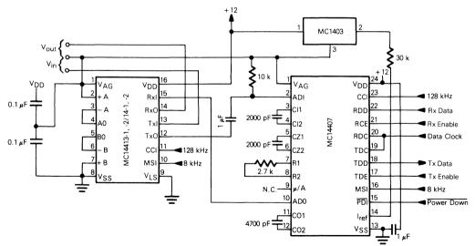
\*Keep all capacitors as near to device pins as possible.
