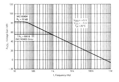
FIGURE 1 - TYPICAL OPEN LOOP FREQUENCY RESPONSE
