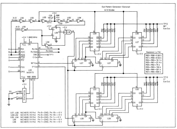
FIGURE 5 - 2400 BPS DPSK Demodulator System (2 of 2)
