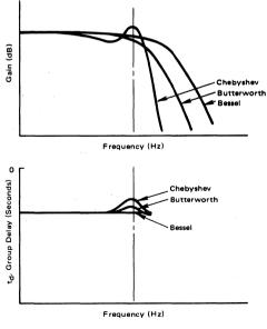
FIGURE 10 - Filter Approximation Characteristics
