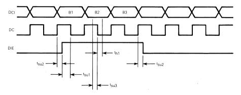
FIGURE 1A - CM = LOW SYNCHRONOUS INPUT SWITCHING CHARACTERISTICS
