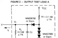
$C_T = 20 \text{ pF} = \text{total parasitic capacitance, which includes probe, wiring, and load capacitances.}$
