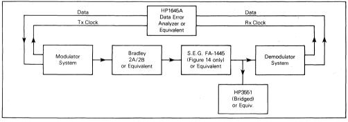
FIGURE 9 - Equipment Setup
