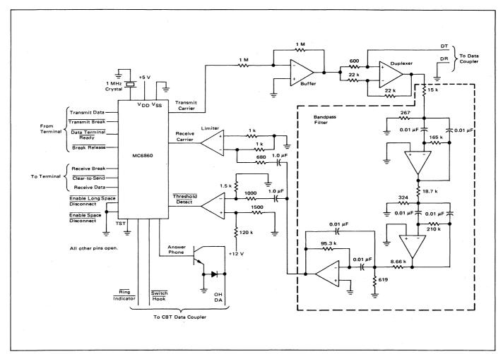
FIGURE 9 – Originate Modem
