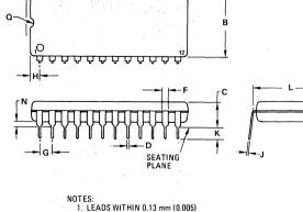
1. LEADS WITHIN 0.13 mm (0.005) RADIUS OF TRUE POSITION AT SEATING PLANE AT MAXIMUM MATERIAL CONDITION. 2. DIMENSION "L'TO CENTER OF LEADS WHEN FORMED PARALLEL.
