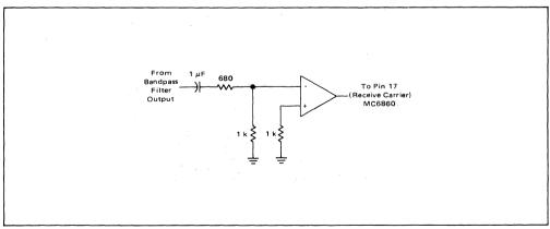
FIGURE 11 - Limiter Schematic
