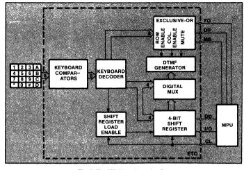
Fig. 3 The MPU interface circuit.
