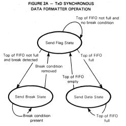
follows five continuous 1's in order to recover the transmitted data. (Note that a binary 1 which follows five continuous 1s is not removed so that flags and breaks may be detected.) Figure 2B shows an example of this process.
