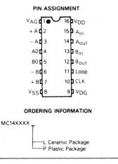
This device contains circuitry to protect the inputs against damage due to high static voltages or electric fields; however, it is advised that normal precautions be taken to avoid application of any voltage higher than maximum rated voltages to this high impedance circuit. For proper operation it is recommended that  $V_{in}$  and  $V_{out}$  be constrained to the range  $V_{SS} \leq (V_{in} \text{ or } V_{out}) \leq V_{DD}$ .
