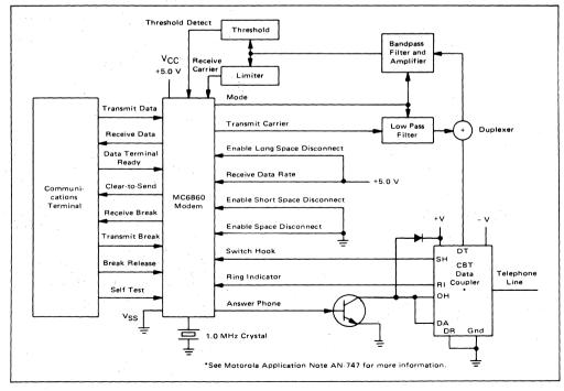
When utilizing the 1.0 MHz crystal, external parasitic capacitance, including crystal shunt capacitance, must be  $\leq 9$  pF at the crystal input. Reliable crystal oscillator start-up requires that the V<sub>CC</sub> power-on transition time be >15 milliseconds.
