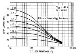
can be used to determine the value of  $R_{\ensuremath{OB}}$  that will yield the desired maximum loop current.
