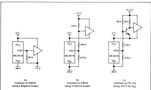
FIGURE 18 - INTERFACE-TO-DIGITAL LOGIC
