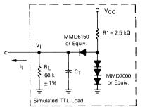
$C_T$  = 20 pF = total parasitic capacitance, which includes probe, wiring, and load capacitances.
