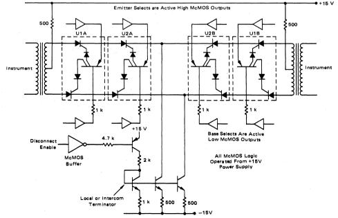
current restriction is not a restriction in the design of an efficient crosspoint array. Because of the current sink terminations, a signal path may use differing numbers of crosspoints in any connection or in two sides of the same connection further relaxing restrictions in array design.
