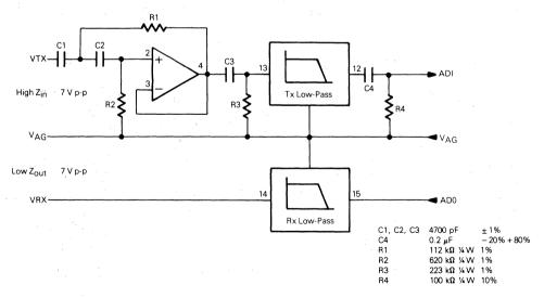
\*In noisy environments, R1-R4 should be 10 k $\!\Omega$  or less to minimize pickup.
