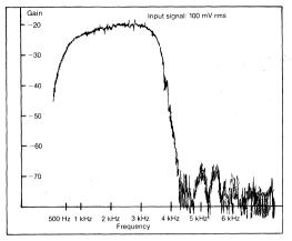
The switched-capacitor low-pass filter limits both input and output frequencies to about 3.7 kHz, as reflected by the system frequency response curve. Input frequencies are limited to prevent aliasing; filtering the output smooths it out. Bandwidth for the circuit ranges from 500 Hz to 3.7 kHz.
