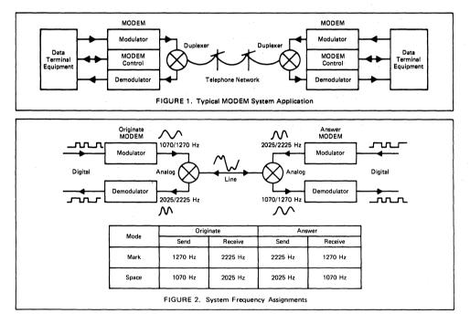
the data terminal receiving this call is the answer MODEM, (transmitting tones of 2025 Hz and 2225 Hz).
