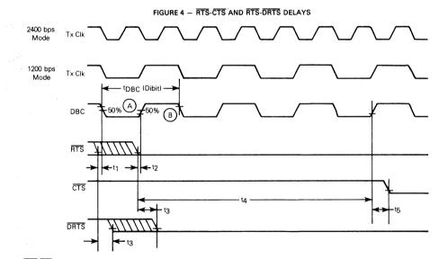
.  $\overline{RTS}$ - $\overline{CTS}$  delay options are selected by the CTS1 and CTS2 inputs, and are stated as time delay interval t4. An  $\overline{RTS}$  input signal synchronized about point A will synchronize  $\overline{CTS}$  with the positive transition of DBC (Dibit Clock). Delay t4 is measured with respect to the negative transition of  $\overline{RTS}$ .
