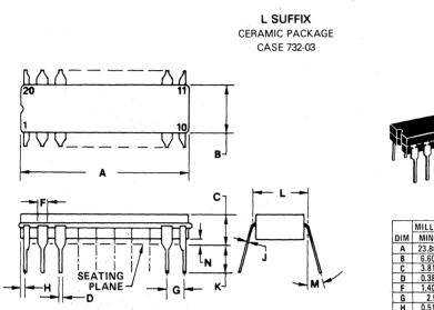
NOTES: 1. LEADS WITHIN 0.25 mm (0.010) DIA, TRUE POSITION AT SEATING PLANE, AT MAXIMUM MATERIAL CONDITION.
