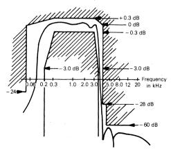
GAIN vs FREQUENCY, SINUSOIDAL
