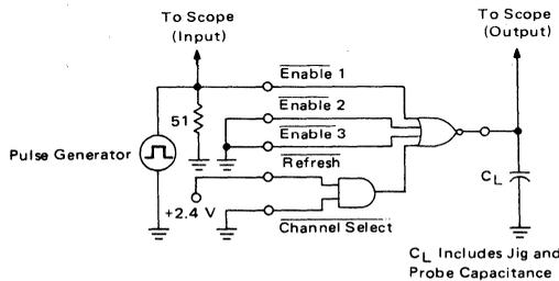
FIGURE 4 – SWITCHING TEST CIRCUIT FOR REFRESH MODE – MC3460
