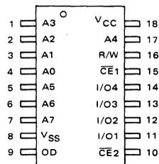
This device contains circuitry to protect the inputs against damage due to high static voltages or electric fields; however, it is advised that normal precautions be taken to avoid application of any voltage higher than maximum rated voltages to this high impedance circuit.
