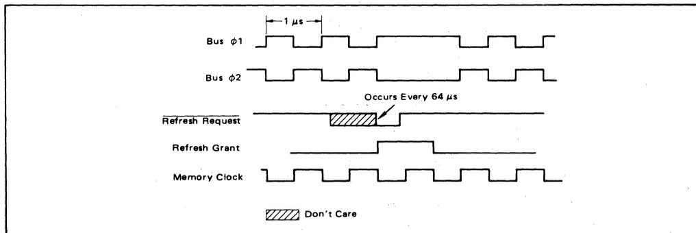
FIGURE 16 – MEMORY TIMING IN STANDBY MODE
