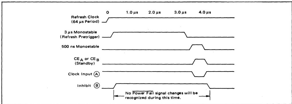
FIGURE 11 – Power Up/Down Synchronization
