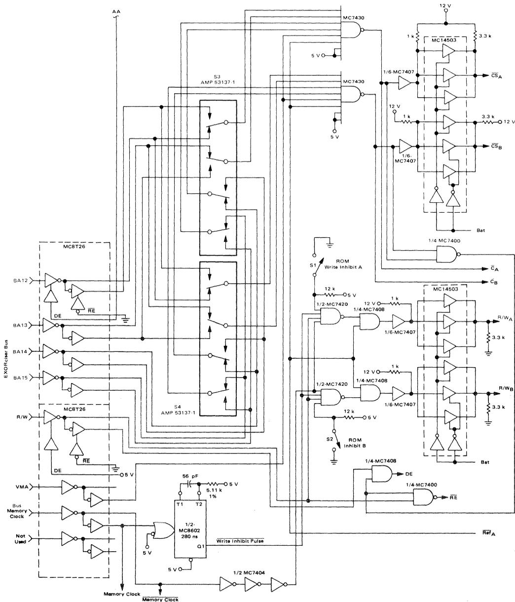
FIGURE 6 – Address Buffers and Decoding Logic
