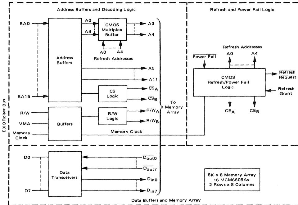
FIGURE 3 - Non-Volatile Memory System Block Diagram
