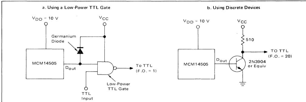
FIGURE 13 – CMOS-TO-TTL INTERFACE FOR  $V_{DD} = 15\text{ V}$
