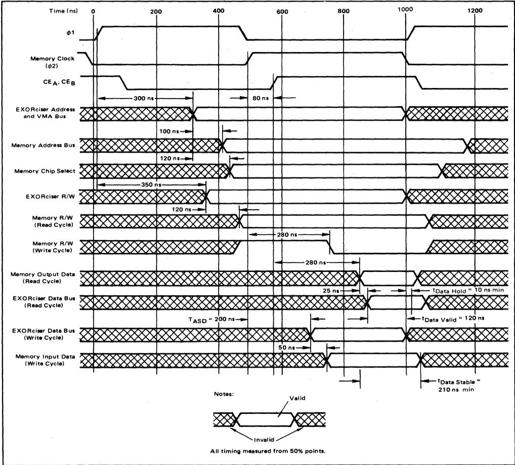
FIGURE 4 – EXORciser/4K Memory System Timing Diagram
