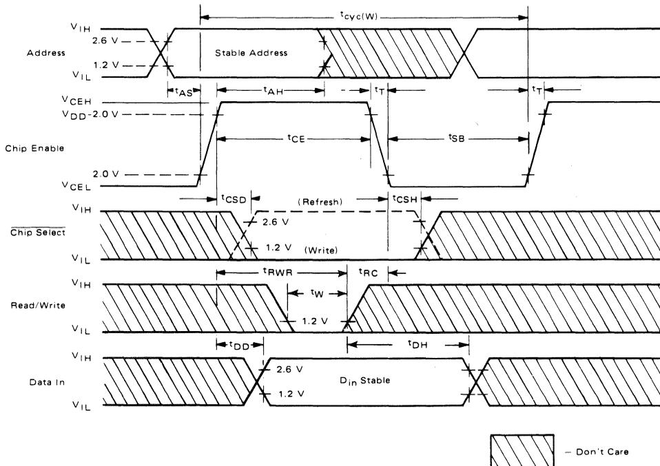
**READ-MODIFY-WRITE ( $R/W = V_{IH} \rightarrow V_{IL}$ ,  $\overline{CS} = V_{IL}$ )**
