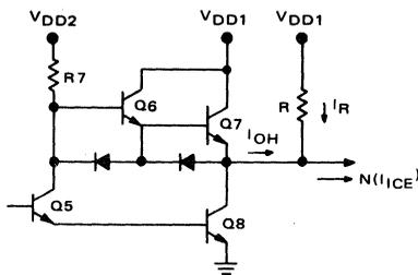
FIGURE 19 – APPLICATION OF CLAMPING DIODES TO LIMIT OVERSHOOT
