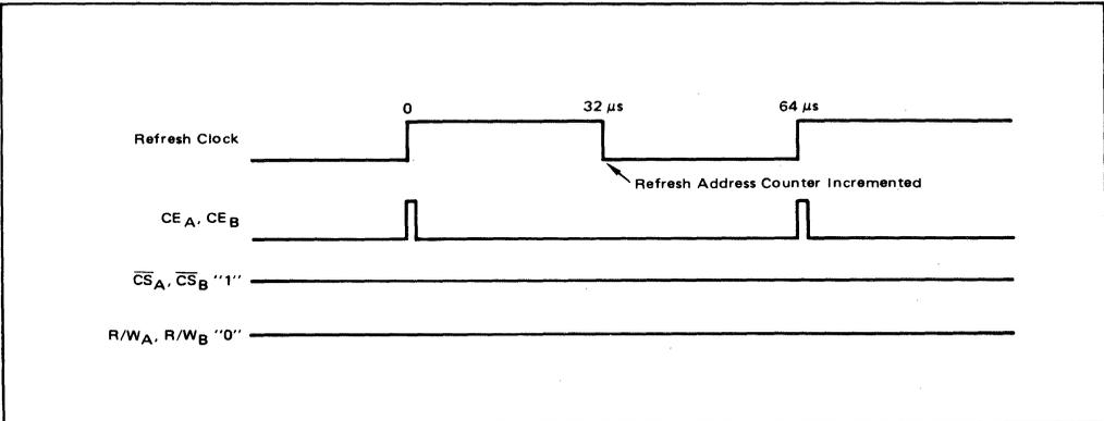
FIGURE 5 – Memory Timing in Standby Mode
