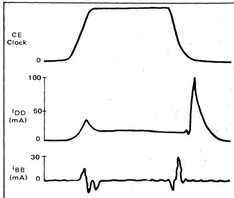
FIGURE 19 – Typical Supply Current Transient Waveforms
