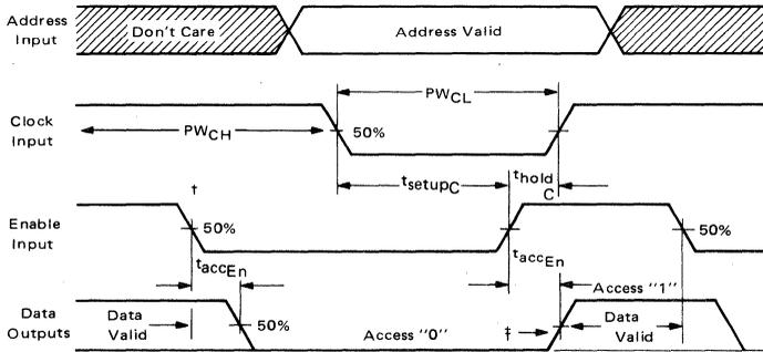
† In this mode of operation, the negative going edge of Enable should occur on or before the clock negative edge.
