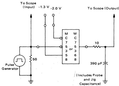
The pulse generator has the following characteristics:
