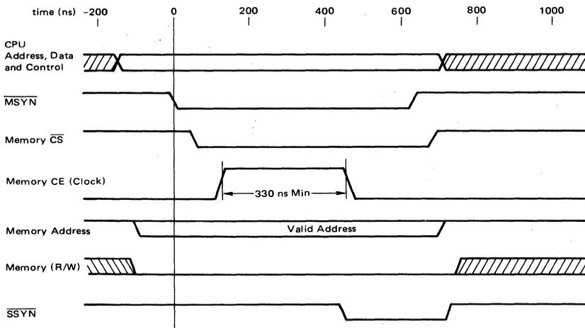
FIGURE 10 – Typical System Write Cycle Time
