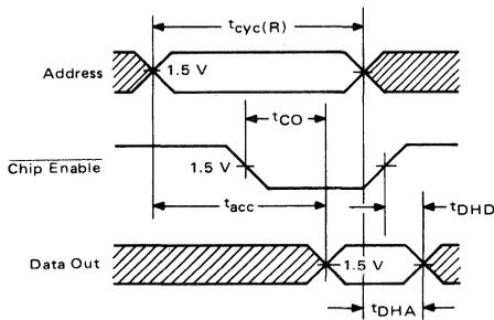
\*R/W =  $V_{IH}$  for a Read Cycle.
