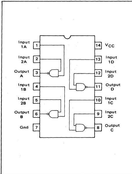
FIGURE 15 – MC3459 Pin Assignment
