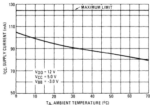
FIGURE 3 –  $V_{DD}$  SUPPLY CURRENT versus TEMPERATURE
