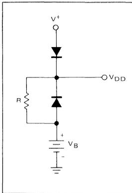
FIGURE 10 – TTL TO CMOS INTERFACE
