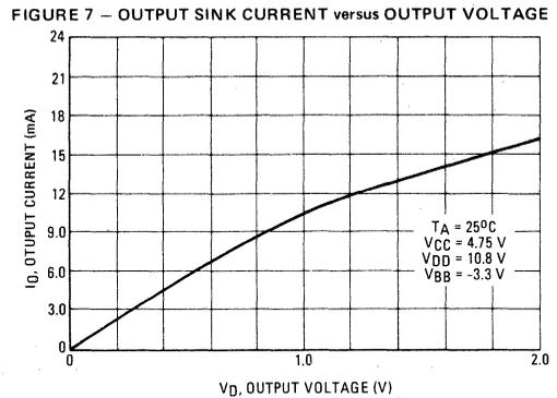
\*These curves represent averaged MCM6591 currents over address cycling in the selected mode. More dense patterns can be expected to shift these curves upward, bounded by the maximum dc values stated in the DC Characteristics Table.
