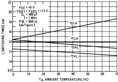
FIGURE 12 – SWITCHING TIMES versus TEMPERATURE (REFRESH MODE)
