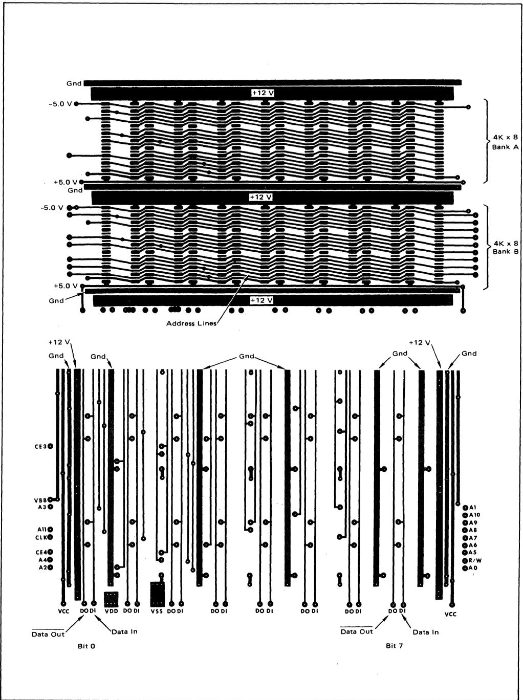
FIGURE 14 – Memory PC Board Array
