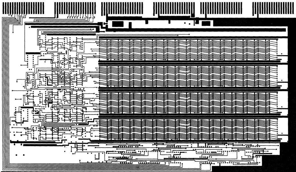
FIGURE 17 - PC Board Layout of Memory System
