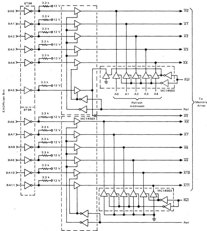
FIGURE 6 – Address Buffers and Decoding Logic
