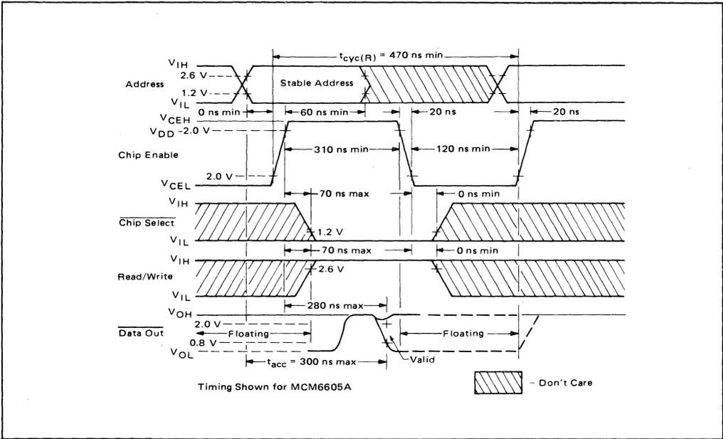
FIGURE 2a – Read Cycle Timing (Minimum Cycle)
