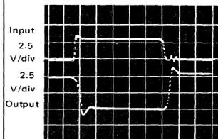
$V_{CC} = 5.0 \text{ V}$      $50 \text{ ns/div}$      $C_L = 360 \text{ pF}$
