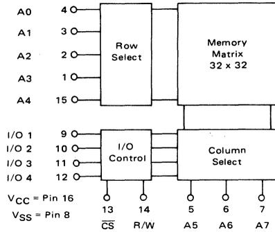
This device contains circuitry to protect the inputs against damage due to high static voltages or electric fields; however, it is advised that normal precautions be taken to avoid application of any voltage higher than maximum rated voltages to this high impedance circuit.
