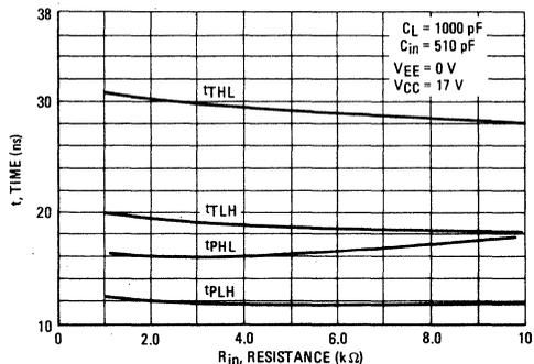
FIGURE 14 – DC-COUPLED SWITCHING versus  $C_{in}$  (See Figure 4.)
