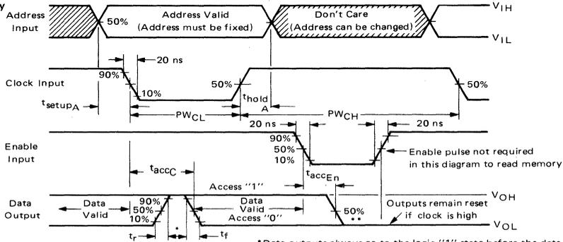
\*Data outputs always go to the logic "1" state before the data is valid between accessing successive "0's"
