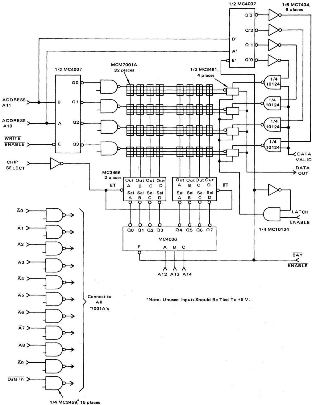
FIGURE 23 - 4K x 18 MEMORY BOARD (TTL INTERFACE)
