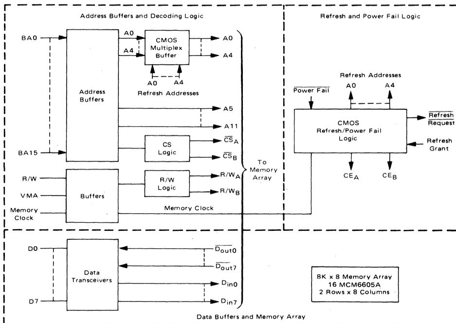
MC14503. The Memory Clock (used during normal operation) is translated to 12 V levels by use of an MC3460 Clock Driver. Decoding of the CE<sub>A</sub> and CE<sub>B</sub> signals (i.e., clocking only the memory bank addressed) to conserve power is accomplished by the logic within the MC3460.
