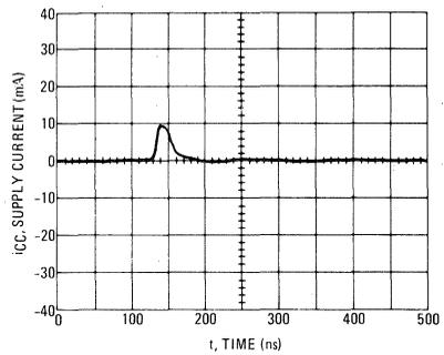
FIGURE 11 –  $i_{BB}$  SUPPLY CURRENT
