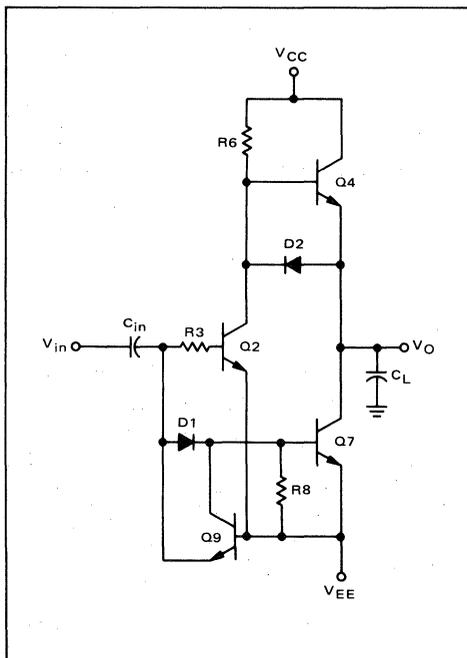
The complete circuit, Figure 1, basically creates Darlington devices of transistors Q7, Q4 and Q2 in the simplified circuit of Figure 17. Note in Figure 1 that when the input goes negative with respect to  $V_{EE}$ , diodes D7 through D10 turn "on" assuring faster turn "off" of transistors Q1, Q2, Q6 and Q7. Resistor R6 insures that the output will charge to within one  $V_{BE}$  voltage drop of the  $V_{CC}$  supply.
