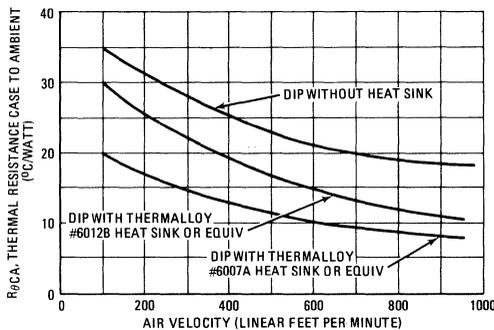
Note from Table 1 and Figure 15 that if the 16-pin ceramic package is mounted directly to the PC board (2 oz. cu. underneath), that typical  $R_{\theta JA}$  is considerably less than for socket mount with still air and no heat sink. The following procedure can be employed to determine the maximum power dissipation for this condition.
