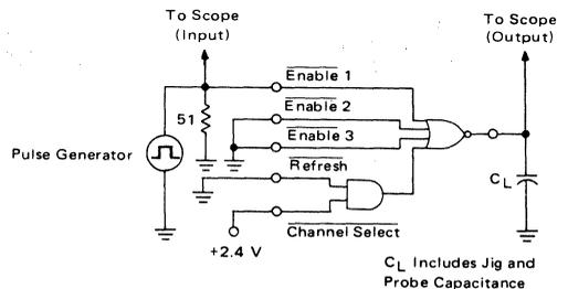
FIGURE 5 – SWITCHING TEST CIRCUIT FOR READ/WRITE MODE – MC3466
