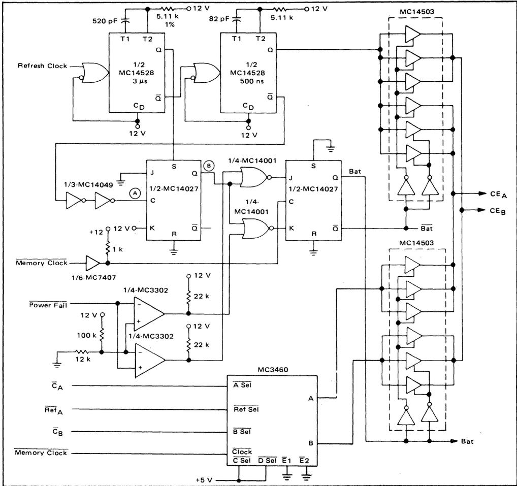
FIGURE 10 – Power Fail Logic
