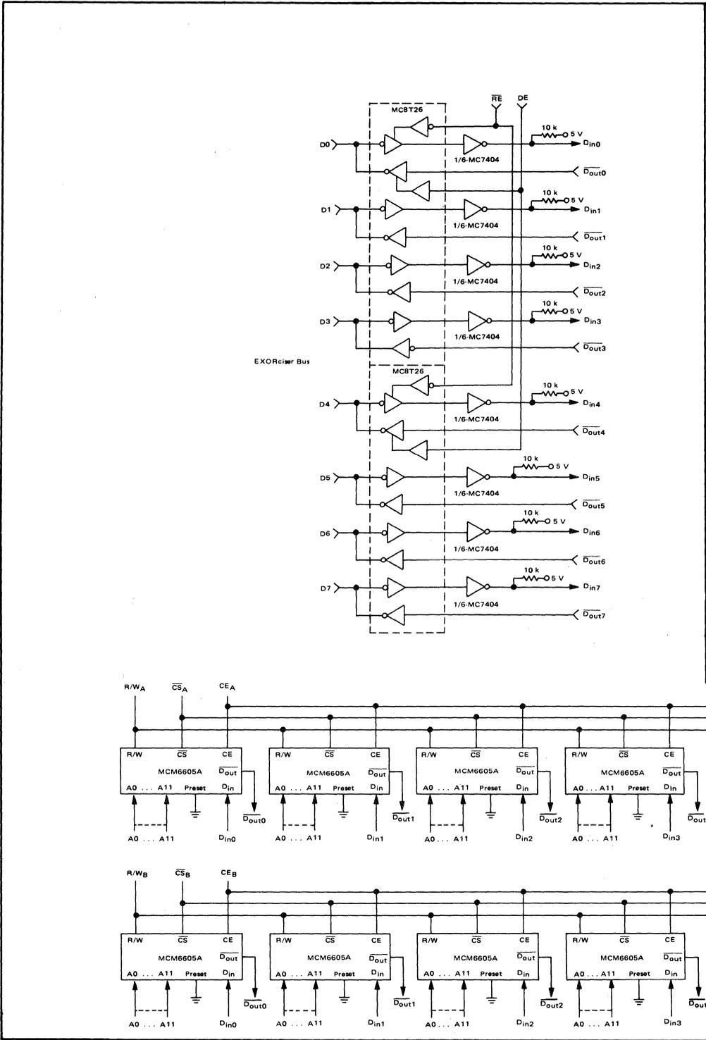
FIGURE 7 – Data Buffers and Memory Array
