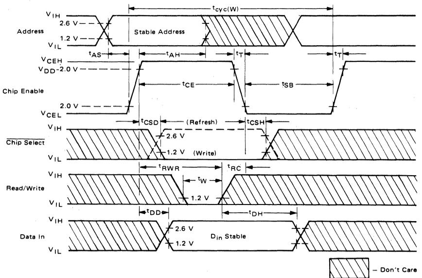
FIGURE 4 - Write and Refresh Cycle Timing
