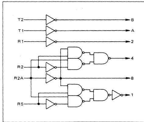
FIGURE 21 - EBCDIC TO ASCII CODE CONVERSION
