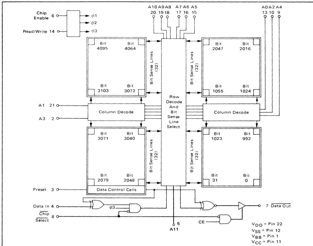
FIGURE 1 — MCM6605A 4K RAM Block Diagram
