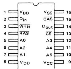
This device contains circuitry to protect the inputs against damage due to high static voltages or electric fields; however, it is advised that normal precautions be taken to avoid application of any voltage higher than maximum rated voltages to this high-impedance circuit.
