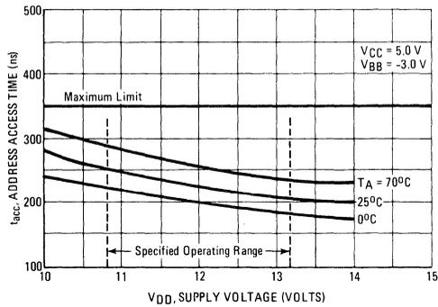
FIGURE 7 – ADDRESS ACCESS TIME versus TEMPERATURE
