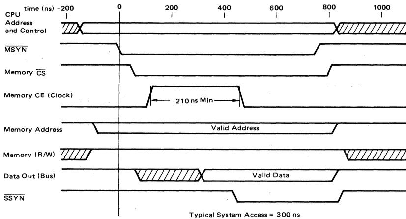
FIGURE 9 – Typical System Read Cycle Time
