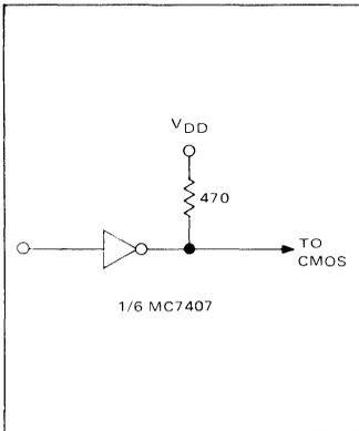
FIGURE 11 – CMOS-TO-TTL INTERFACE FOR  $V_{DD} = 5.0\text{ V}$
