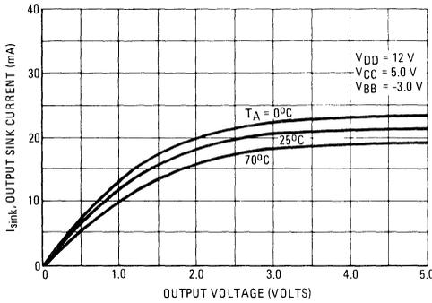
FIGURE 5 – OUTPUT SOURCE CURRENT versus OUTPUT VOLTAGE
