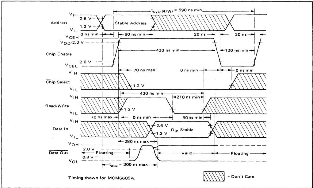
FIGURE 2c - Read-Modify-Write Timing (Minimum Cycle)
