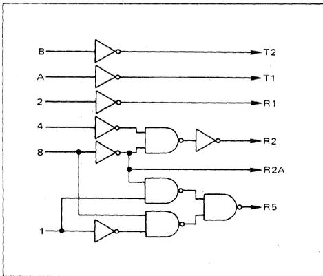
FIGURE 20 - BAIL CODE TO SELECTRIC LINE CODE CONVERSION
