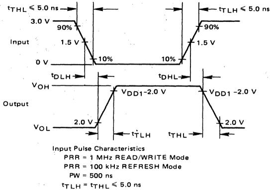
FIGURE 2 – SWITCHING TEST WAVEFORMS – MC3466
