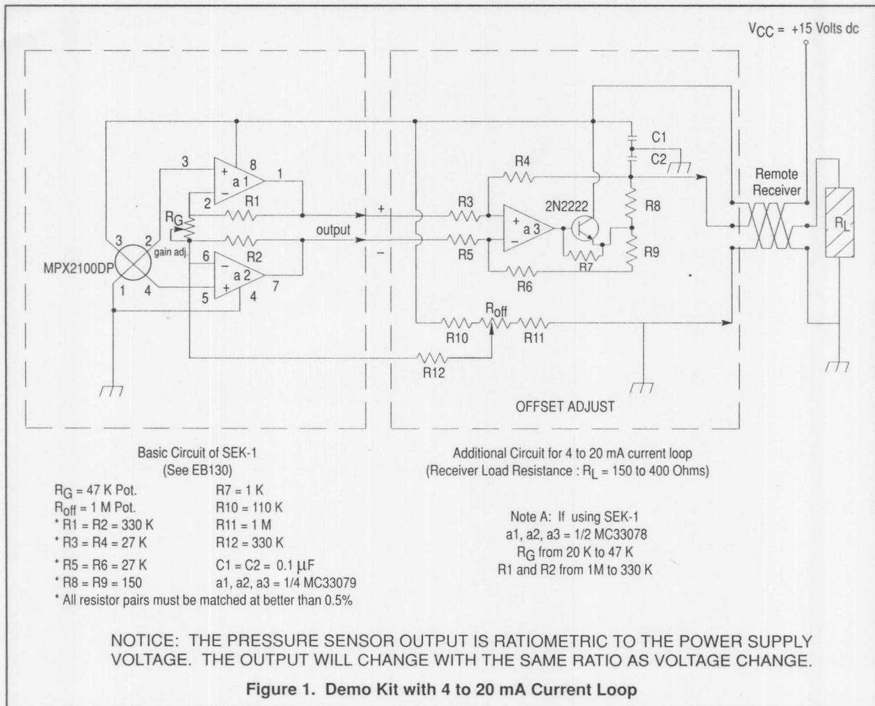
To achieve good performance with a very long transmission line it may be necessary to place some capacitors (C1, C2) between the power supply and output to prevent oscillations.
