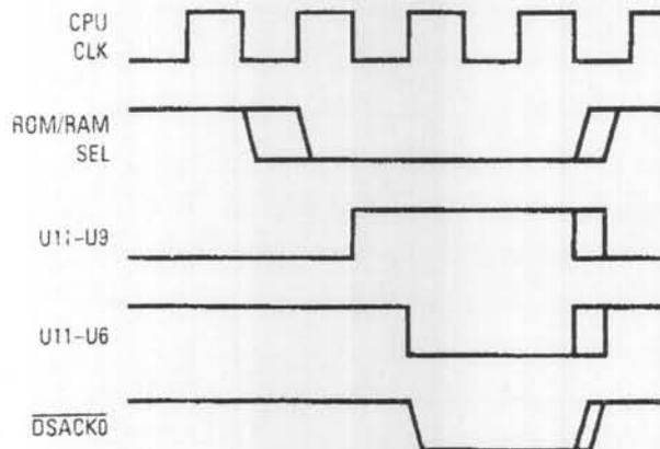
Figure 3.  $\overline{DSACK}$  Timing Diagram
