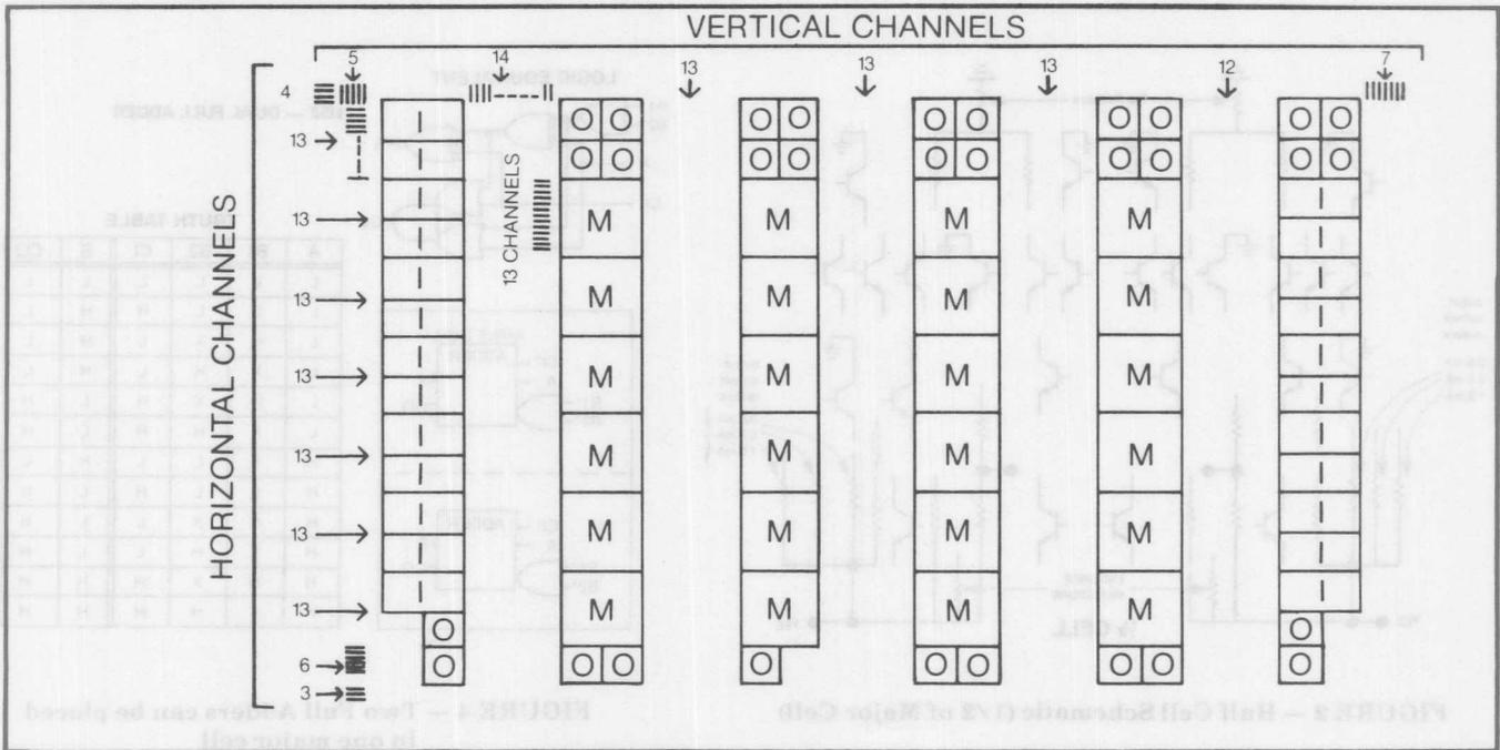
**FIGURE 5 — MCA500ALS Macrocell layout shows the relative positions of macrocells within the array. Horizontal and vertical routing channels connect macrocells, much as a printed circuit board layout.**
