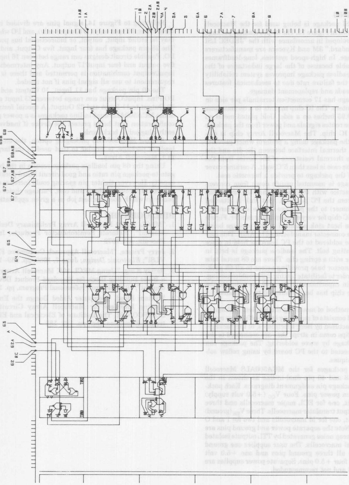
FIGURE 12 — Macrocell Logic Diagram 4-Bit Programmable Counter
