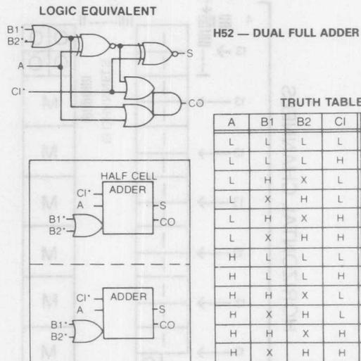
FIGURE 4 — Two Full Adders can be placed in one major cell
