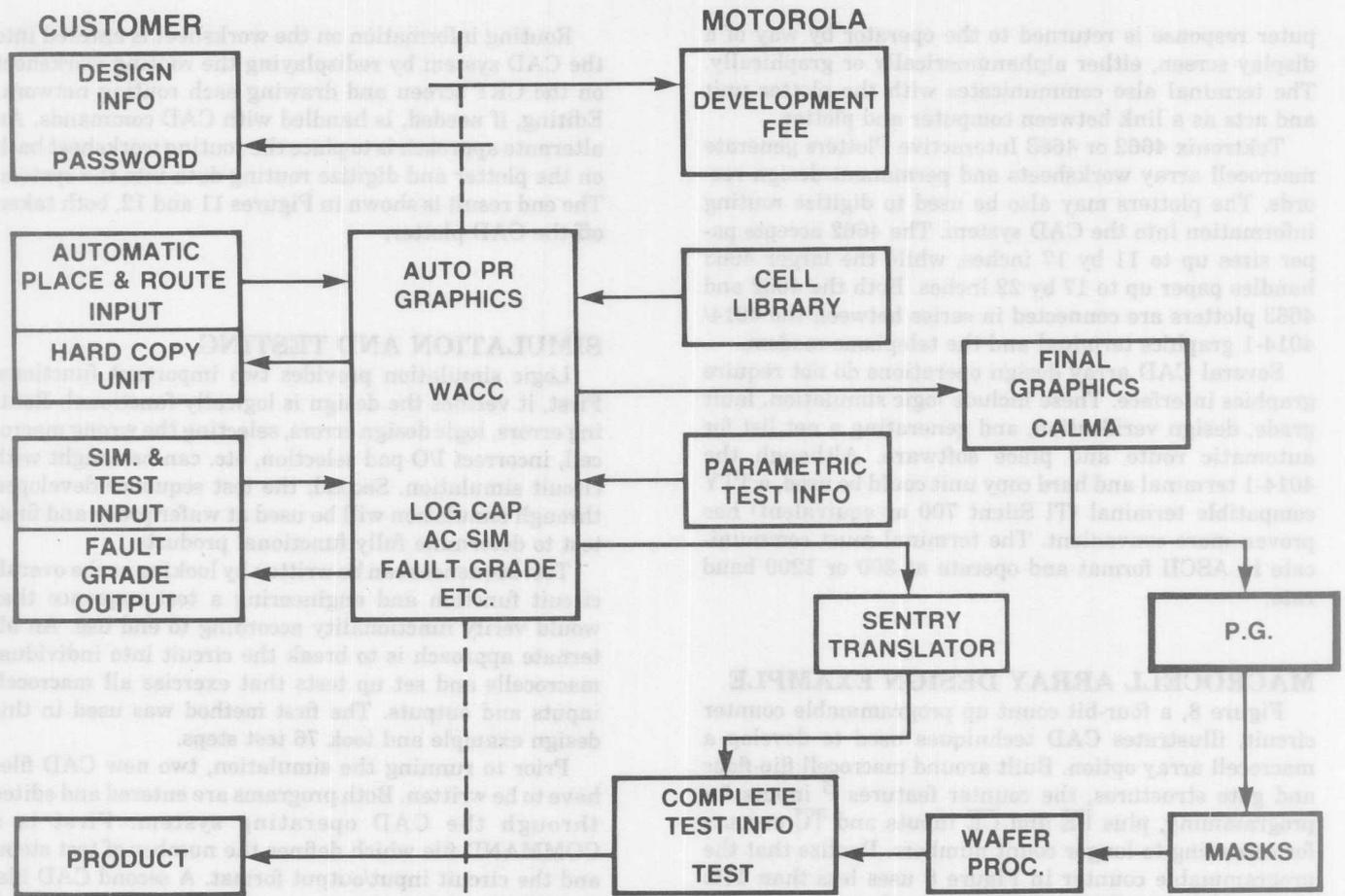
FIGURE 7 — Macrocell Array Option Development Flow
