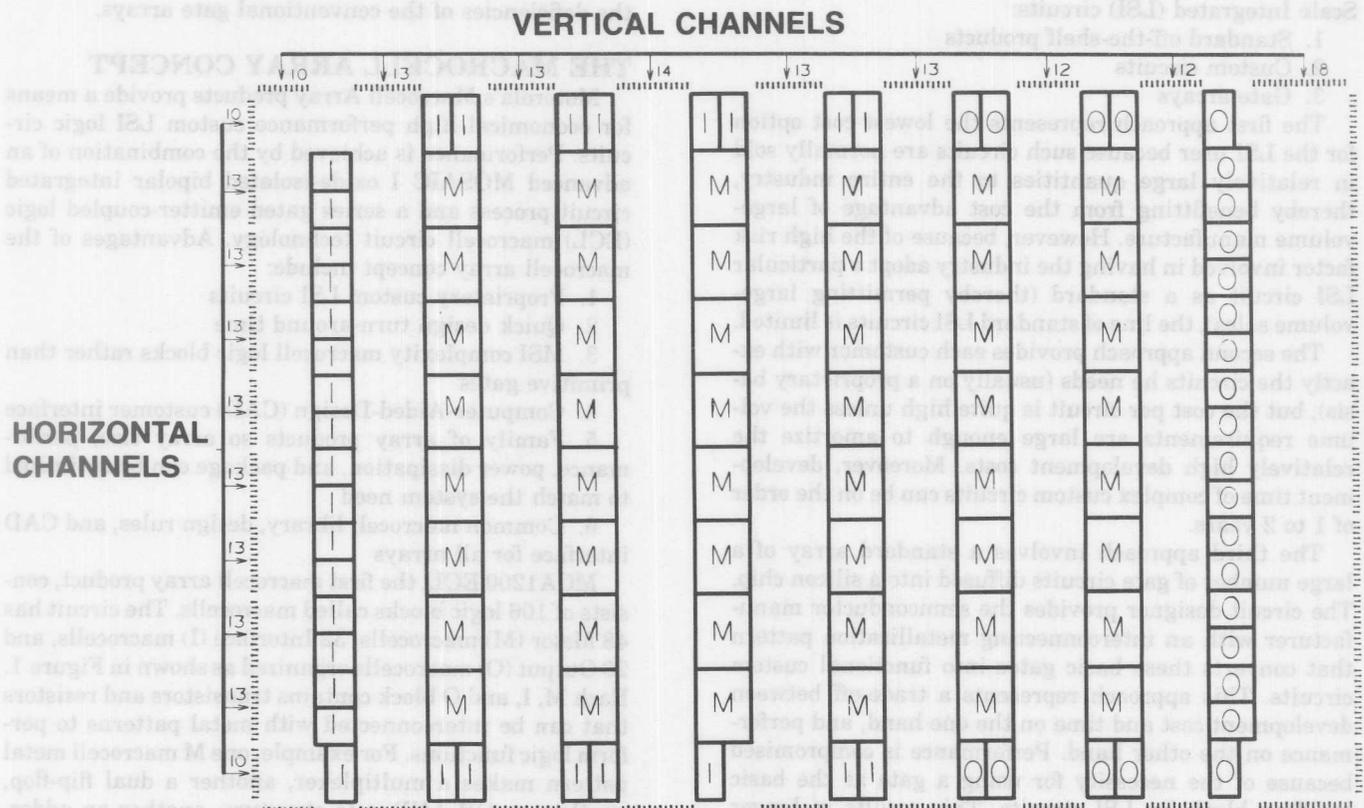
FIGURE 1 — MCA1200ECL Macrocell Array Metal Interconnect Channels
