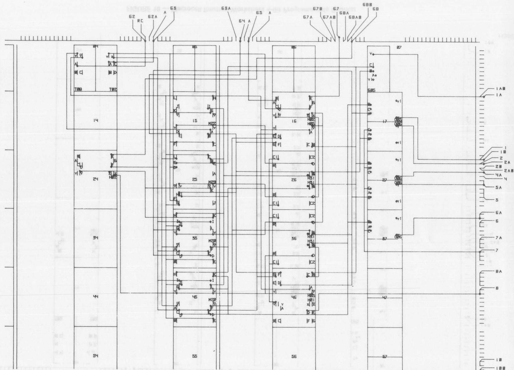
FIGURE 11 — Macrocell Routing Diagram 4-Bit Programmable Counter
