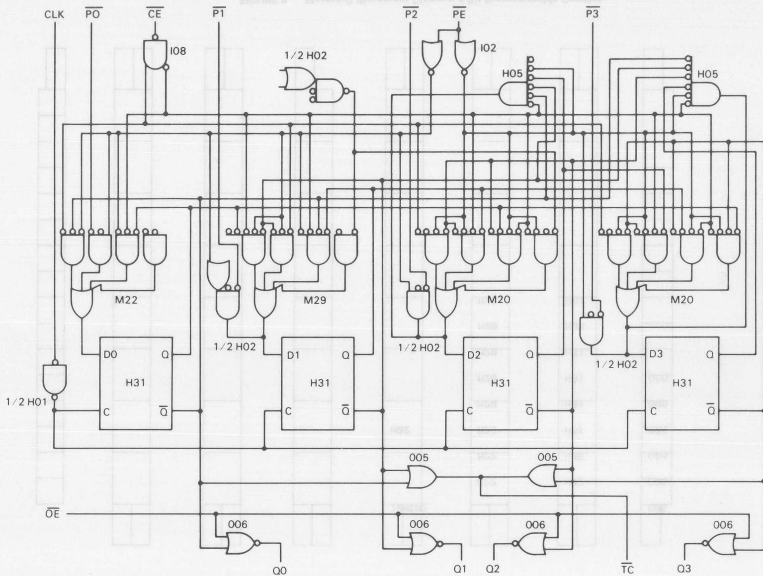
FIGURE 8 — 4-Bit Programmable Counter
