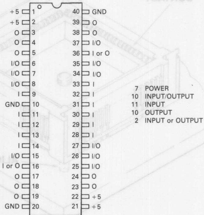
FIGURE 14 — MCA500ALS Macrocell Array Package Pin Assignments
