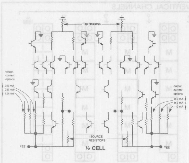
FIGURE 2 — Half Cell Schematic (1/2 of Major Cell)
