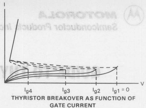
FIGURE 2 — Thyristor Characteristics Illustrating Breakover as a Function of Gate Current.
