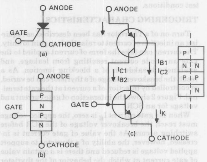
**FIGURE 1 — Two-transistor analogy of an SCR:**
