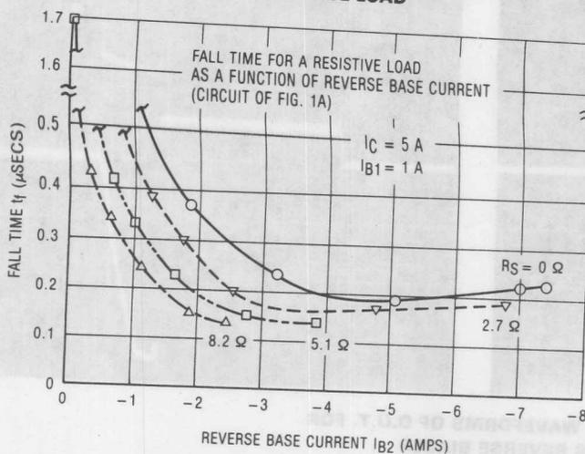
**FIGURE 6 — FALL TIME OF THE 2N6250 WITH VARIABLE REVERSE BASE CURRENT AND LOWER COLLECTOR CURRENT**
