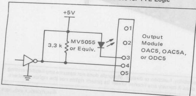
ure 2. This configuration may be used with standard TTL, Schottky (S), low-power Schottky (LS), and high-speed (H) series devices. Low-power TTL (L) may be buffered with an LS device. Although the standard TTL output configuration will drive the module, it may be desirable to use open-collector devices for the output module drivers.
