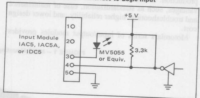
In all three illustrations, an indicator LED is added to indicate the status of the device. If a mounting board such as the MS16 is used, both the indicator LED and the 3.3 kΩ resistor are installed on the board at the factory.
