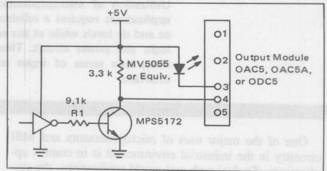
of an NPN transistor, which, in turn, drives the output module. By changing the value of R1 to 39 kΩ, this configuration may be used to interface CMOS operating at 15 volts with 15-volt logic modules OAC15, OAC15A, and ODC15.
