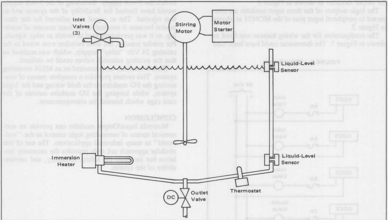
in a plant that batch-processes liquids through a number of mixing, stirring, and heating cycles. The original plant was controlled by relay logic and had high operating cost due to direct operating labor and maintenance expense. The goal of the conversion of the plant to a distributed processor-based control system was to increase flexibility while increasing reliability and reducing labor.
