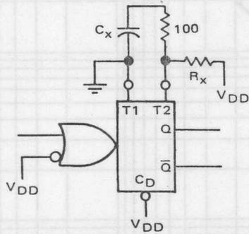
FIGURE 8 — Use of 100 Ohm Resistor to Limit Power Down Current Surge
