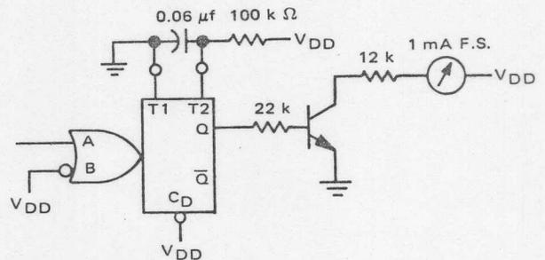
FIGURE 13 — Precision Analog Tachometer
