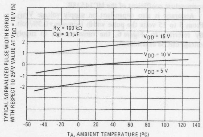
FIGURE 4 – Typical Pulse Width Error versus Temperature
