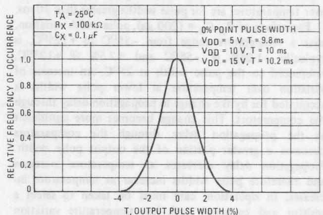
FIGURE 3 – Typical Normalized Distribution of Units for Output Pulse Width
