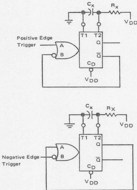
FIGURE 11 — Non-retriggerable Monostables Circuitry
