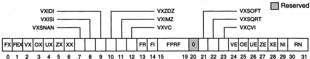
**Figure 2-5. Floating-Point Status and Control Register (FPSCR)**
