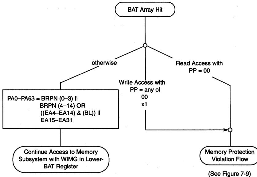
Figure 7-11. Block Address Translation Flow
