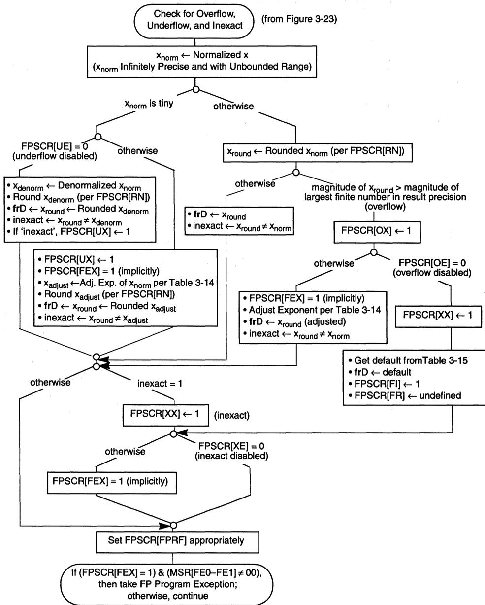
Figure 3-24. Checking of Remaining Floating-Point Exception Conditions
