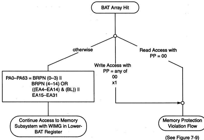
Figure 7-11. Block Address Translation Flow
