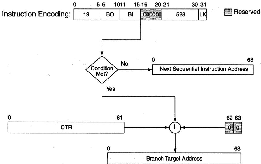
Figure 4-11. Branch Conditional to Count Register Addressing
