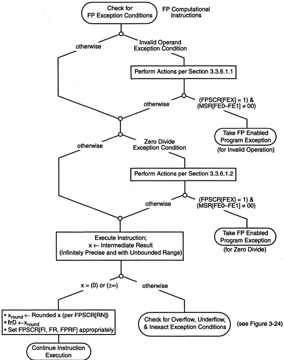
**Figure 3-23. Initial Flow for Floating-Point Exception Conditions**
