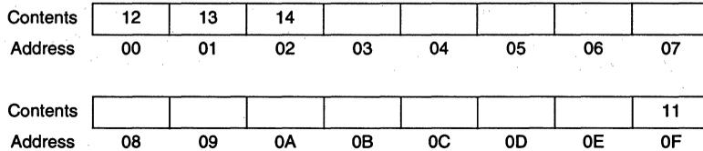
**Figure 3-8. Word Stored at Little-Endian Address 05 as Seen by the Memory Subsystem**
