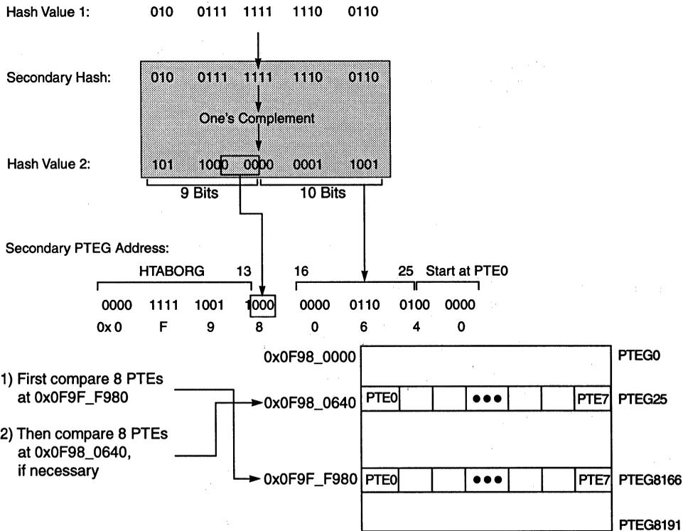
**Figure 7-24. Example Secondary PTEG Address Generation**
