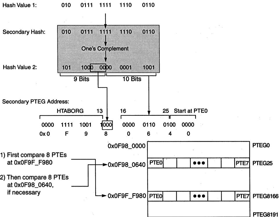
**Figure 7-24. Example Secondary PTEG Address Generation**
