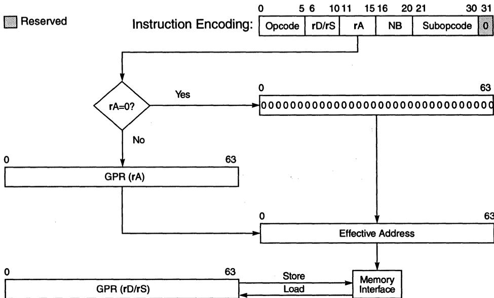
Figure 4-3. Register Indirect Addressing for Integer Loads/Stores
