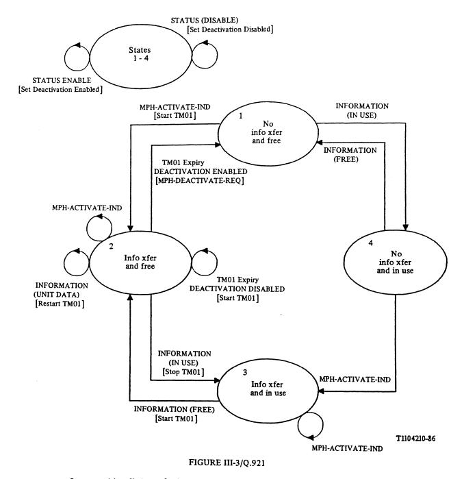
State transition diagram of a deactivation procedure without MPH-DEACTIVATE-IND
