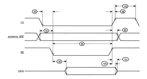
Figure 8-13. MPU Read Timing (80186 Mode)
