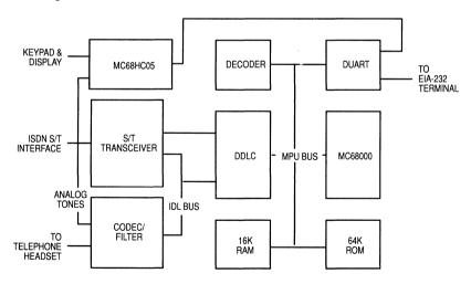
Figure 7-1. ISDN Terminal Adapter and Voice and Data Block Diagram
