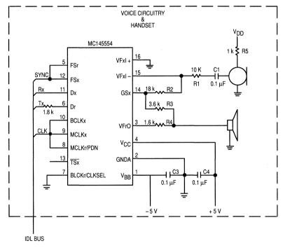
Figure 7-14. Macintosh SE ISDN Terminal Card (Codec/Filter Section)
