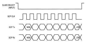
Figure 6-15. SCP Pin Functions — Slave Mode
