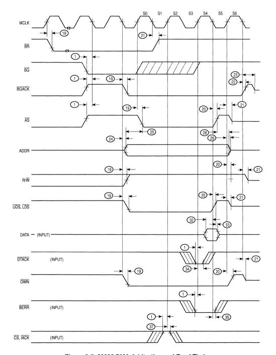
Figure 8-5. 68000 DMA Arbitration and Read Timing
