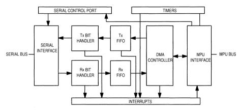
Figure 2-1. DDLC Block Diagram (One Transceiver Shown)
