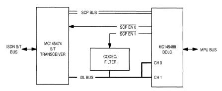
Figure 6-12. ISDN Terminal Application
