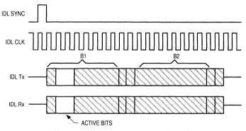
Figure 6-4. IDL Subrate Multiplexing
