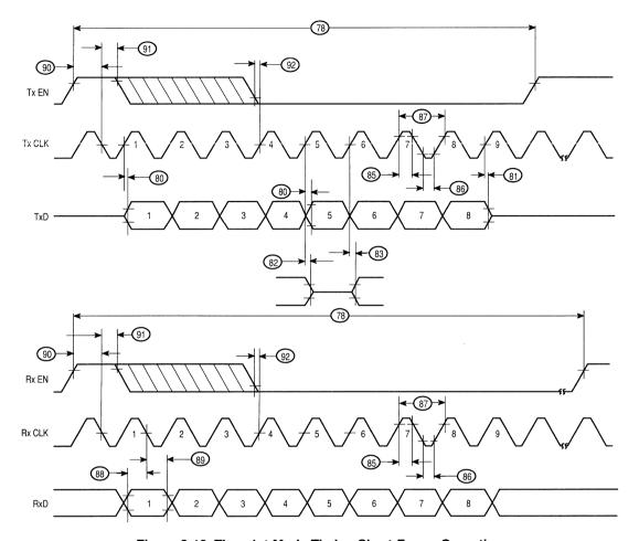
Figure 8-12. Timeslot Mode Timing Short-Frame Operation
