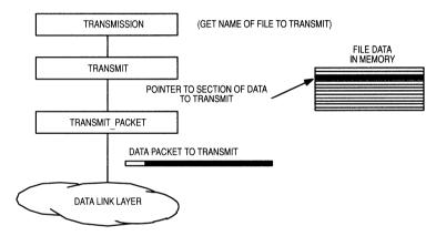
Figure 7-16. Transmit Procedure
