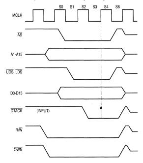
Figure 5-3. 68000 DMA Write Cycle
