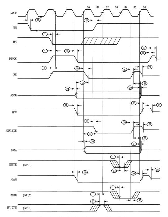
Figure 8-4. 68000 DMA Arbitration and Write Timing
