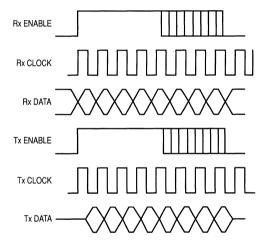
Figure 6-8. Timeslot Operation Long-Frame
