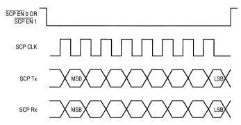
Figure 6-14, SCP Pin Functions — Master Mode
