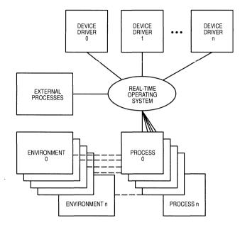
Figure 7-4. Real-Time Multitasking Operating System
