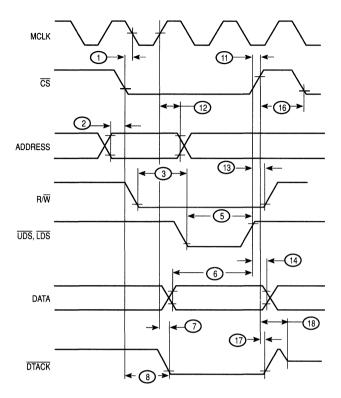
Figure 8-2. 68000 MPU Write Timing
