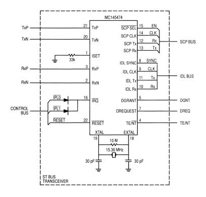
Figure 7-12. Macintosh SE ISDN Terminal Card (S/T Transceiver Section)
