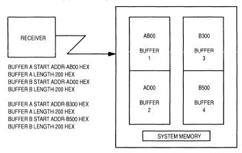
Figure 2-4. Alternate Receive Buffer Operation
