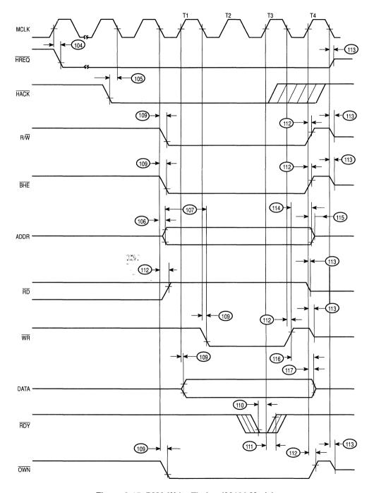
Figure 8-15. DMA Write Timing (80186 Mode)
