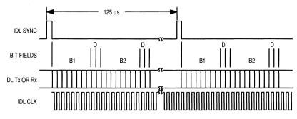
Figure 6-2. IDL Frame Timing
