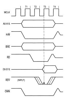
Figure 5-9. 80186 DMA Write Cycle
