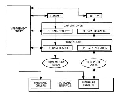
Figure 7-15. Terminal Card Software **Block Diagram**
