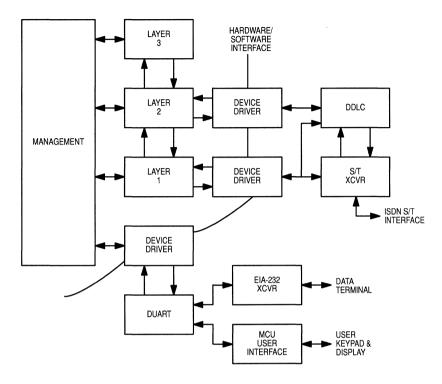
Figure 7-5. Terminal Adapter Software/Hardware Model
