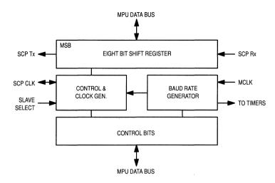
Figure 6-13. SCP Module Block Diagram
