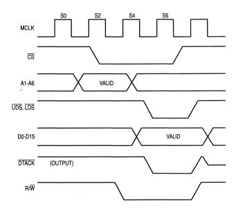
Figure 5-1. 68000 Host Write Cycle
