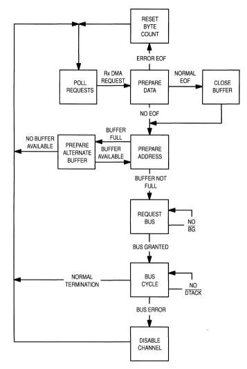
Figure 2-6. DMA Receive State Diagram
