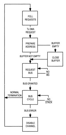
Figure 2-5. Transmit DMA State Diagram
