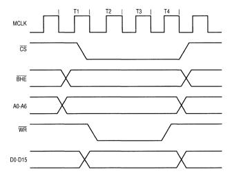
Figure 5-7. 80186 Host Write Cycle
