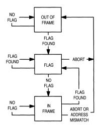
Figure 2-3. Receiver State Diagram HDLC Operation
