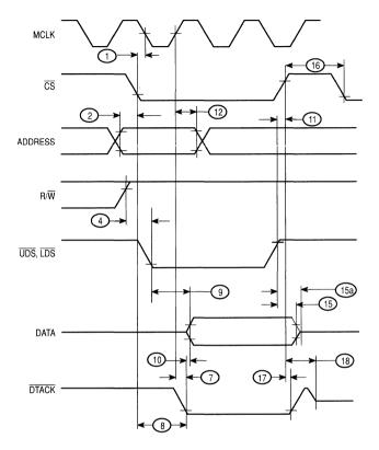
Figure 8-3. 68000 MPU Read Timing
