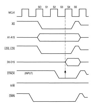
Figure 5-4. 68000 DMA Read Cycle
