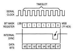
Figure 6-5. Transparent Byte Alignment
