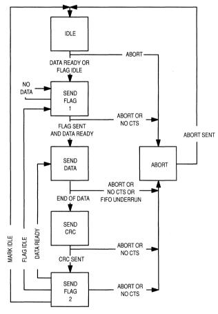
Figure 2-2. Transmitter State Diagram HDLC Operation
