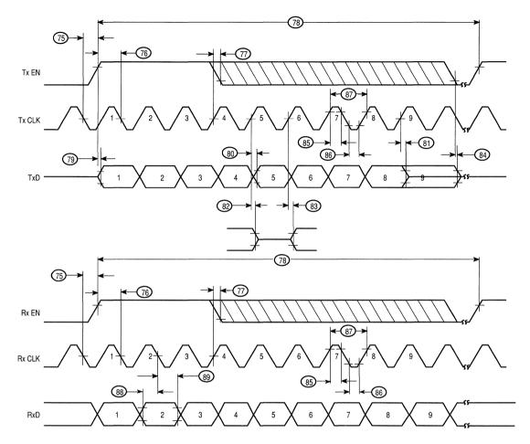
Figure 8-11. Timeslot Mode Timing Long-Frame Operation
