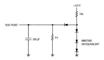
Figure 8-1. Test Load
