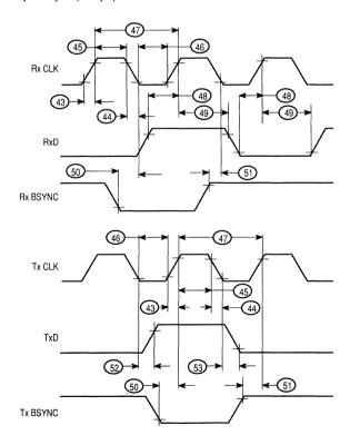
Figure 8-7. Serial Interface (Modem Mode) Timing Diagram
