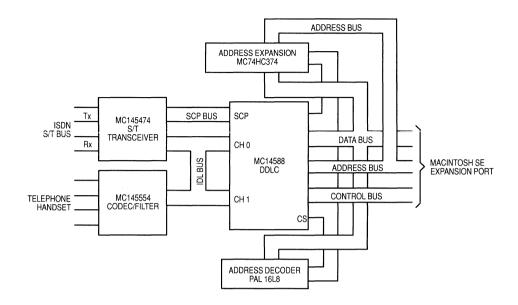
Figure 7-6. Macintosh SE ISDN Terminal Card Hardware Block Diagram
