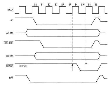
Figure 5-5. 68000 DMA Write Cycle with One Programmed Wait-State and a Delayed DTACK
