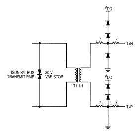
Figure 7-13. ISDN Transmit Pair Interface and Protection
