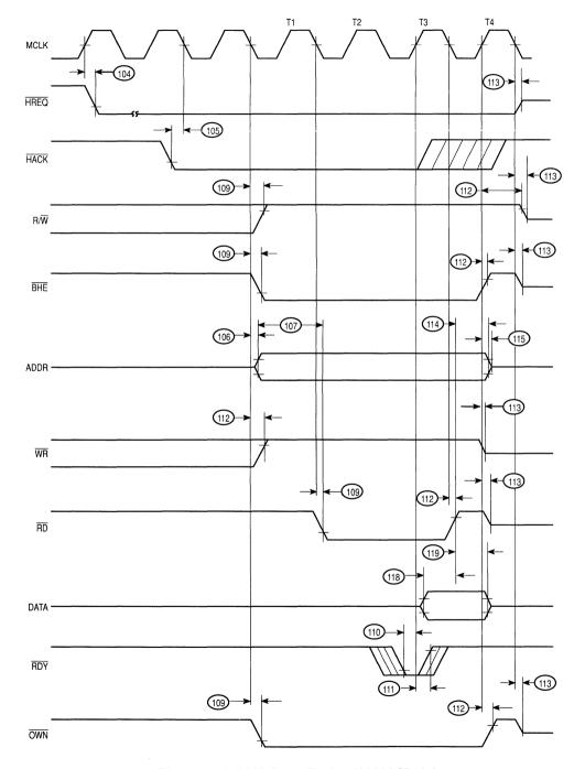
Figure 8-16. DMA Read Timing (80186 Mode)
