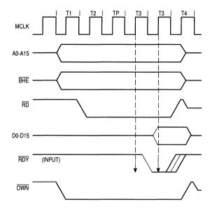
Figure 5-11. 80186 DMA Cycle with One Programmed Wait-State and Delayed RDY
