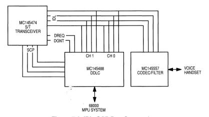
Figure 7-2. IDL. SCP Bus Connections
