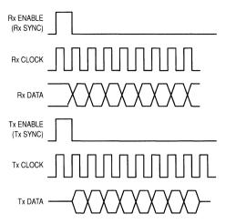
Figure 6-9. Timeslot Operation Short-Frame
