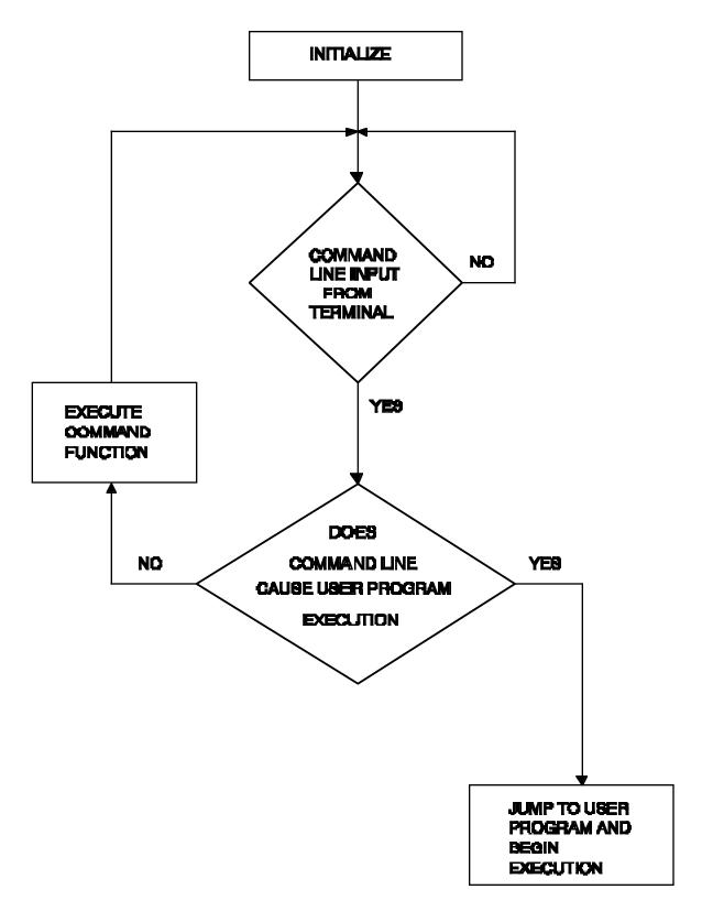
Figure 2-1. Flow Diagram of dBUG Operational Mode.
