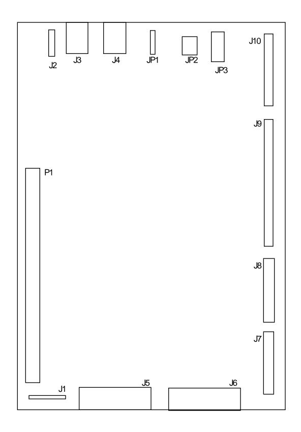
Figure 1.3. Jumper and connector placement.
