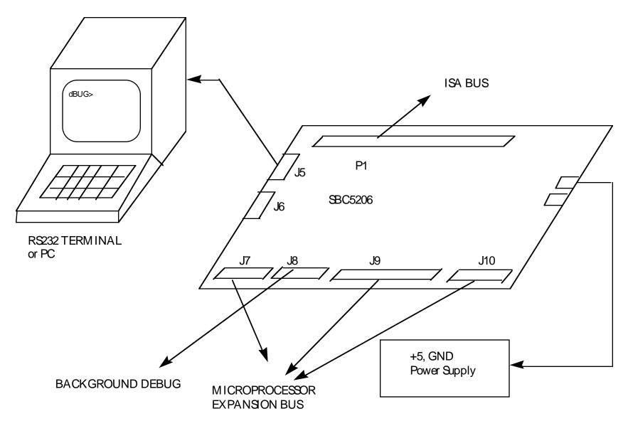
Figure 1.2. System Configuration
