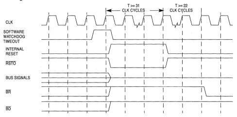
Figure 6-51. Software Watchdog Timer Reset Timing
