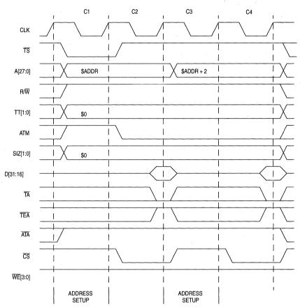
Figure 9-6. Longword Burst Read Transfer from a 16-Bit Port (No Wait States, Address Setup, No Address Hold)
