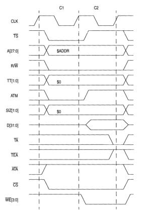
Figure 9-2. Longword Write Transfer from a 32-Bit Port (No Wait State, No Address Setup, No Address Hold)
