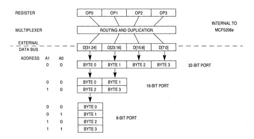
Figure 6-3. MCF5206e Interface to Various Port Sizes
