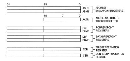
Figure 15-6. Debug Programming Model
