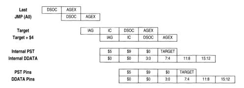
Figure 15-2. Pipeline Timing Example (Debug Output)
