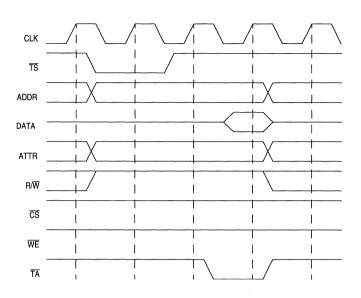
Figure 9-19. Default Memory Address Hold Timing with RDAH = 0
