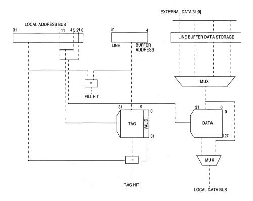
Figure 4-1. Instruction Cache Block Diagram
