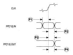
Figure 17-14. General-Purpose I/O Port Timing
