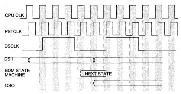
Figure 15-3. DBM Serial Transfer
