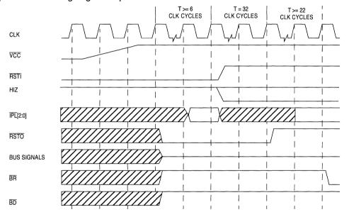
Figure 6-50. Normal Reset Timing
