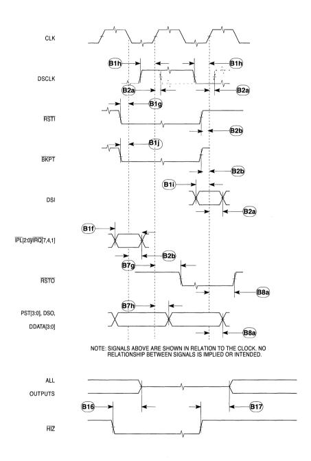
Figure 17-10. Miscellaneous Signal Timing
