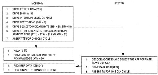
Figure 6-30. Interrupt-Acknowledge Cycle Flowchart
