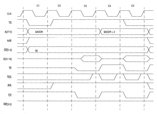
Figure 9-10. External Master Longword Read Transfer from a 16-Bit Port (No Wait State, With Address Setup Or Read Address Hold)
