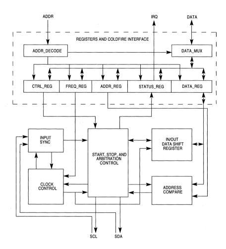
Figure 13-1. M-Bus Module Block Diagram
