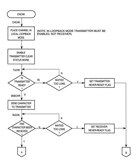
Figure 11-9. UART Software Flowchart (2 of 5)
