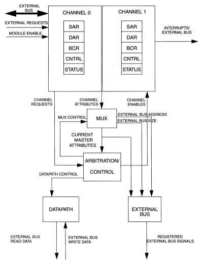
Figure 7-1. DMA Signal Diagram
