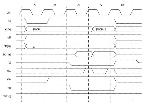
Figure 9-9. External Master Longword Read Transfer from a 16-bit Port (No Wait State, No Address Setup, No Address Hold)
