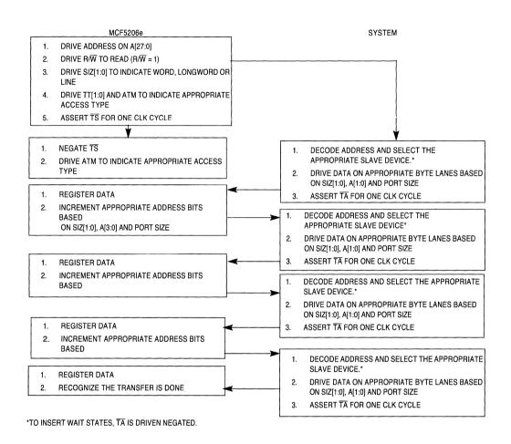
Figure 6-8. Bursting Word-, Longword-, and Line-Read Transfer Flowchart
