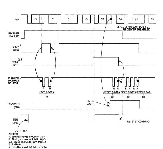
Figure 12-6. Receiver Timing Diagram
