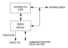
Figure 15-1. Processor/Debug Module Interface
