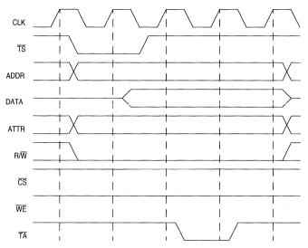
Figure 9-18. Default Memory Address Hold Timing with WRAH = 1
