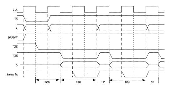
Figure 11-19. Fast Page Mode or Burst Page Mode DRAM Transfer Timing
