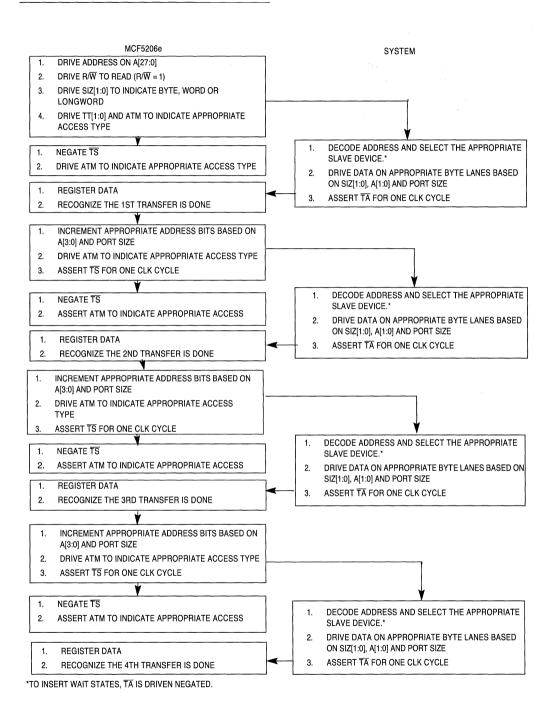
Figure 6-12. Burst-Inhibited Word-, Longword-, and Line-Read Transfer Flowchart
