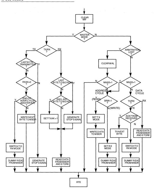
Figure 13-4. Flow-Chart of Typical M-Bus Interrupt Routine
