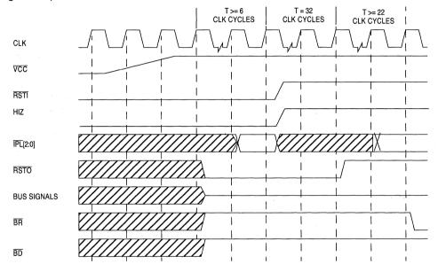
Figure 6-49. Master Reset Timing
