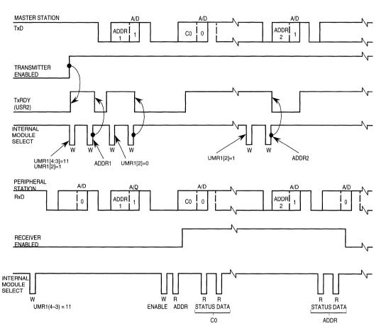
Figure 12-8. Multidrop Mode Timing Diagram
