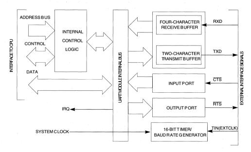
Figure 12-2. External and Internal Interface Signals
