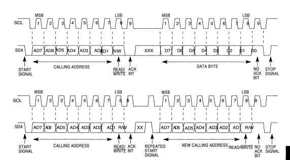
Figure 13-2. M-Bus Standard Communication Protocol
