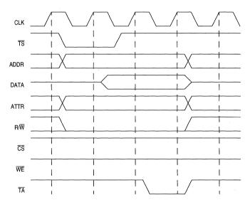
Figure 9-17. Default Memory Address Hold Timing with WRAH = 0
