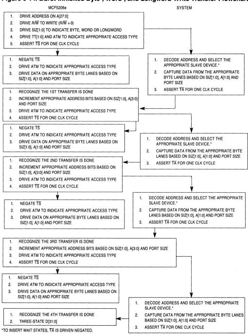
Figure 6-15 shows a burst-inhibited supervisor data longword-write transfer to a 16-bit port.
