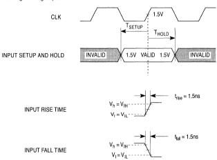
Figure 17-2. Input Timing Waveform Requirements
