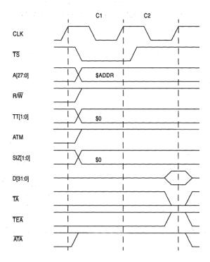
Figure 6-5. Longword-Read Transfer From a 32-Bit Port (No Wait States)
