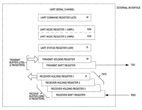
Figure 12-4. Transmitter and Receiver Functional Diagram
