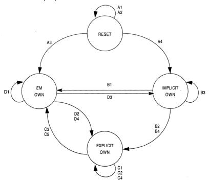
Figure 6-40. MCF5206e Bus Arbitration Protocol State Diagram
