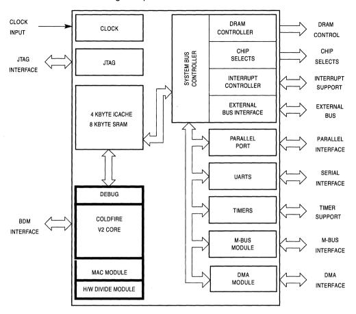
Figure 1-1. MCF5206e Block Diagram
