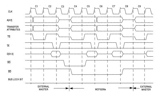
Figure 6-35. Two-Wire Bus Arbitration with Bus Lock Negated
