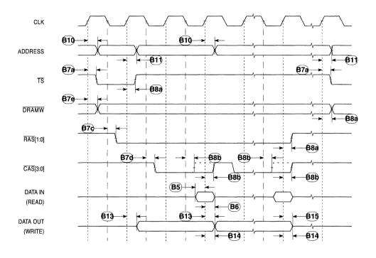
Figure 17-7. DRAM Signal Timing
