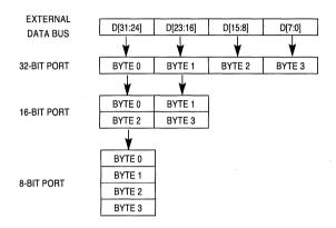
Figure 11-1. MCF5206e Interface to Various Port Sizes
