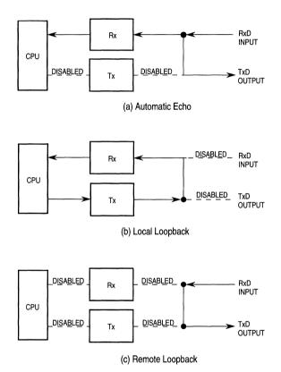
Figure 12-7. Looping Modes Functional Diagram
