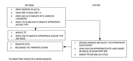
Figure 6-4. Byte-, Word-, and Longword-Read Transfer Flowchart
