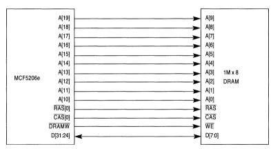
Figure 11-4. Diagram for 1 MByte DRAM with 8 Bit Port and 1 KByte Page
