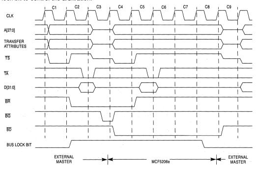
Figure 6-39. Three-Wire Bus Arbitration with Bus Lock Bit Asserted
