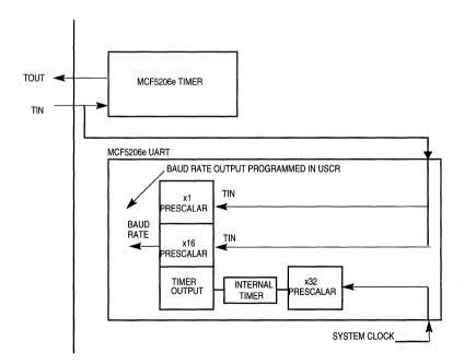
Figure 12-3. Baud-Rate Timer Generator Diagram
