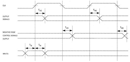
TVO = PROPAGATION DELAY OF SIGNAL RELATIVE TO CLK EDGE
