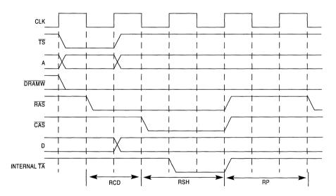
Figure 11-17. Normal Mode DRAM Transfer Timing
