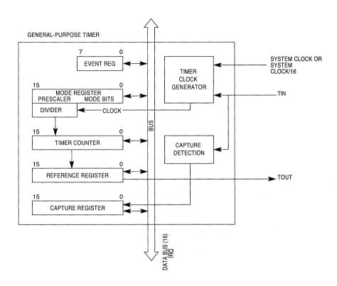
Figure 14-1. Timer Block Diagram Module Operation
