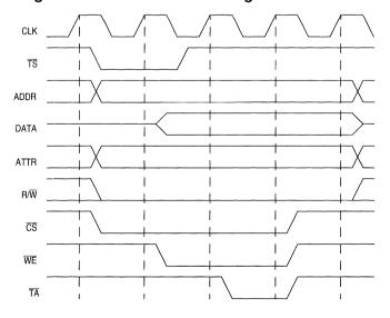
Figure 9-14. Address Hold Timing with WRAH = 1
