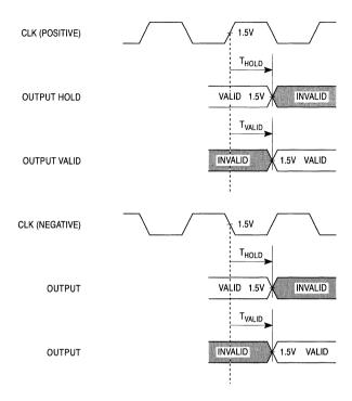
Figure 17-3. Output Timing Waveform
