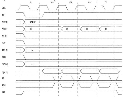
Figure 6-11 shows a user data bursting line-write transfer to a 32-bit port.
