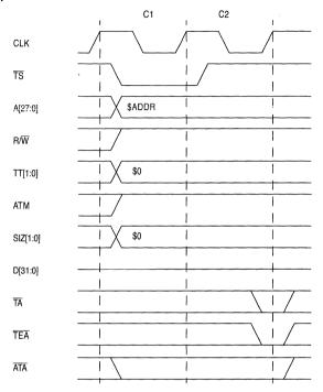
Figure 6-32. Bursting Longword-Read Access from 16-Bit Port Terminated with TEA Timing
