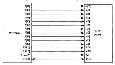
Figure 11-3. Diagram for 4 MByte DRAM with 8 bit Port and 1 KByte Page
