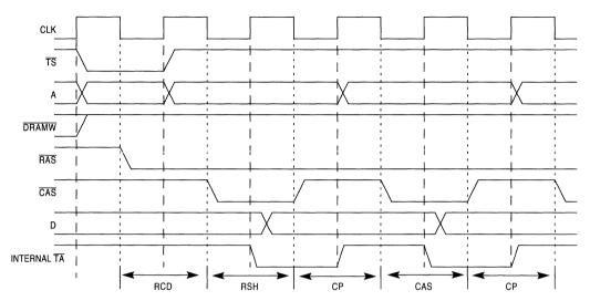
Figure 11-21. Fast Page Mode or Burst Page Mode EDO DRAM Transfer Timing
