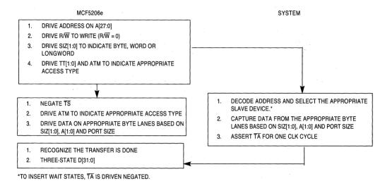
Figure 6-6. Byte-, Word-, and Longword-Write Transfer Flowchart
