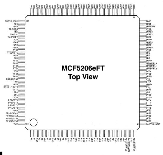
Figure 18-1. MCF5206e Package Diagram & Pinout
