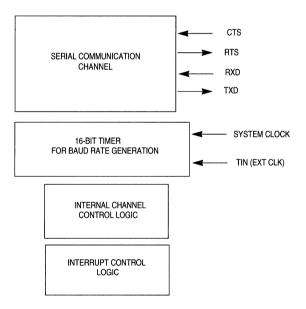
Figure 12-1. UART Block Diagram
