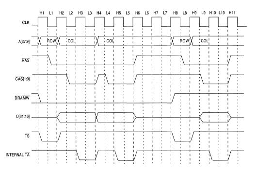
Figure 11-12. Longword Write Transfer Followed by a Word Read Transfer in Burst Page Mode with 16-Bit DRAM
