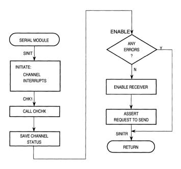
Figure 11-9. UART Software Flowchart (1 of 5)
