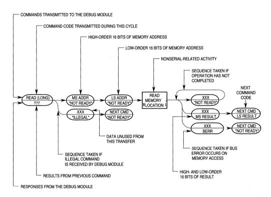
Figure 15-5. Command Sequence Diagram
