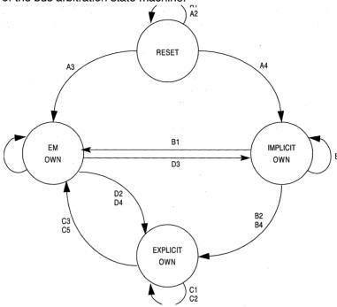
Figure 6-37. MCF5206e Two-Wire Bus Arbitration Protocol State Diagram
