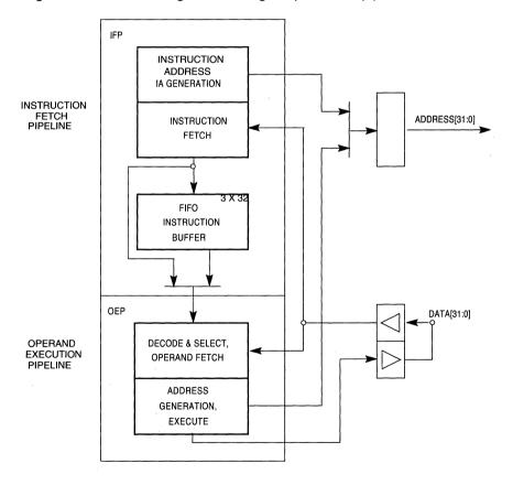
Figure 3-1. ColdFire Processor Core Pipelines
