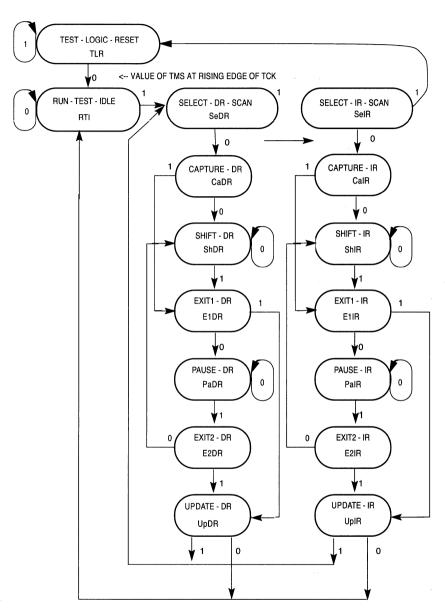
Figure 16-2. JTAG TAP Controller State Machine
