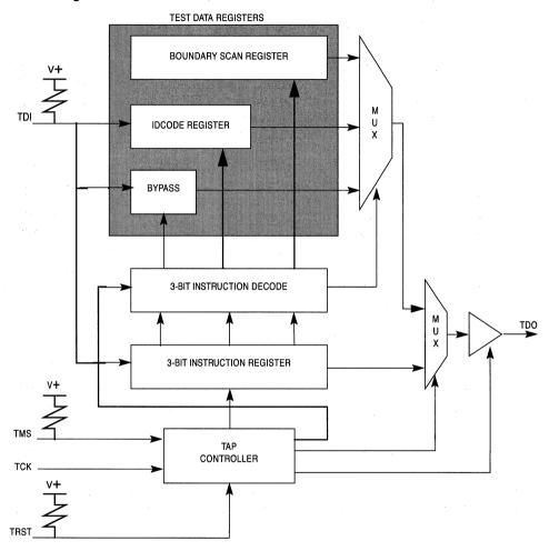
Figure 16-1. JTAG Test Logic Block Diagram
