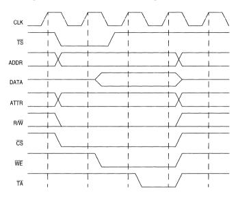
Figure 9-13. Address Hold Timing with WRAH = 0
