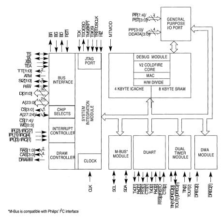
Figure 2-1. MCF5206e Block Diagram
