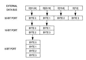
Figure 9-1. MCF5206e Interface to Various Port Sizes
