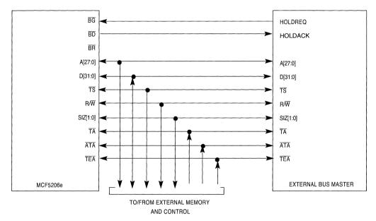
Figure 6-33. MCF5206e Two-Wire Mode Bus Arbitration Interface
