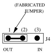
**NOTE**: Using the F4EM with the fabricated jumper installed between pins 2 and 3 will interfere with correct operation of the RESETIN and RESETOUT commands. The J4 pins 2-and-3 configuration is **not** correct for a F4EM that is part of an MMDS05 system.
