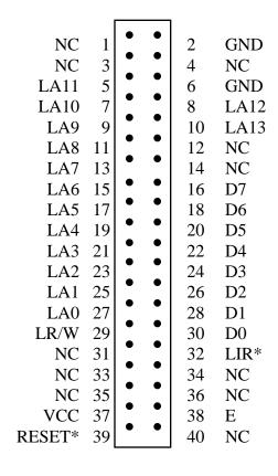
Figure 3-1. Connector P1 Pin Assignments
