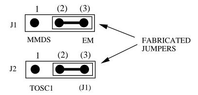
Alternatively, you may use a clock source originating from the MMDS05 control board. To do so, reposition the J1 jumper between pins 1 and 2. Then use the MMDS OSC command to select clock frequency.
