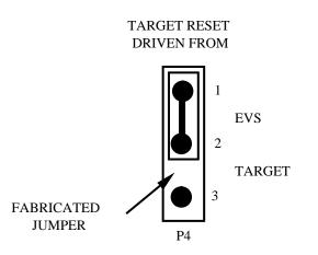
Alternatively, you may enable the target system to reset the L1EVS. To do so:
