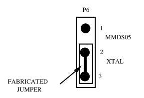
Alternatively, you may use a clock source originating from the control board. To do so, reposition the P6 jumper between pins 1 and 2, then use the MMDS05 OSC command to select a frequency.
