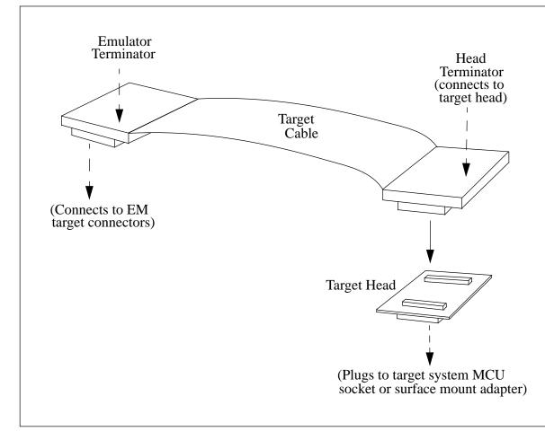
Figure 1-3 A Generic Representation of Target Cable assembly
