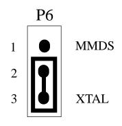
Alternatively, you may use a clock source originating from the control board. To do so, reposition the P6 jumper between pins 1 and 2, then use the MMDS05 OSC command to select a frequency.
