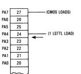
PORT A, BIT 7 PROGRAMMED AS OUTPUT, DRIVING CMOS LOADS AND BIT 4 DRIVING ONE LSTTL LOAD DIRECTLY (USING CMOS OUTPUT OPTION).
