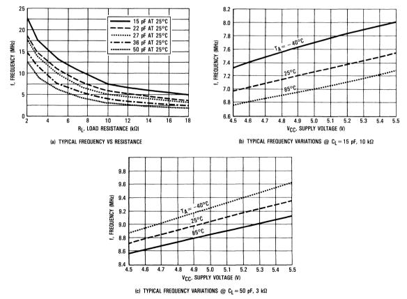
Figure 4-8. Typical Frequency Selection for Resistor-Capacitor Oscillator Options
