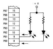
PORT B, BIT O, AND BIT 1 PROGRAMMED AS OUTPUT, DRIVING LEDs DIRECTLY.
