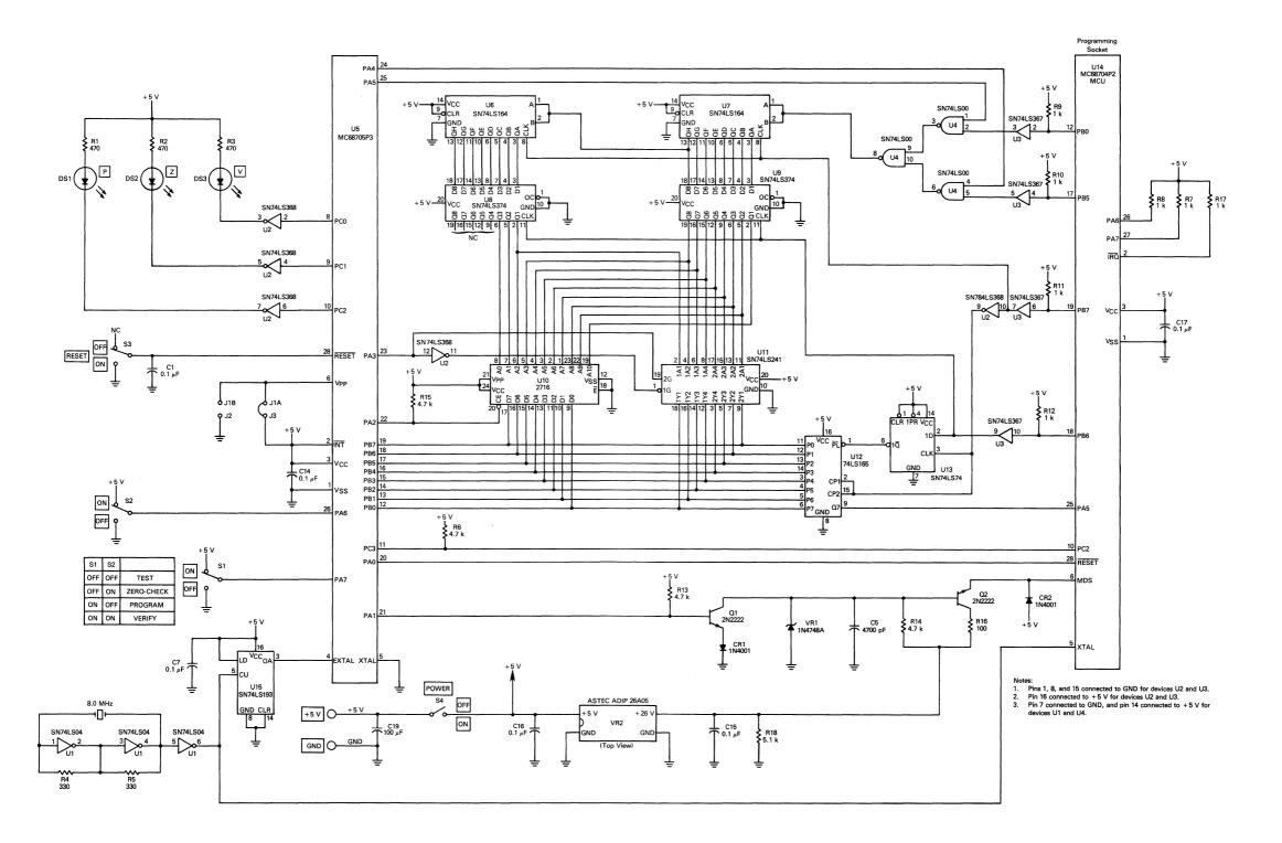
Figure D-1. MC68704P2 EPROM MCU Programming Board/Circuitry
