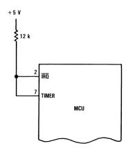
Figure 4-3. Timer Interrupt Connection
