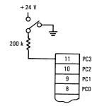
(USE OF LOW CURRENT CLAMPING DIODE TO CLAMP VOLTAGES >> VCC.) LSTTL/OPEN-DRAIN OPTIONS ONLY
