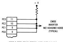
PORT C OPEN DRAIN OPTION, WITH BITS 0-3 PRO-GRAMMED AS OUTPUT, DRIVING CMOS LOAD VIA WIRED-ORed CONFIGURATION.
