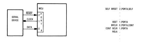
Figure 6-1. Bit Manipulation Example
