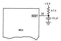
Figure 4-5. Power-Up Reset Delay Circuit
