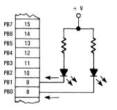
PORT B, BIT O, AND BIT 1 PROGRAMMED AS OUTPUT, DRIVING LEDS DIRECTLY.
