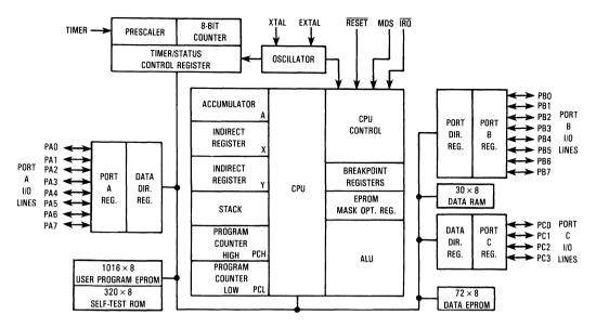
Figure C-1. MC68704P2 Block Diagram
