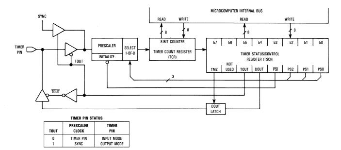
Figure 3-1. Timer Block Diagram
