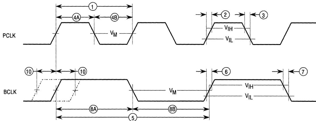
Figure 7. Clock Input Timing Diagram
