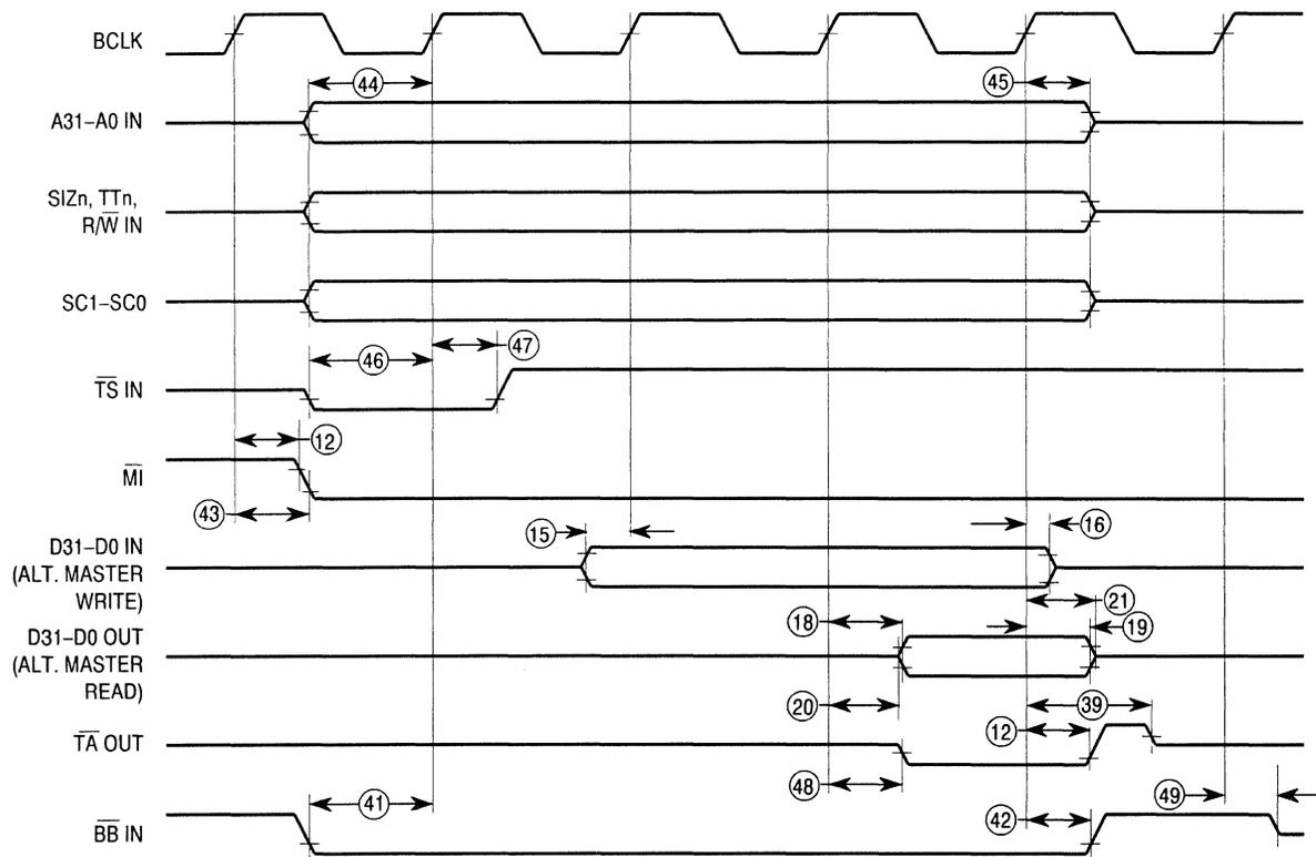
Figure 10. Snoop Hit Timing
