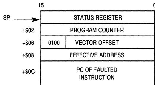
Figure 4. Floating-Point Unimplemented Instruction Stack Frame
