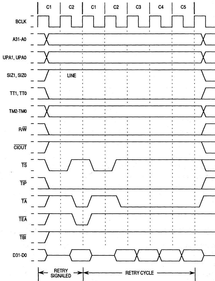
Figure 8-27. Retry Operation on Line Write
