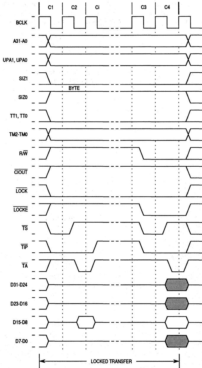
Figure 8-18. Locked Transfer for TAS Instruction
