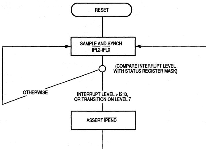
**Figure 9-2. Interrupt Pending Procedure**
