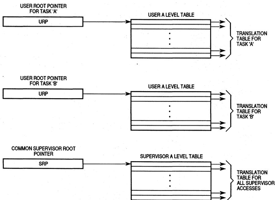
**Figure 6-20. Translation Tree Structure for Two Tasks — Example**
