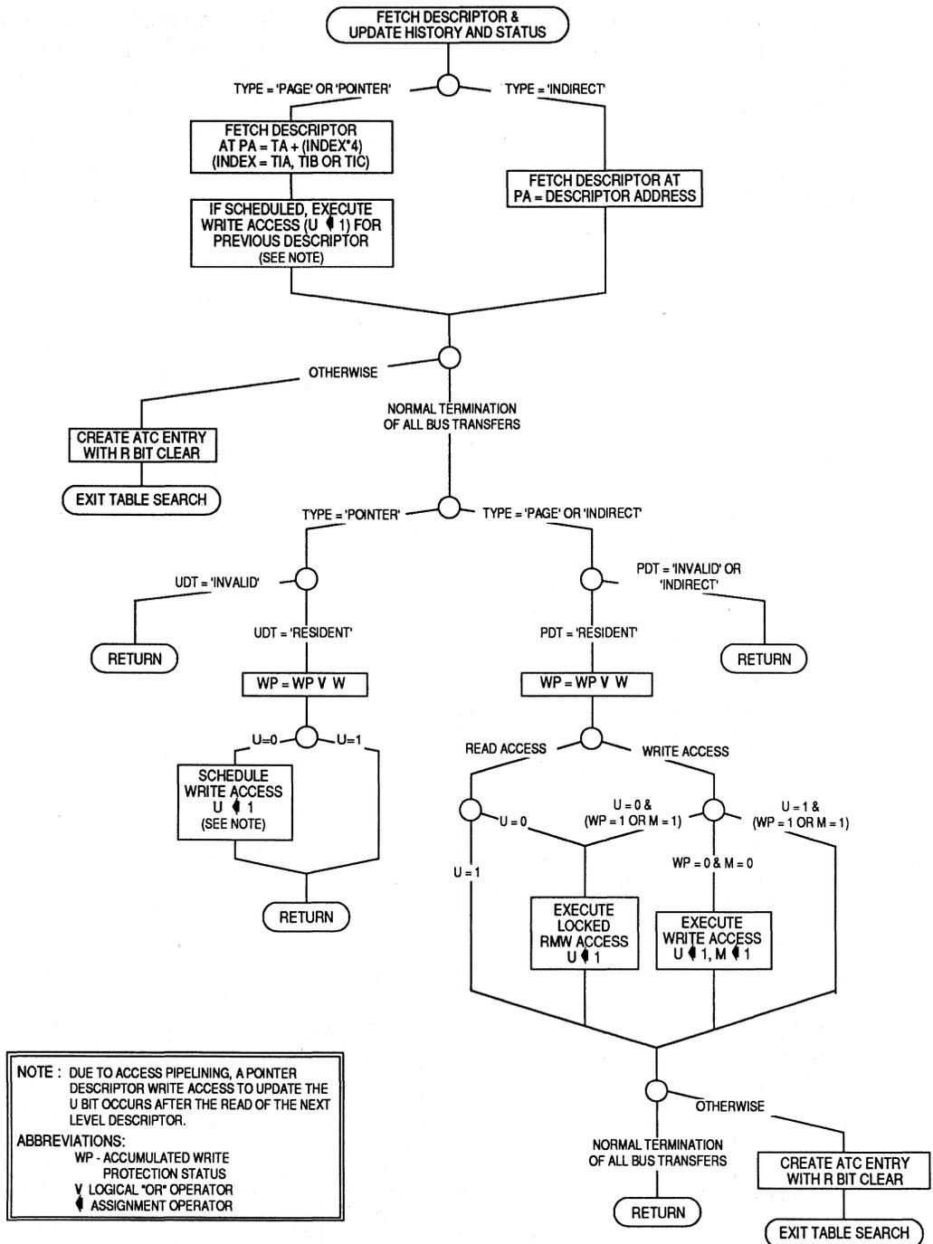
Figure 6-19. Detailed Flowchart of Descriptor Fetch Operation
