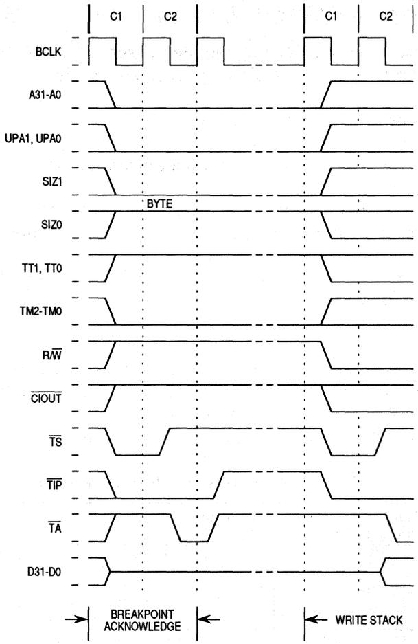
Figure 8-23. Breakpoint Acknowledge Cycle Timing
