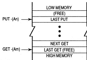
To implement the queue as a circular buffer, the "get" or "put" operation should be performed first, and then the relevant address register should be checked and adjusted, if necessary. The address register is adjusted by adding the buffer length (in bytes) to the register contents.
