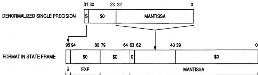
**Figure 9-9. Format of Denormalized Single Precision Source Operand in State Frame**
