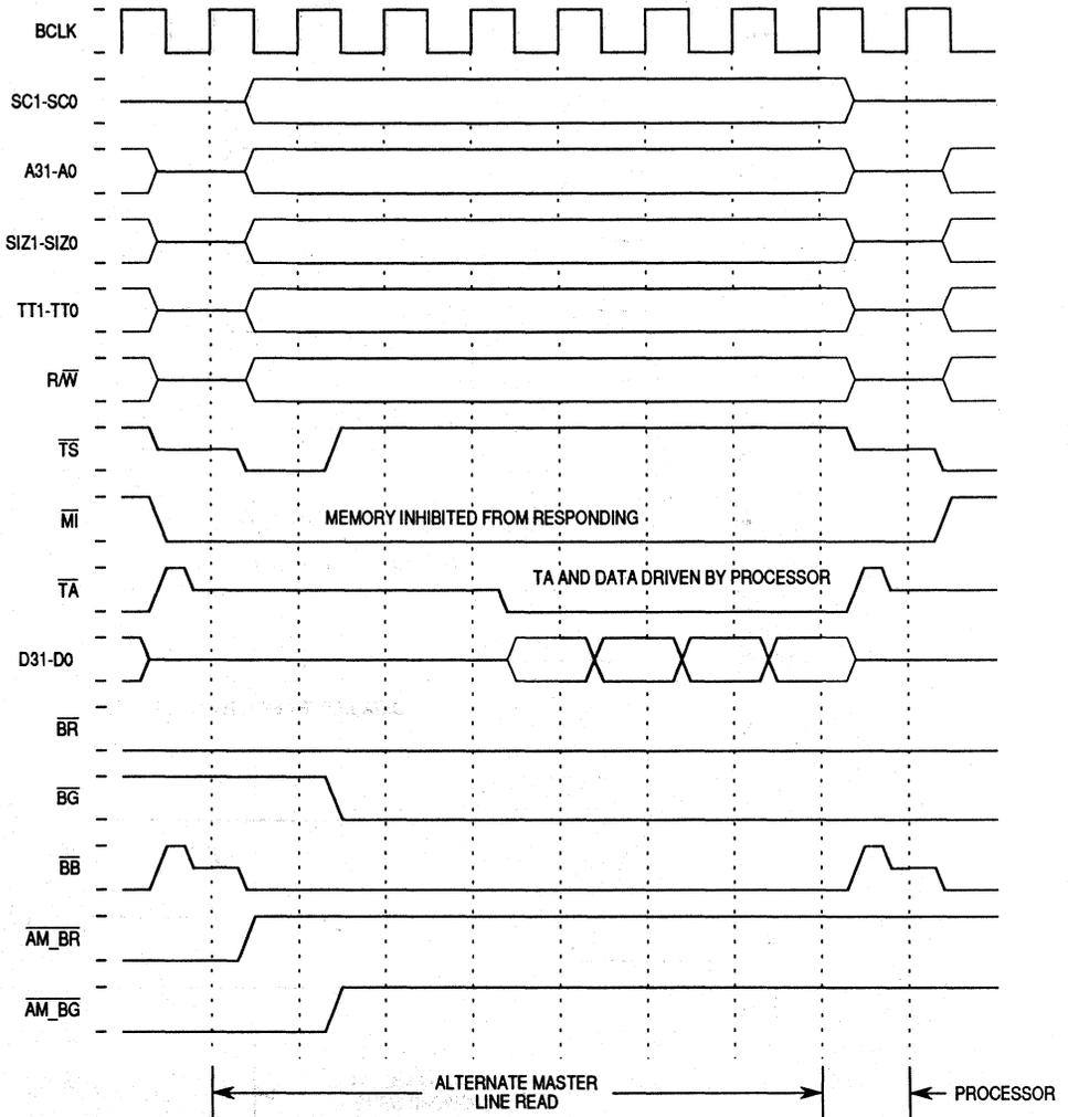
Figure 8-33. Snoop Line Read, Memory Inhibited
