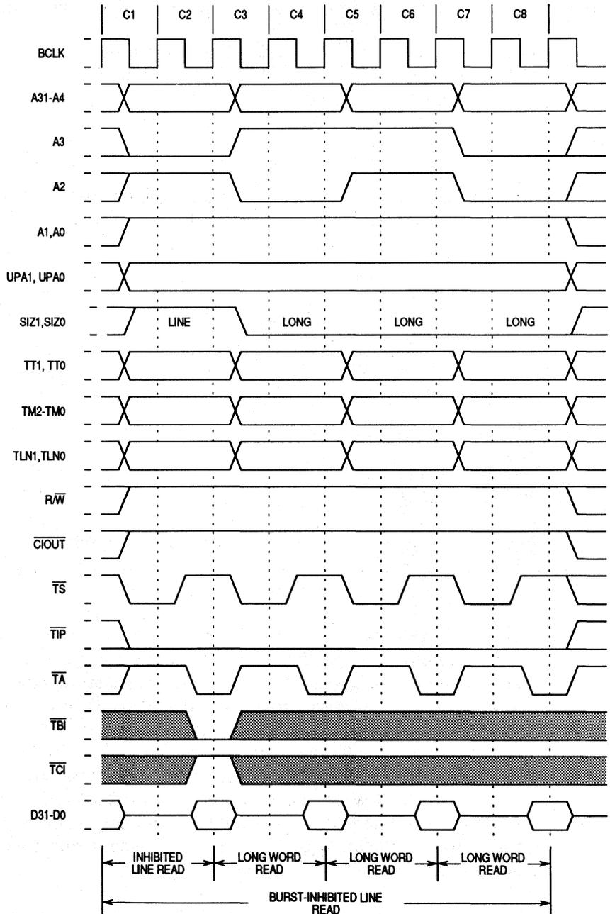
Figure 8-13. Burst-Inhibited Line Read
