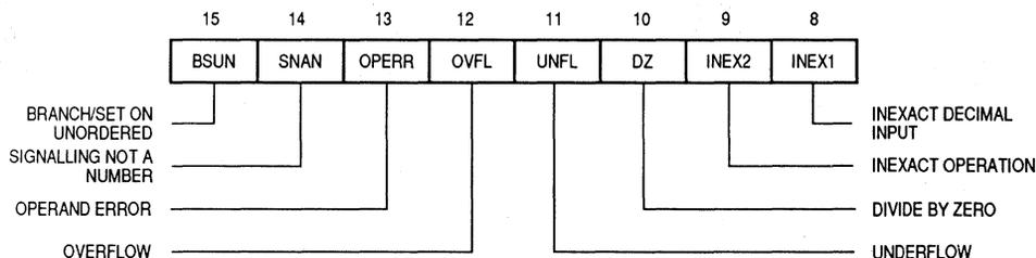
**Figure 2-3. FPCR Exception Enable Byte**
