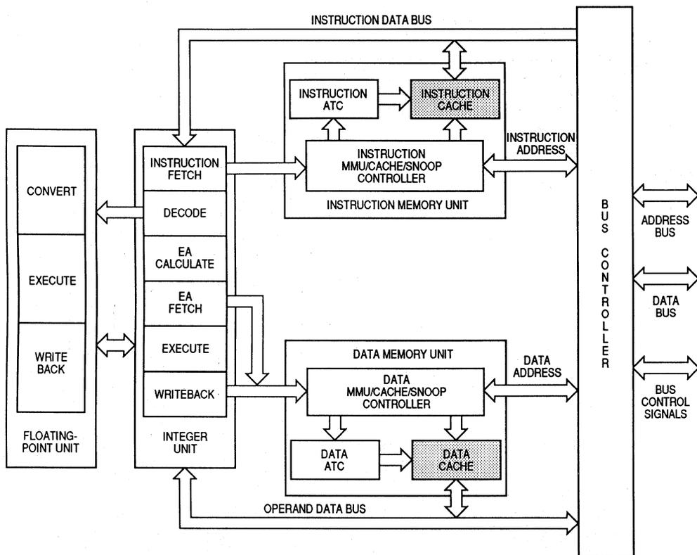
**Figure 7-1. Overview of Internal Caches**
