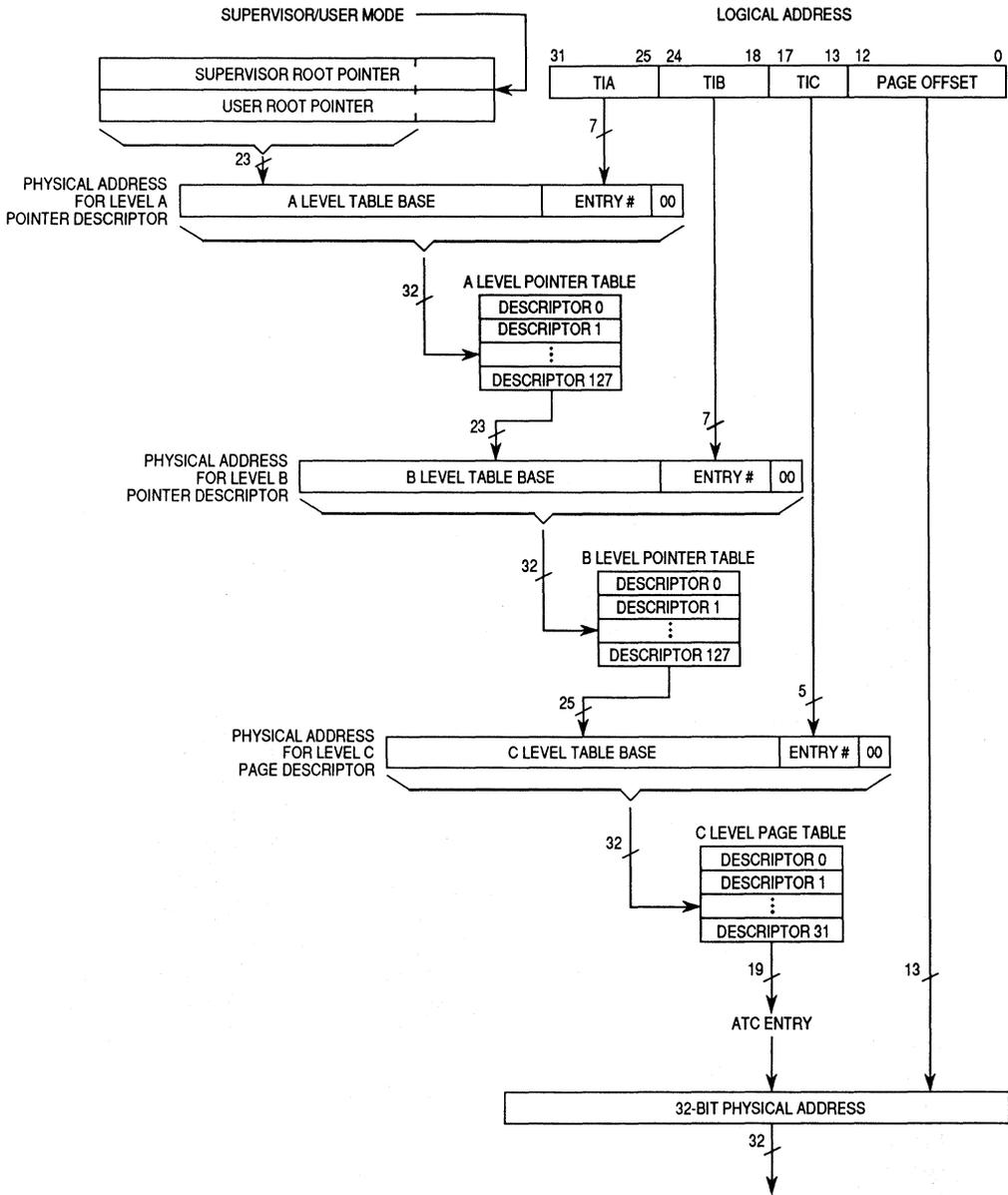
Figure 6-14. Physical Address Generation (8K Page Size)
