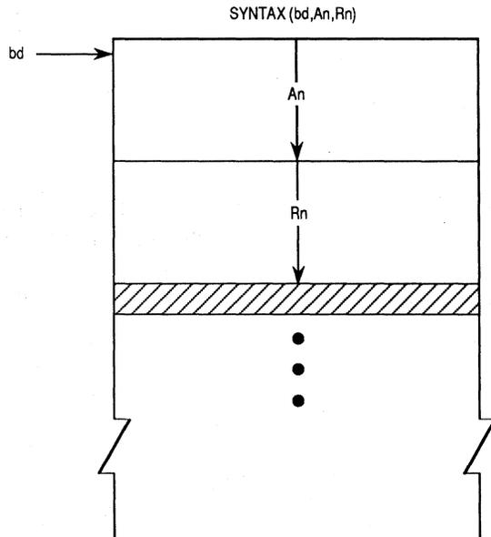
**Figure 3-16. Using Absolute Address with Indexes**
