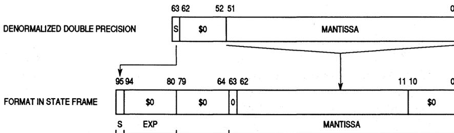
**Figure 9.10. Format of Denormalized Double Precision Source Operand in State Frame**
