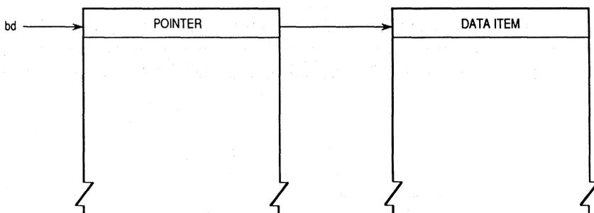
**Figure 3-18. Using Indirect Absolute Memory Addressing**
