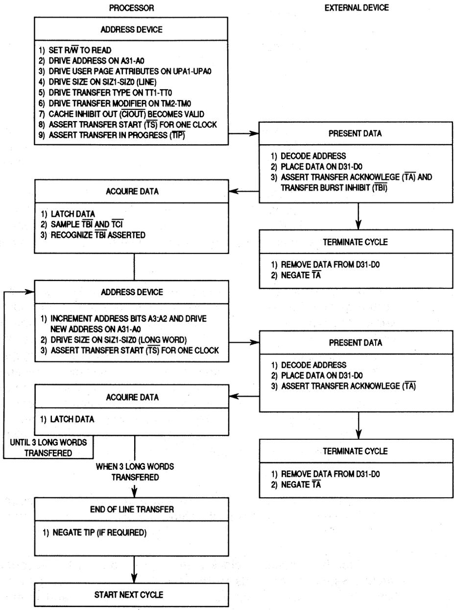
Figure 8-12. Burst-Inhibited Line Read Flowchart
