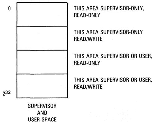
**Figure 6-21. Logical Address Map with Shared Supervisor and User Address Spaces — Example**
