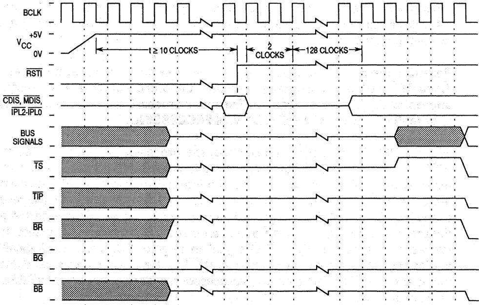
Figure 8-38. Initial Power-On Reset Timing
