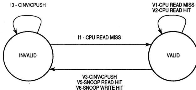
**Figure 7-4. Instruction-Cache-Line State Diagram**
