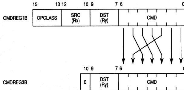
**Figure 9-8. Mapping of Command Bits for CMDREG3B Field**
