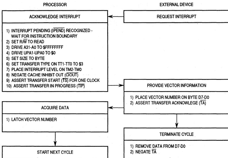
**Figure 8-19. Interrupt Acknowledge Cycle Flowchart**
