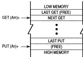
To implement the queue as a circular buffer, the relevant address register should be checked and adjusted, if necessary, before performing the "put" or "get" operation. The address register is adjusted by subtracting the buffer length (in bytes) from the register.
