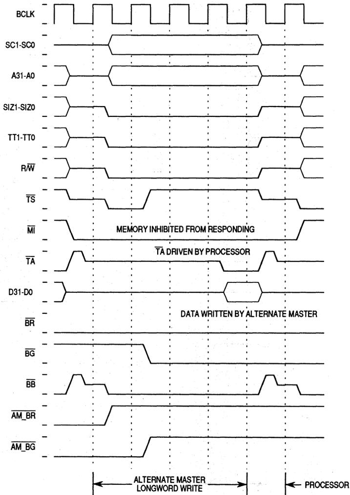
Figure 8-34. Snoop Longword Write, Memory Inhibited
