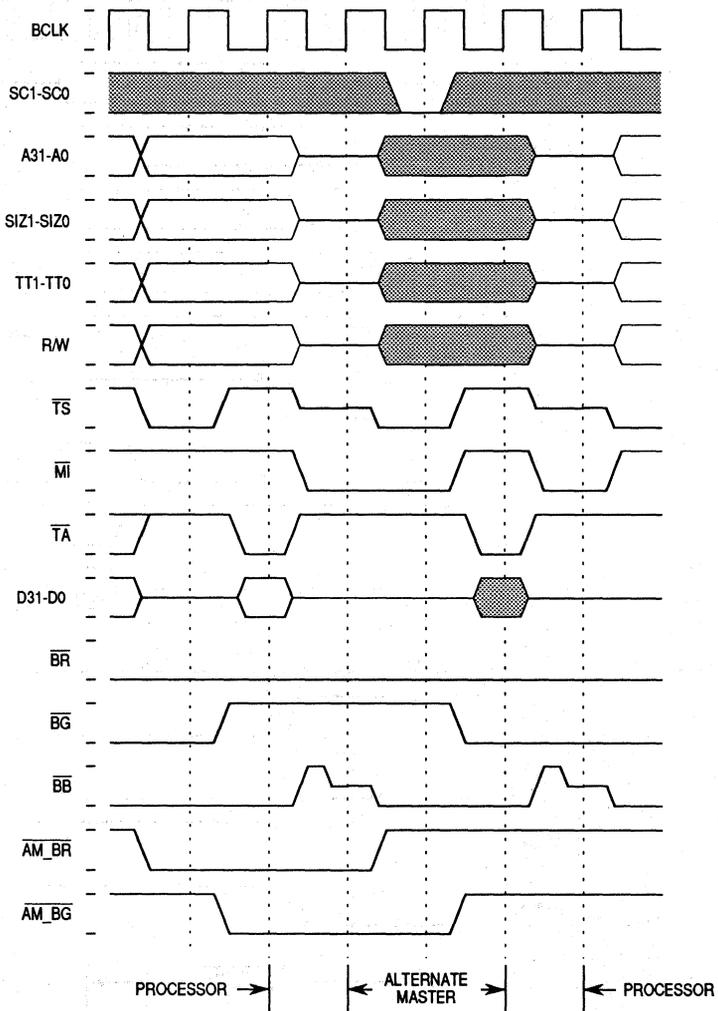
**Figure 8-31. Snoop Inhibited Bus Cycle**
