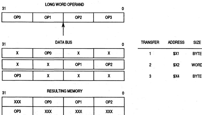
**Figure 8-4. Example of a Misaligned Long-Word Read Transfer**
