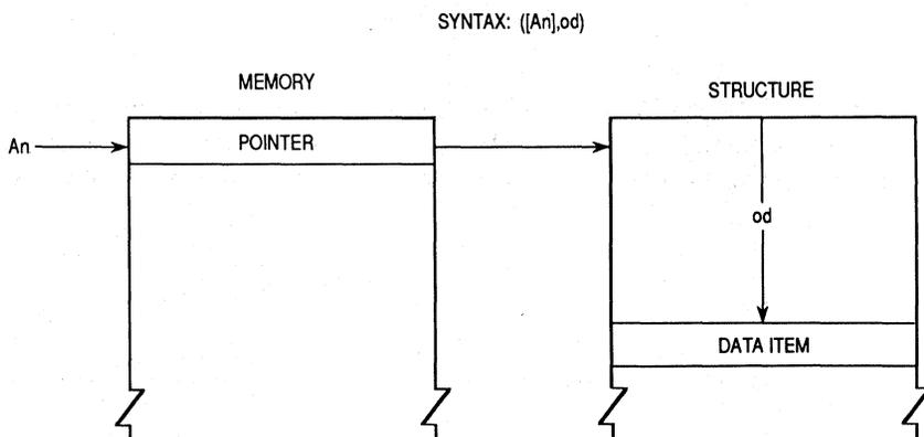
**Figure 3-19. Accessing an Item in a Structure Using Pointer**
