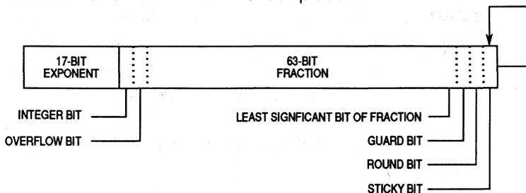
**Figure 9-11. Intermediate Results Format**
