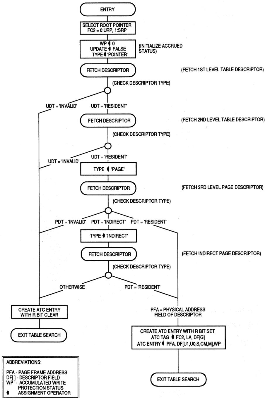
Figure 6-18. Detailed Flowchart of Table Search Operation
