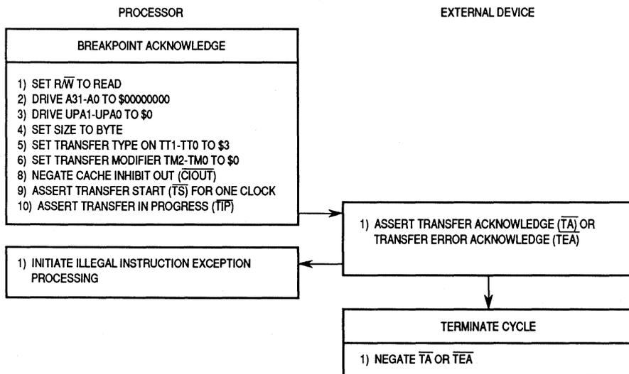
Figure 8-22. Breakpoint Operation Flow
