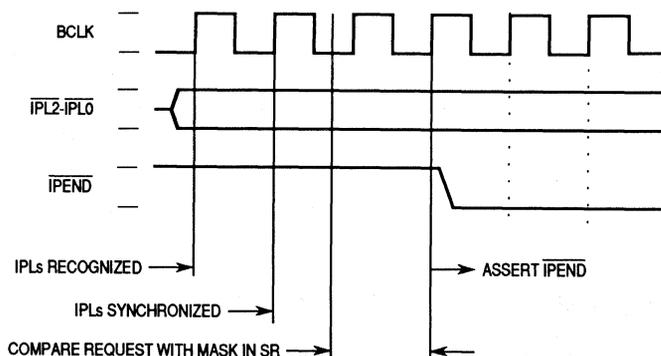
**Figure 9-4. Assertion of  $\overline{\text{IPEND}}$**
