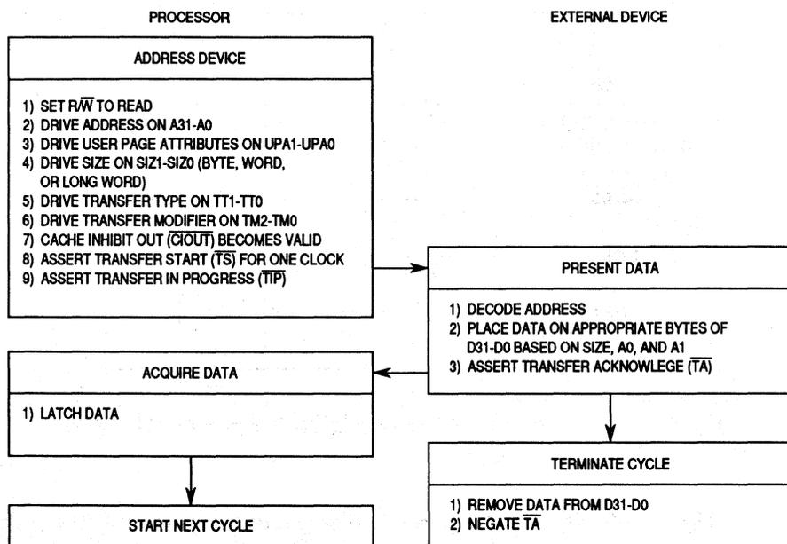
Figure 8-8. Byte, Word, and Long-Word Read Cycle Flowchart
