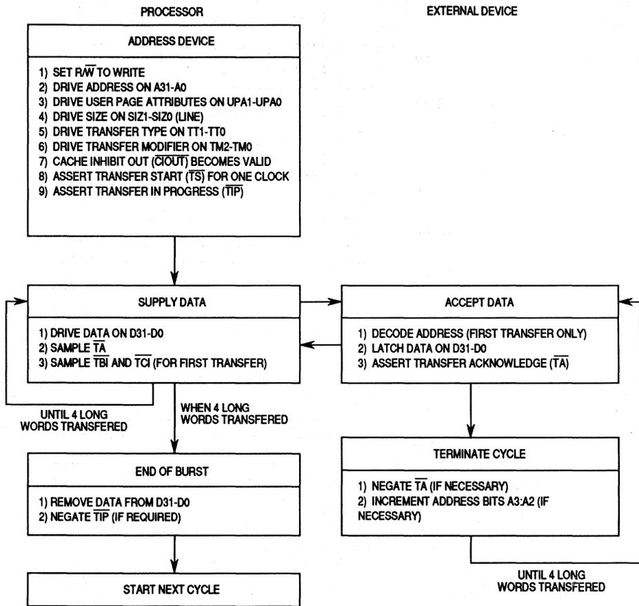
**Figure 8-16. Line Write Cycle Flowchart**
