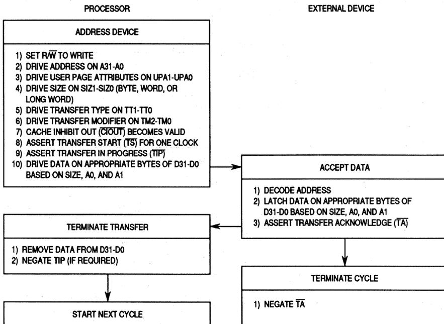
**Figure 8-14. Byte, Word, and Long-Word Write Cycle Flowchart**
