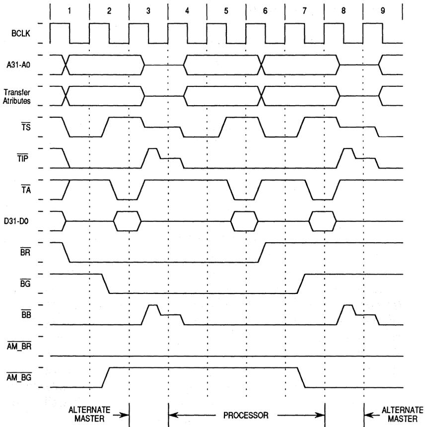
**Figure 8-28. Processor Bus Request Example**
