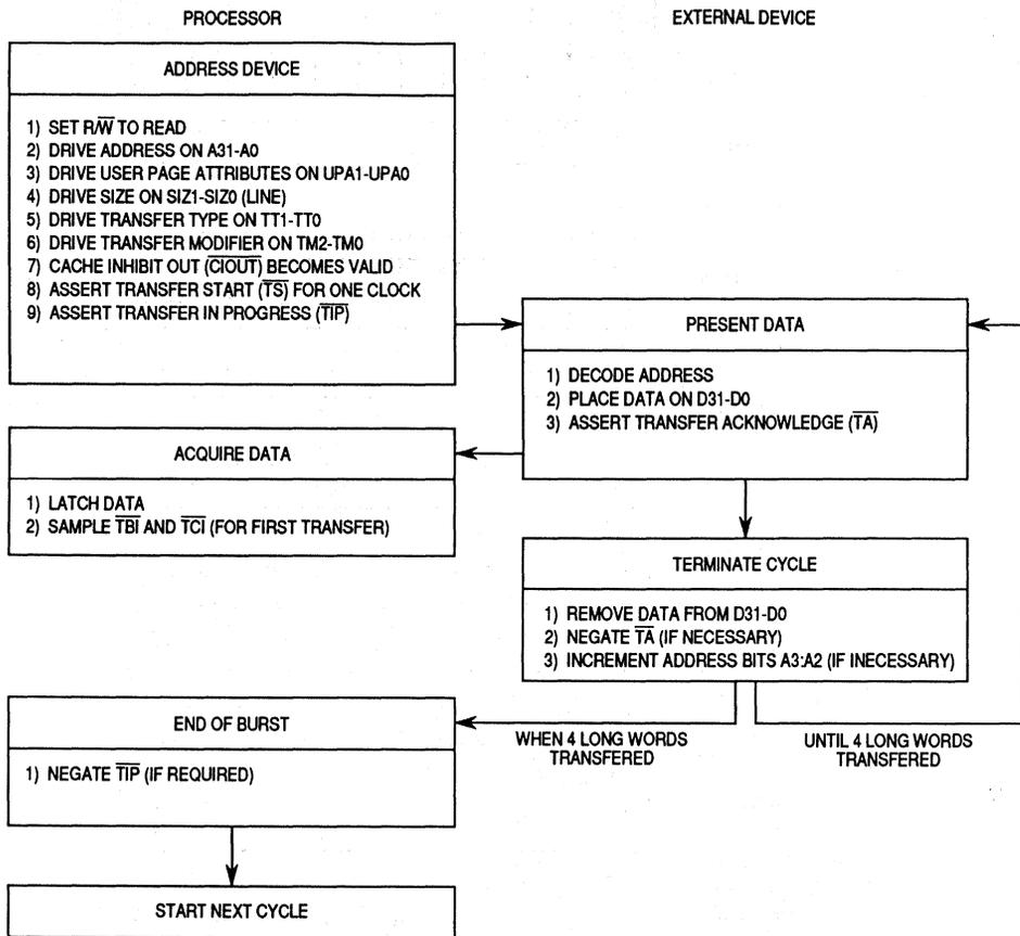
**Figure 8-10. Line Read Cycle Flowchart**
