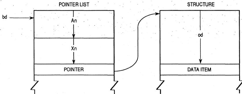
**Figure 3-23. Preindexed Indirect with Outer Displacement**
