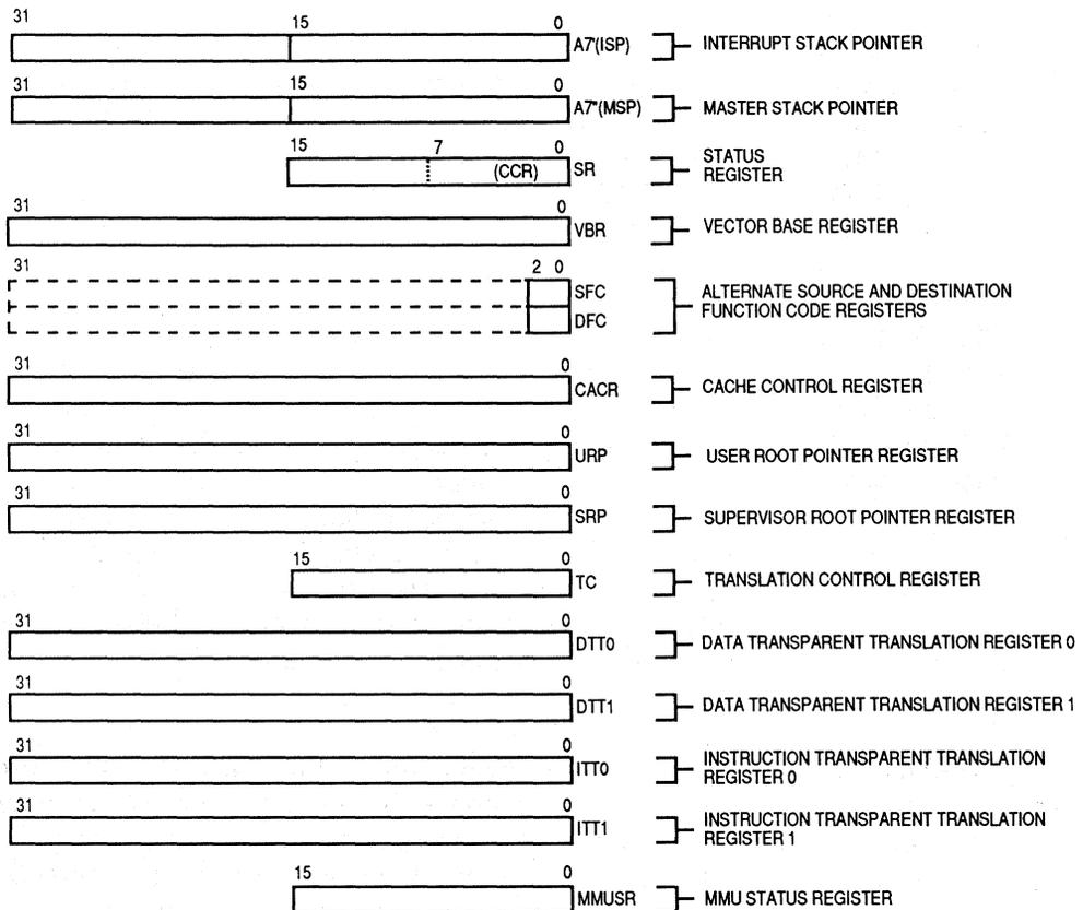
Figure 2-9. Supervisor Programming Model
