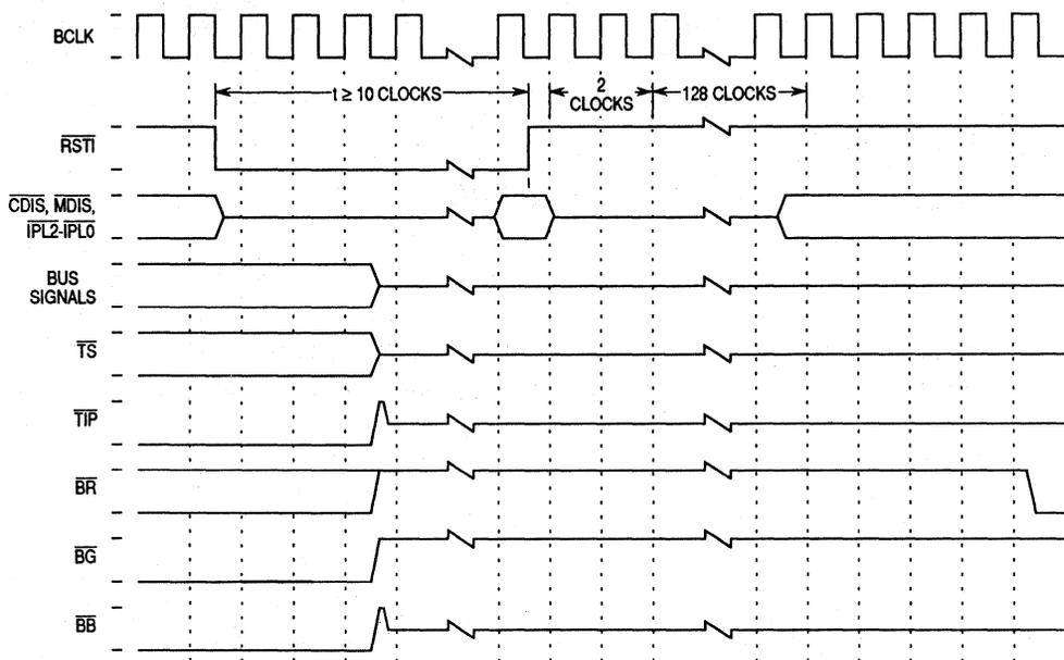
Figure 8-39. Normal Reset Timing
