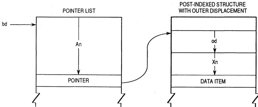
Figure 3-24. Postindexed Indirect Addressing with Outer Displacement
