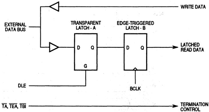
Figure 8-36. DLE Mode Block Diagram
