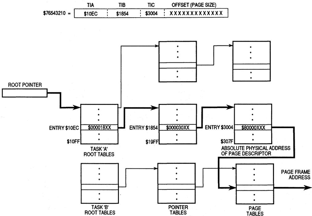
Figure 6-15. Translation Tree Using Indirect Descriptors — Example
