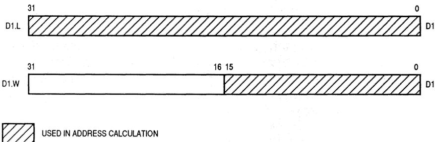
**Figure 3-15. Using SIZE in the Index Selection**
