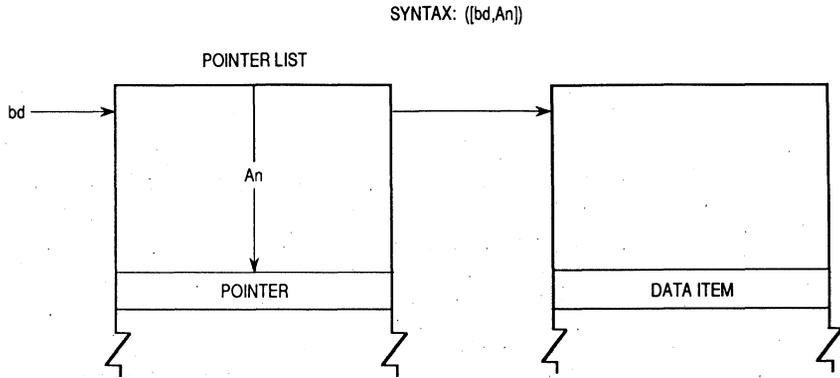
**Figure 3-20. Indirect Addressing, Suppressed Index Register**
