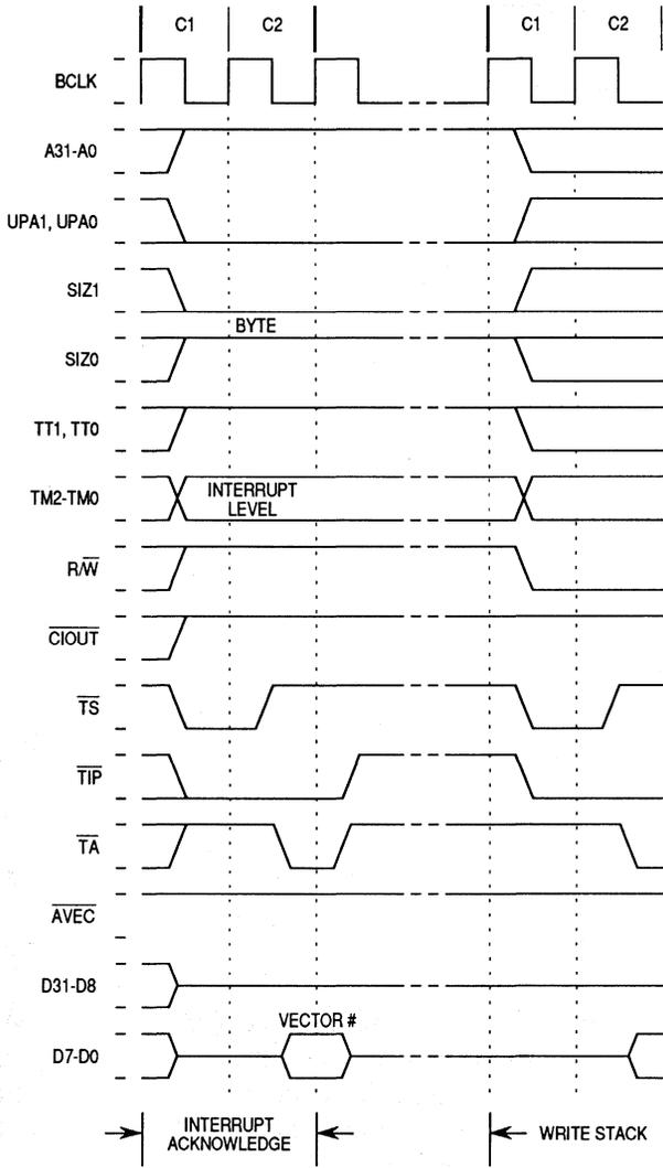
Figure 8-20. Interrupt Acknowledge Cycle Timing
