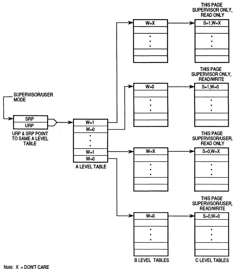
Figure 6-22. Translation Tree Using S and W Bits To Set Protection — Example
