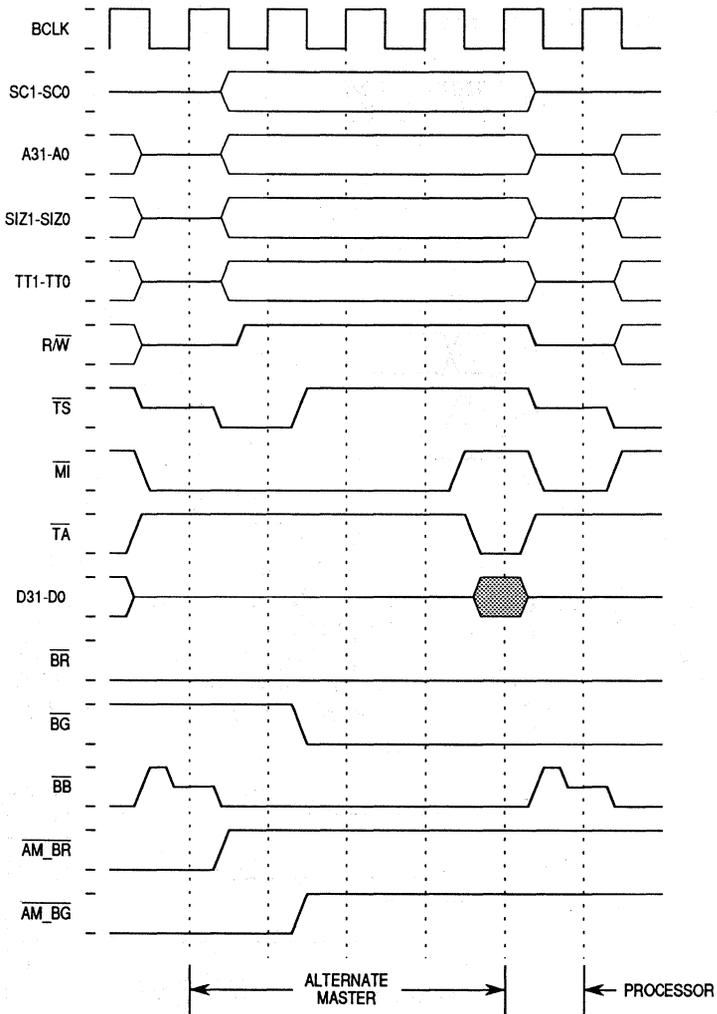
Figure 8-32. Snoop Access with Memory Response
