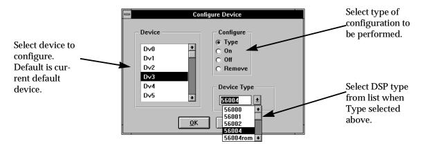
Figure 9-60. MODIFY//DEVICE//CONFIGURE Dialog Box
