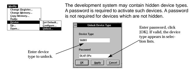
Figure 9-61. MODIFY//DEVICE//UNLOCK Dialog Box
