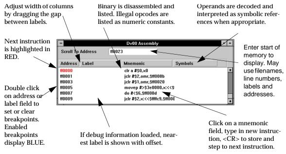
Figure 9-72. ASSEMBLY Window
