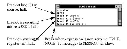
Figure 9-45. DISPLAY//BREAKPOINTS Output
