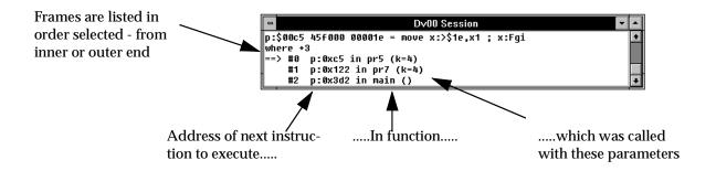
Figure 9-38. DISPLAY//CALL STACK Output
