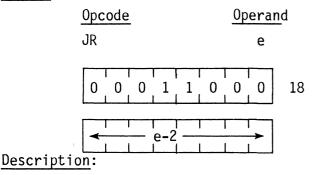
This instruction provides for unconditional branching to other segments of a program. The value of the displacement e is added to the Program Counter (PC) and the next instruction is fetched from the location designated by the new contents of the PC. This jump is measured from the address of the instruction opcode and has a range of -126 to +129 bytes. The assembler automatically adjusts for the twice incremented PC.
