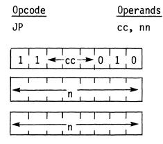
Note: The first n operand in this assembled object code is the low order byte of a 2-byte memory address.
