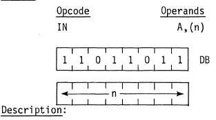
The operand n is placed on the botton half (AO through A7) of the address bus to select the I/O device at one of 256 possible ports. The contents of the Accumulator also appear on the top half (A8 through A15) of the address bus at this time. Then one byte from the selected port is placed on the data bus and written into the Accumulator (register A) in the CPU.
