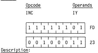
The contents of the Index Register IY are incremented.
