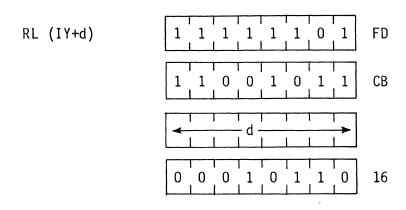
\*r identifies register B,C,D,E,H,L or A specified as follows in the assembled object code above;
