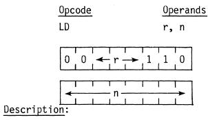
The eight-bit integer n is loaded into any register r, where r identifies register A, B, C, D, E, H or L, assembled as follows in the object code:
