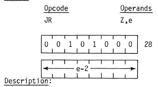
This instruction provides for conditional branching to other segments of a program depending on the results of a test on the Zero Flag. If the flag is equal to a '1', the value of the displacement e is added to the Program Counter (PC) and the next instruction is fetched from the location designated by the new contents of the PC. The jump is measured from the address of the instruction opcode and has a range of -126 to +129 bytes. The assembler automatically adjusts for the twice incremented PC.
