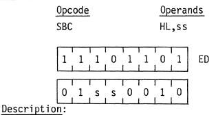
The contents of the register pair ss (any of register pairs BC,DE,HL or SP) and the Carry Flag (C flag in the F register) are subtracted from the contents of register pair HL and the result is stored in HL. Operand ss is specified as follows in the assembled object code.
