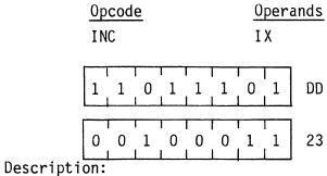
The contents of the Index Register IX are incremented.
