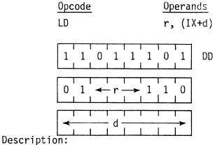
The operand (IX+d) (the contents of the Index Register IX summed with a displacement integer d) is loaded into register r, where r identifies register A, B, C, D, E, H or L, assembled as follows in the object code:
