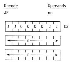
Note: The first operand in this assembled object code is the low order byte of a 2-byte address.
