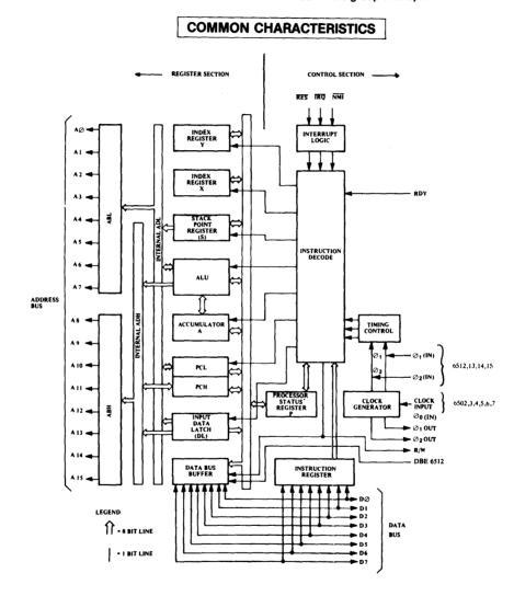
Note: 1. Clock Generator is not included on 6512,13,14,15 2. Addressing Capability and control options vary with each of the 6500 Products.
