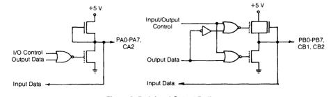
Figure 2. Peripheral Output Buffers
