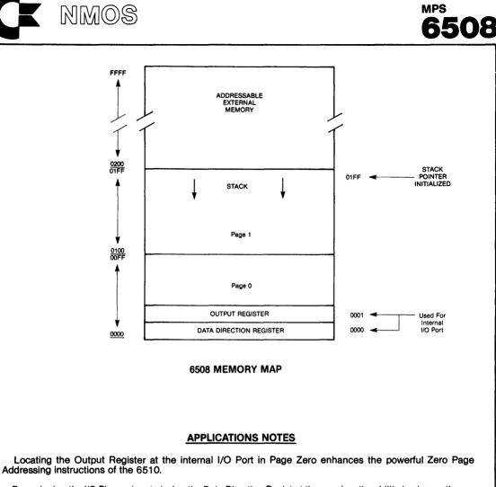
By assigning the I/O Pins as inputs (using the Data Direction Register) the user has the ability to change the contents of address 0001 (the Output Register) using peripheral devices. The ability to change these contents using peripheral inputs, together with Zero Page Indirect Addressing instructions, allows novel and versatile programming techniques not possible earlier.
