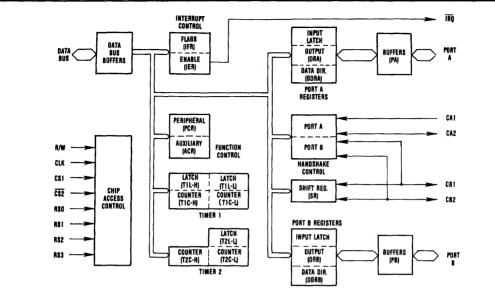
Figure 1. 6522 Block Diagram
