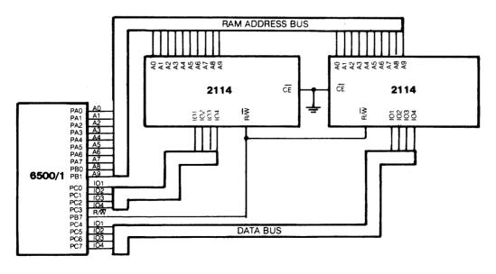
Figure 1 — Schematic for 1K Byte Expansion
