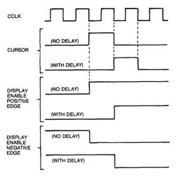
Figure 7. Cursor and Display Enable Skew
