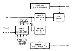
Figure 5. Transmitter/Receiver Clock Circuits
