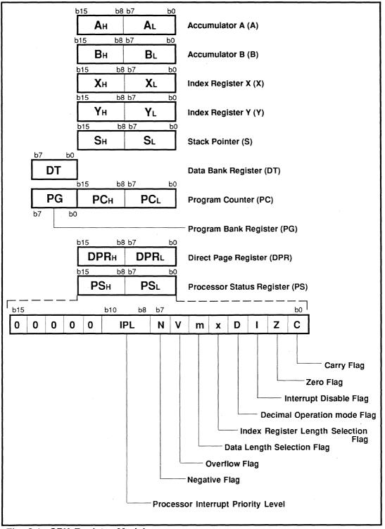
Fig. 2.1 CPU Register Model
