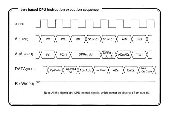
(Example 2-1) When the internal as well as the external memories are used together while wait is commanded by the wait bit.
