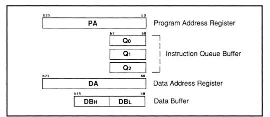
Fig. 6.1.1 Bus Interface Unit Register Model
