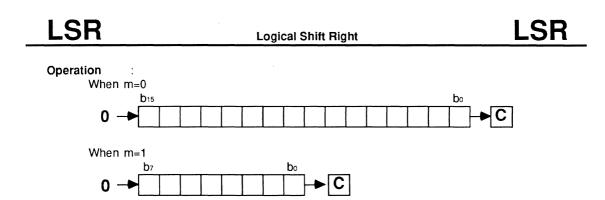
**Description** : Shifts all bits of the accumulator or memory one place to the right. Bit 15 (or bit 7 if the data length selection flag m is set to 1) of the accumulator or memory is loaded with 0.
