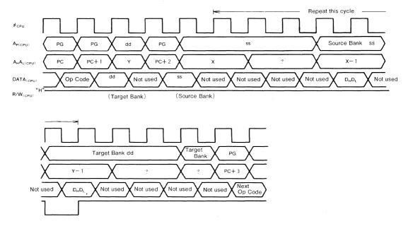
(Note) This figure is shown that transfered the 2-bytes data started from even address. If transfered more than 3-bytes data, the cycle (↔) is repeated each 2-bytes.
