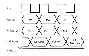
Instruction : ADC, AND, CMP, CPX, CPY, EOR, LDA, LDX, LDY, ORA, SBC
