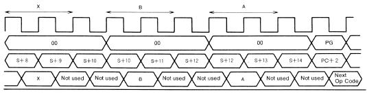
(Note) This figure is an example pulled all the registers by PUL instruction. If some register is not pulled, its cycle (++) is nothing.
