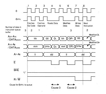
Note. The operation when internal ROM and internal RAM are used, will be as shown above, regardless of the level of the BYTE terminal. However, the address/data bus, BHE, R/W signal cannot be observed from outside, when the mode is single chip mode.
