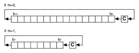
**Description** : The carry flag C is linked to the accumulator or memory, and the combined contents are rotated by 1 bit to the left.
