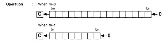
**Description** : Shifts all bits of the accumulator or memory one place to the left. Bit 0 is loaded with 0. The carry flag C is loaded from bit 15 (or bit 7 when the data length selection flag m is set to 1) of the data before the shift.
