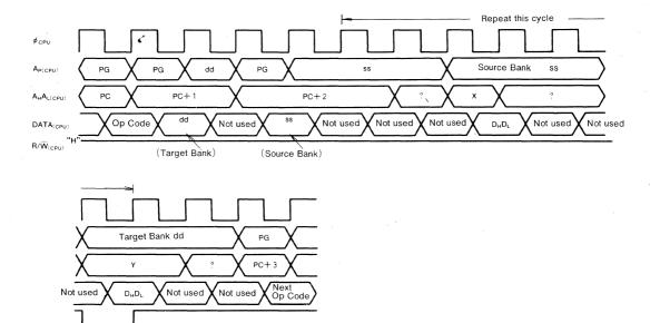
(Note) This figure is shown that transfered the 2-bytes data started from even address. If transfered more than 3-bytes data, the cycle (↔) is repeated each 2-bytes.
