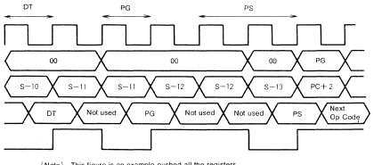
(Note) This figure is an example pushed all the registers by PSH instruction. If any register is not pushed, its cycle (++) is nothing,
