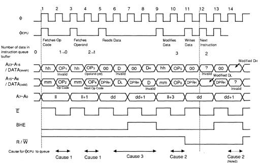
Note1. The operation when internal ROM and internal RAM are used, will be as shown above, regardless of the level of the BYTE terminal. However, the address/data bus, BHE, R/W signal cannot be observed from outside, when the mode is single chip mode.
