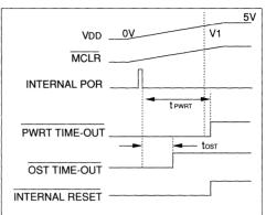
Note: In this example t<sub>PWRT</sub> > t<sub>OST</sub> as would be the case in higher frequency crystals. For lower frequency crystals (i.e. 32 Khz) t<sub>OST</sub> will be greater.
