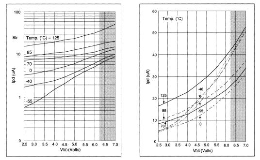
FIGURE 18.0.7 - MAXIMUM Ipd vs VDD WATCHDOG DISABLED FIGURE 18.0.8 - MAXIMUM Ipd vs VDD WATCHDOG ENABLED\*
