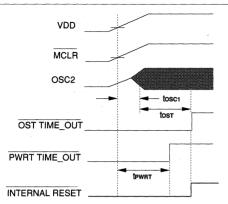
This figure shows in greater detail the timings involved with the oscillator start-up timer. In this example the low frequency crystal start-up time is larger than power-up time (**b**war).
