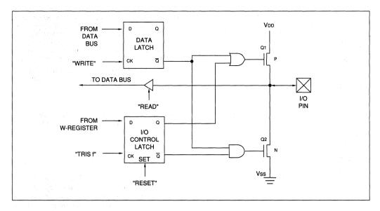
b) A pin actively outputting a "0" or "1" should not be driven from external devices at the same time in order to change the level on this pin ("wired-or", "wired-and"). The resulting high output currents may damage the chip.
