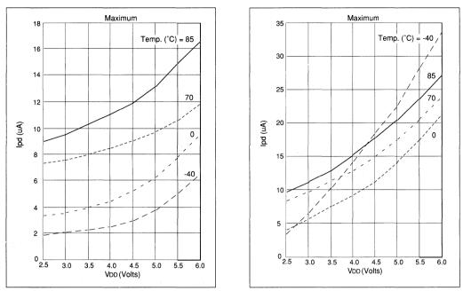
\* IPD, with watchdog timer enabled, has two components: The leakage current which increases with higher temperature and the operating current of the watchdog timer logic which increases with lower temperature. At -40°C, the latter dominates explaining the apparently anomalous behavior.
