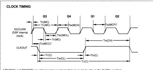
\* TD(MCC) and TW(MCP) are referenced to an intermediate level of 1.5 volts on the CLKIN waveform. Note: Timing measurements are referenced to and from a low voltage of 0.8 volts and a high voltage of 2.0 volts, unless otherwise noted. 6
