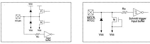
Notes to figures 7.6.1 and 7.6.2: The diodes and the grounded gate (or output driver) NMOS device are carefully designed to protect against ESD (Electrostatic discharge) and EOS (Electrical overstress). Rin is a small resistance to further protect the input buffer from ESD.
