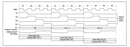
Program Counter (PC) which automatically increments to execute in-line programs. Program control operations, supporting direct, indirect, relative addressing modes, can be performed by Bit Test and Skip instructions, Call instructions, Jump instructions or by loading computed addresses into the PC. In addition, an on-chip two-level stack is employed to provide easy to use subroutine nesting.
