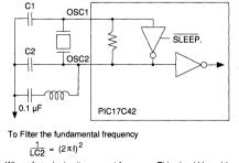
Where f= tank circuit resonant frequency. This should be midway between the fundamental and the 3rd overtone frequencies of the crystal.
