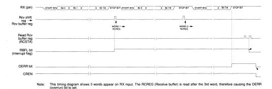
bit will be set again. To enable receive interrupt, the Peripheral Interrupt Enable bit, PEIE (bit3, INTSTA register, file 07h). must be set and the Global Interrupt Disable bit, GLINTD (bit4, CPUSTA register, file 06h), must be cleared.
