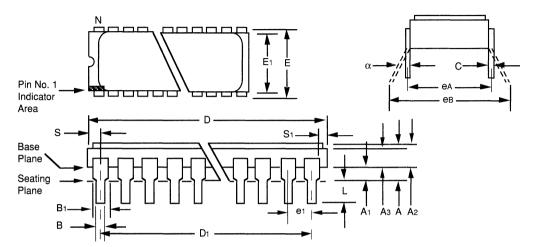
Package Type: 48-Lead Ceramic Side Brazed Dual In-line (.600 mil)
