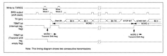
If 9 bit transmission is selected (TX8/9=1, bit 6, register TXSTA) the 9th bit should be written to TXD8 (bit0, TXSTA). This bit is double buffered as well. The 9th bit must be written before writing the data word to TXREG, since the latter triggers the transfer of the entire word to the transmit shift register.
