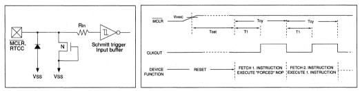
Notes to figures 16.9.1 and 16.9.2: The diodes and the grounded gate (or output driver) NMOS device are carefully designed to protect against ESD (Electrostatic discharge) and EOS (Electrical overstress). Rin is a small resistance to further protect the input buffer from ESD.
