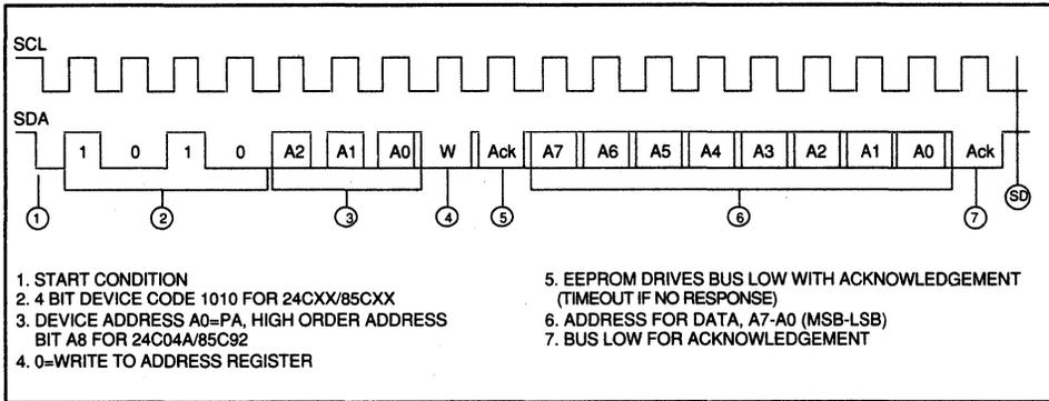
Fig. 3A Setting The Internal Word Address Of The 24Cxx/85Cxx
