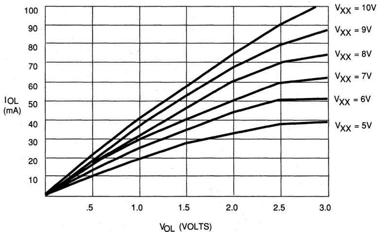
The Output Sink Current is dependent on the V<sub>XX</sub> supply and the output load. This chart shows the typical curves used to express the output drive capability.
