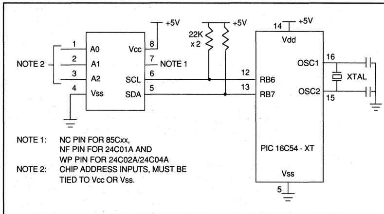
Fig. 2 A Simple Hardware Connection
