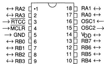
The PIC1654S is fabricated with N-Channel Silicon Gate technology resulting in a high performance product with proven reliability and production history. Only a single wide range power supply is required for operation, and an on-chip oscillator provides the operating clock with an external crystal or ceramic resonator to establish the frequency. Inputs and outputs are TTL-compatible.
