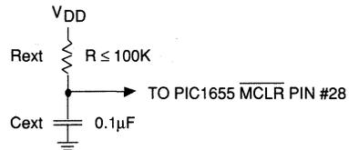
Master Clear requires >1.0ms delay before activation after power is applied to the V<sub>DD</sub> pin, for the oscillator to start up. To achieve this, an external RC configuration as shown can be used (assuming V<sub>DD</sub> is applied as a step function).
