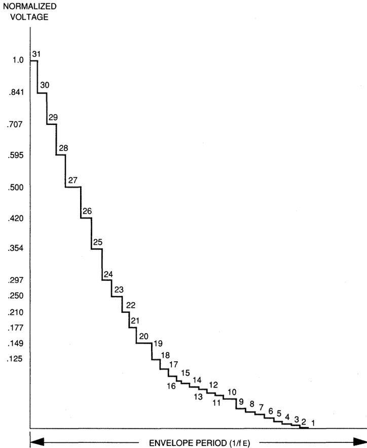
THIS FIGURE ILLUSTRATES THE D/A CONVERTER OUTPUT WHICH WOULD RESULT IF NOISE AND TONES WERE DISABLED AND AN ENVELOPE CONTROLLED VARIABLE AMPLITUDE WERE SELECTED.
