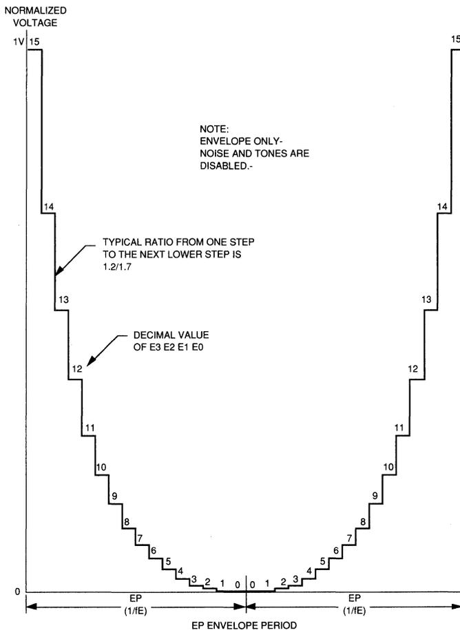
FIG. 4 SINGLE TONE WITH ENVELOPE SHAPE/CYCLE PATTERN 1010
