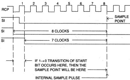
**FIG. 8 RECEIVER DURING 1ST STOP BIT**
