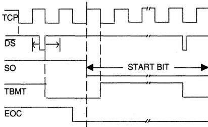
**FIG. 3 TRANSMITTER AT START BIT**
