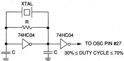
The buffer must be capable of driving 120Ω, min. (800Ω, typ.) to 2.0V. However, it is recommended that the pull-down transistor on the OSC pin be removed (an option) if OSC is to be driven externally.
