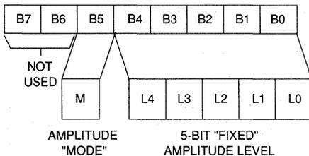
The amplitude "mode" (bit M) selects either fixed level amplitude (M = 0) or variable level amplitude (M = 1). It follows that bits L4 - L0, defining the value of a "fixed" level amplitude, are only active when M = 0. The amplitude is only "fixed" in the sense that the amplitude level is under the direct control of the system processor via an address latch/write data sequence.
