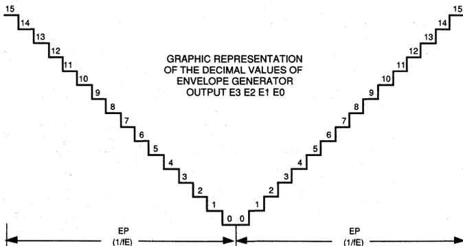
FIG. 3 D/A CONVERTER OUTPUT
