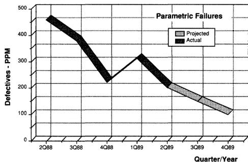
as speed, power and device leakage. Its present level has reached 200 ppm after programming, with a goal of 100 ppm.
