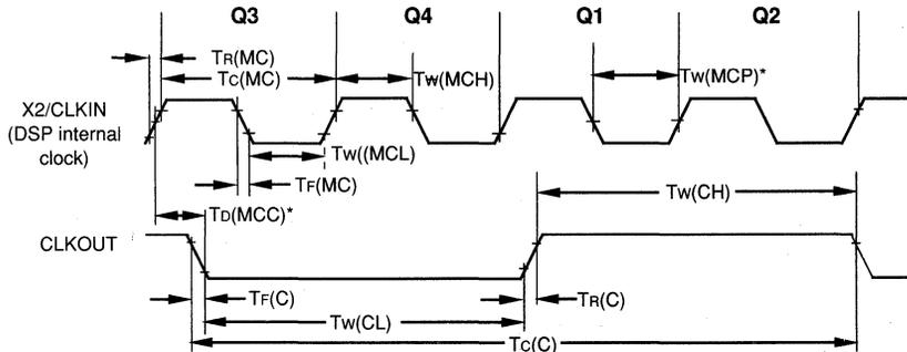
\* T<sub>d</sub>(MCC) and T<sub>w</sub>(MCP) are referenced to an intermediate level of 1.5 volts on the CLKIN waveform.
