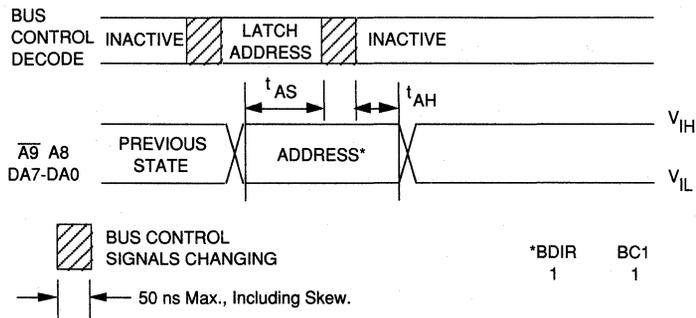
FIG. 10 WRITE DATA TIMING
