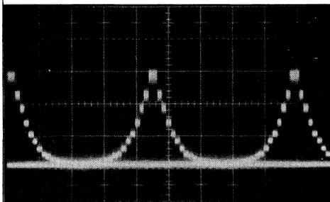
FIG. 5 MIXTURE OF THREE TONES WITH FIXED AMPLITUDES
