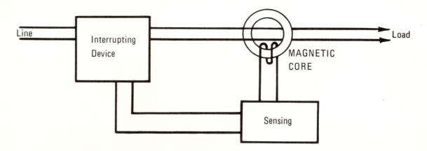
The heart of a ground fault detector is a high initial permeability magnetic core with a sensitivity capable of detecting minute differences in currents entering and leaving a load. The following are typical core requirements for meeting GFI specifications:
