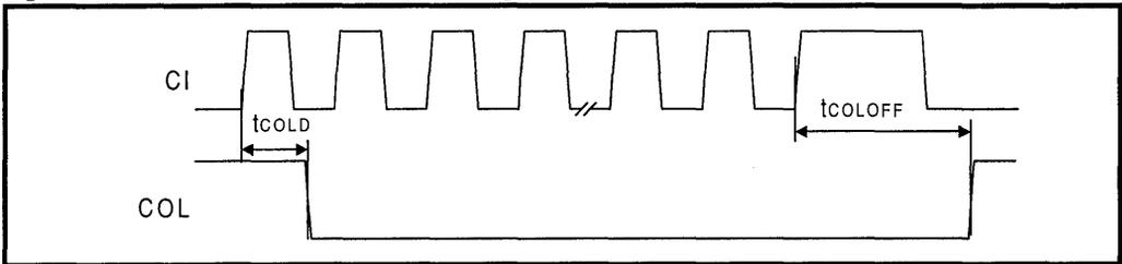
Figure 31: Mode 3 COL/SQE Output Timing
