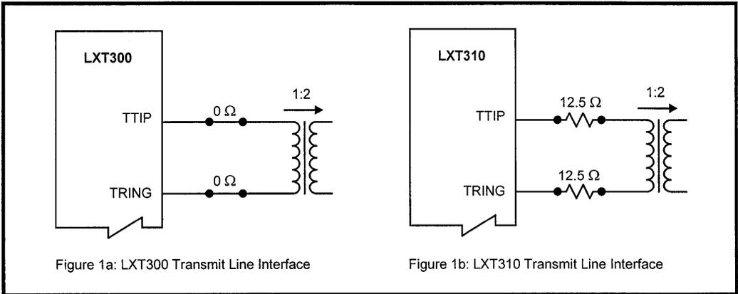
Figure 1a: LXT300 Transmit Line Interface
