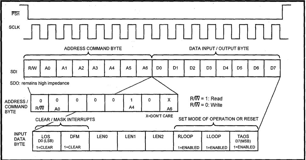
**Figure 5: LXT332 SIO Read Operation**
