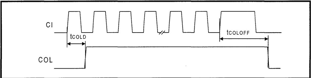
Figure 43: Mode 5 COL/SQE Output Timing
