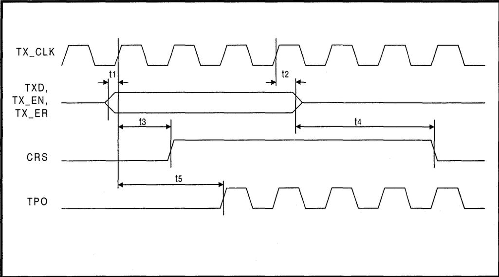
Table 36: MII - 10BASE-T Transmit Timing Parameters (Over Recommended Range)
