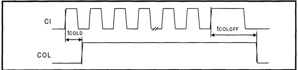
Figure 20: Mode 1 COL/CI Output Timing
