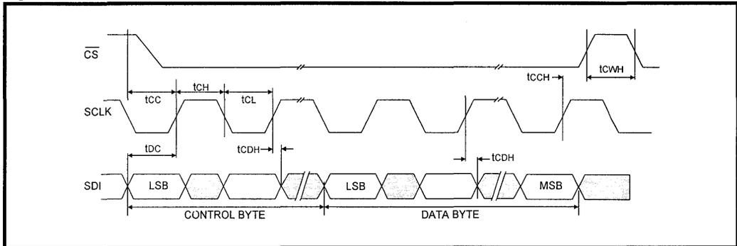
Figure 11: LXT305A Serial Data Output Timing Diagram
