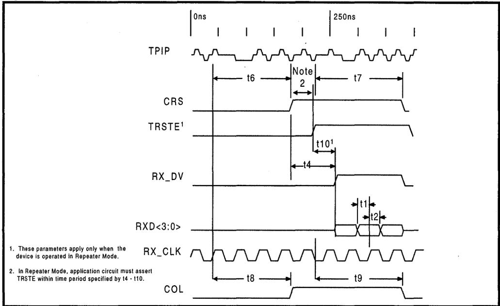
**Table 29: MII - 100BASE-TX Receive Timing Parameters / 4B Mode (Over Recommended Range)**
