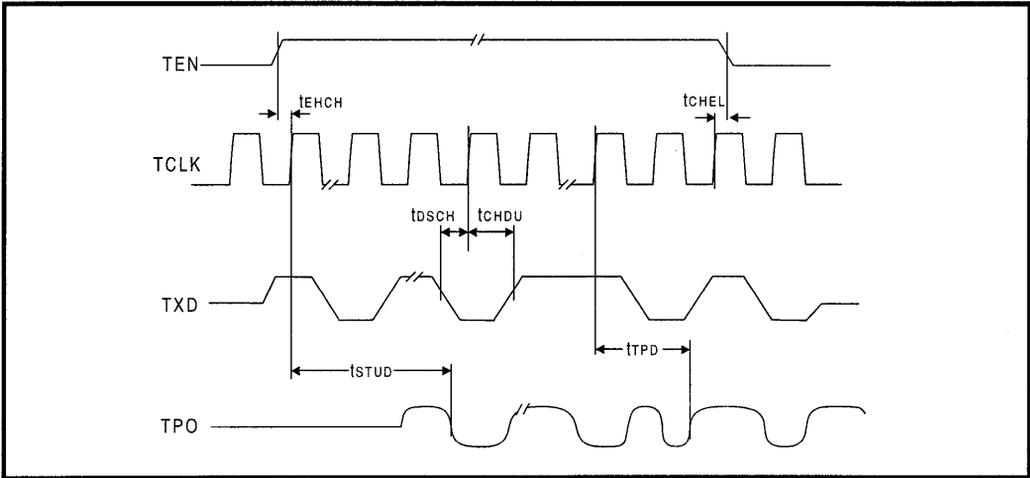
Figure 39: Mode 4 Collision Detect Timing
