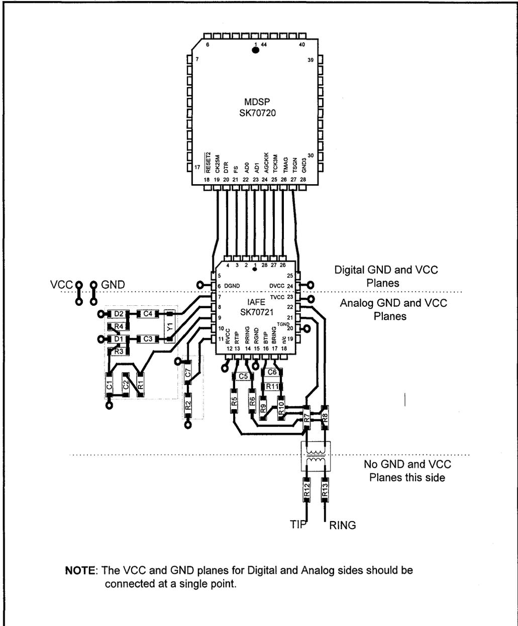
Figure 13: Typical Application for Master Mode Operation (Microprocessor Interface Mode)
