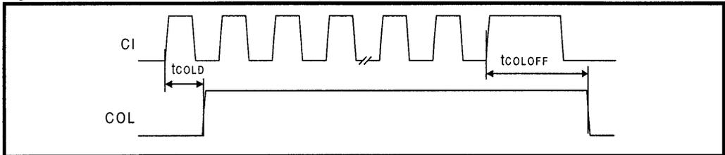
Figure 25: Mode 4 COL/CI Output Timing
