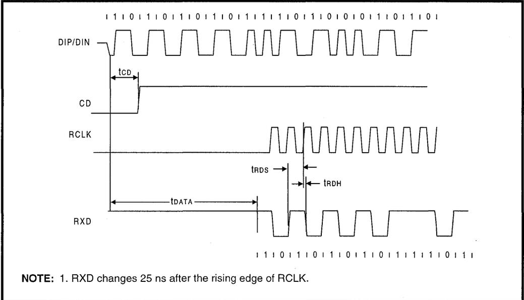
**Figure 4: Mode 1 RCLK/End-of-Frame Timing**
