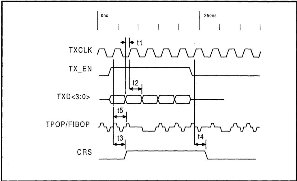
Table 34: MII - 100BASE-FX Transmit Timing Parameters / 4B Mode (Over Recommended Range)
