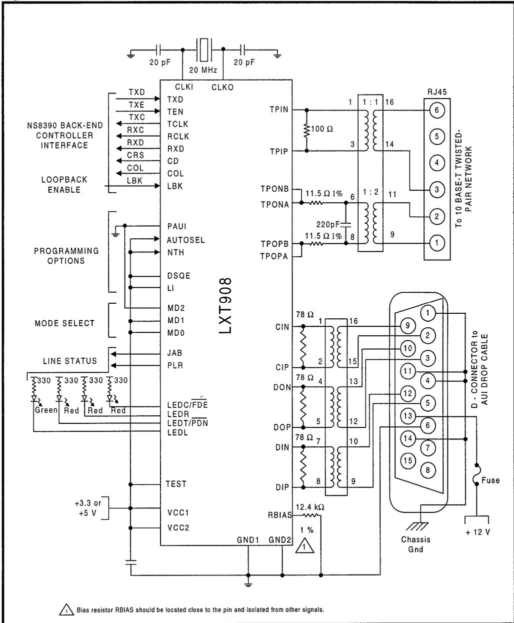
△ Bias resistor RBIAS should be located close to the pin and isolated from other signals.
