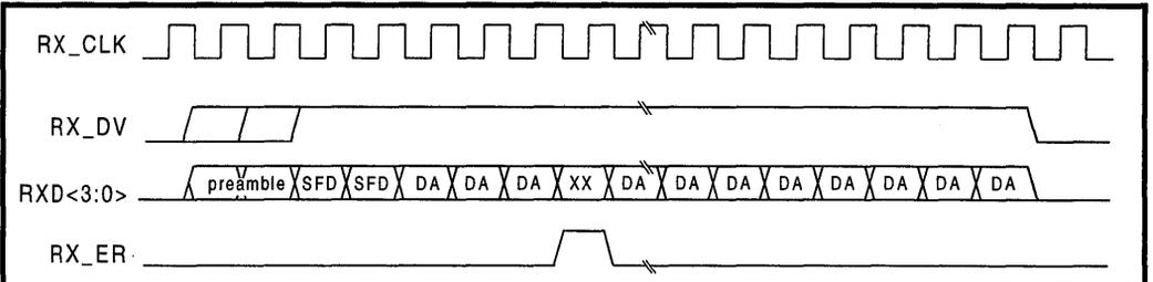
**Figure 12: 100BASE-TX Transmission with No Errors**
