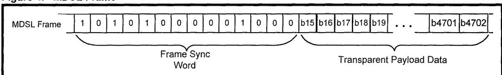
The MDP receiver detects the incoming FSW and provides a blanking signal (RDATA\_ST) at its output to indicate that payload data is not present during the FSW. The RDATA\_ST signal can also be used to gate the receiver clock signal (BIT\_CK) so that clock transitions are present only when payload data is available. The resulting gapped clock is similar to that found in many other data transport systems.
