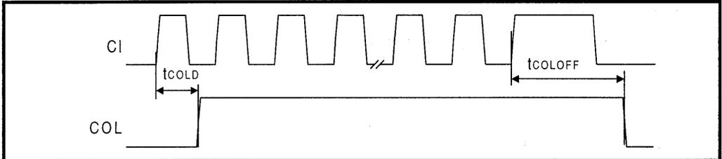
Figure 37: Mode 4 COL/SQE Output Timing
