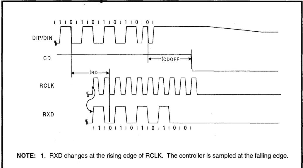
Figure 11: Mode 2 Transmit Timing
