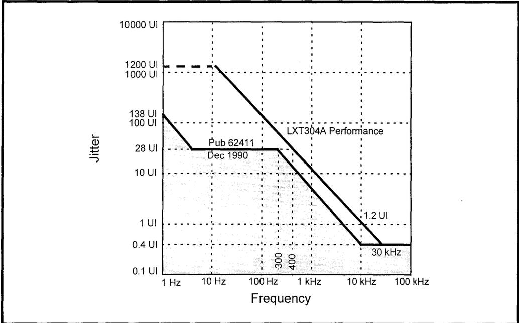
Figure 7: LXT304A Receive Jitter Transfer Performance (Typical)
