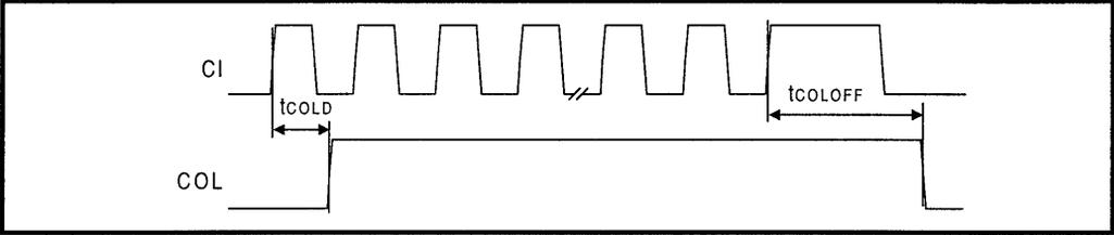
Figure 7: Mode 1 COL/CI Output Timing
