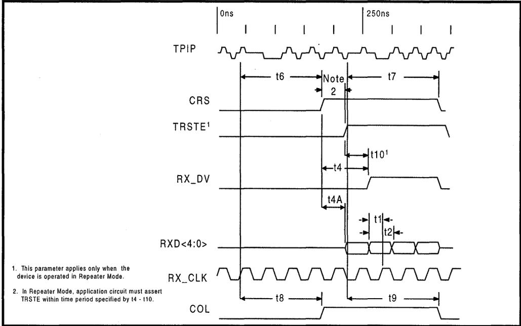
**Table 31: MII - 100BASE-TX Receive Timing Parameters / 5B Mode (Over Recommended Range)**
