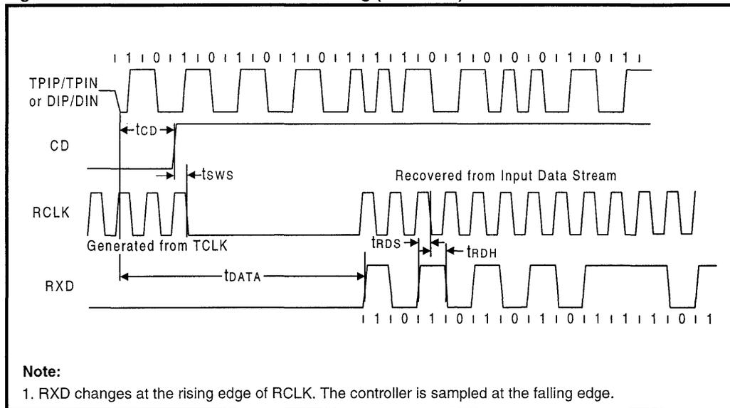
Figure 31: Mode 3 RCLK/End-of-Frame Timing (LXT907A)
