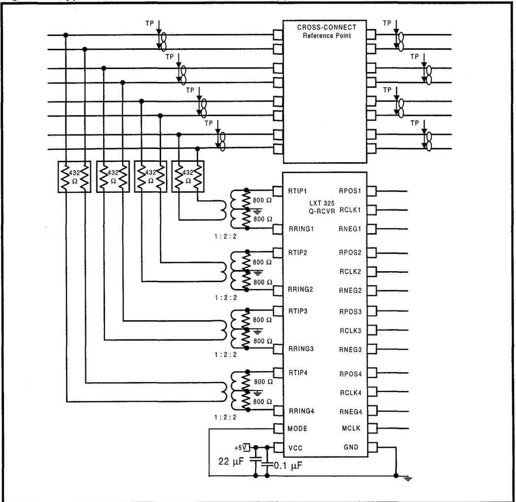
Figure 3: Typical DSX-1/E1 Receiver Application
