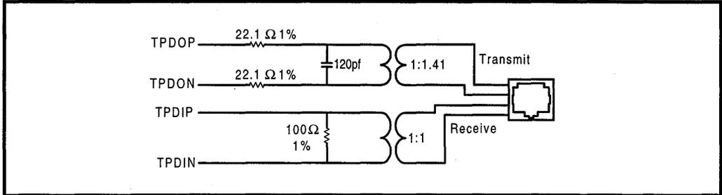
**Figure 12: Normal AUI Circuit**
