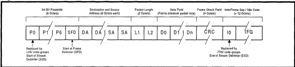
Figure 9: 100BASE-TX Data Flow
