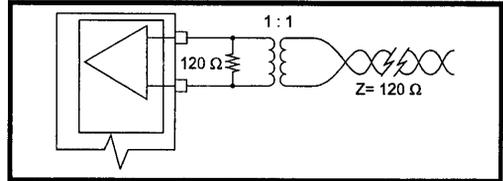
Figure 9: T1 Low Power Tx I/F for Twisted-Pair Lines
