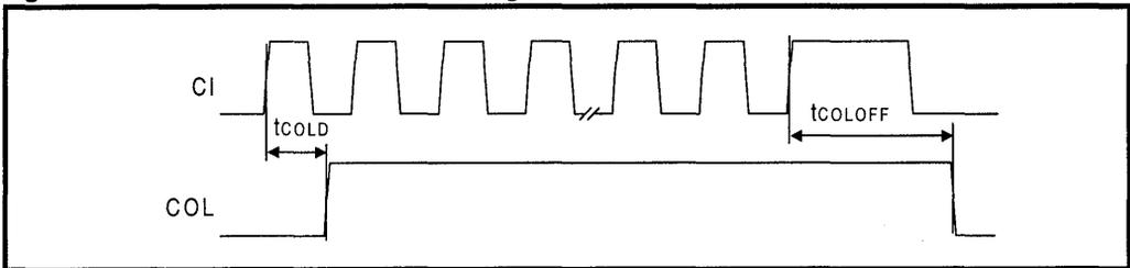
Figure 19: Mode 1 COL/SQE Output Timing/CI Output Timing
