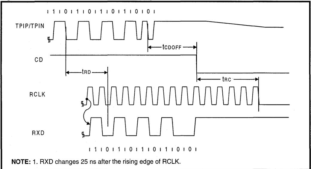
Figure 12: Mode 1 Transmit Timing
