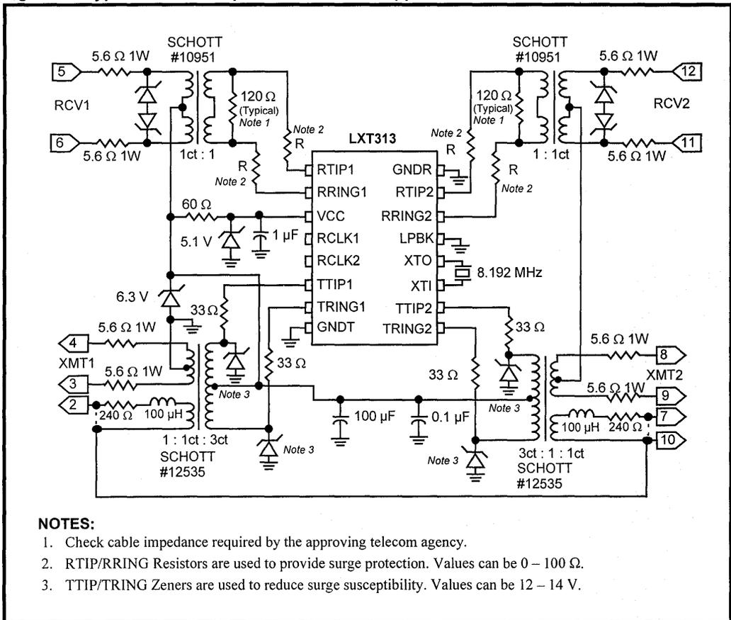
Figure 3: Alternate Timing Reference Circuitry
