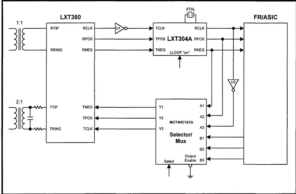
Figure 3: LXT304A Configuration as Standalone Jitter Attenuator
