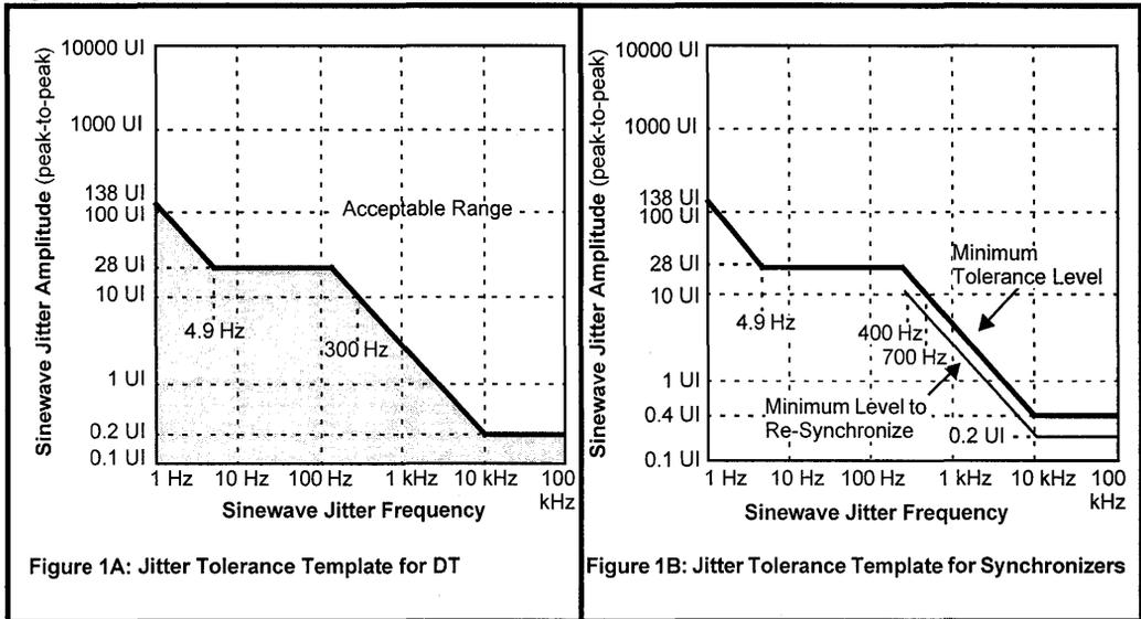
**Jitter Tolerance Test Procedures**
