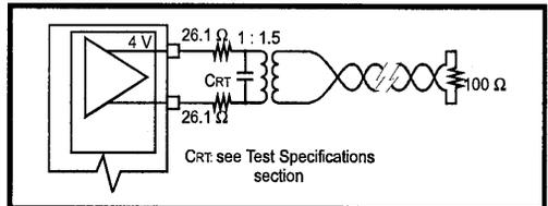
Figure 11: T1 Rx I/F for Twisted-Pair Lines
