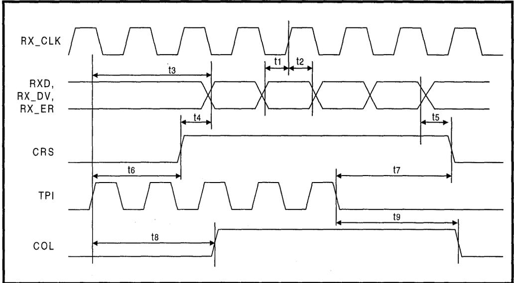
**Table 35: MII - 10BASE-T Receive Timing Parameters (Over Recommended Range)**
