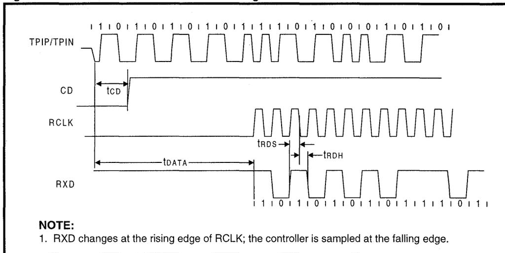
**Figure 15: Mode 2 RCLK/End-of-Frame Timing**
