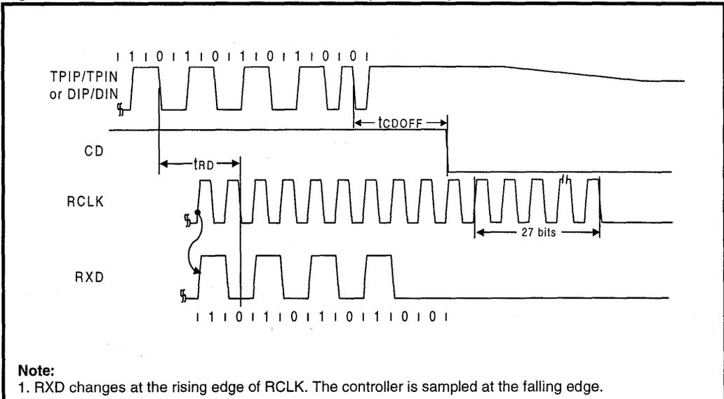
Figure 30: Mode 3 RCLK/Start-of-Frame Timing (LXT907A)
