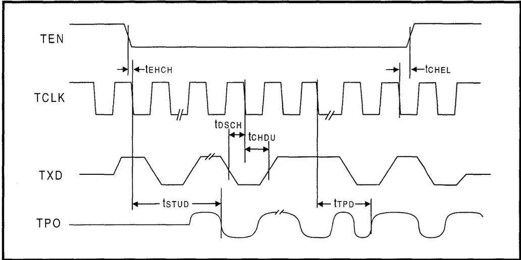
Figure 17: Mode 2 COL Output Timing
