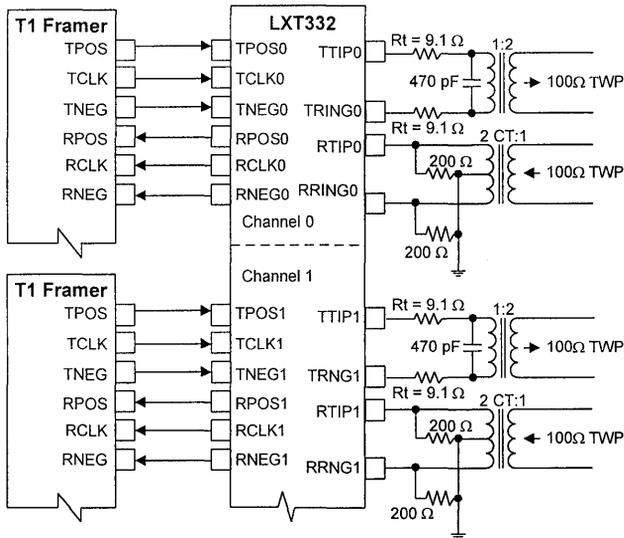
Figure 1B: LXT332 100 Ω T1 Line Interface
