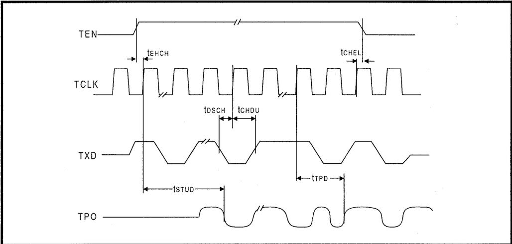
Figure 36: Mode 4 Collision Detect Timing
