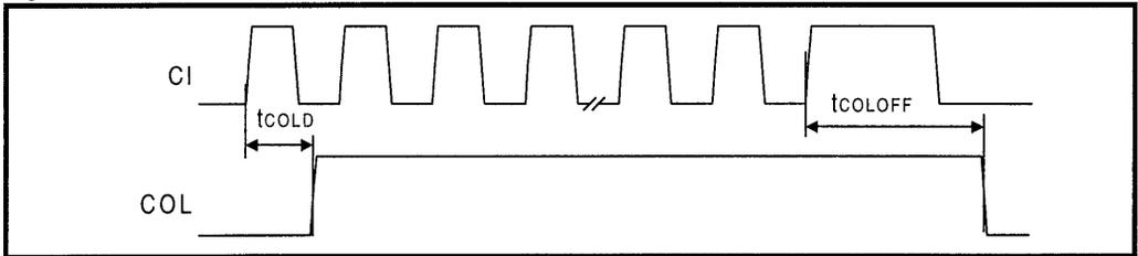
Figure 40: Mode 4 COL/CI Output Timing
