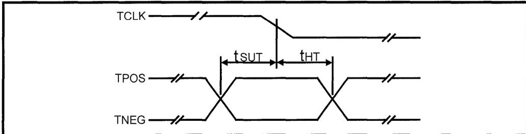
Figure 15: LXT318 Receive Clock Timing
