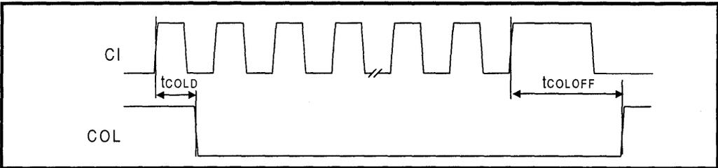
Figure 26: Mode 2 COL/CI Output Timing
