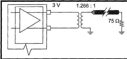
**Figure 3: Transmit Interface for Coax Cables**
