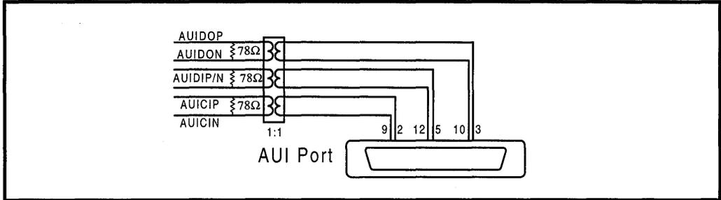
**Figure 13: Reversed AUI Circuit**
