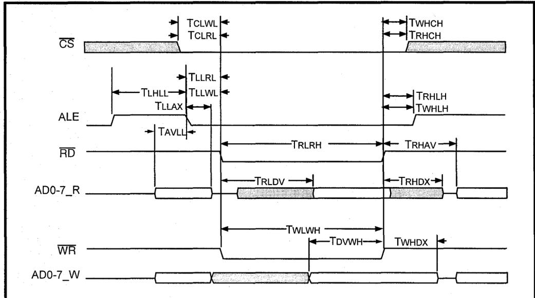
**Table 46: LXT361 16.78 MHz Motorola Bus Parallel I/O Timing Characteristics**
