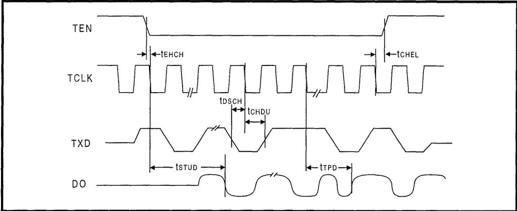
Figure 12: Mode 2 Collision Detect Timing
