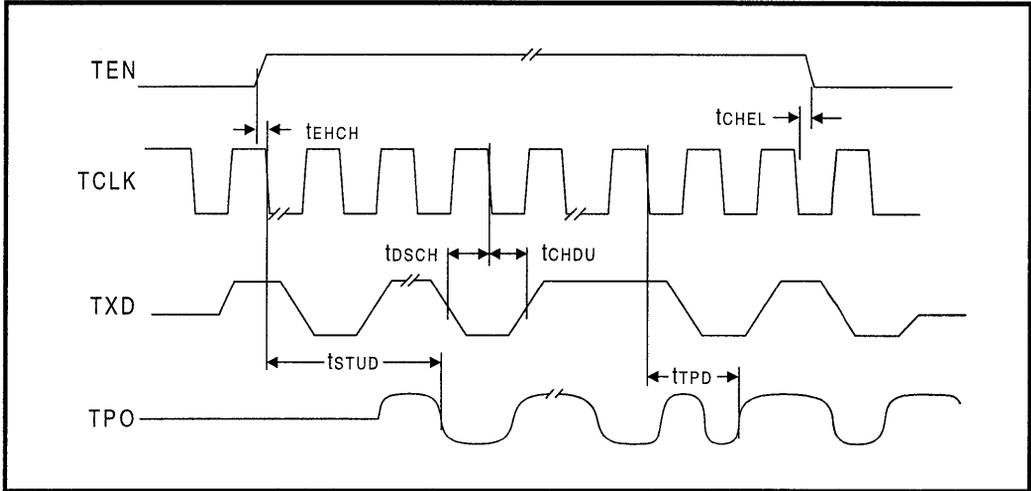
Figure 21: Mode 3 COL Output Timing
