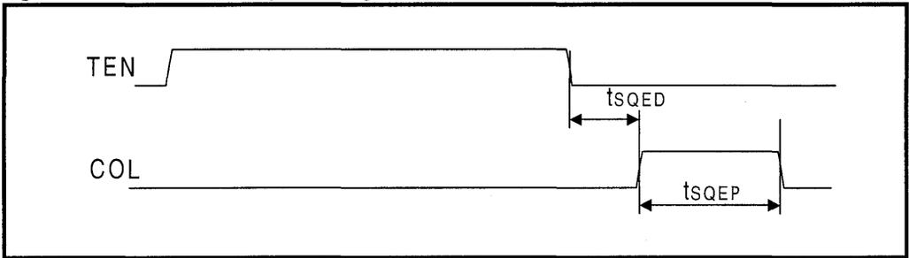
**Timing Diagrams for Mode 2** (MD1=Low, MD0=High) Figures 14 through 17
