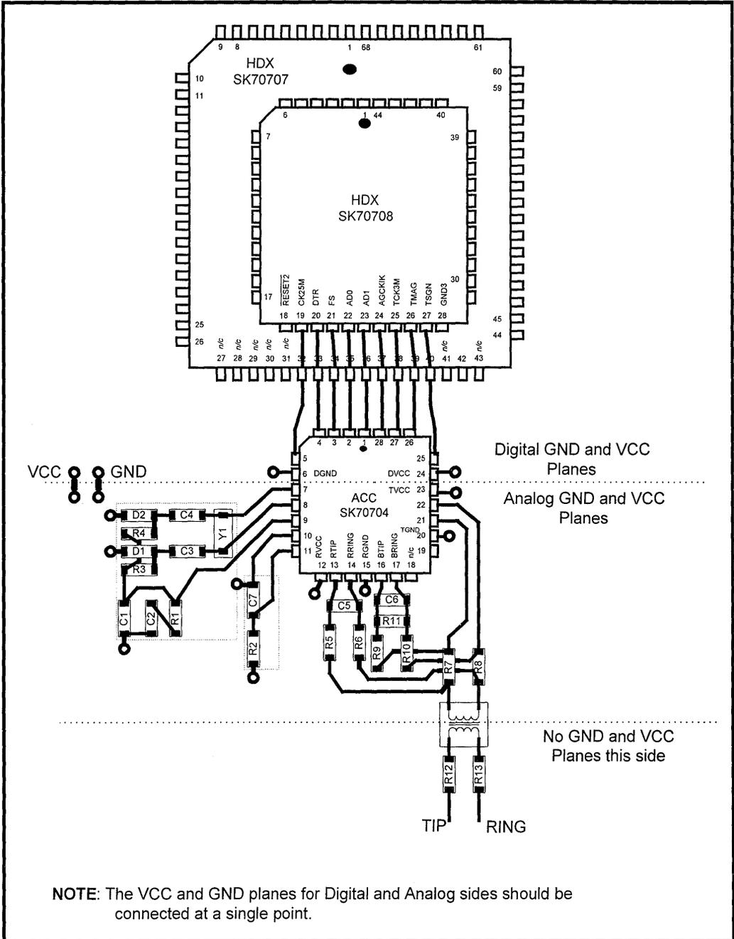
Figure 11: Typical Support Circuitry for LTU Applications
