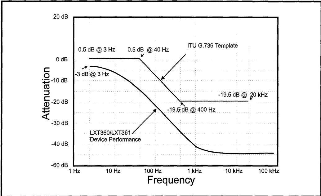
Figure 26: T1 Jitter Attenuation (Typical)
