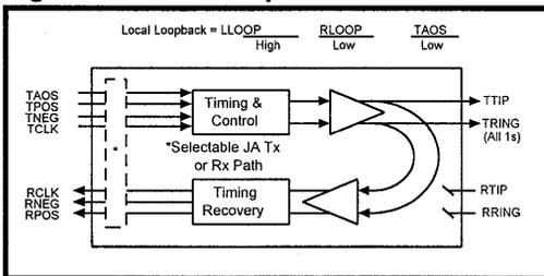
**Local Loopback.** See Figure 8. Local Loopback (LLOOP) is designed to exercise the maximum number of functional blocks. During LLOOP operation, the RTIP/RRING inputs from the line are disconnected. Instead, the transmit out-
