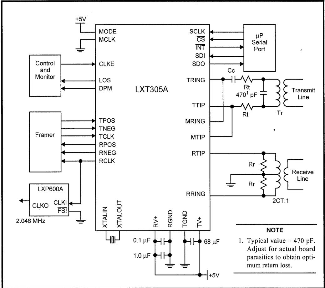
Figure 5: Typical LXT305A 120 Ω 2.048 Mbps E1 Application (Hardware Mode)
