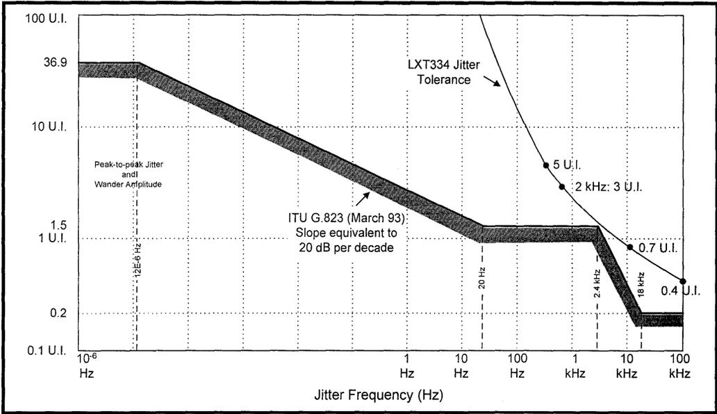
Figure 18: Jitter Attenuation—G.735
