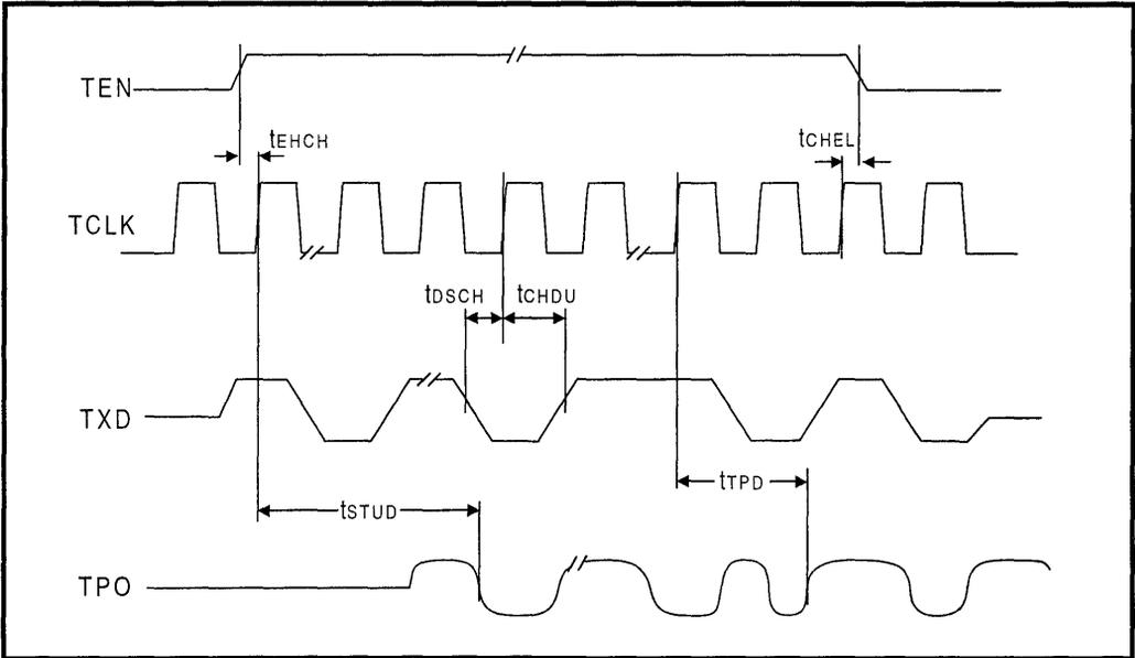
Figure 25: Mode 4 COL Output Timing
