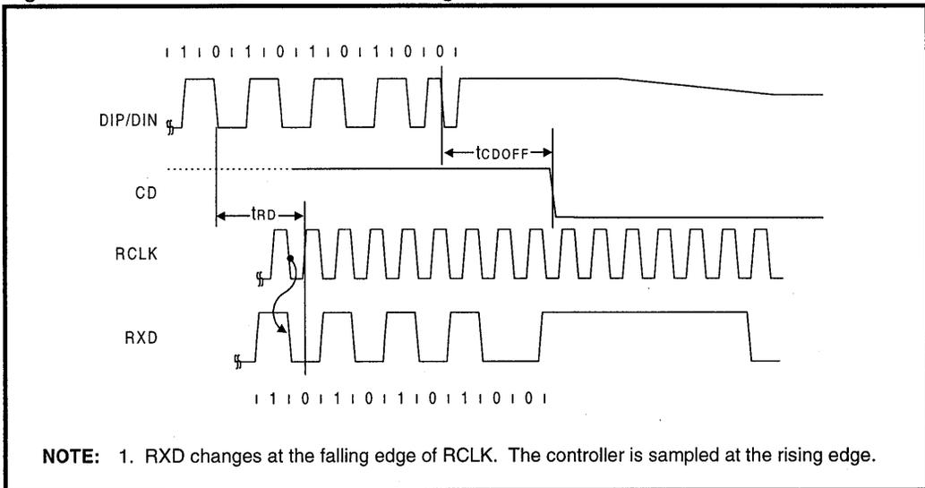
Figure 23: Mode 4 Transmit Timing
