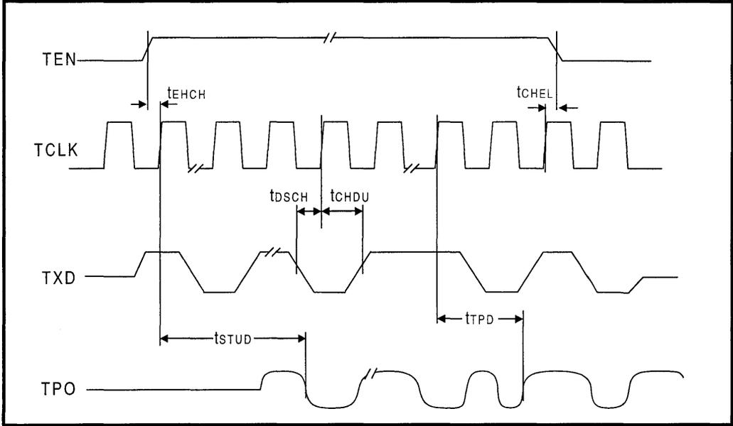
Figure 25: Mode 4 COL Output Timing
