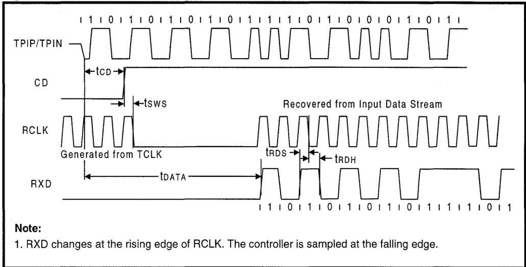
**Figure 19: Mode 3 RCLK/End-of-Frame Timing**
