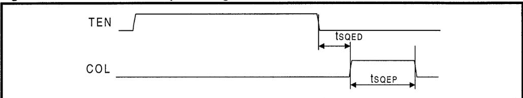
Figure 41: Mode 4 Loopback Timing
