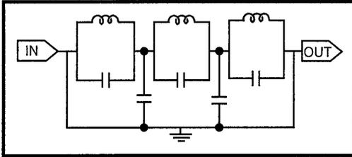
Figure 9: Typical Receive Filter
