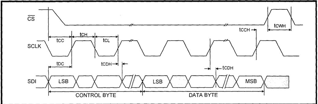
**Figure 15: LXT300Z Serial Data Output Timing Diagram**
