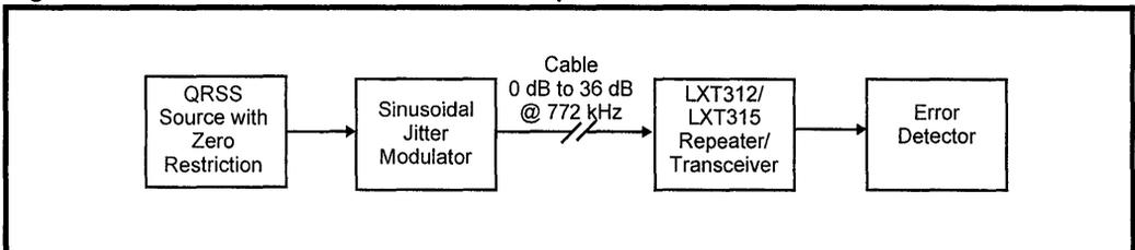
Figure 7: Receiver Jitter Transfer Test Setup
