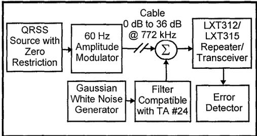
Figure 11: Receiver Timing Recovery Phase Shift Modulation Test Setup
