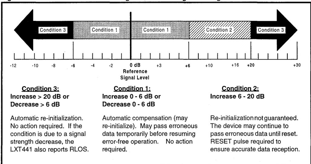
Figure 4: RLOS Timing for a True Loss of Signal
