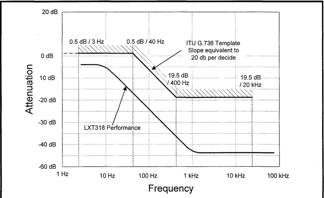
Figure 20: Input and Maximum Output Jitter Specified by TBR12/13
