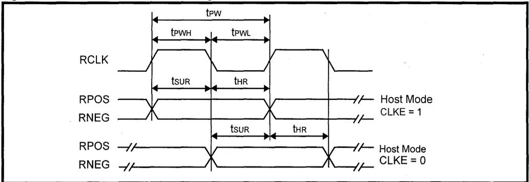
Figure 19: LXT332 Transmit Clock Timing
