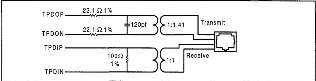
**Figure 11: Normal AUI Circuit**
