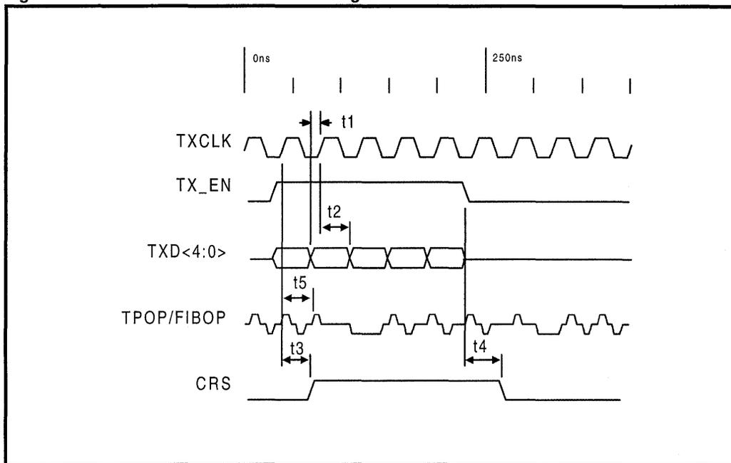
Table 32: MII - 100BASE-TX Transmit Timing Parameters / 5B Mode (Over Recommended Range)
