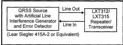
Figure 9: Receiver Gaussian Noise Immunity Test Setup
