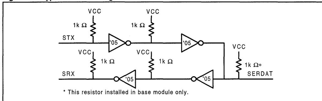
Figure 15: Typical Chip ID Architecture
