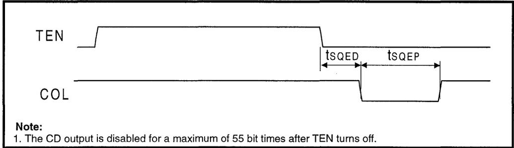
Figure 35: Mode 3 Loopback Timing
