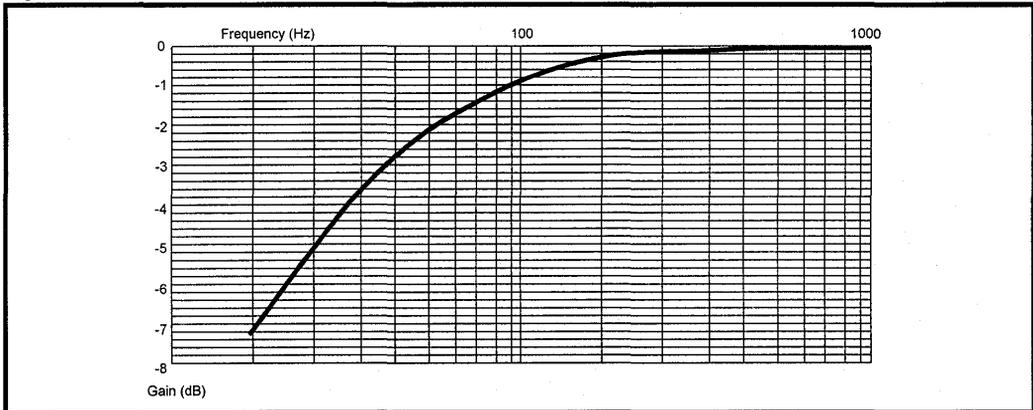
Figure 5: Typical LXT304A Jitter Attenuation Performance
