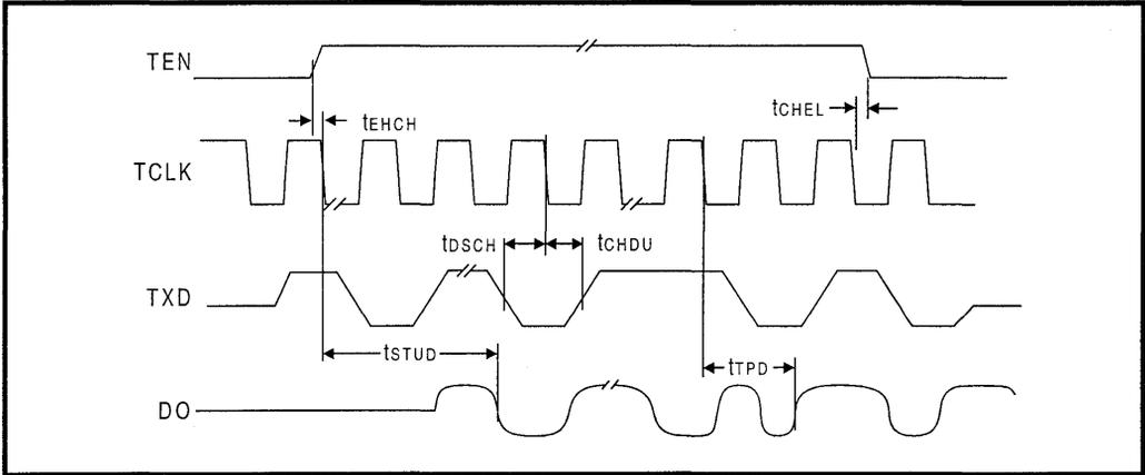
Figure 18: Mode 3 Collision Detect Timing
