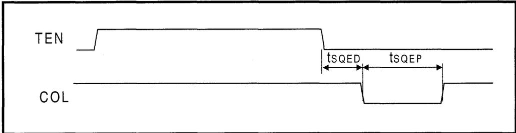
**Timing Diagrams for Mode 4** (MD1 = High, MD0 = High) *Figures 22 through 25*
