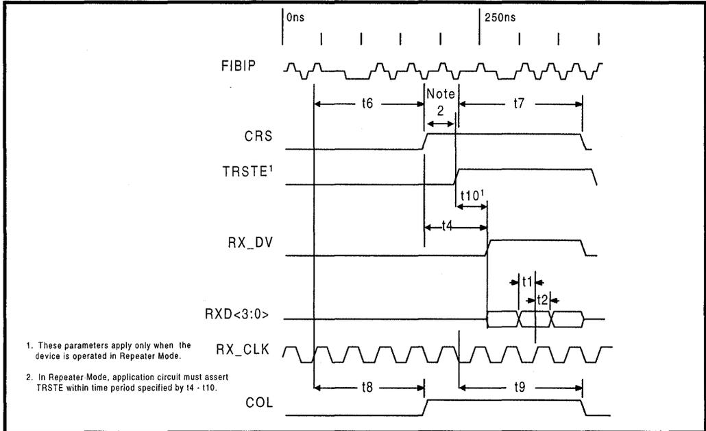
**Table 33: MII - 100BASE-FX Receive Timing Parameters / 4B Mode (Over Recommended Range)**
