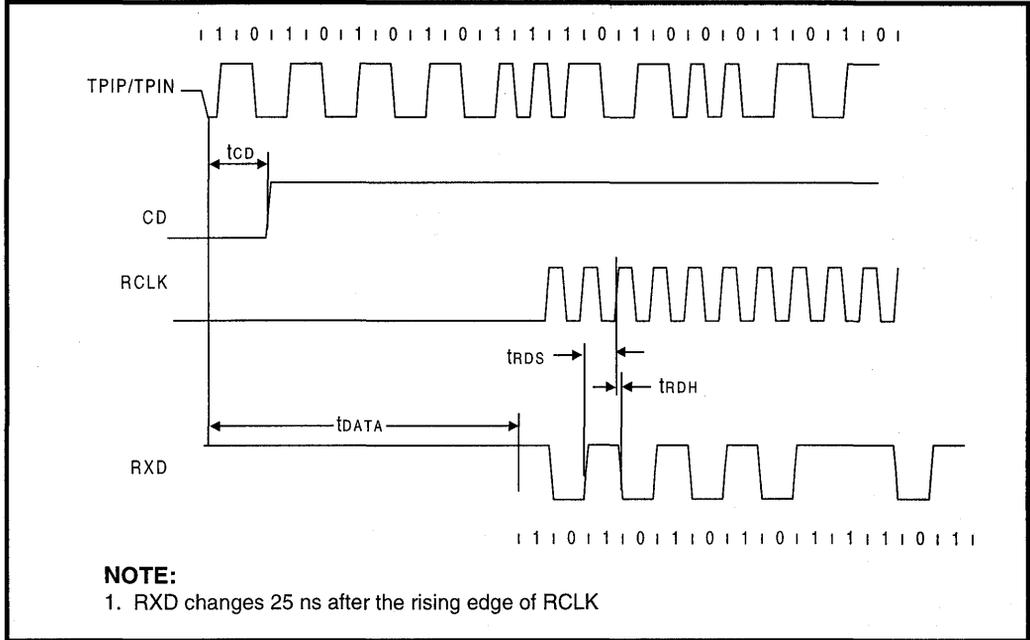
**Figure 11: Mode 1 RCLK/End-of-Frame Timing**
