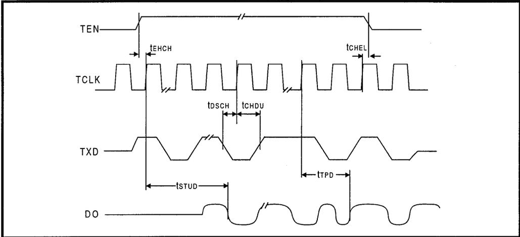
Figure 24: Mode 4 Collision Detect Timing
