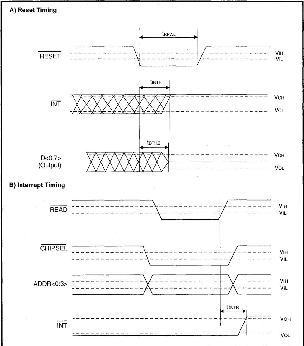
Figure 23: Parallel Data Channel Timing
