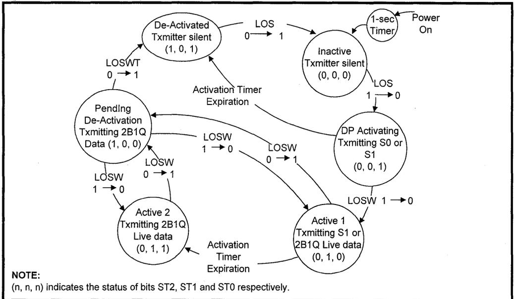
**Figure 9: HTU-R HDSL Framer Activation State Machine**
