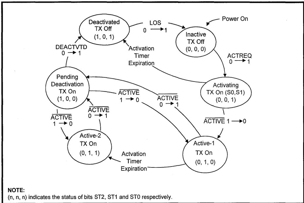
In Pending Deactivation, the Master Data Pump progresses to the Deactivated and Inactive States with the expiration of the respective timers. If the sync word is detected before the Pending Deactivation timer expires, the Master Data Pump returns to either Active-1 or Active-2. (The Master Data Pump returns to which ever state it occupied before transitioning to Pending Deactivation.)
