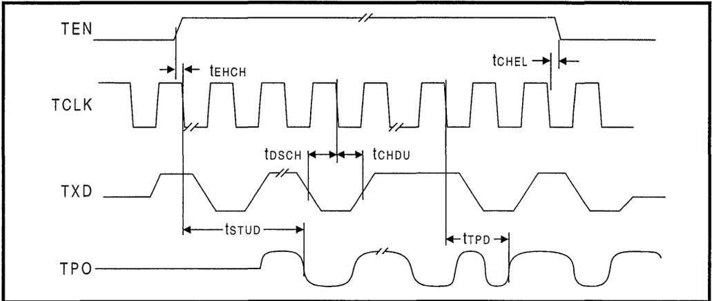
Figure 33: Mode 3 Collision Detect Timing
