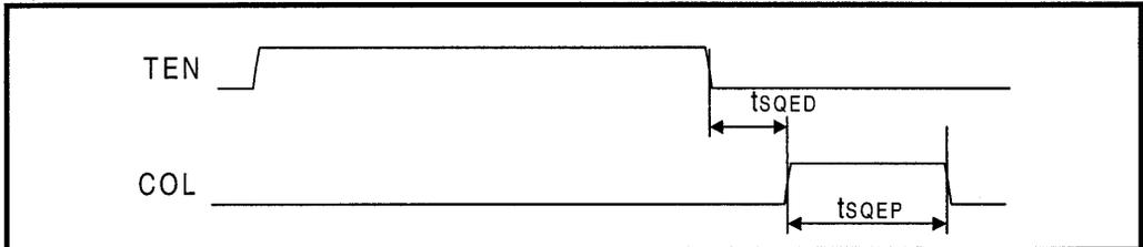
Figure 26: Mode 4 Loopback Timing
