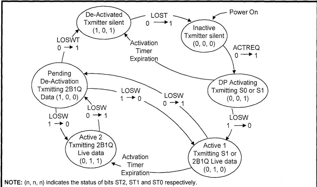
Figure 6: LTM HDSL Framer Activation State Machine
