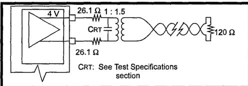
**Figure 6: Receive Interface for Twisted Pair Lines**
