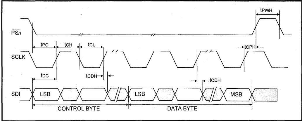
**Figure 16: LXT331 Serial Output Timing Diagram**
