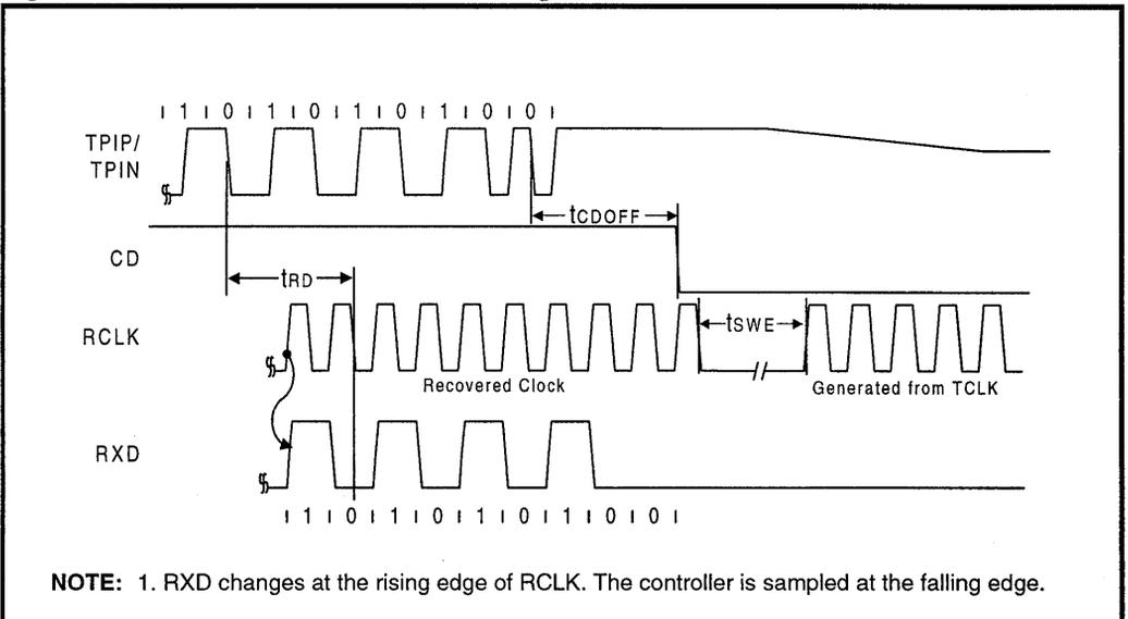
Figure 29: Mode 3 Transmit Timing
