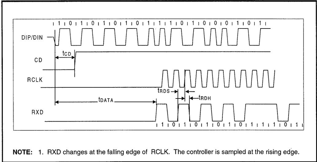
**Figure 22: Mode 4 RCLK/End of Frame Timing**
