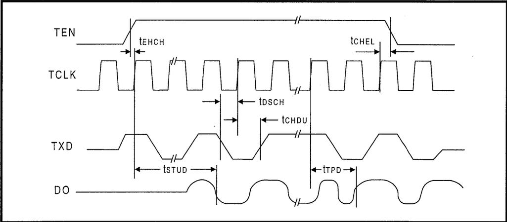
Figure 6: Mode 1 Collision Detect Timing
