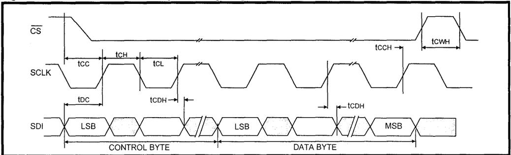
**Figure 11: LXT304A Serial Data Output Timing Diagram**
