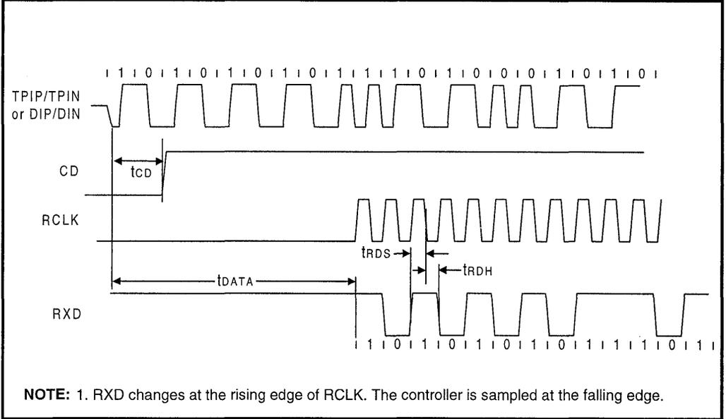
**Figure 22: Mode 2 RCLK/End-of-Frame Timing**
