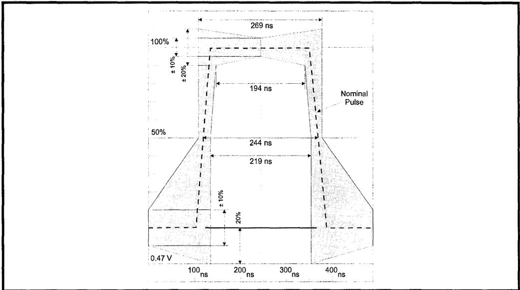
Figure 16: 1.544 MHz Pulse Mask I.431
