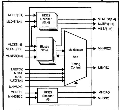
Data enters a first-in/first-out (FIFO) elastic store block. The FIFO receives the data along with the tributary clock and a pointer generated from the timing control. The output of the elastic store block is clocked by the tributary enable
