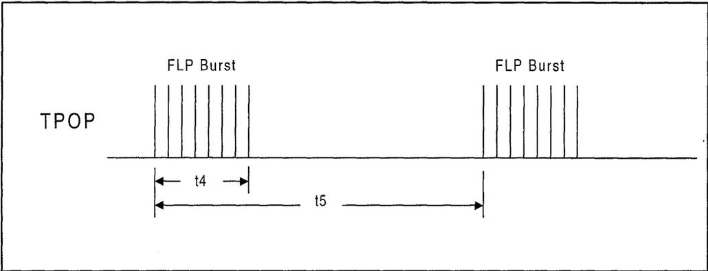
Table 39: Auto Negotiation and Fast Link Pulse Timing Parameters (Over Recommended Range)
