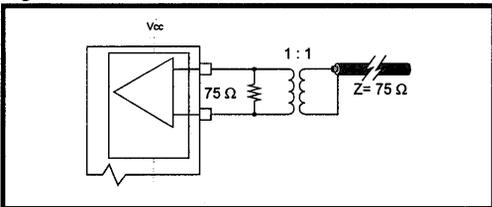
Figure 8: E1 Rx I/F for Twisted-Pair Lines
