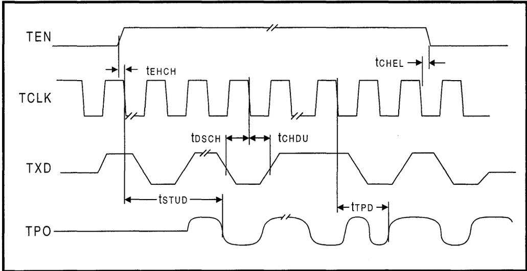
Figure 21: Mode 3 COL Output Timing
