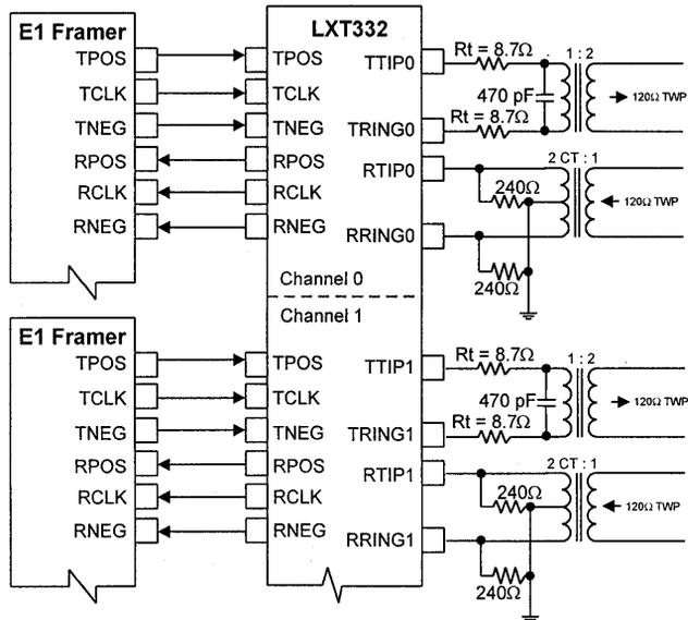
**Figure 2B: LXT332 120 Ω E1 Line Interface**
