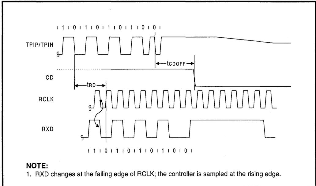
Figure 24: Mode 4 Transmit Timing
