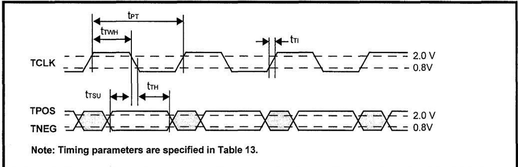
Figure 12: LS Serial Port Timing - 8-Bit Word
