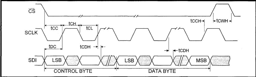
**Figure 17: LXT318 Serial Data Output Timing Diagram**
