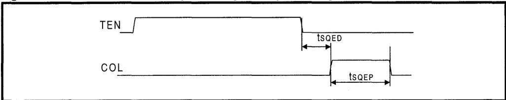
Figure 20: Mode 1 Loopback Timing
