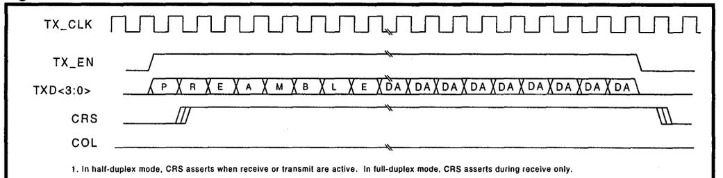
**Figure 13: 100BASE-TX Transmission with Collision**
