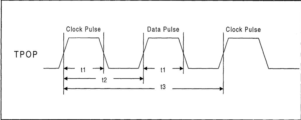
Figure 27: Fast Link Pulse Timing
