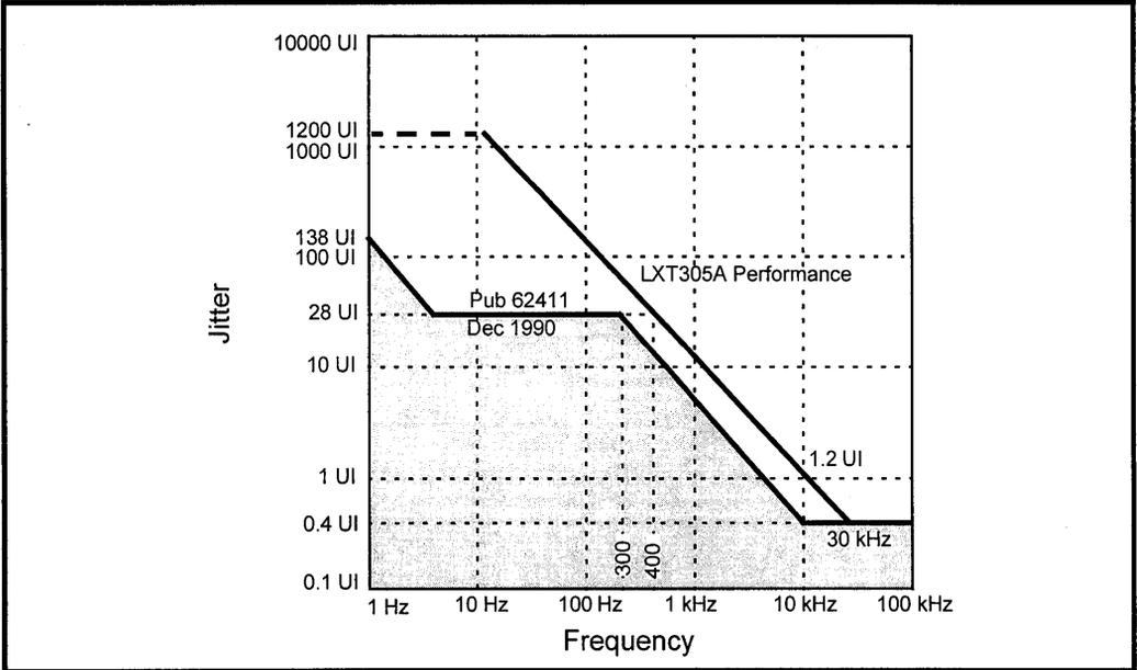
**Figure 7: LXT305A Transmit Jitter Transfer Performance (Typical)**
