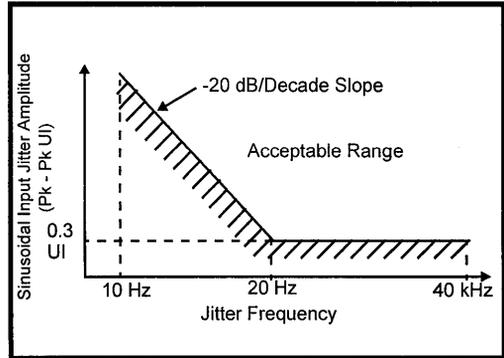
Figure 6: Receiver Jitter Transfer Template
