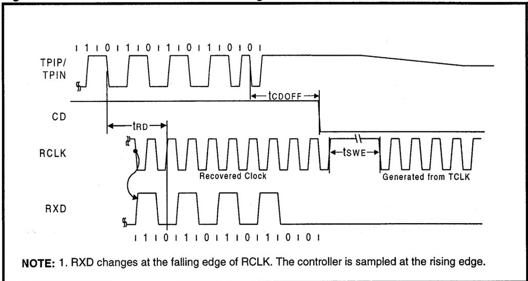
Figure 41: Mode 5 Transmit Timing
