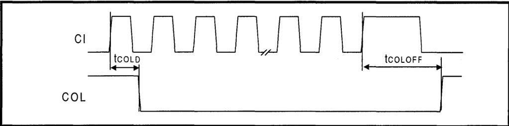
Figure 25: Mode 2 COL/SQE Output Timing
