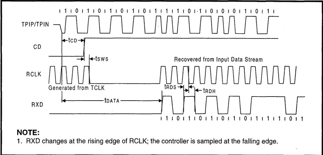
**Figure 19: Mode 3 RCLK/End-of-Frame Timing**
