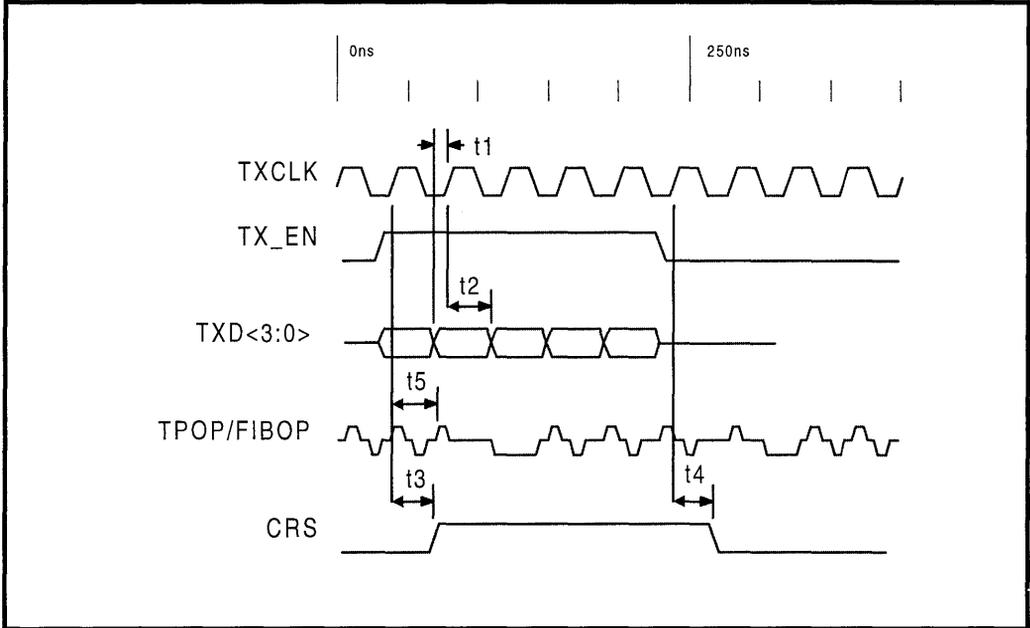
Table 30: MII - 100BASE-TX Transmit Timing Parameters / 4B Mode (Over Recommended Range)
