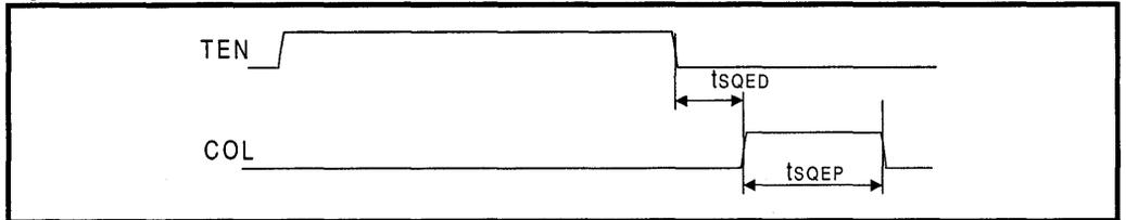
Figure 21: Mode 1 Loopback Timing
