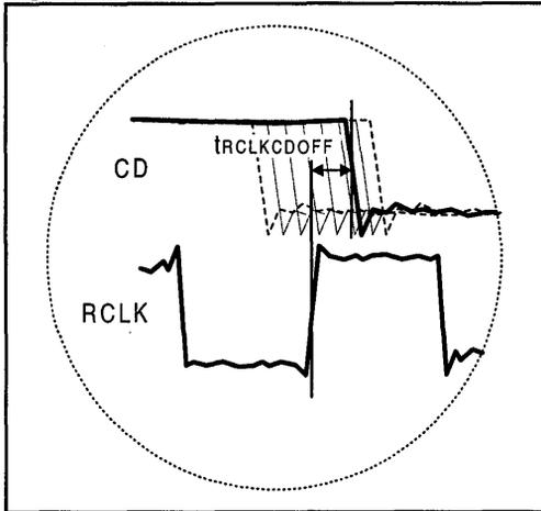
When  $trCLKCDOFF$  goes negative, the RCLK edge which normally precedes CD de-assertion now comes after CD de-assertion. This condition (Figure 3) presents compatibility problems with certain MAC chips from Intel and Motorola.
