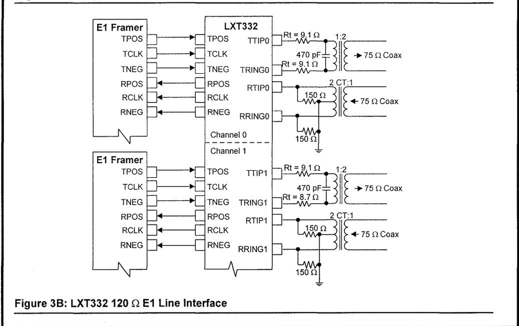
Figure 3B: LXT332 120 Ω E1 Line Interface
