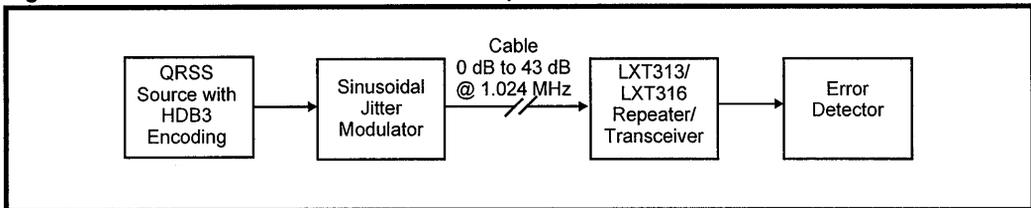
Figure 8: Receiver Jitter Transfer Test Setup
