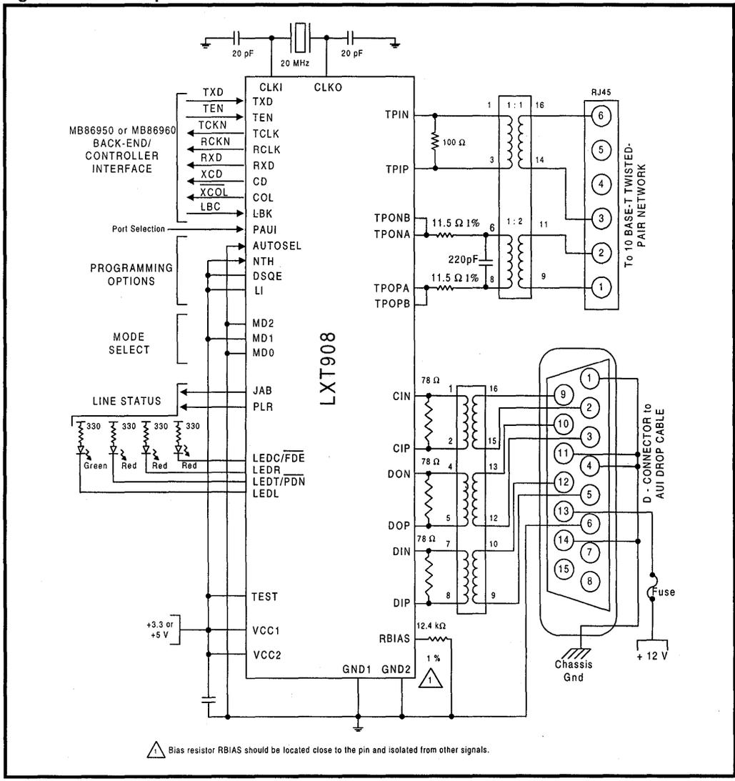
Figure 12: Manual Port Select with Seeq 8005 Controller
