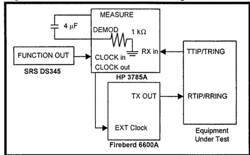
**Figure 3: Filter Calibration**
