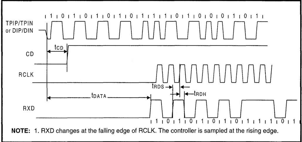
**Figure 34: Mode 4 RCLK/End-of-Frame Timing**
