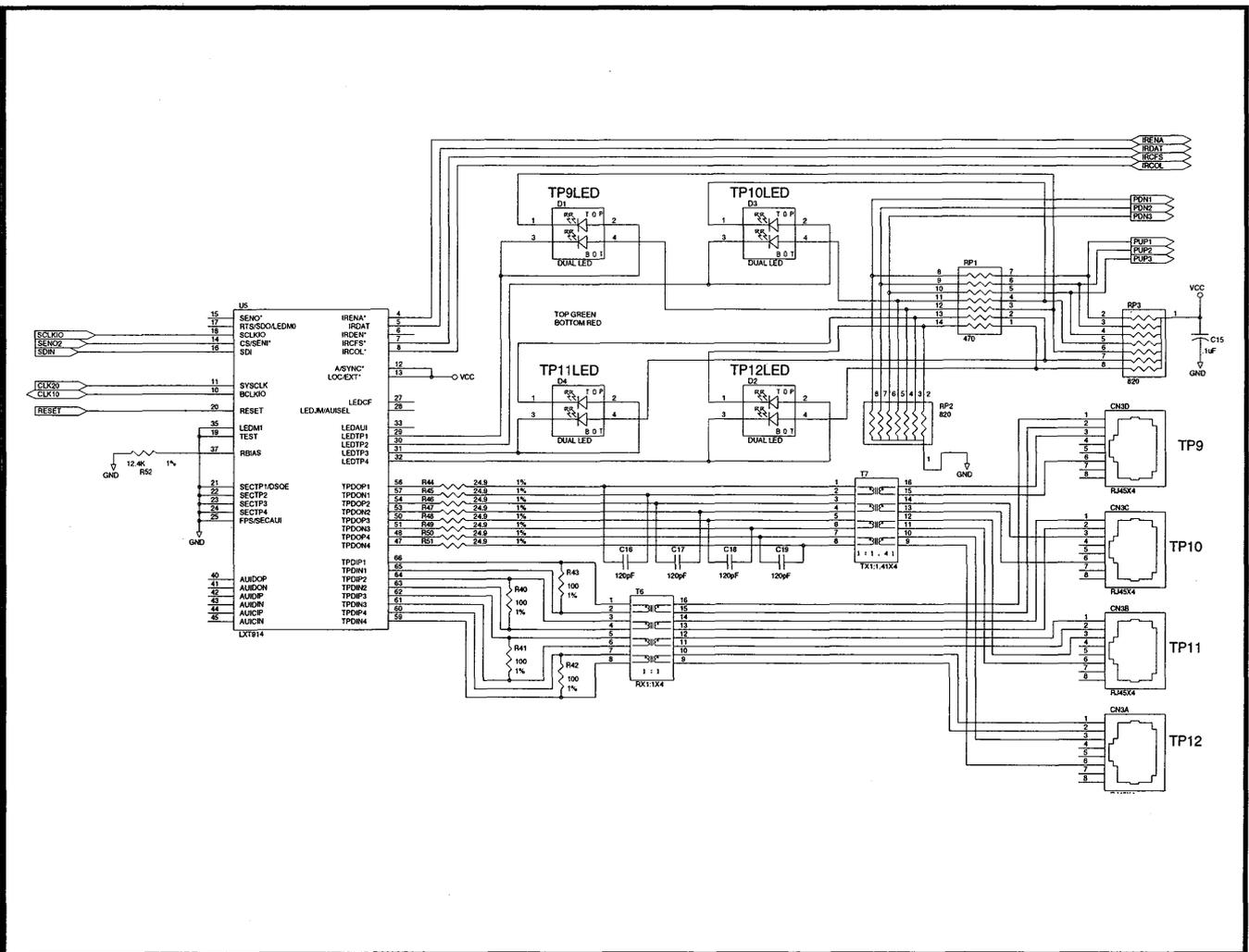
Figure 5: 12-Port Application Schematic, 68-Pin PLCC Package (Sheet 4 of 4)
