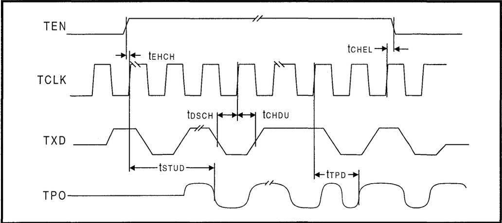
Figure 42: Mode 5 Collision Detect Timing
