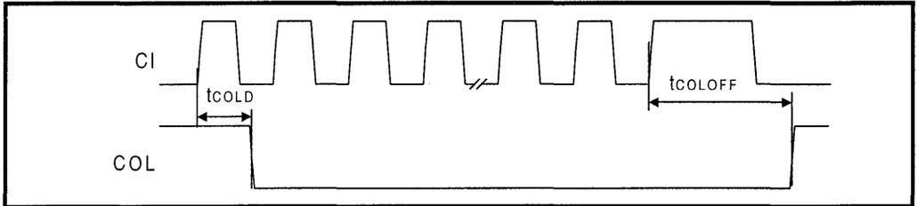
Figure 19: Mode 3 COL/CI Output Timing
