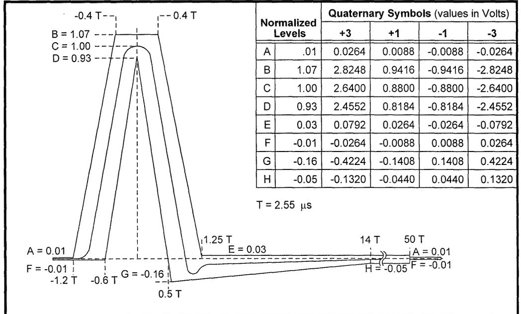
Figure 16: ACC Transmitter Timing
