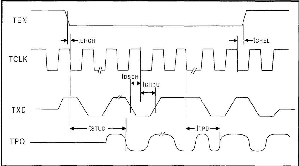
Figure 17: Mode 2 COL Output Timing
