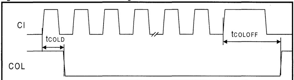
Figure 34: Mode 3 COL/CI Output Timing
