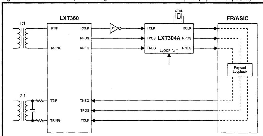
Figure 2: TBR12/13 Compliant Design with LOC Standalone JA (external loopback)
