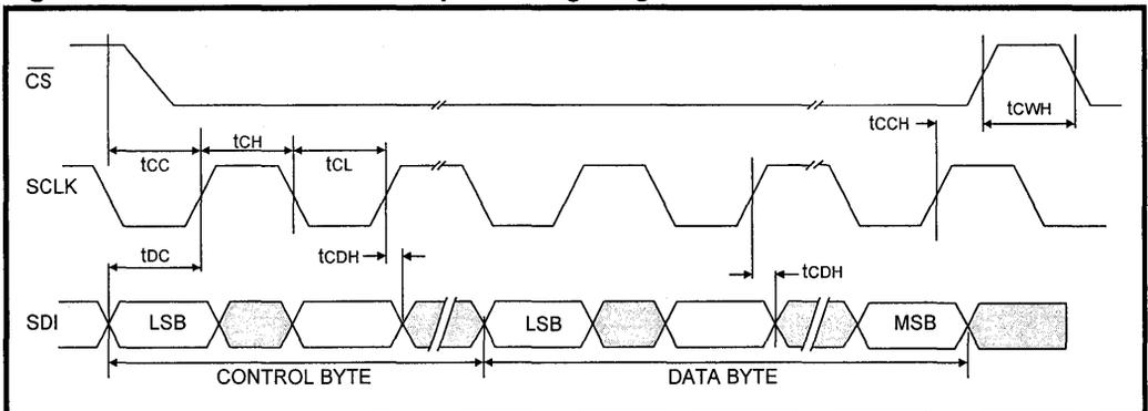
Figure 16: LXT307 Serial Data Output Timing Diagram
