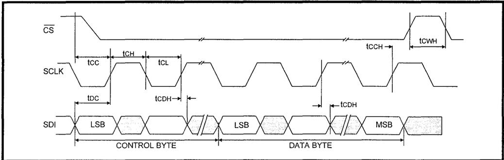
Figure 12: LXT310 Serial Data Output Timing Diagram
