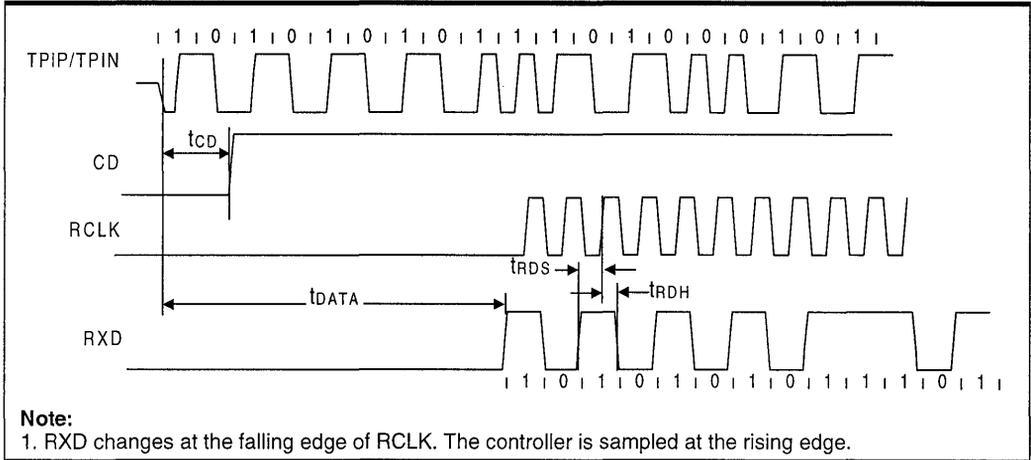
**Figure 23: Mode 4 RCLK/End-of-Frame Timing**
