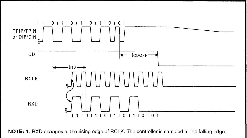
Figure 23: Mode 2 Transmit Timing
