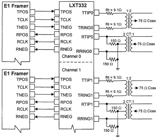
Figure 3B: LXT332 120 Ω E1 Line Interface
