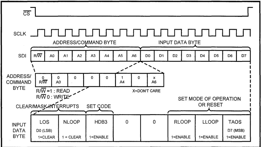
Figure 5: LXT318 Serial I/O Output Data Structure
