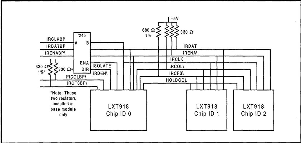
Figure 15: Typical Serial Management Interface Connections
