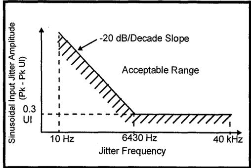
Figure 5: Receiver Jitter Transfer Template
