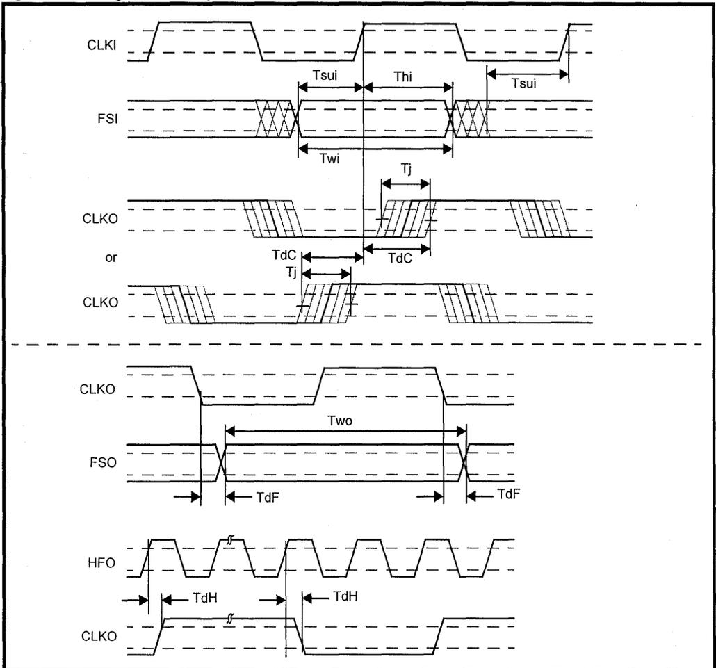
Figure 8: Output Frame Sync Alignment when  $HFO = 2 \times CLKO$
