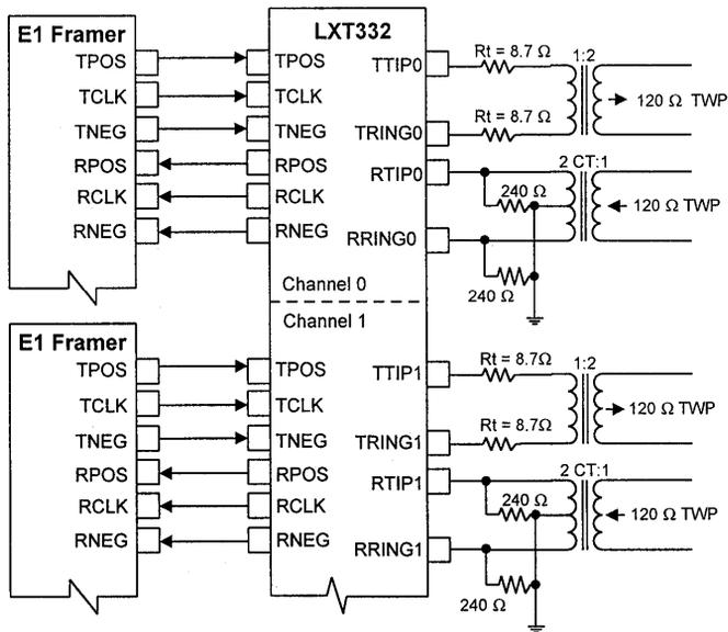
Figure 2B: LXT332 120 Ω E1 Line Interface
