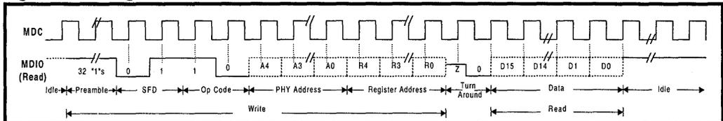
**Figure 5: Management Interface - Write Frame Structure**
