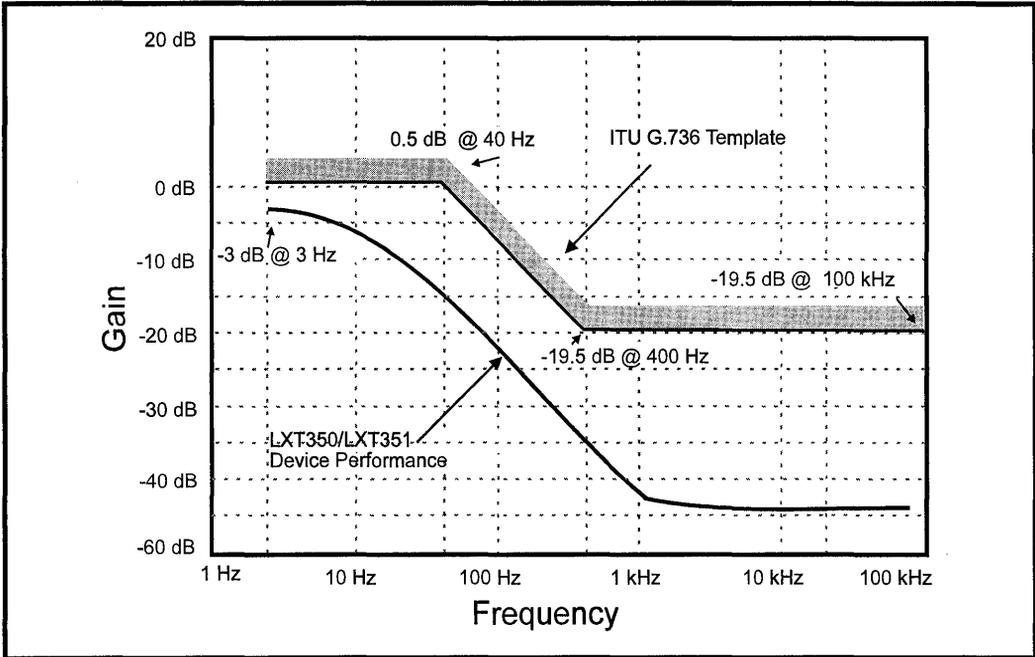
Figure 26: T1 Jitter Transfer Performance (Typical)
