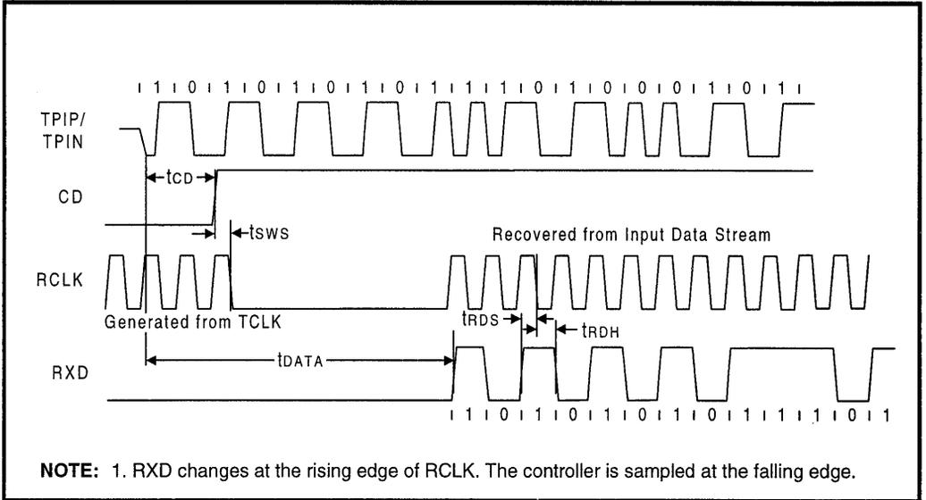
**Figure 28: Mode 3 RCLK/End-of-Frame Timing**
