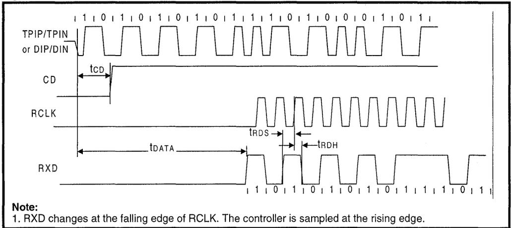
**Figure 37: Mode 4 RCLK/End-of-Frame Timing**
