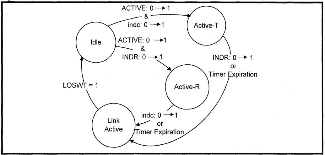
Figure 10: HDSL Synchronization State Machine
