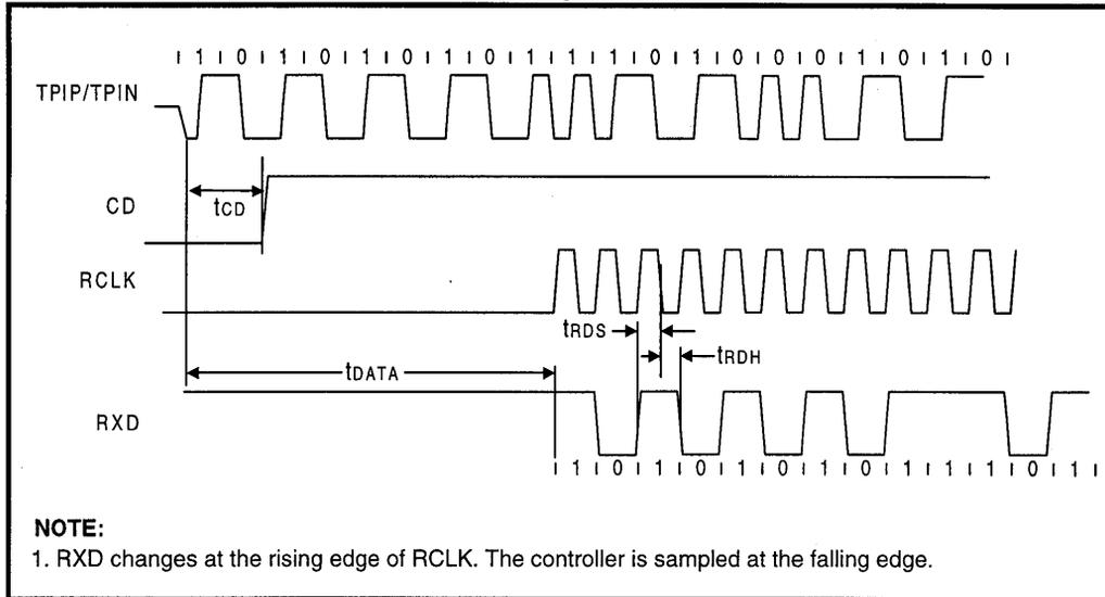
**Figure 15: Mode 2 RCLK/End-of-Frame Timing**
