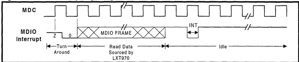
**Figure 4: Management Interface - Read Frame Structure**
