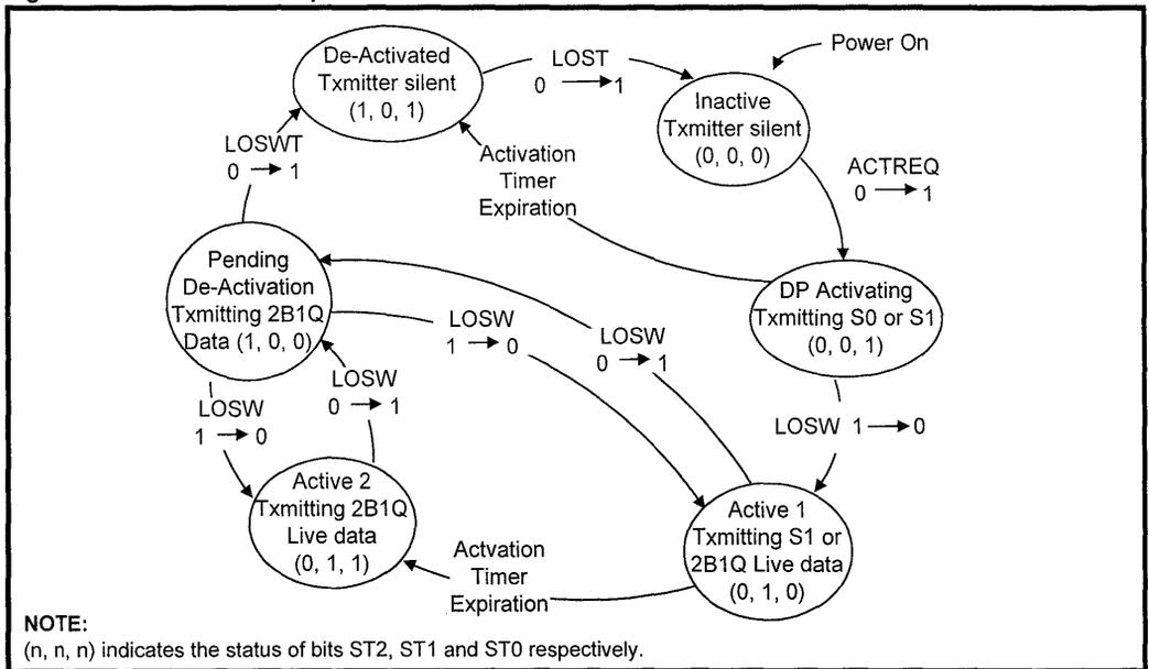
Figure 7: HTU-C HDSL Framer Activation State Machine
