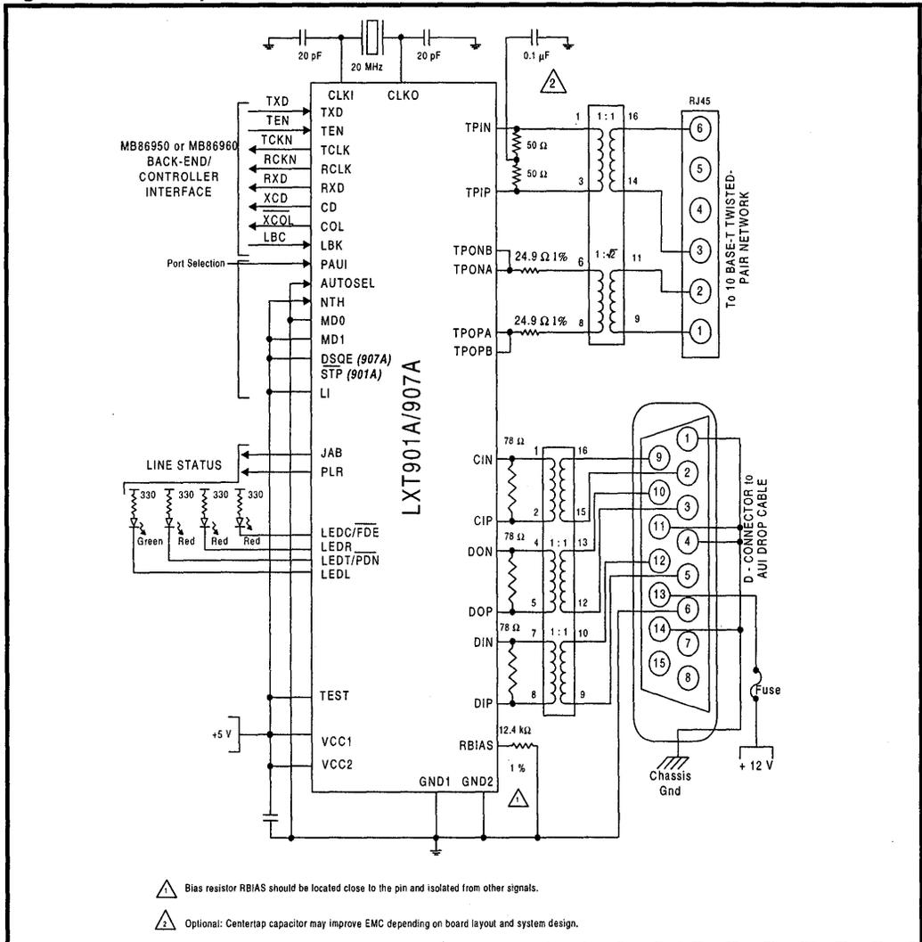
Figure 12: Manual Port Select with Seeg 8005 Controller
