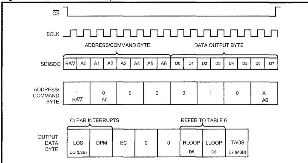
Figure 5: LXT307 Interrupt Handling
