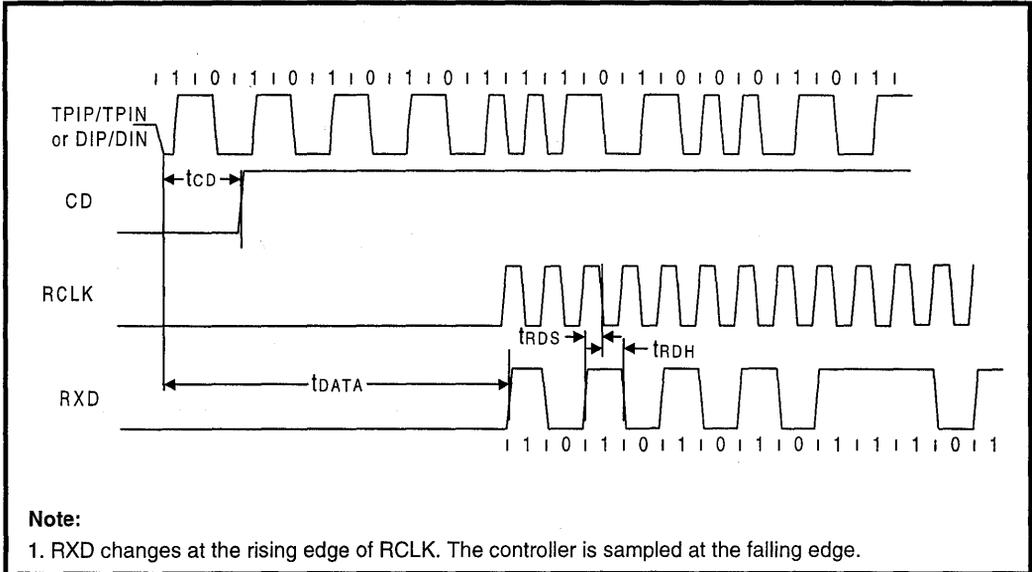
**Figure 29: Mode 3 RCLK/End-of-Frame Timing (LXT901A)**
