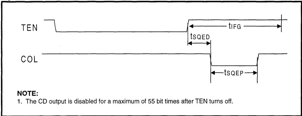
**Timing Diagrams for Mode 3** (*MD1=High, MD0=Low*) Figures 18 through 21
