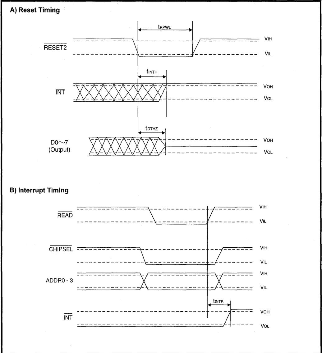
Figure 21: Parallel Data Channel Timing
