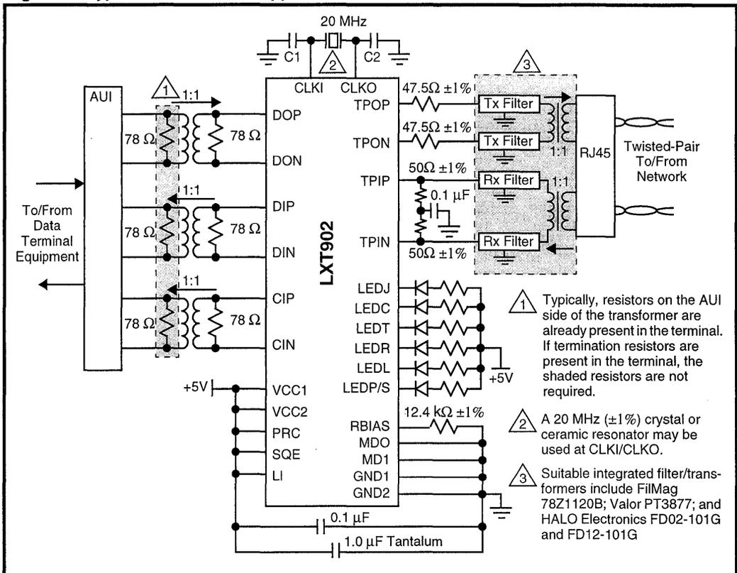
Figure 8: Typical Transmit Filter
