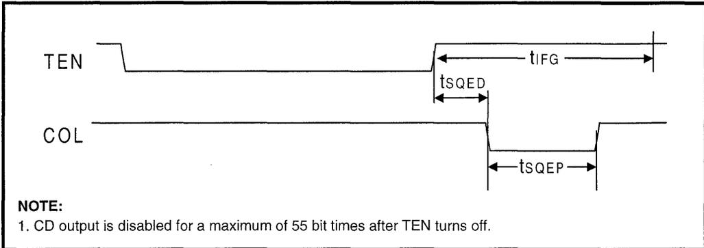
**Timing Diagrams for Mode 3** (MD1 = High, MD0 = Low) *Figures 18 through 21*
