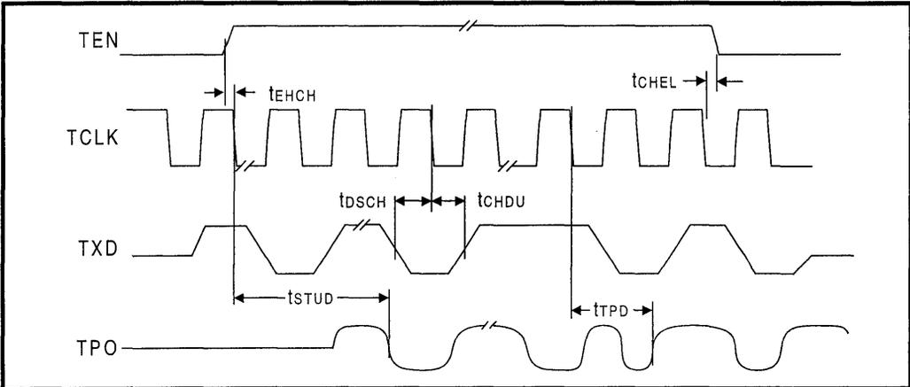
Figure 30: Mode 3 Collision Detect Timing
