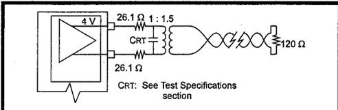
Figure 6: E1 Low Power Tx I/F for Twisted-Pair Lines
