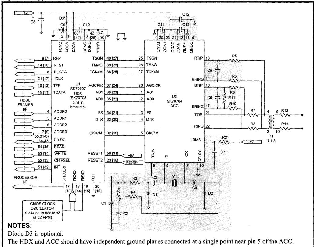
Figure 13: SK70707/SK70708 HDX Control and Status Signals (Hardware Mode)
