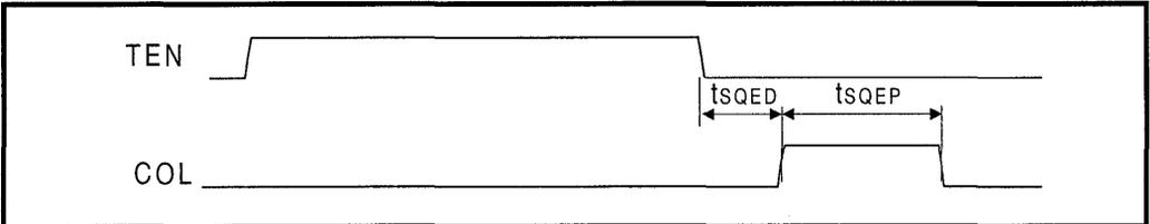
Figure 44: Mode 5 Loopback Timing
