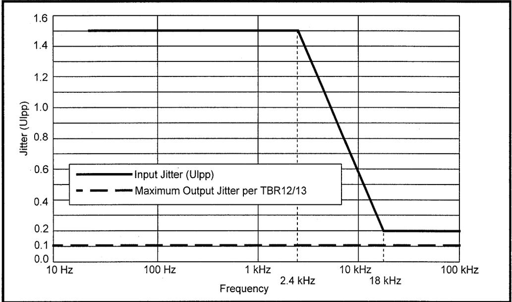
**Figure 5: Combined Jitter Attenuation Performance (LXT304A and LXT360)**
