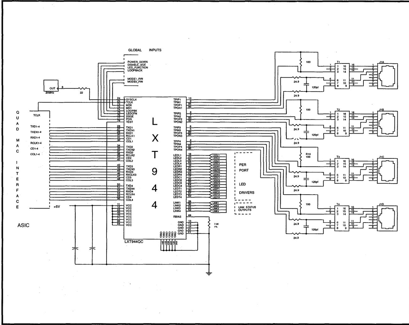
Figure 8: Receive Quad and Transmit Quad Application
