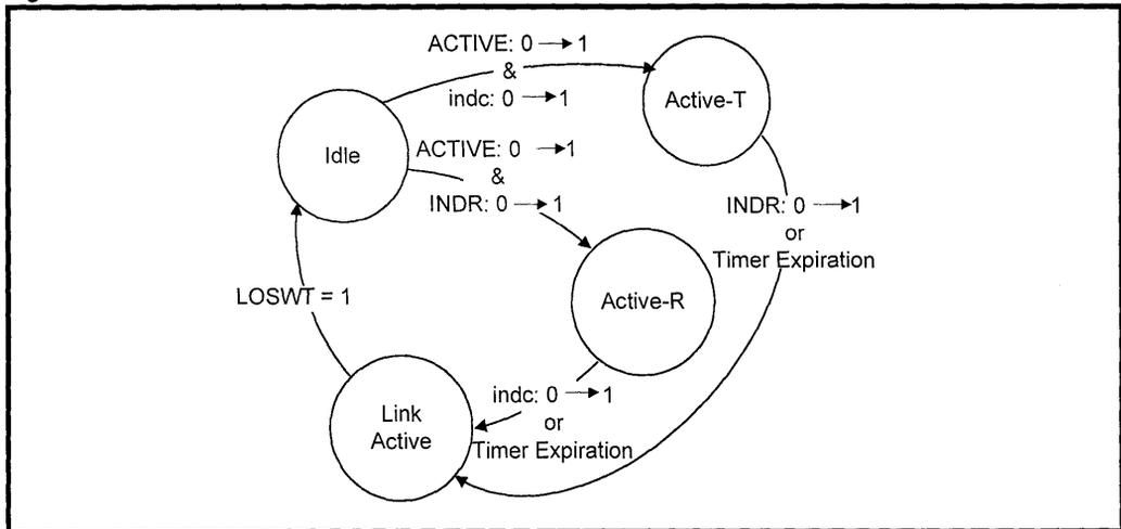
Figure 9: HDSL Synchronization State Machine
