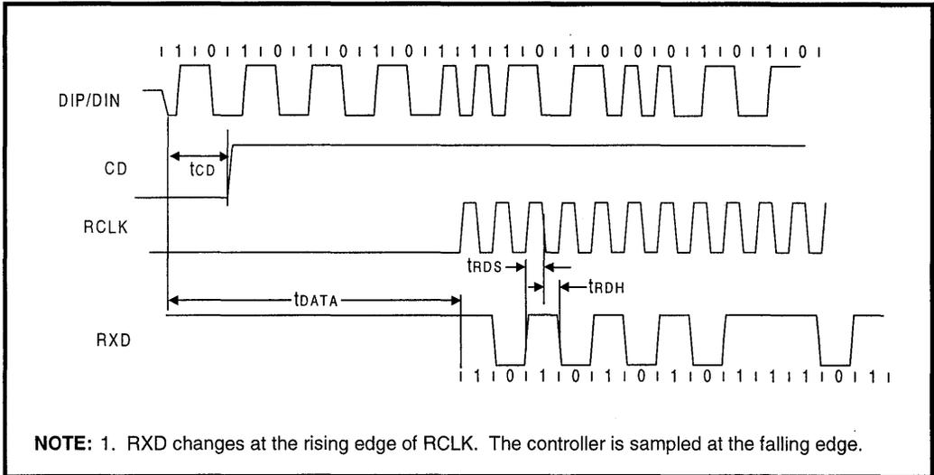
**Figure 10: Mode 2 RCLK/End-of-Frame Timing**
