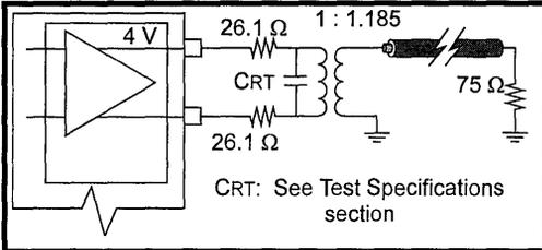
**Figure 4: Low Power Transmit Interface for Twisted Pair Lines**
