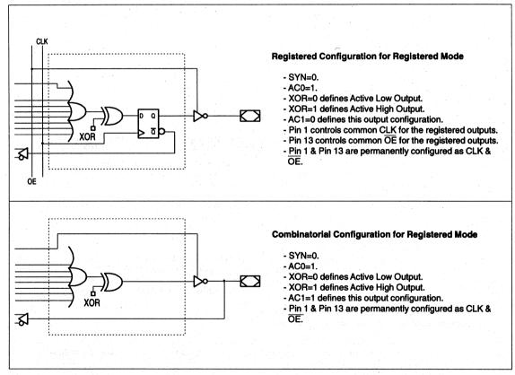
Note: The development software configures all of the architecture control bits and checks for proper pin usage automatically.
