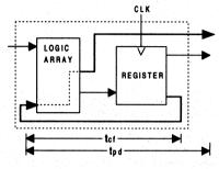
fmax with Internal Feedback 1/(tsu+tcf)
