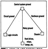
2. SEPARATE DEDICATED grounds should be supplied for the logic circuitry, noisy high-current devices, and the chassis. The three should come together at one point, the central system ground, which is usually located near the power supply.
