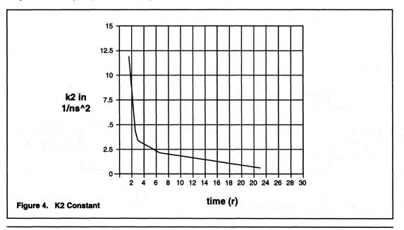
For a more quantitative look at the phenomenon of metastability, refer to the table beneath each plot. These tables list the measured values of the constants  $\Delta o$  and k2 for the device whose plot is shown, and for similar devices. Recall that large k2 and small  $\Delta o$  values are desirable. The numbers in the tables correlate closely with the results of earlier tests [1,5], confirming the validity of our test method.
