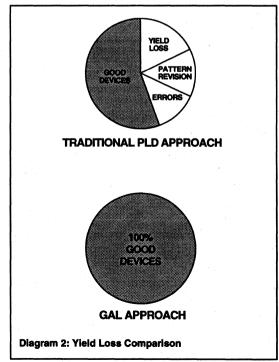
In a typical manufacturing environment, device programming hardware patterns the array, and assuming the engineer has provided test vectors, the hardware performs a basic (slow) functional test of the device. Yield losses at these two operations average 2% to 5% and 1% to 2%, respectively.
