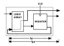
fmax with Internal Feedback 1/(tsu+tcf)
