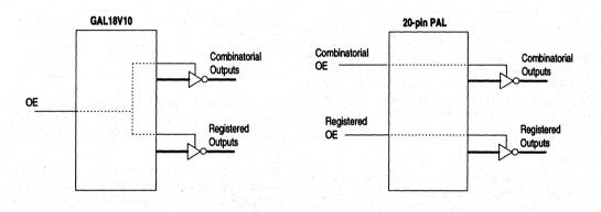
Figure 2. Output Enable Pin Consolidation
