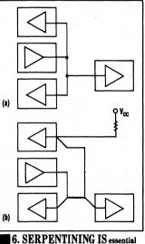
when terminating a line. Never split the line to feed parallel devices (a). Rather, feed them sequentially with a serpentined line (h)
