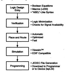
The pDS—PC Entry Level Software supports over 200 macros to help the design process. These macros cover most TTL functions, from gate primitives to 16-bit counters. pDS The software also supports user-definable macros which can be modifications of existing macros or custom creations.
