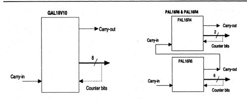
Figure 1. 8-bit Counter with Carry-In and Carry-Out
