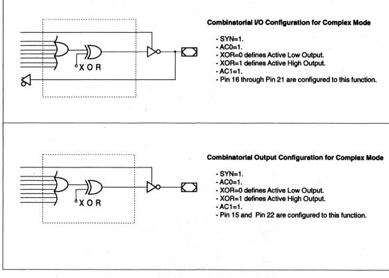
Note: The development software configures all of the architecture control bits and checks for proper pin usage automatically.
