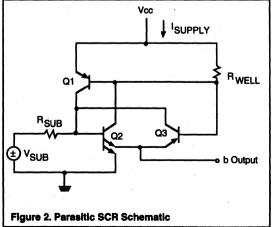
To prevent latch-up by large positive swings on the device outputs or I/O pins, NMOS output drivers were used. This eliminates the possibility of turning on  $Q_3$  (Figure 2) with an output bias in excess of the device supply voltage. Figure 3 contains the effective NMOS output driver and its switching characteristics. Note that the output does not fully reach the supply voltage, but still provides adequate  $V_{out}$  margin for TTL compatibility.
