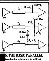
requires a separate 3-V supply (a). The Thevenin equivalent eliminates the need for a separate supply, but dissipates extra power from the regular 5-V supply (b). The use of a capacitor cuts dc dissipation altogether while supplying ac termination (c).
