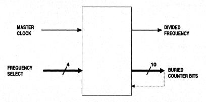
Figure 1. Block Diagram of Programmable Frequency Divider
