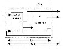
fmax with Internal Feedback 1/(tsu+tcf)
