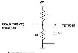
C LINCLUDES JIG AND PROBE TOTAL CAPACITANCE
