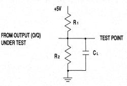
CL INCLUDES JIG AND PROBE TOTAL CAPACITANCE
