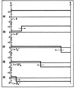
3. WAVE PROPAGATION along a transmission line occurs as follows: Prior to time zero, there is a steady-state voltage of 2.5 V dc on the line (a). At t = 0, the voltage at point A drops to 0.5 V, sending a negative pulse of -2 V toward point B (b). At  $t = T_D$ , that negative pulse is reflected from point B. It adds algebraically to the 0.5 V on the line and sends a -1.5-V pulse back toward point A (c). The reflections then continue as in (d) and (e).
