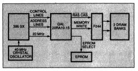
Fig 1—The PLD's internal circuitry can clock on both edges of the  $\mu$ P's clock, thereby synthesizing a 40-MHz clock for the memory system.
