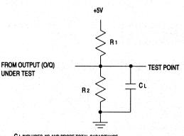
C L INCLUDES JIG AND PROBE TOTAL CAPACITANCE
