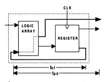
fmax with Internal Feedback 1/(tsu+tcf)
