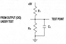
CL INCLUDES JIG AND PROBE TOTAL CAPACITANCE
