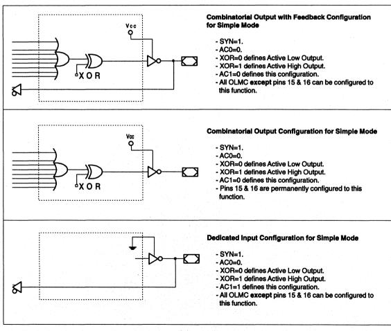
Note: The development software configures all of the architecture control bits and checks for proper pin usage automatically.
