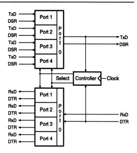
Figure 2. Block diagram of Port MUX
