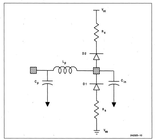
Figure 10. Input Buffer Model, Except Special Group
