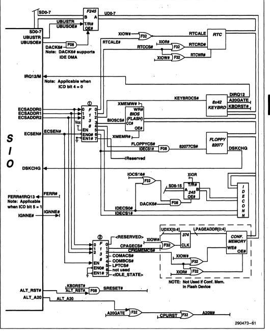
Figure 19. Utility Bus External Support Logic
