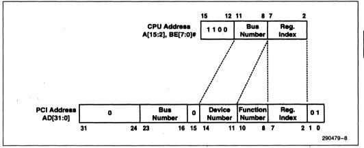
Figure 7. Mechanism #2 Type 1 Host-to-PCI Address Mapping
