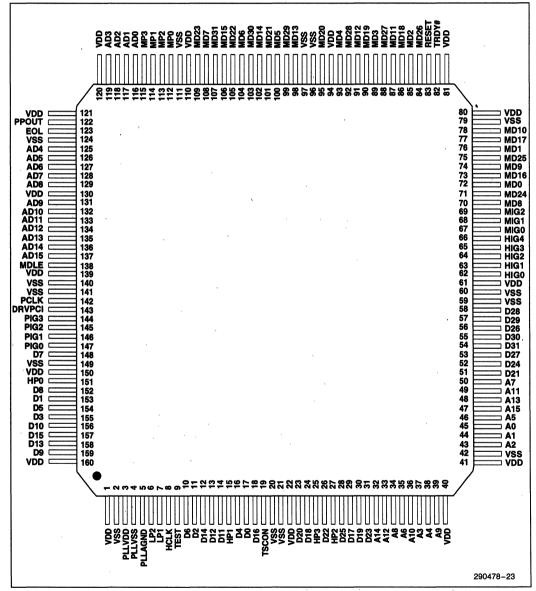
Figure 22. 82433LX and 82433NX Pin Assignment
