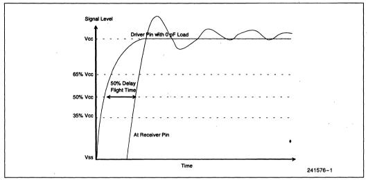
Figure 1. Flight Time Measurement
