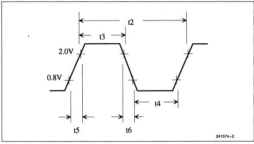
Figure 2. Clock Requirements for the Pentium™ Processor and CPU-Cache Chip Set
