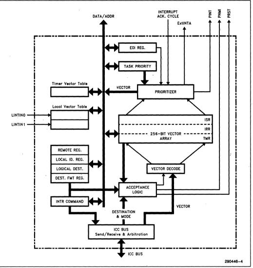
Figure 3. 82489DX Local Unit Block Diagram
