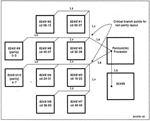
Figure 32. Improved Topology of A12 Net
