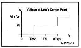
Figure 17. Voltage at the Midpoint of Circuit in Figure 16
