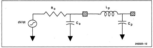
Figure 12. First Order Output Buffer Model
