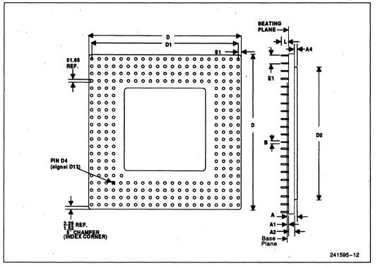
Figure 4-1. Pentium™ Processor (510\60, 567\66) Package Dimensions
