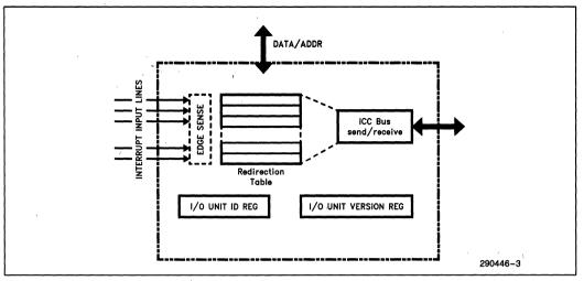
Figure 2. 82489DX I/O Unit Block Diagram
