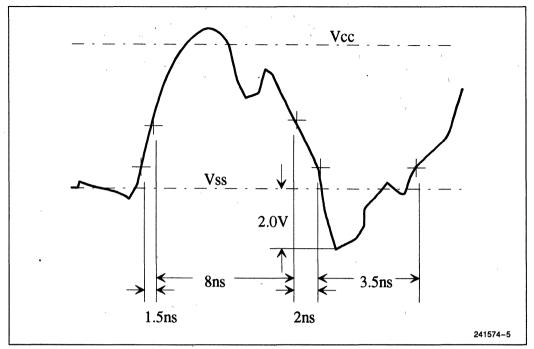
Figure 5. An Example of an Unacceptable Clock Waveform (Diodes Are Absent from the Input Model)
