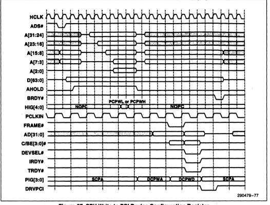
Figure 67. CPU Write to PCI Device Configuration Register
