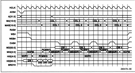
Figure 47. Burst DRAM Write Cycle-Page Hit
