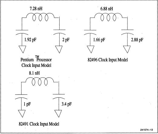
Figure 13. Pentium™ Processor, 82496 and 82491 Clock Input Models
