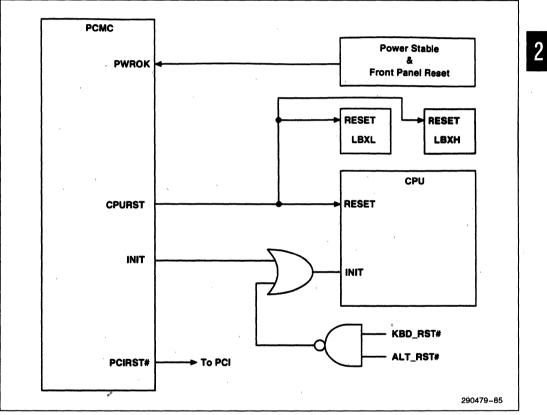
Figure 75. PCMC System Reset Logic
