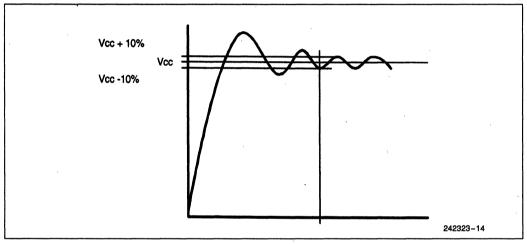
Figure 14. Settling Time
