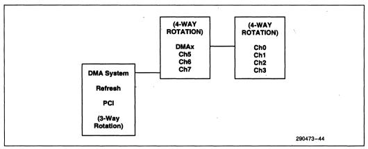
Figure 9. ISA Arbiter with DMA in Rotating Priority
