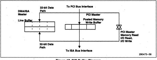
Figure 17. SIO Buffer Diagram
