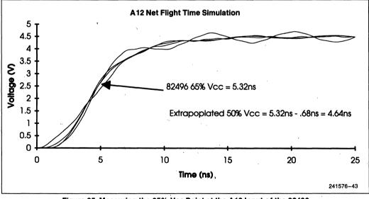
Figure 35. Measuring the 65% Vcc Point at the A12 Input of the 82496
