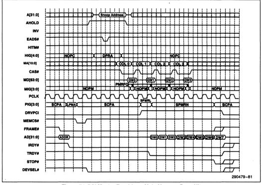
Figure 71. PCI Master Read from Main Memory-Page Hit
