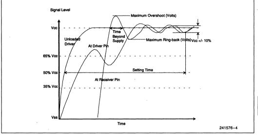
Figure 4. Signal Quality Parameter Measured for Low-to-High Transitions
