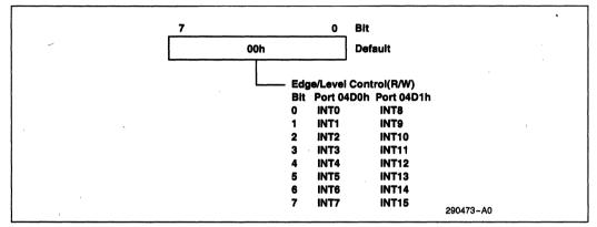
Figure 4. Edge/Level Select Register
