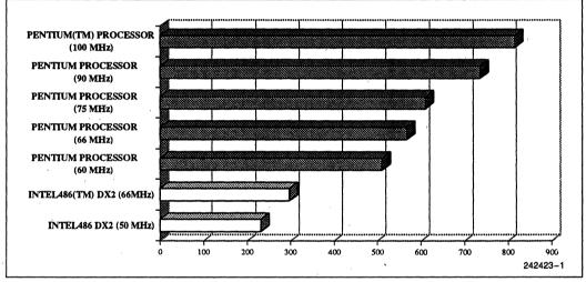
Figure 1. iCOMP™ Index Ratings for Intel Processors
