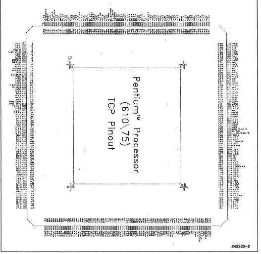
Figure 2. Pentium™ Processor (610\75) TCP Pinout
