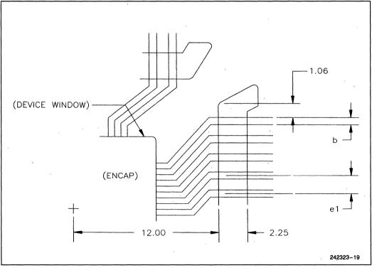
Figure 19. Outer Lead Bond (OLB) Window Detail
