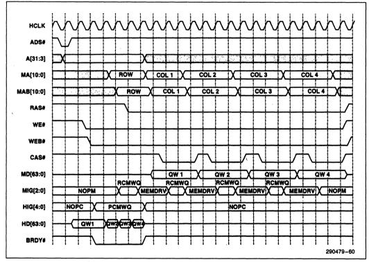
Figure 51. Burst DRAM Write Cycle, 0-Active RAS# Mode
