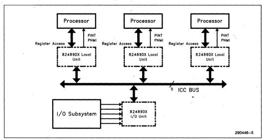
Figure 4. I/O Units and Local Units
