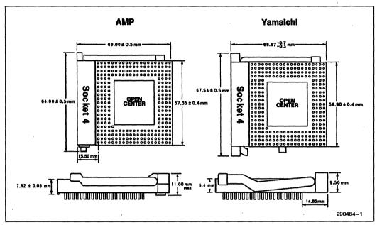
Figure 1. Socket 4 Footprint Dimensions (See socket manufacturer for the most current information.)
