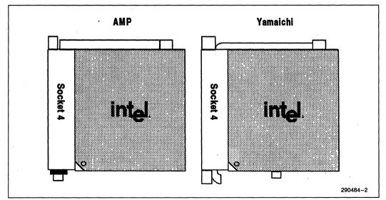
Figure 2. Chip Orientation in Socket 4
