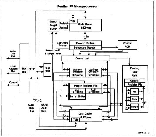
Figure 1-1. Pentium™ Processor (510\60, 567\66) Block Diagram
