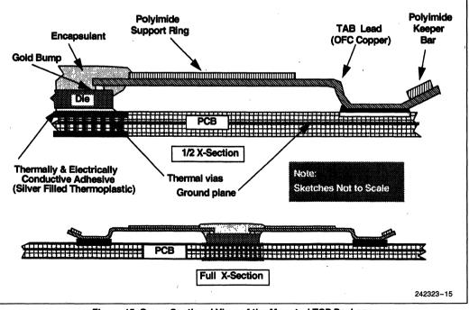
Figure 15. Cross-Sectional View of the Mounted TCP Package
