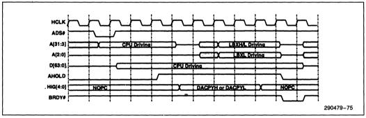
Figure 65. CPU Write to a PCMC Configuration Register
