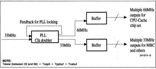
Figure 9. Clock Generation Using Clock Doubler
