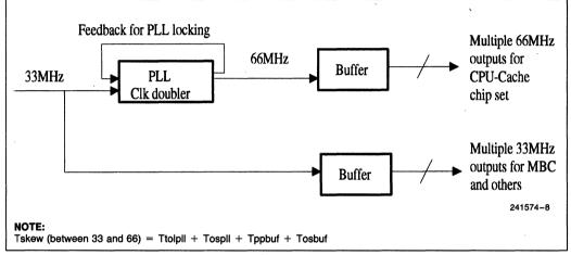
Figure 8. Clock Generation Using Clock Doubler
