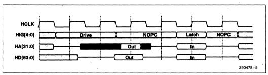
Figure 4. HIG[4:0] Command Timing
