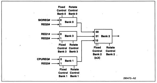
Figure 6. Arbiter Configuration Diagram for 82378ZB
