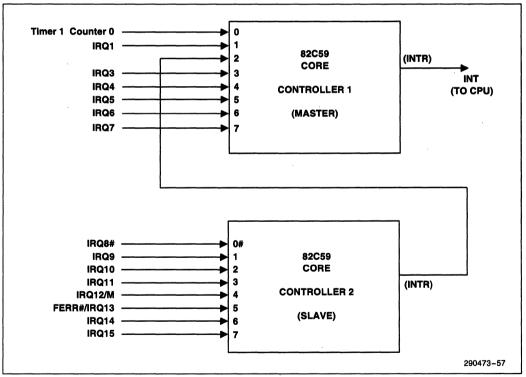
Figure 18. Block Diagram of the Interrupt Controller
