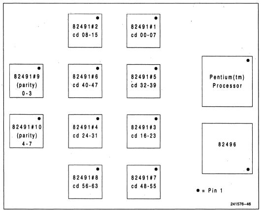
Figure 38. Component Placement
