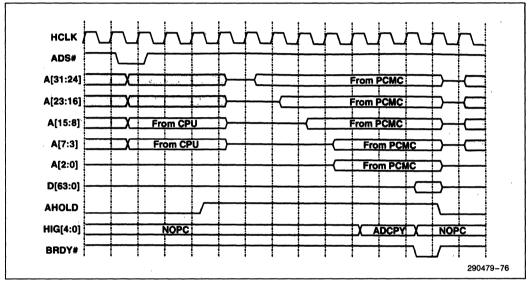
Figure 66. CPU Read from PCMC Configuration Register
