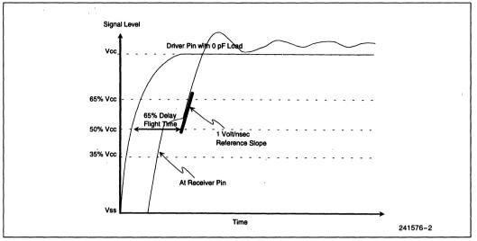
Figure 2. Flight Time Extrapolated from 65% Point
