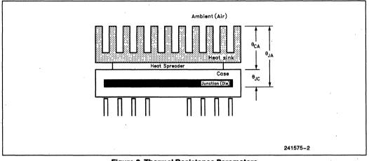
Figure 2. Thermal Resistance Parameters
