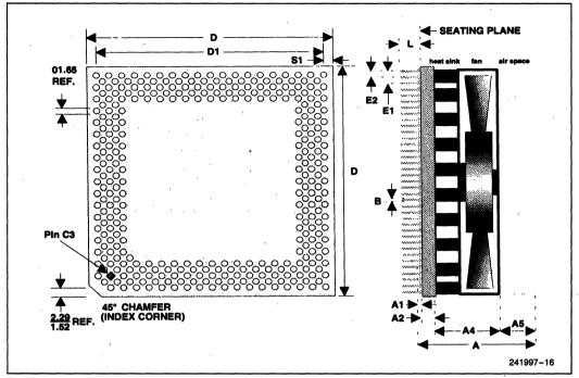
Figure 16. Future Pentium™ OverDrive™ Processor Package Dimensions
