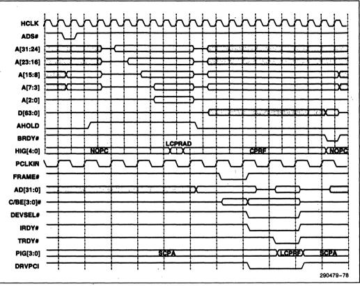
Figure 68. CPU Read from PCI Device Configuration Register
