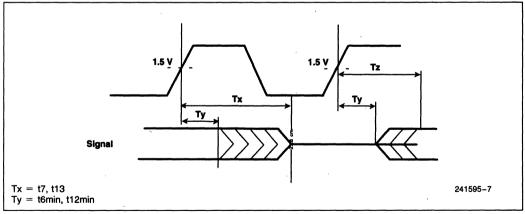
Figure 3-3. Float Delay Timings
