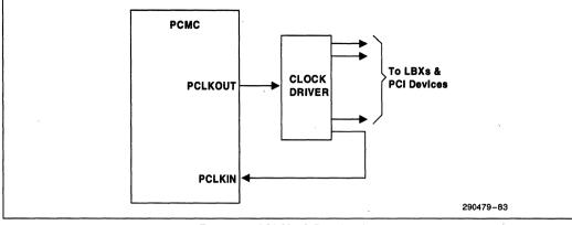
Figure 73. PCI Clock Distribution
