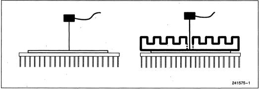
Figure 1. Thermocouple Attachment
