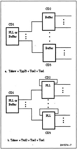
Figure 7. Examples of Clock Generation
