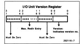
I/O Unit Version Register is read only register. It reads as 000F 00XX where XX is version.
