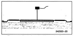
Figure 20. Technique for Measuring Case Temperature (T<sub>C</sub>)
