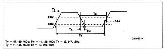
Figure 4. Clock Waveform
