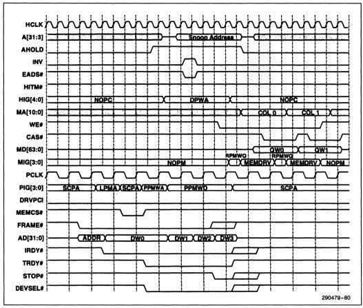
Figure 70. PCI Master Write to Main Memory-Page Hit
