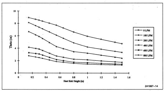
Figure 14. Thermal Resistance vs. Heatsink Height
