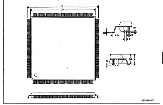
Figure 87. 208-Pin Quad Flatpack (QFP) Dimensions
