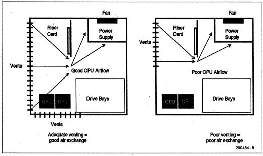
**Figure 8. Airflow Design Examples**
