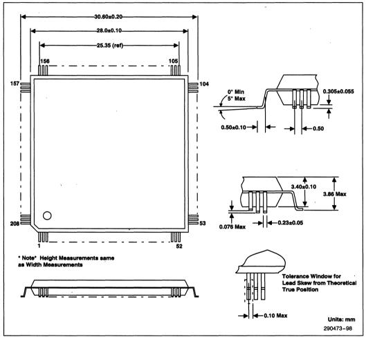
Figure 23. 208-Pin Quad Flat Pack (QFP) Package Dimensions
