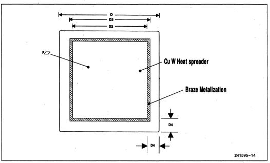
Figure 4-2. Pentium™ Processor (510\60, 567\66) Package Dimensions
