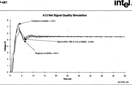
Figure 37. Measuring the Signal Quality of the 82496
