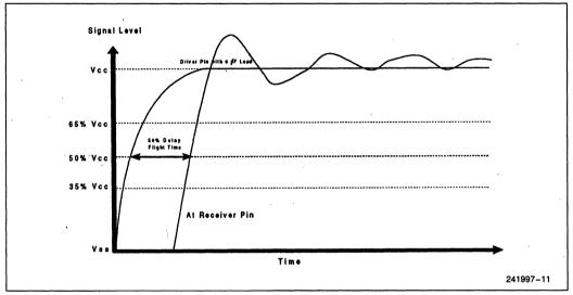
Figure 11. 50% V<sub>CC</sub> Measurement of Flight Time
