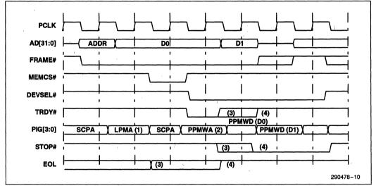
Figure 9. EOL Signal Timing for PCI Master Writes
