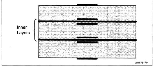
Figure 78. Board Layer Stackup
