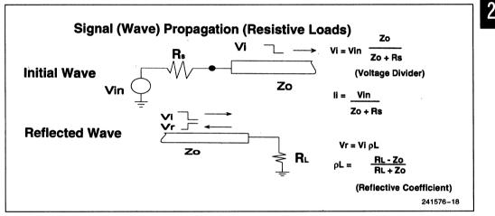
Figure 16. Signal Propagation Along a Transmission Line with Resistive Loads
