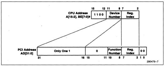
Figure 6. Mechanism #2 Type 0 Host-to-PCI Address Mapping
