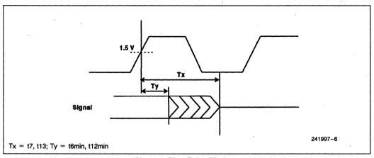
Figure 6. Float Delay Timings
