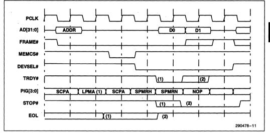
Figure 10. EOL Signal Timing for PCI Master Reads
