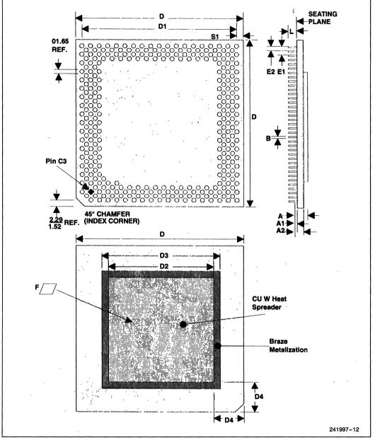
Figure 12. Pentium™ Processor (610\75, 735\90, 815\100) Package Dimensions
