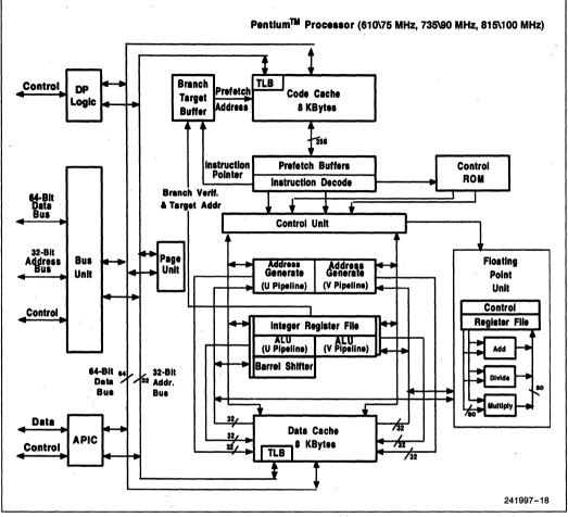
Figure 1. Pentium™ Processor Block Diagram
