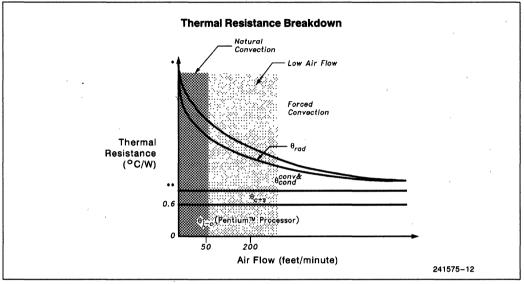
Figure A-1. Thermal Resistance
