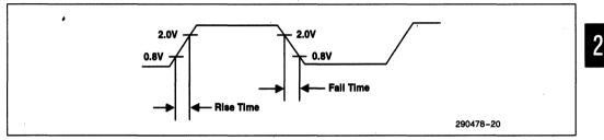
Figure 19. Clock Rise and Fall Times
