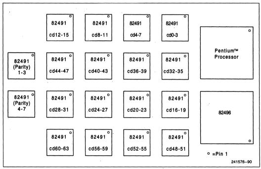
**Figure 59. Component Placement**
