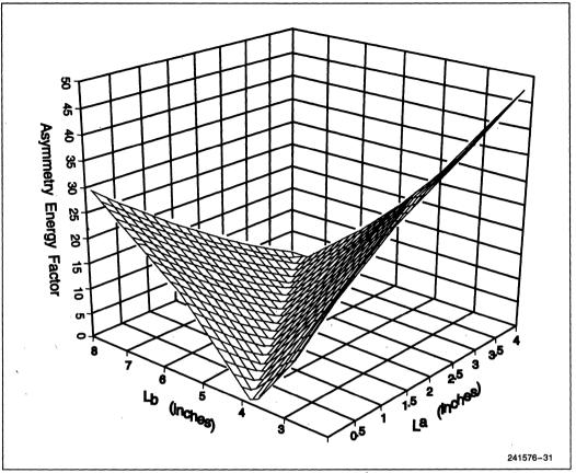
Figure 25. Energy Minimization for a Given Topology
