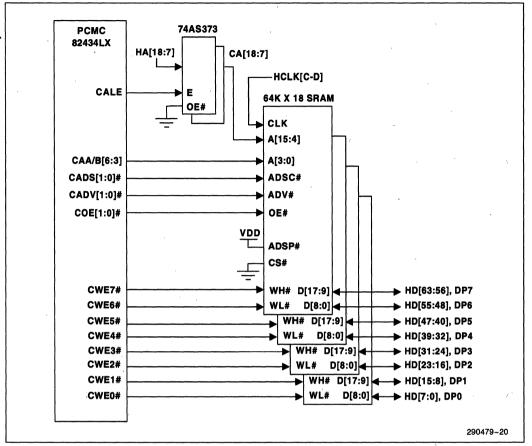
Figure 18. 82434LX Connections for 512-KByte Cache with Burst SRAM
