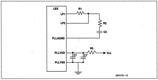
Figure 11. Loop Filter Circuit
