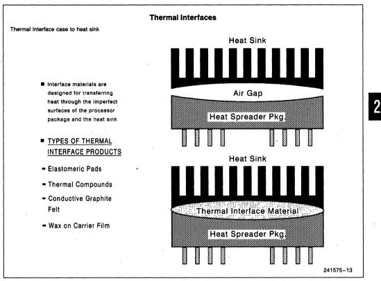
**Figure A-2. Thermal Interfaces**
