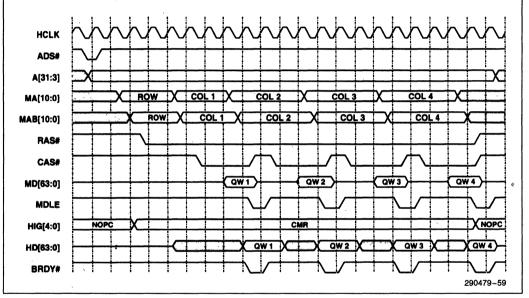
Figure 50. Burst DRAM Read Cycle, 0-Active RAS# Mode
