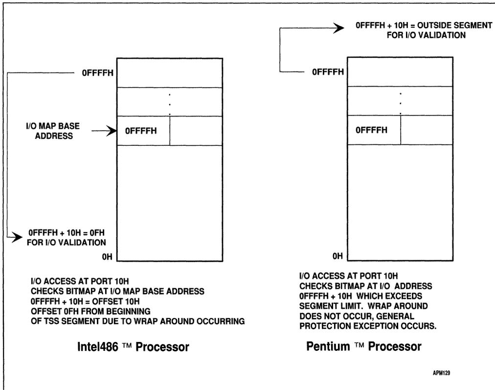
Figure 23-3. I/O Map Base Address Differences
