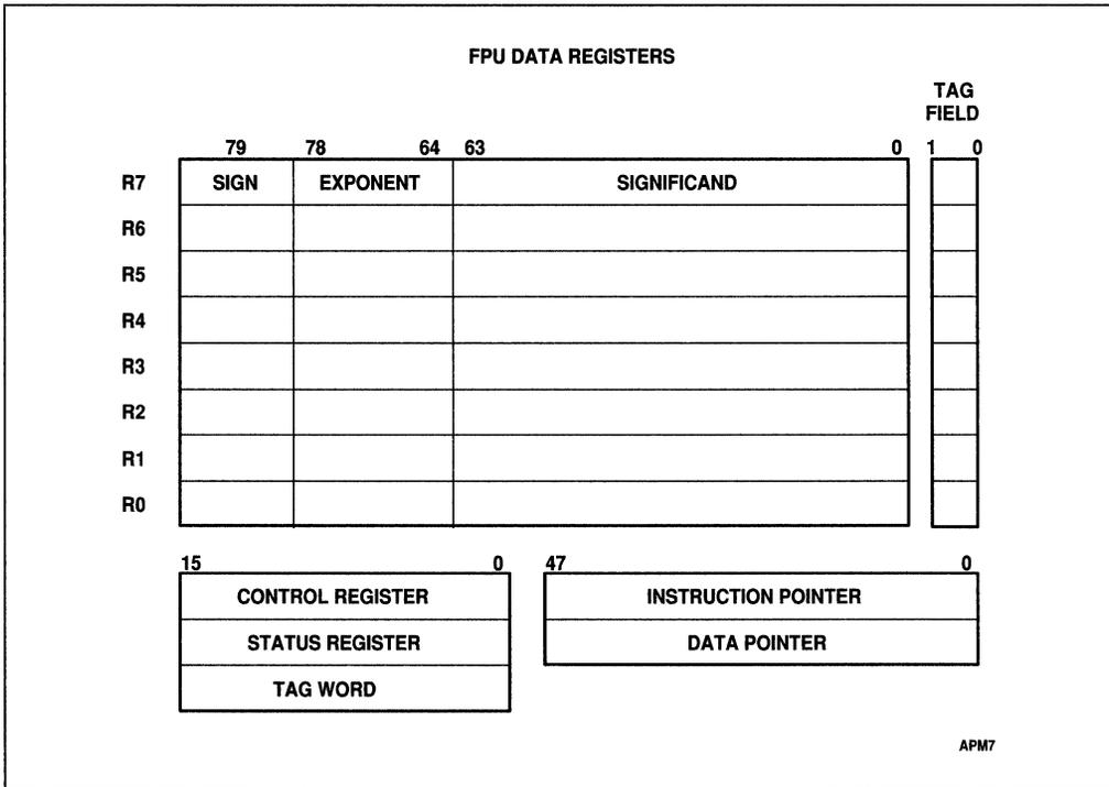
**Figure 6-1. Floating-point Unit Register Set**
