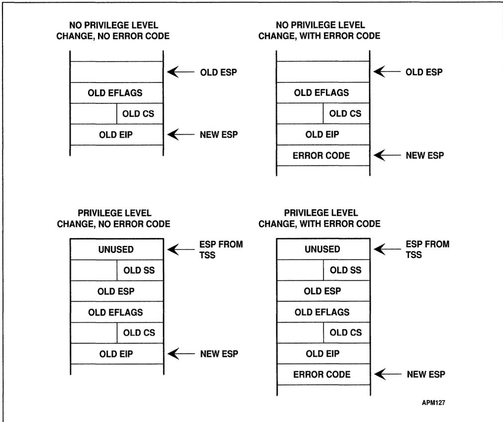
Figure 14-4. Stack Frame after Exception or Interrupt
