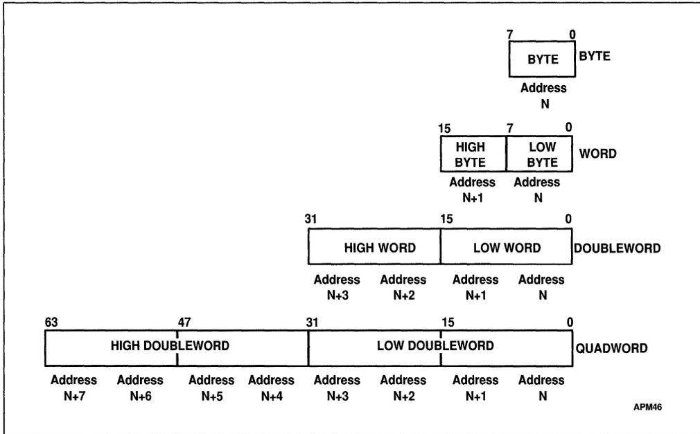
Figure 3-2. Fundamental Data Types
