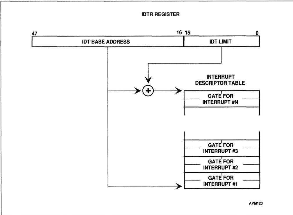
**Figure 14-1. IDTR Locates IDT in Memory**
