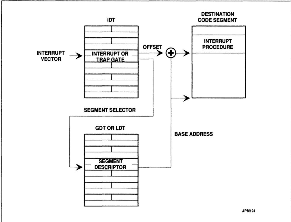
Figure 14-3. Interrupt Procedure Call
