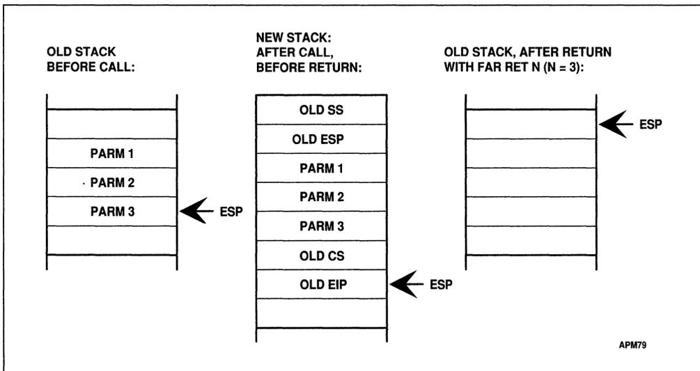
**Figure 12-9. Stack Frame During Interlevel Call**
