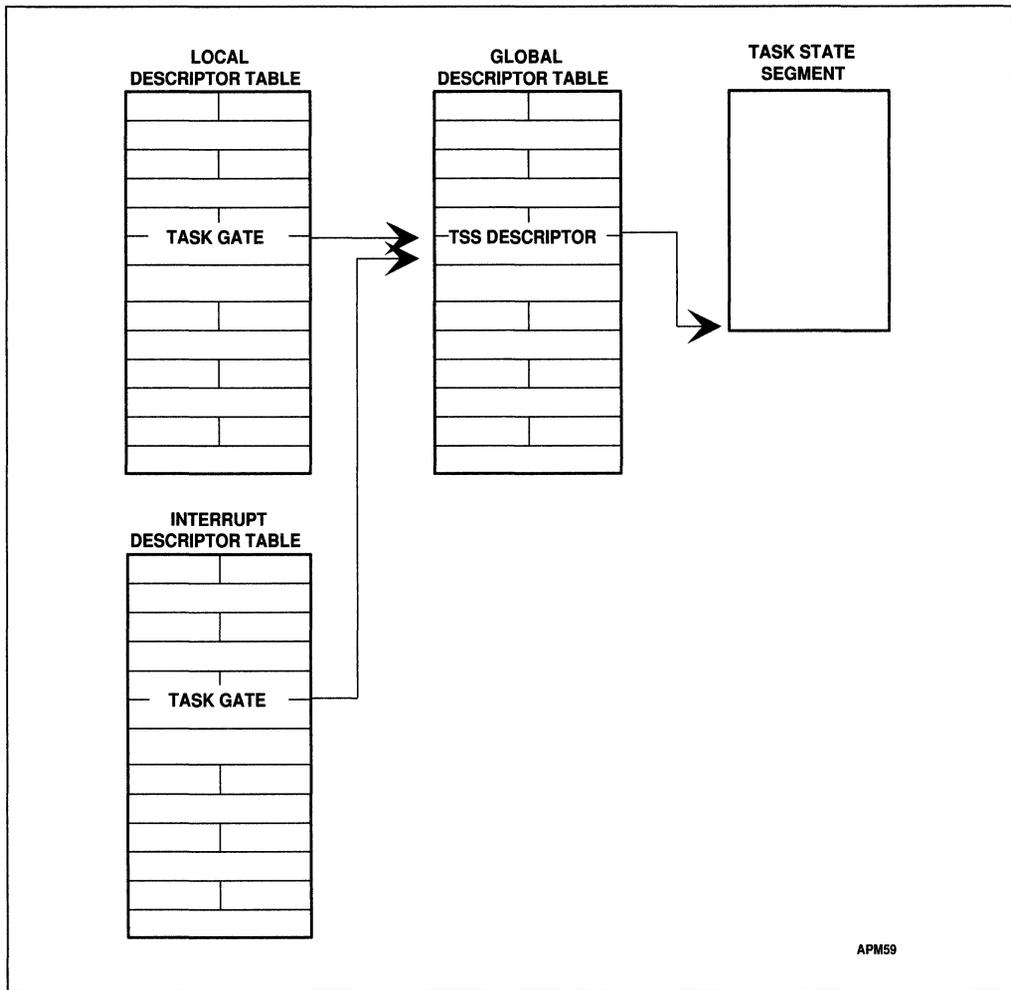
Figure 13-5. Task Gates Reference Tasks
