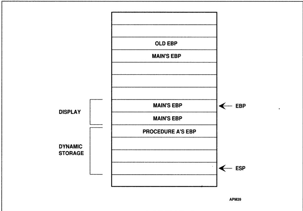
Figure 4-17. Stack Frame After Entering PROCEDURE A
