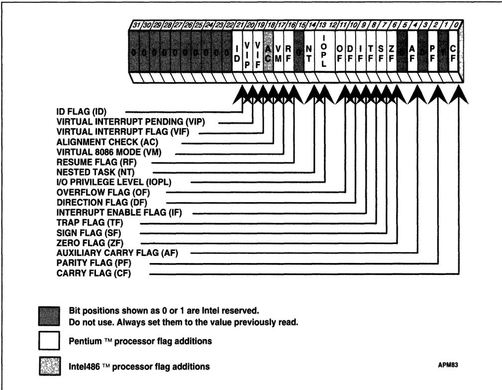
Figure 23-1. Pentium™ Processor EFLAGS Register
