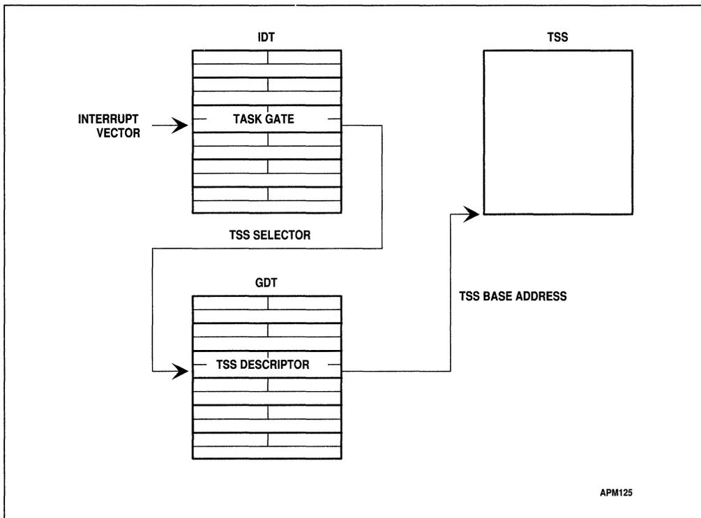
**Figure 14-5. Interrupt Task Switch**
