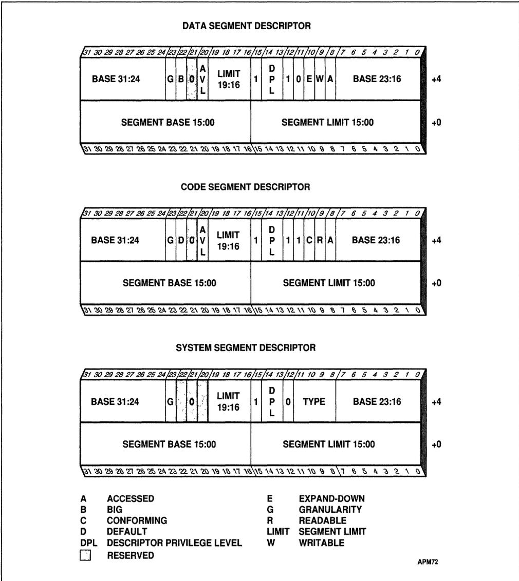
Figure 12-1. Descriptor Fields Used for Protection
