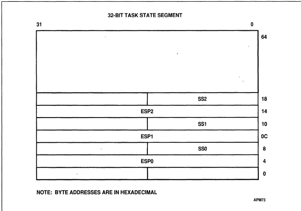
**Figure 12-8. Initial Stack Pointers in a TSS**
