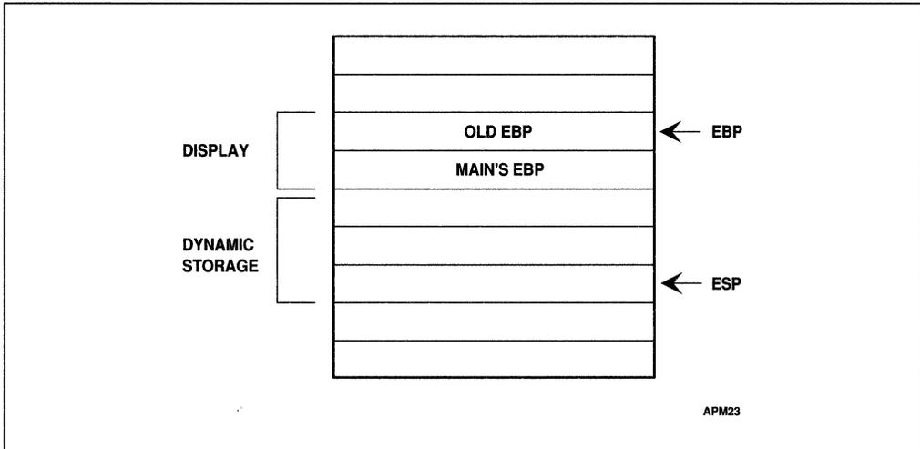
**Figure 4-16. Stack Frame After Entering MAIN**
