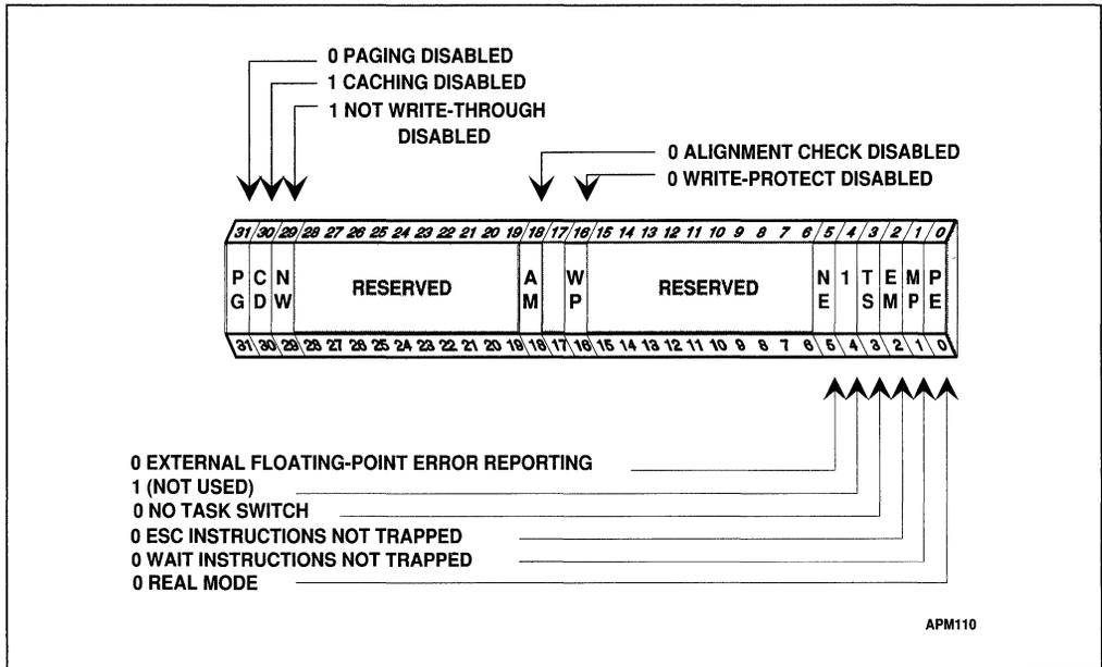
Figure 16-2. Contents of CR0 Register After Reset
