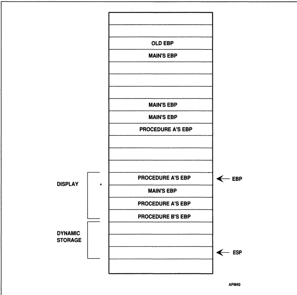
Figure 4-18. Stack Frame After Entering PROCEDURE B
