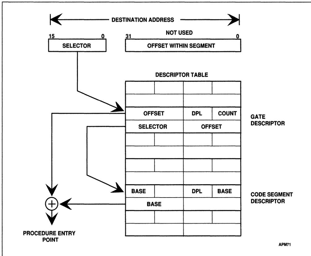
Figure 12-6. Call Gate Mechanism
