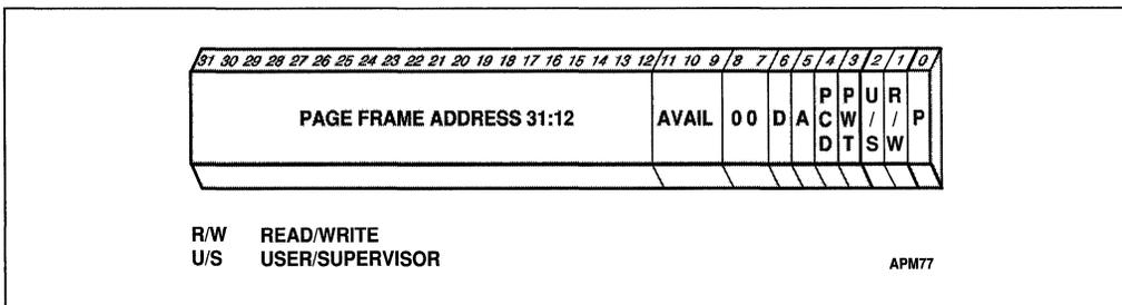
Figure 12-10. Protection Fields of a Page Table Entry
