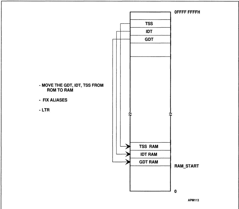
Figure 16-5. Moving The GDT, IDT, and TSS from ROM to RAM
