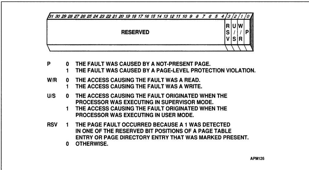
Figure 14-7. Page Fault Error Code
