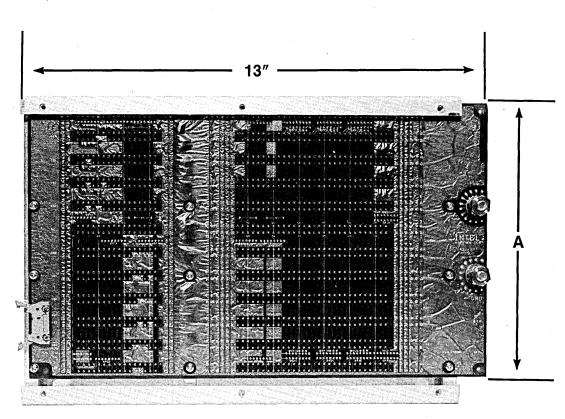
6 SLOT 4.5" A = 12 SLOT 9" 18 SLOT 13.5"
