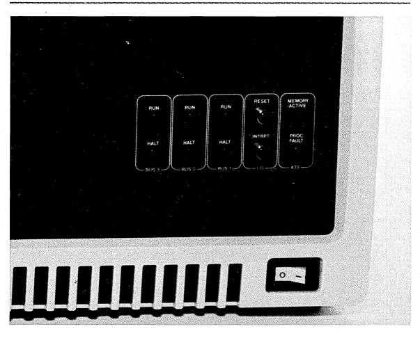
Figure 2-8. Operator's Panel
