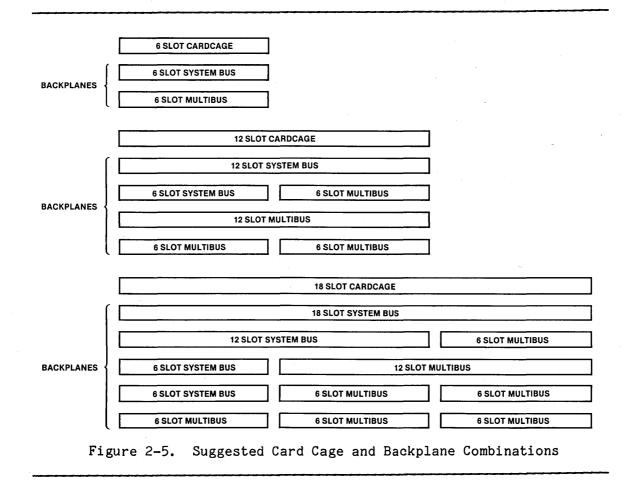
More than one card cage may be used in a single system, and card cage sizes may be intermixed in a system.
