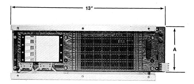
$A = \frac{6 \text{ SLOT } 4.5''}{12 \text{ SLOT } 9''}$
