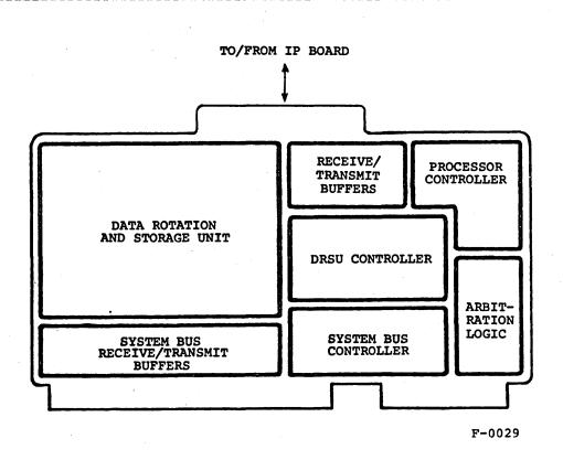
Figure 3-3. Interface Processor Link Board Block Diagram
