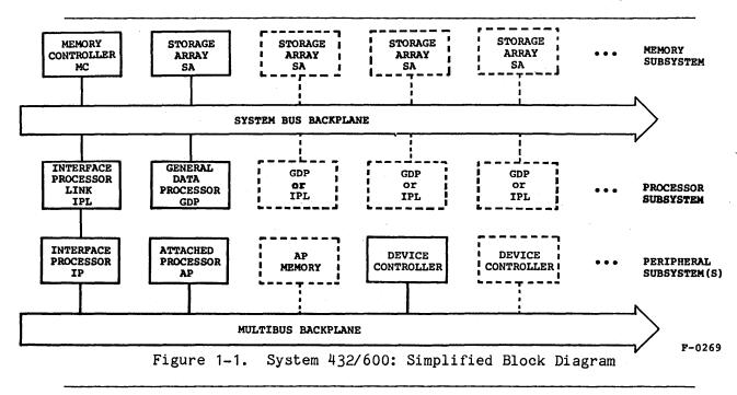
A System 432/600 comprises one Processor Subsystem, one Memory Subsystem, and one to five Peripheral Subsystems.
