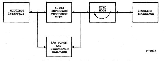
Figure 6-1. Interface Processor Board Functions
