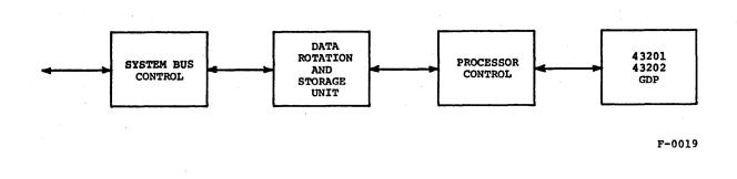
Figure 6-5. General Data Processor Board Functions
