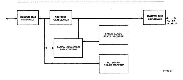
Figure 6-3. Memory Controller Board Functions
