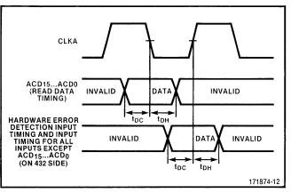
Figure 22. 43203 Input Timing Specification
