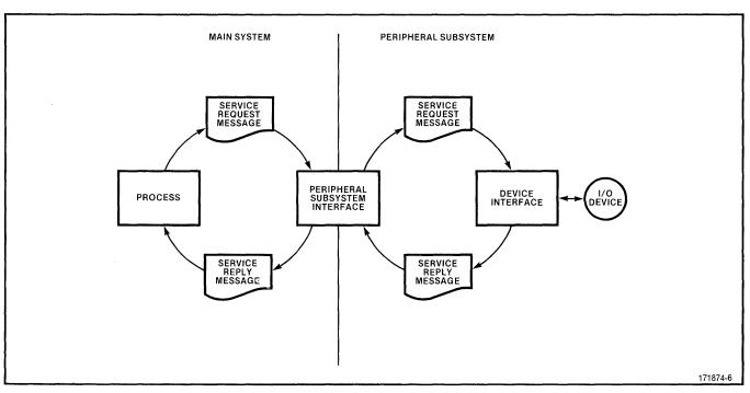
Figure 6. Peripheral Subsystem Interface
