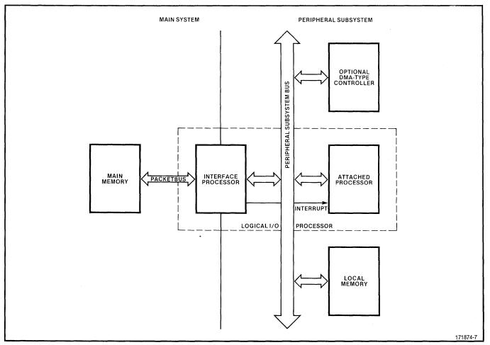
Figure 7. Peripheral Subsystem Interface Hardware
