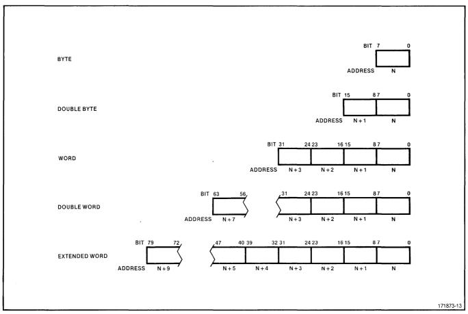
Figure 9. Basic iAPX 432 Data Lengths
