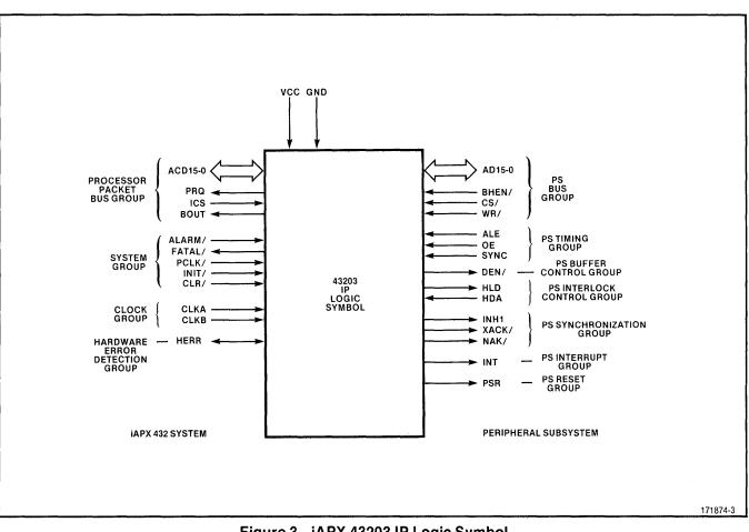
Figure 3. iAPX 43203 IP Logic Symbol
