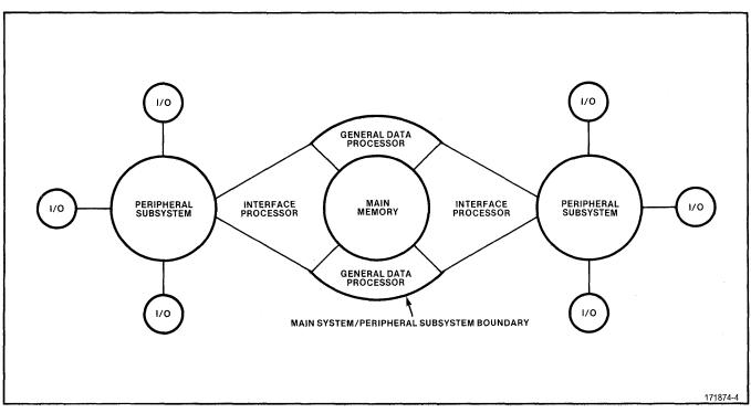
Figure 4. Main System and Peripheral Subsystem
