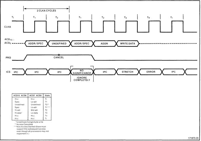
Figure 17. Minimum Faulted Access Cycle
