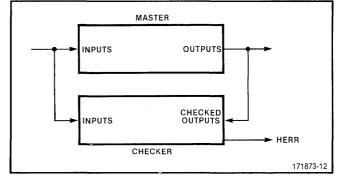
Figure 10. Hardware Error Detection
