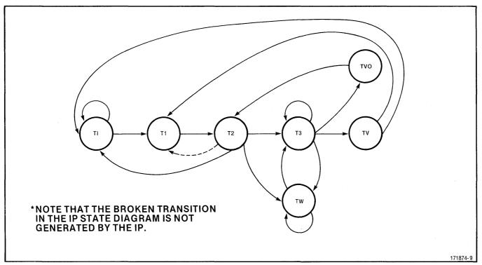
Figure 18. IP State Diagram
