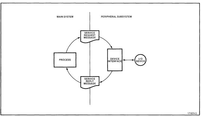
Figure 5. Basic IO Service Cycle
