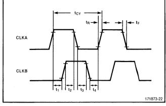
Figure 20. 43203 Clock Input Specification
