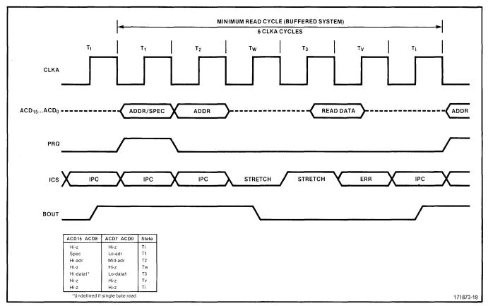
Figure 16. Minimum Read Cycle (Buffered System)
