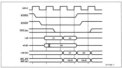
Figure 8. Two dword DMA Read Operation (with No Wait States)
