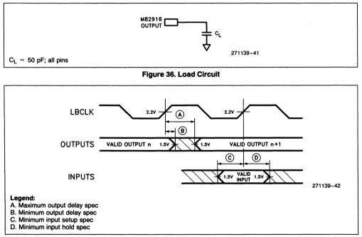
Figure 37. Drive Levels and Measurement Points for A.C. Specifications
