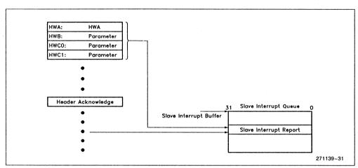
Figure 26. Parameter Write Sequence for a Direct Message
