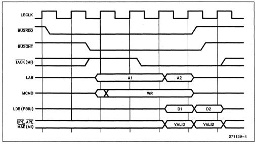
Figure 4. Local Bus Acquisition with Waits (Two dword Write)
