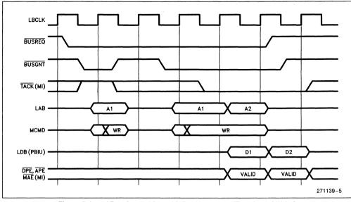
Figure 5. Local Bus Acquisition with Re-Arbitration (Two dword Write)
