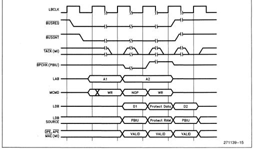
Figure 12. Block Protect Check (Optional Wait States Shown)
