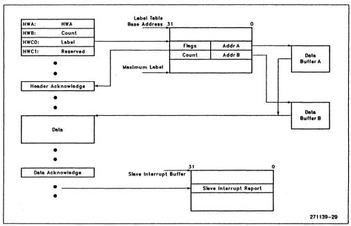
Figure 25. Block Message Read Sequence for a Label Message
