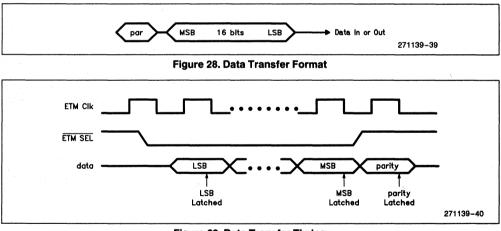
Figure 29. Data Transfer Timing
