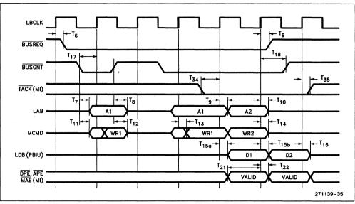
Figure 33. Local Bus Acquisition and DMA Write Timings
