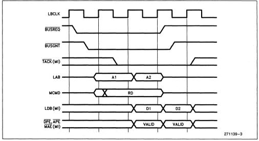
Figure 3. Local Bus Acquisition with No Waits (Two dword Read)
