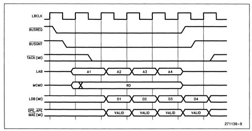
Figure 10. Four dword DMA Read Operation (with No Wait States)
