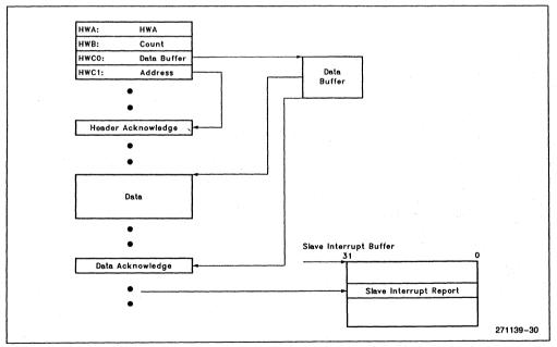
Figure 24. Block Message Read Sequence for a Direct Message
