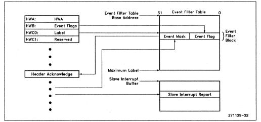
Figure 27. Parameter Write Sequence for Event Filter Message
