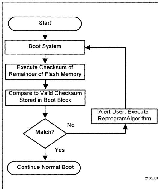
Figure 3. Checksum Validation Confirms Flash Memory Integrity
