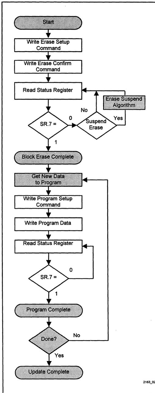
Figure 2. Simple Code/Data Block Update Algorithm Shows Shaded "Window" Opportunities for Array Reads
