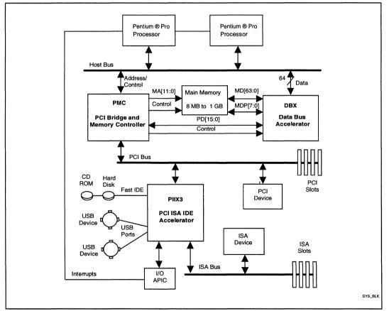
Figure 1. 440FX PCIset System Block Diagram
