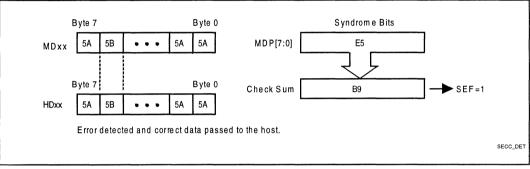
Figure 6. Single Bit Error Detection and Correction (SEC)
