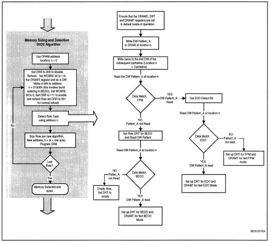
Figure 4. DRAM Auto-Detection Algorithm
