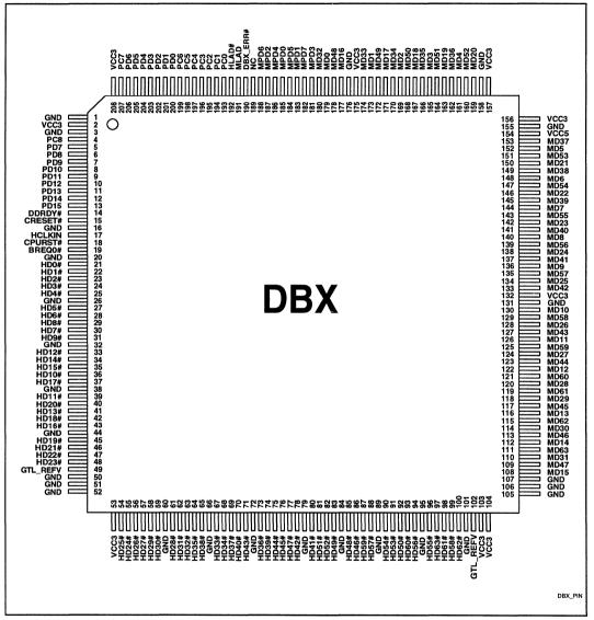
Figure 17. DBX Pinout Diagram
