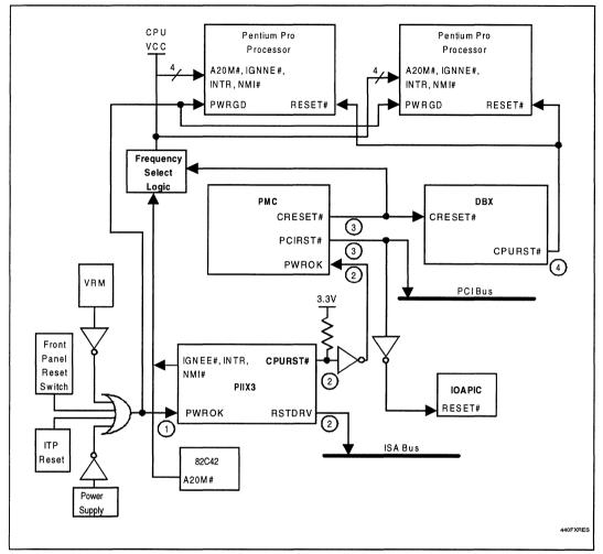
Figure 13. Reset Structure for 440FX PCIset with PIIX3
