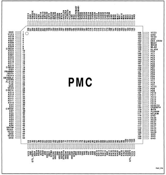
Figure 16. PMC Pinout Diagram
