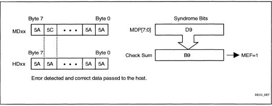
Figure 7. Multiple Bit Error Detection (DED)
