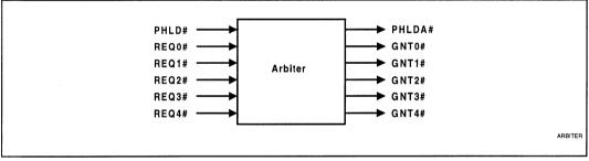
Figure 11. PCI Bus Arbiter
