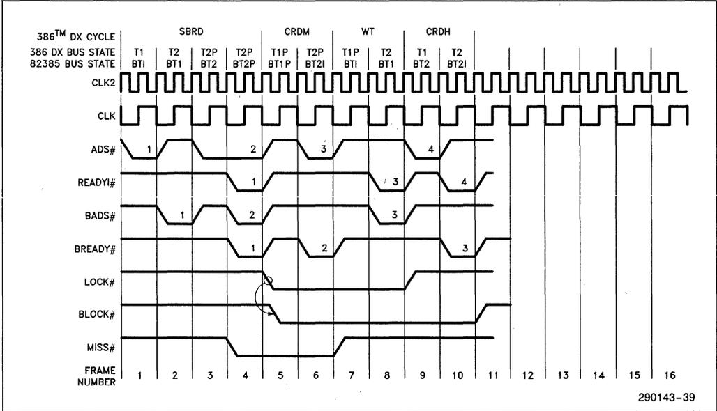
Figure 5-3K. LOCK # /BLOCK # in Non-Cacheable or Miss Cycles—(N = 1)
