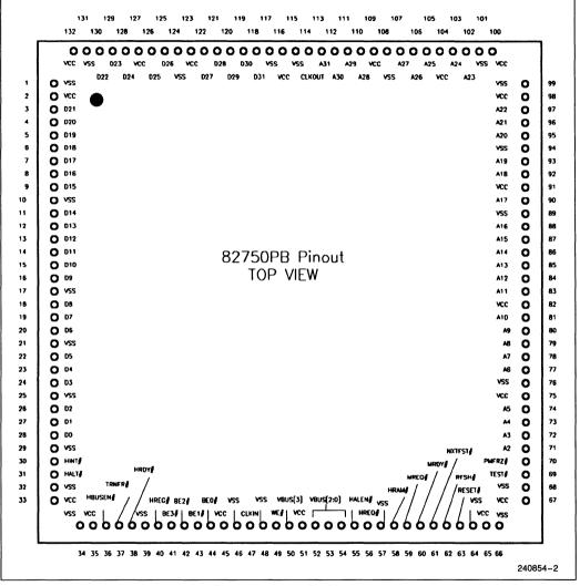
Figure 1-1. 82750PB Pinout
