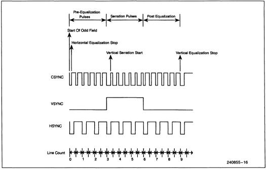
Figure 4-1. Programming the Video Sync Outputs
