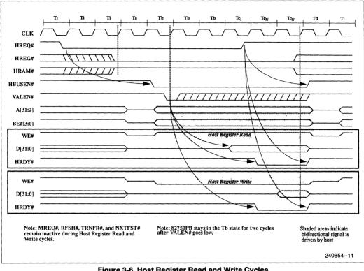
Figure 3-6. Host Register Read and Write Cycles
