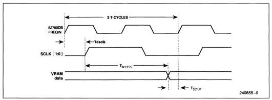
Figure 2-6. 82750DB 1/2X Shift Clock Operation
