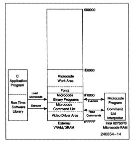
Figure 5-1. Execution of an Intel 82750PB Microcode Function
