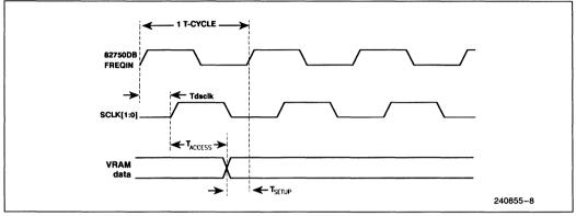
Figure 2-5. 82750DB 1X Shift Clock Operation
