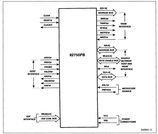
Figure 1-2. 82750PB Functional Signal Groupings
