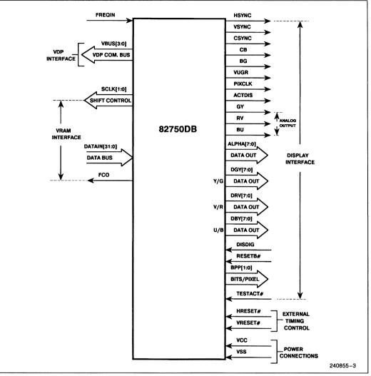
Figure 1-2. 82750DB Functional Signal Groupings
