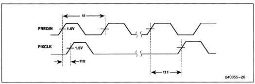
Figure 5-7. PIXCLK Waveforms
