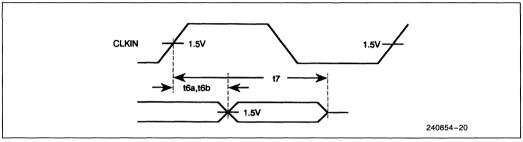
Figure 7-2. Output Waveforms
