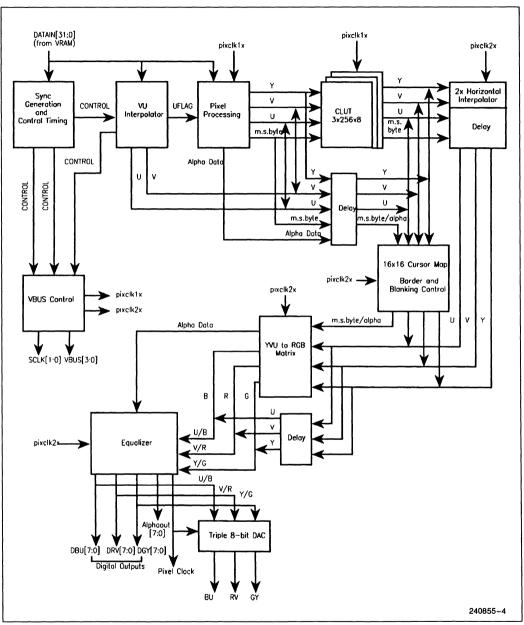
Figure 2-1. 82750DB Unit Level Diagram
