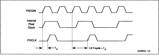
Figure 2-9 Divide by 2.5 Pixel Clock
