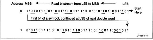
Figure 2-5. VRAM Bitstream Decoding Addresses
