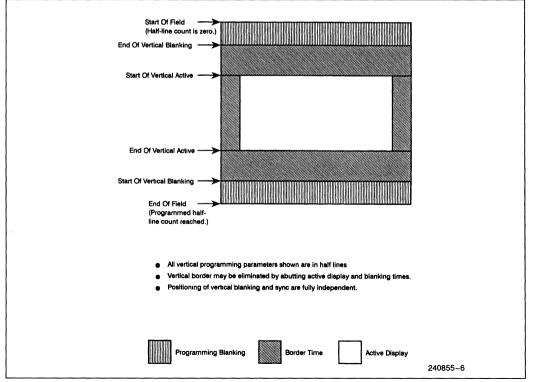
Figure 2-3. Vertical Programming Parameters
