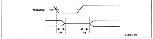
Figure 5-9. TESTACT # Float Delay
