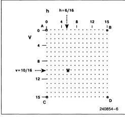
Figure 2-6. Pixel Interpolation
