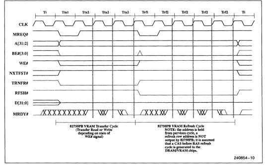
Figure 3-5. VRAM Transfer and Refresh Cycles
