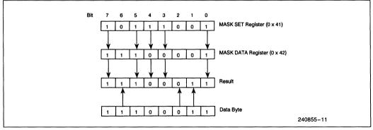
Figure 2-8. Mask Operation on CLUT Address
