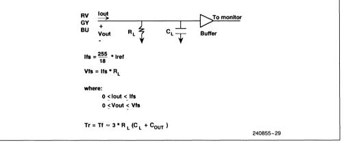
Figure 5-10. Typical Output Configuration
