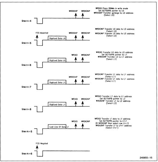
Figure 3-3. Digitizing Example with Line Replicate
