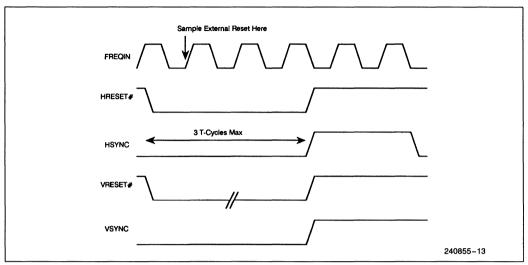
Figure 3-1. Horizontal and Vertical Reset Timing
