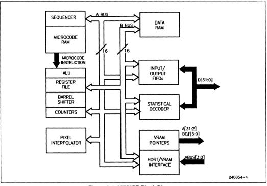
Figure 2-1. 82750PB Block Diagram
