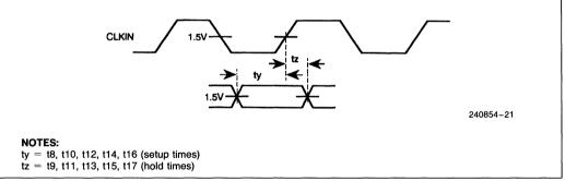
Figure 7-3. Input Waveforms
