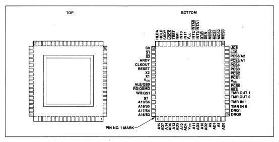
Figure 2. 80188 Pinout Diagram
