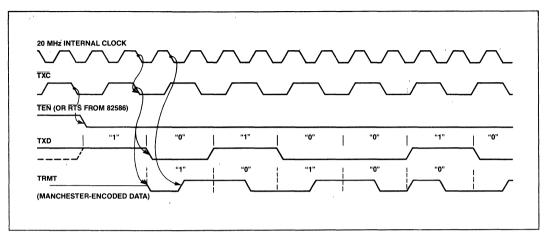
Figure 3. Start of Transmission and Manchester Encoding
