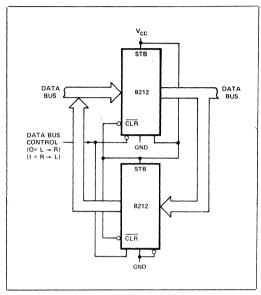
Figure 5. Bidirectional Bus Driver
