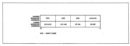
Figure 18a. DMA Memory Pointer Register Format
