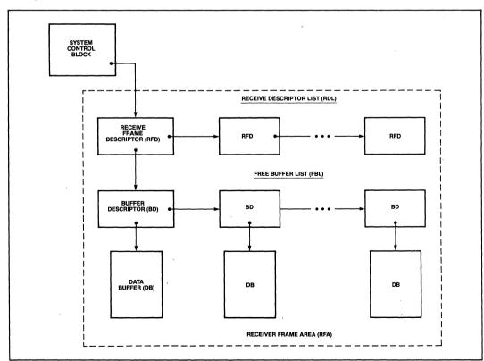
Figure 8. Receive Frame Area Diagram
