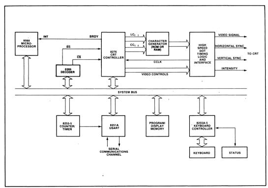
Figure 3. CRT System Block Diagram
