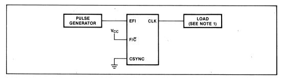
Clock High and Low Time (Using EFI)
