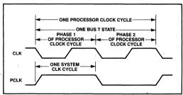
Figure 21. System and Processor Clock Relationships
