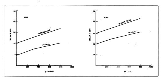
**Output Delay versus Capacitance**
