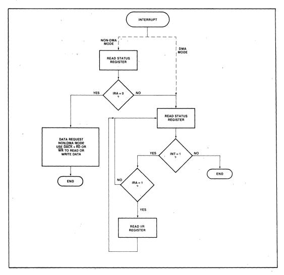
Figure 12. Result Phase Flowchart—Interrupt Results
