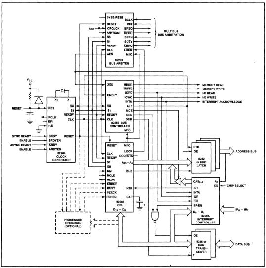
Figure 32. Multibus System Bus Interface
