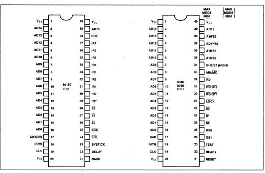
Figure 2. iAPX 86/50, 88/50 Pin Configuration
