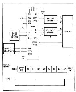
Figure 5. Serial Interface to UART (8251A)
