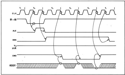
Figure 10. Idle-Write-Idle Bus Cycles with MB = 1
