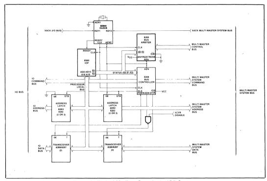
Figure 8. Typical Medium Complexity IOB System
