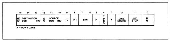
Figure 18. DMA Control Register
