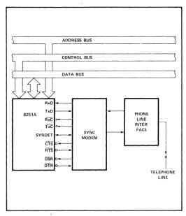
Figure 17. Synchronous Interface to Telephone Lines
