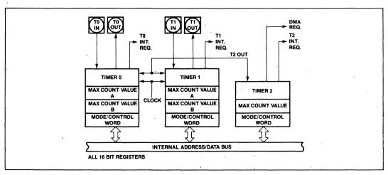
Figure 19. Timer Block Diagram
