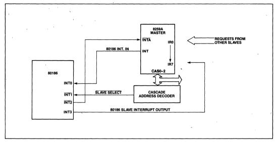
Figure 32. iRMX 86 Interrupt Controller Interconnection
