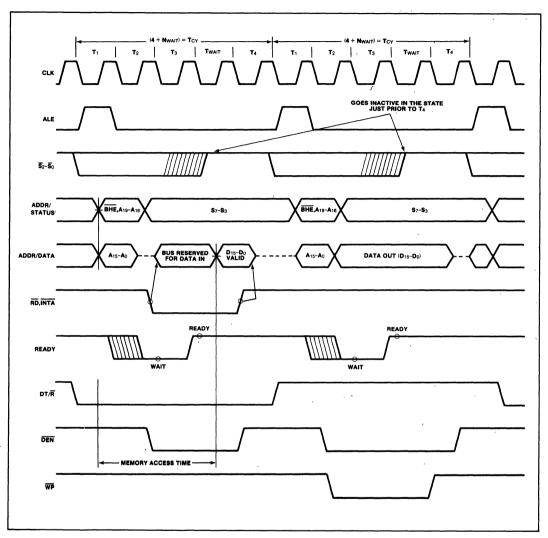
Figure 5. Basic System Timing
