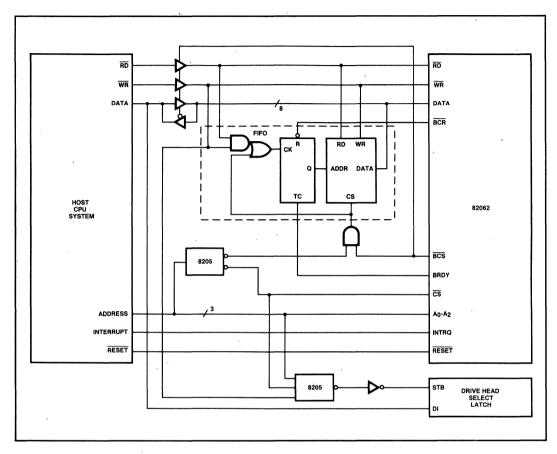
Figure 4. CPU Buffer Interface
