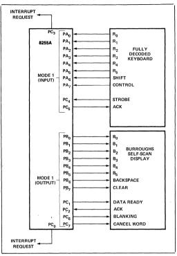
Figure 20. Keyboard and Display Interface
