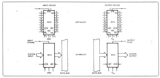
Figure 3. Basic Schematic Symbols
