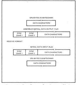
Figure 11. Data Format, Synchronous Mode
