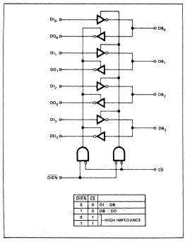
Figure 3b. 8226 Logic Diagram
