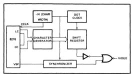
Figure 14. Typical Dot Level Block Diagram
