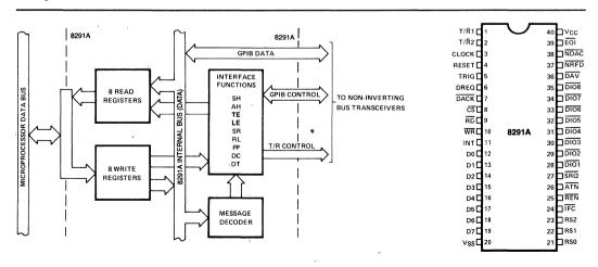
Figure 1. Block Diagram
