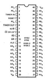
Figure 2. Pin Configuration
