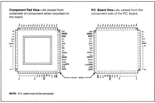
Figure 2. 80286 Pin Configuration
