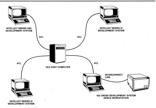
Typical Uses of Asynchronous Communication Link (ACL)
