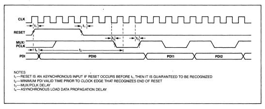
Figure 8. Timing Illustrating External Shift Register Requirements for Programming the 8207
