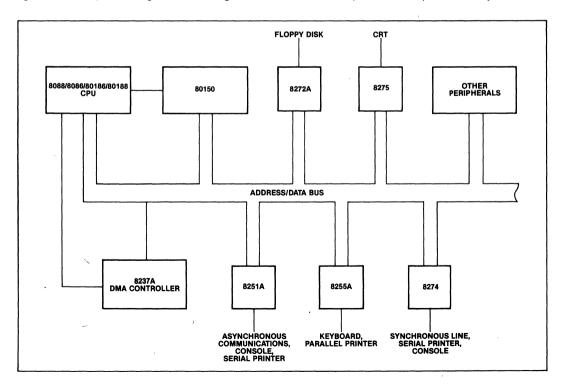
Figure 5. OEM Configurable System
