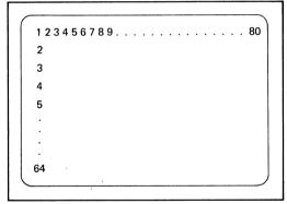
Figure 9. Blank Alternate Rows Mode
