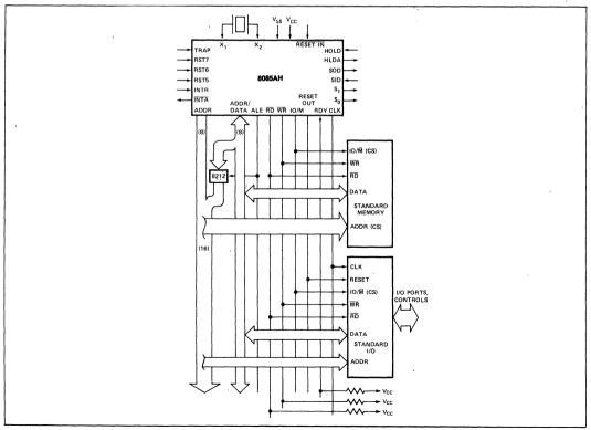
Figure 9. MCS-85® System (Using Standard Memories)
