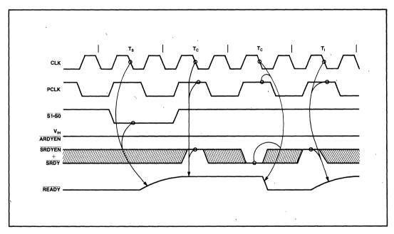
Figure 5. Synchronous Ready Operation
