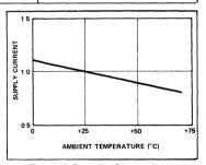
Typical Supply Current vs. Temperature, Normalized<sup>[3]</sup>
