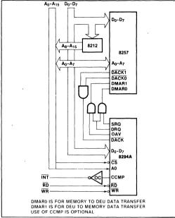
Figure 15. DMA Interface
