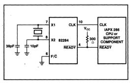
Figure 3. Recommended Crystal and Ready Connections
