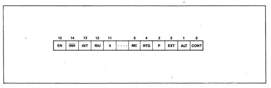
Figure 20. Timer Mode/Control Register
