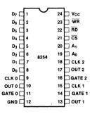
Figure 2. Pin Configuration
