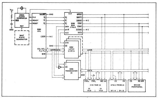
Figure 4b. Maximum Mode iAPX 86/10 Typical Configuration
