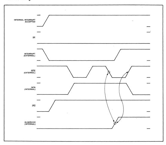
Each of the six interrupt sources has an associated In-Service latch. After priority has been resolved, the
