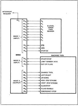
Figure 25. Machine Tool Controller Interface
