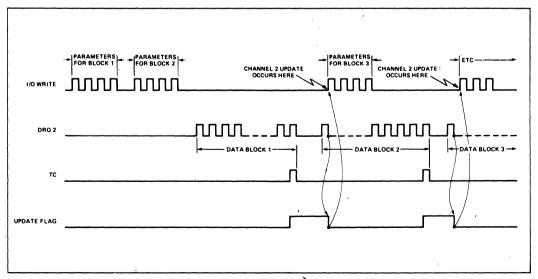
Figure 7. Autoload Timing
