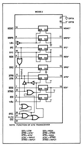
Figure 7. Talker/Listener/Controller Control Configuration
