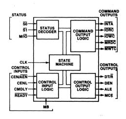
Figure 1. 82288 Block Diagram
