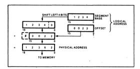
Figure 5. Two Component Address
