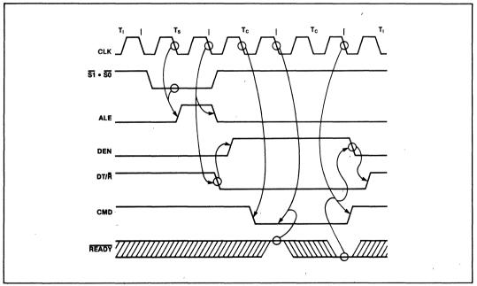
Figure 9. Idle-Read-Idle Bus Cycles with MB = 1
