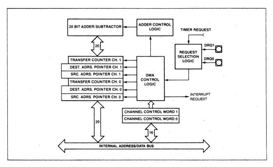
Figure 17. DMA Unit Block Diagram
