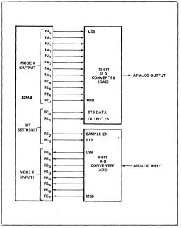
Figure 22. Digital to Analog, Analog to Digital
