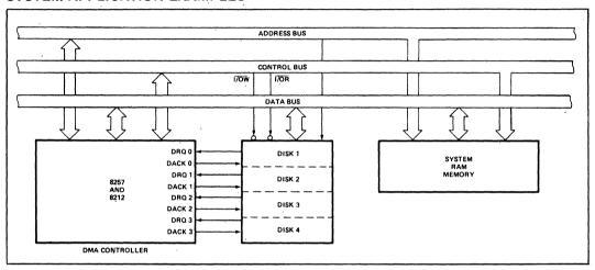
Figure 11. Floppy Disk Controller (4 Drives)
