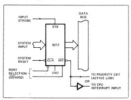
Figure 6. Interrupting Input Port
