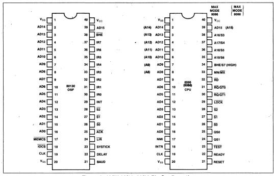
Figure 2. iAPX 86/30, 88/30 Pin Configuration
