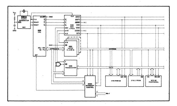
Figure 7. Fully Buffered System Using Bus Controller
