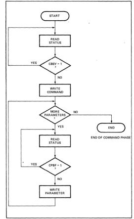
Figure 9. Command Phase Flowchart
