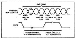
Figure 18. Frame Timing
