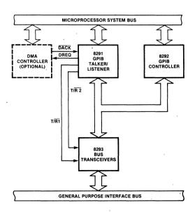
Figure 1. 8291, 8292 Block Diagram
