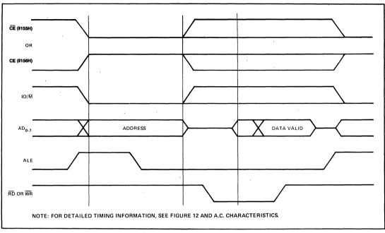
Figure 4. 8155H/8156H On-Board Memory Read/Write Cycle
