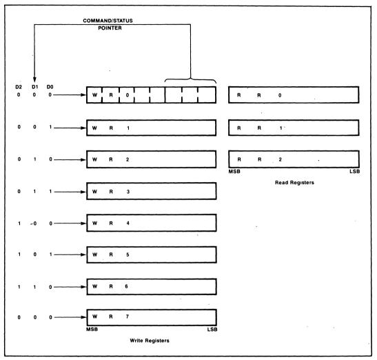
Figure 3. Command/Status Register Architecture (each serial channel)
