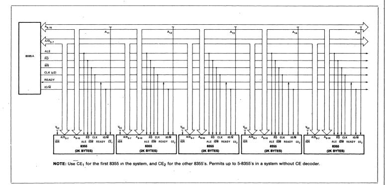
Figure 5b. 8355 in 8085A System (Standard I/O)
