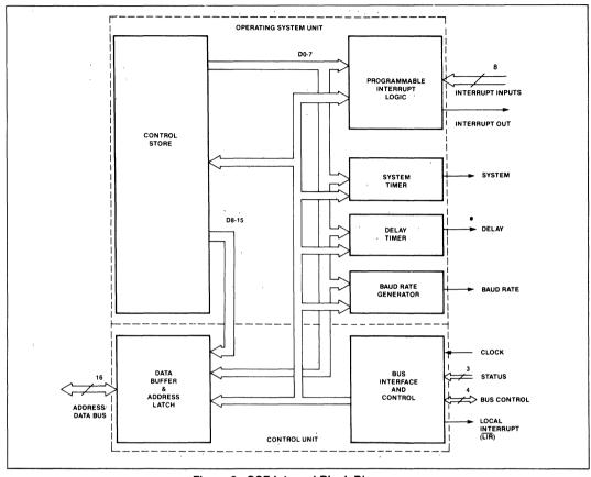
Figure 3. OSF Internal Block Diagram
