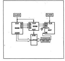
Slow-Cycle Asynchronous-Command Interface
