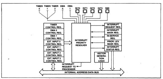
Figure 21. Interrupt Controller Block Diagram
