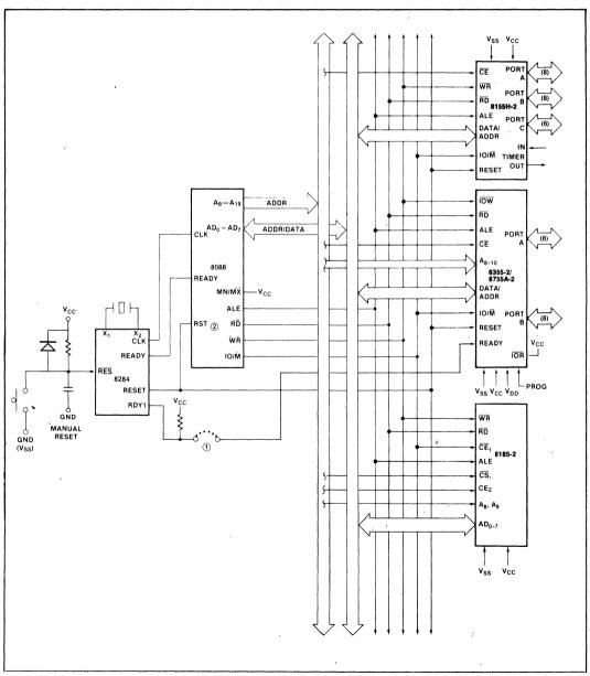
Figure 13b. 8088 Five Chip System Configuration
