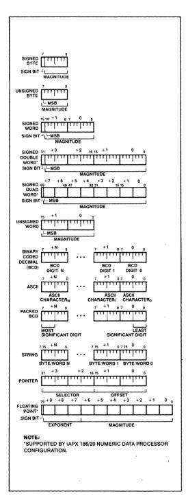
Figure 7. iAPX 186 Supported Data Types
