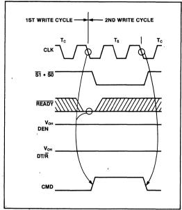
Figure 8. Write-Write Bus Cycles with MB = 0
