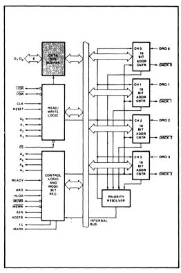
Figure 4. 8257 Block Diagram Showing Data Bus Buffer
