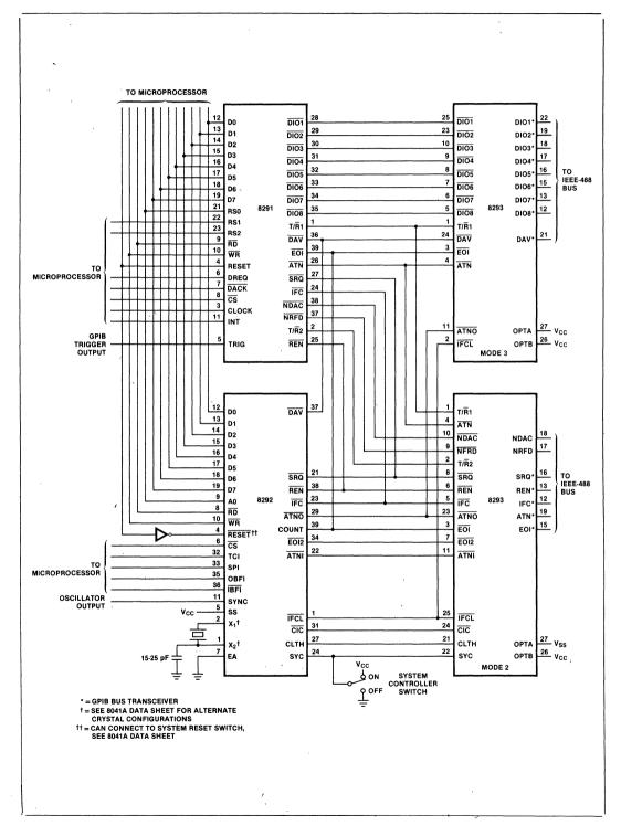
Figure 5. 8291, 8292, and 8293 System Configuration
