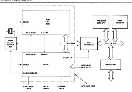
Figure 1. iAPX 86/50, 88/50 Block Diagram
