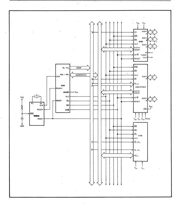
Figure 5. Multiplexed Bus Configuration
