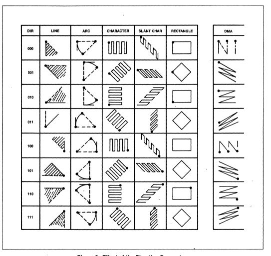
Figure 9. Effect of the Direction Parameter
