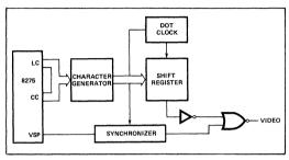
Figure 15. Typical Dot Level Block Diagram
