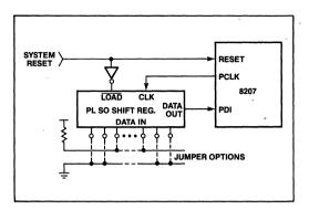
Figure 11. External Shift Register Interface
