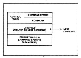
Figure 5. Action Command Format
