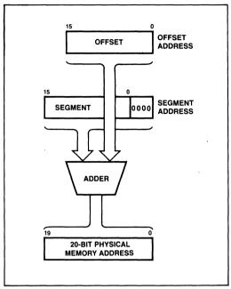
Figure 8. iAPX 86 Real Address Mode Address
