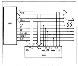
Figure 4. 8355 in 8085A System (Memory-Mapped I/O)
