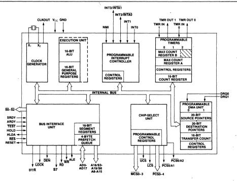
Figure 1. iAPX 188 Block Diagram
