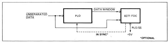
Figure 8. PLO Data Separator Block Diagram
