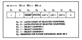
Figure 10. Read-Back Command Format
