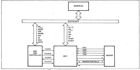
Figure 17. 8273 System Diagram
