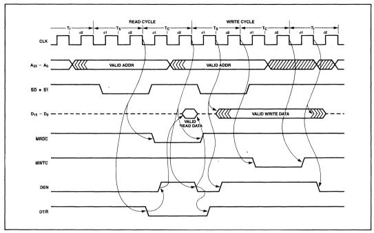
Figure 26. Back to Back Read-Write Cycles
