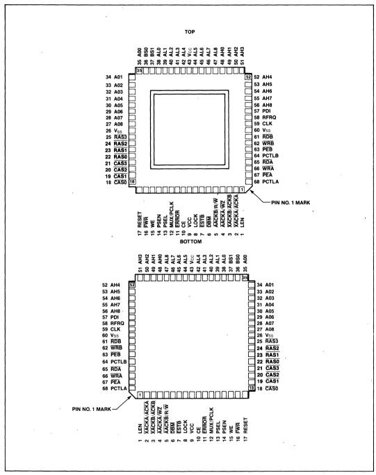
Figure 19. 8207 Pinout Diagram
