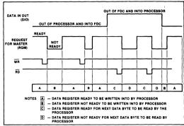
Figure 5. Status Register Timing
