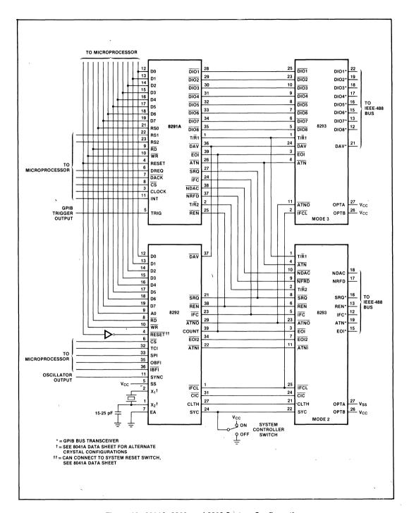
Figure 10. 8291A, 8292, and 8293 System Configuration
