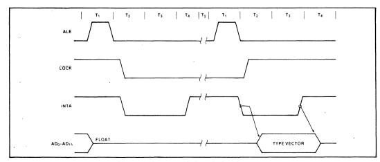
Figure 6. Interrupt Acknowledge Sequence
