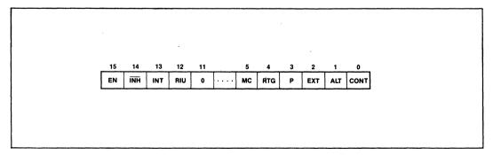
Figure 20. Timer Mode/Control Register
