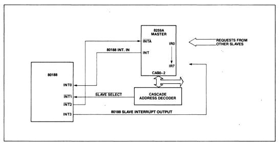
Figure 32. iRMX 86 Interrupt Controller Interconnection
