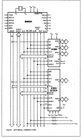
Figure 7. 8085AH Minimum System (Standard I/O Technique)
