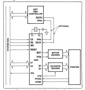
Figure 4. Parallel System Interface
