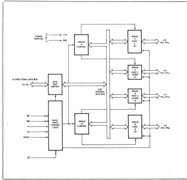
Figure 4. 8225A Block Diagram Showing Group A and Group B Control Functions
