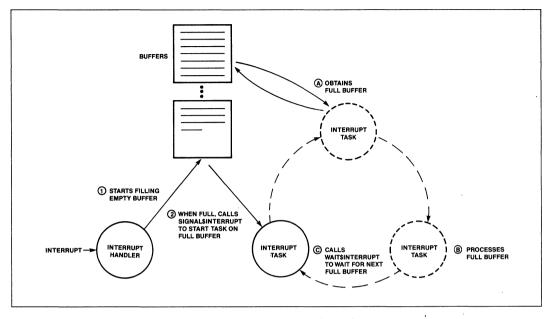
Figure 7. Multiple Buffer Example
