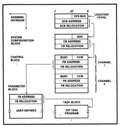
Figure 5. Communication Data Structure Hierarchy
