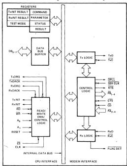
Figure 4. 8273 Block Diagram Showing CPU Interface Functions
