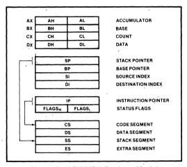
Figure 7. iAPX 86/10 Register Model
