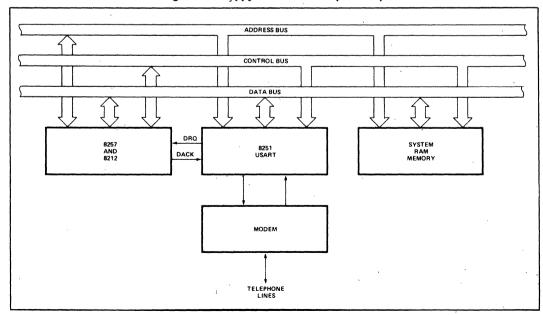
Figure 12. High-Speed Communication Controller
