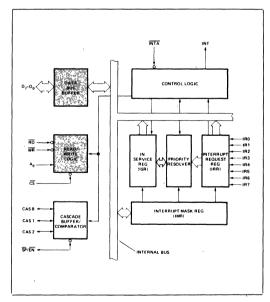
Figure 4b. 8259A Block Diagram
