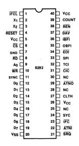
Figure 2. Pin Configuration
