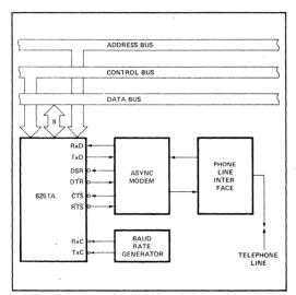
Figure 16. Asynchronous Interface to Telephone Lines
