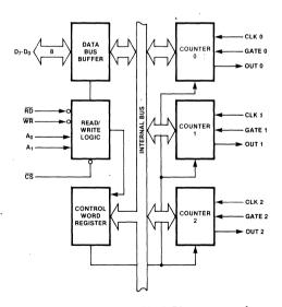
Figure 1. 8254 Block Diagram
