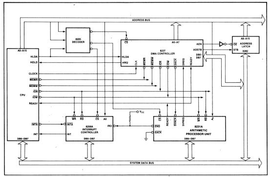
Figure 4. High Performance Configuration Example
