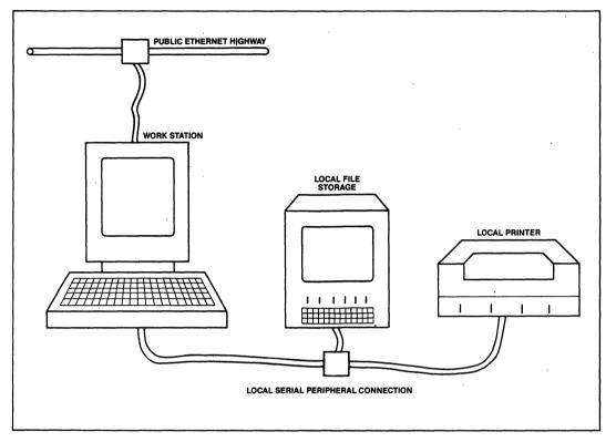
Figure 14. Local Peripheral Interconnection
