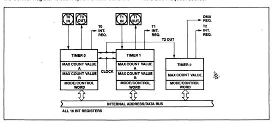
Figure 19. Timer Block Diagram
