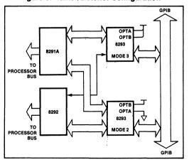
Figure 4. Talker/Listener/Controller Configuration
