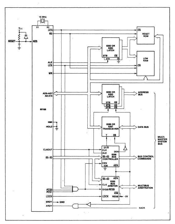
Figure 40. Typical iAPX 188 Multi-Master Bus Interface
