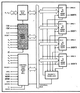
Figure 5. 8257 Block Diagram Showing Read/Write Logic Function
