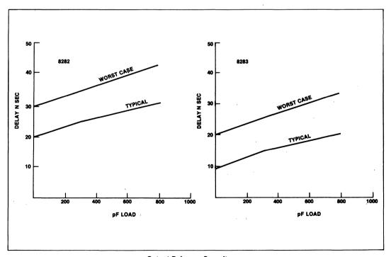
**Output Delay vs. Capacitance**
