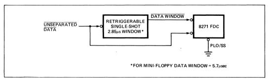
Figure 6. Single-Shot Data Separator Block Diagram
