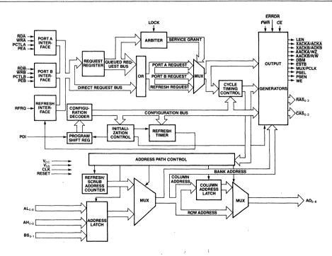
Figure 1. 8207 Block Diagram
