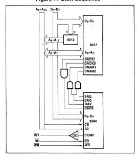
Figure 8. DMA Interface
