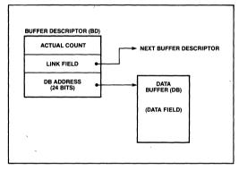
Figure 6. Transmit Data Buffer
