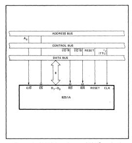
Figure 6. 8251A Interface to 8080 Standard System Bus
