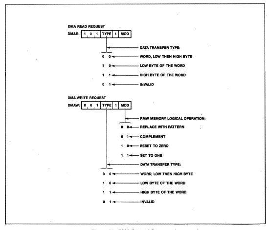
Figure 31. DMA Control Commands
