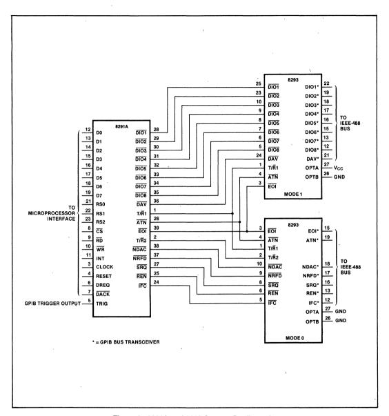
Figure 9. 8291A and 8293 System Configuration
