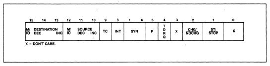
Figure 18. DMA Control Register
