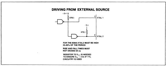
Figure 18. Recommended Connection for External Clock Signal
