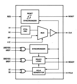
Figure 1. 82284 Block Diagram
