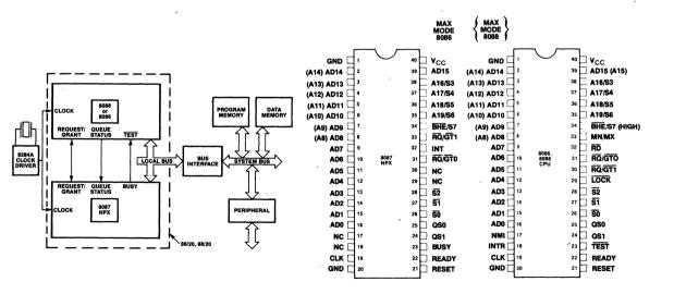
Figure 1. iAPX 86/20, 88/20 Block Diagram
