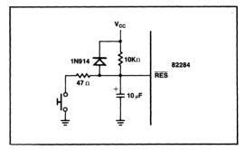
Figure 4. Typical RC RESET Timing Circuit
