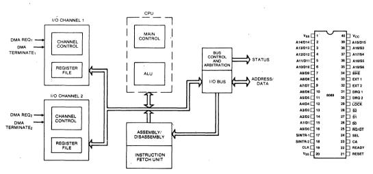
Figure 1. 8089 I/O Processor Block Diagram
