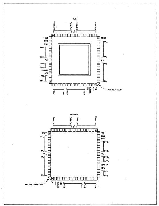
Figure 7. 8206 Pinout Diagram
