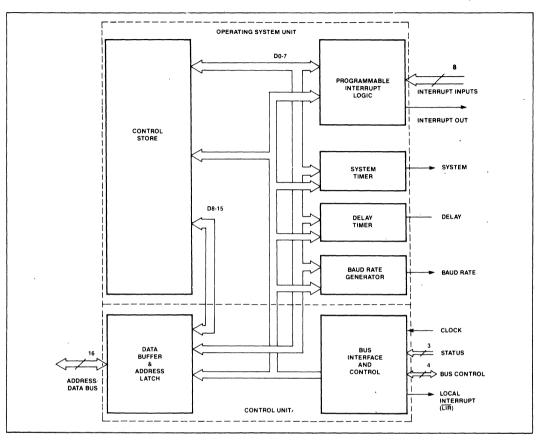
Figure 3, 80150 Internal Block Diagram
