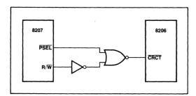
Figure 6. Interface to 8206 CRCT Input When Port
