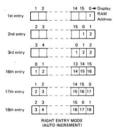
Note that now the display position and register address do not correspond. Consequently, entering a character to an arbitrary position in the Auto Increment mode may have unexpected results Entry starting at Display RAM address 0 with sequential entry is recommended.
