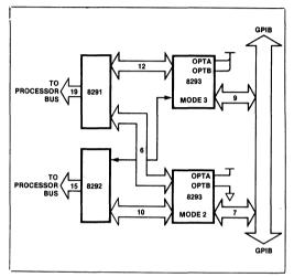
Figure 3. Talker/Listener/Controller Configuration
