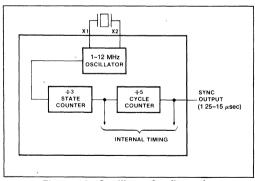
Figure 16. Oscillator Configuration
