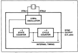
Figure 7. Oscillator Configuration
