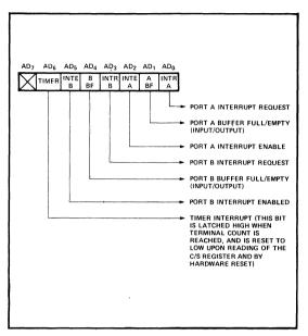
Figure 6. Status Register Bit Assignment
