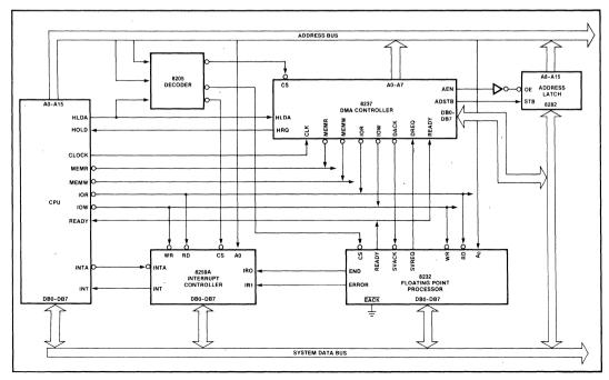
Figure 4. High Performance Configuration Example
