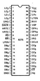
Figure 2. Pin Configuration
