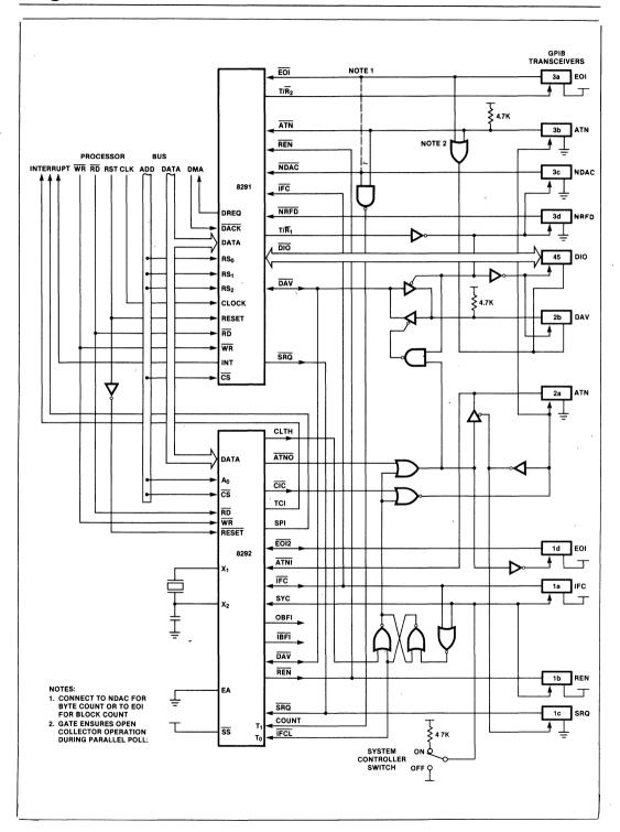
Figure 4. 8291 and 8292 System Configuration
