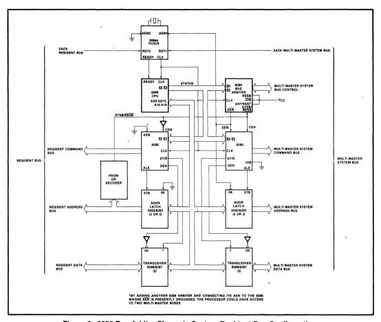
Figure 9. 8289 Bus Arbiter Shown in System-Resident Bus Configuration
