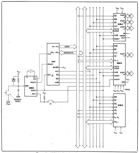
Figure 5a. iAPX 88 Five Chip System Configuration
