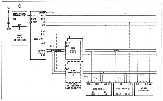
Figure 4a. Minimum Mode iAPX 86/10 Typical Configuration
