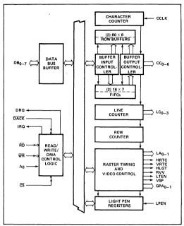
Figure 3. 8275 Block Diagram Showing Counter and Register Functions
