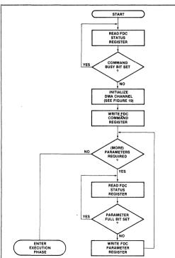
Figure 16. Passing the Command and Parameters to the 8271
