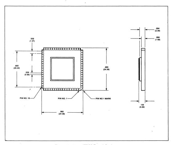
Figure 41. 80188 JEDEC Type A Package
