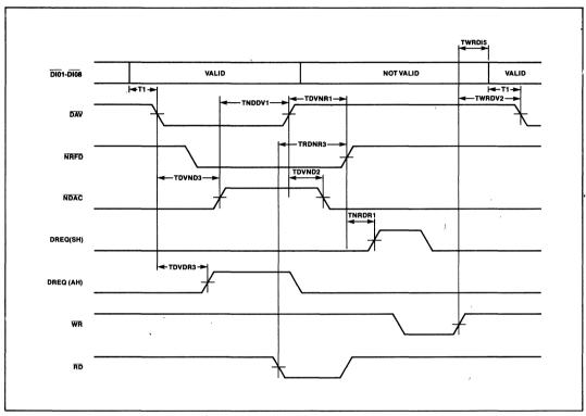
Figure C-1. 3-Wire Handshake Timing at 8291A
