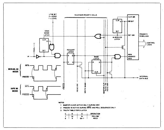
Figure 9. Priority Cell—Simplified Logic Diagram
