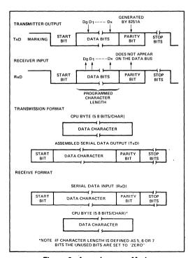
Figure 9. Asynchronous Mode
