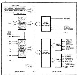
Figure 3. 8271 Block Diagram Showing CPU Interface Functions
