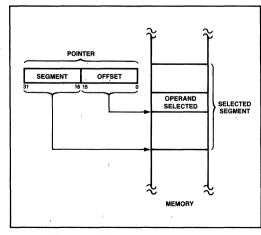
Figure 5. Two Component Address
