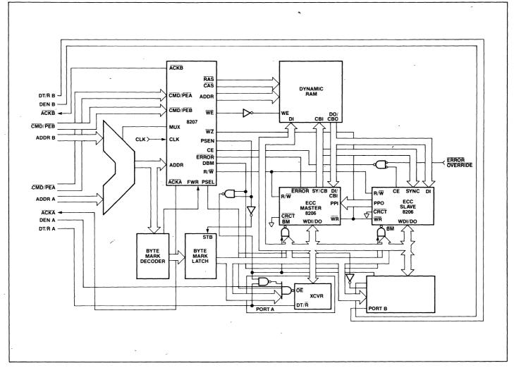
Figure 5. Two-Port ECC Implementation Using the 8207 and the 8206
