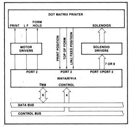
Figure 4. 8041A Matrix Printer Interface
