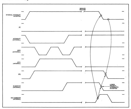
Lower priority interrupts are not accepted internally while the In-Service latch is set. However, higher priority interrupts are accepted internally and a new external INT request is generated. If the CPU responds with a new INTA sequence, the MPSC will respond as before, suspending the lower priority interrupt.
