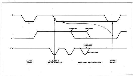
Figure 10. IR Triggering Timing Requirements
