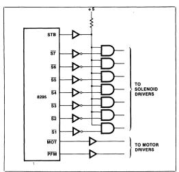
Figure 6. 8295 To Printer Solenoid Interface
