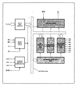
Figure 4a. 8259A Block Diagram
