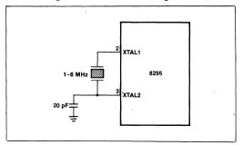
Figure 8. Recommended Crystal Connection
