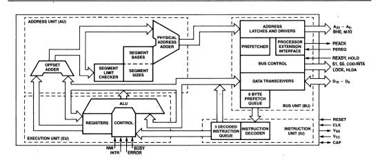
Figure 1. 80286 Internal Block Diagram
