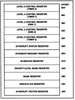
Figure 33. Interrupt Controller Registers (iRMX 86 Mode)
