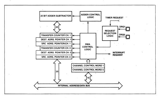
Figure 17. DMA Unit Block Diagram
