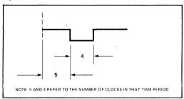
Figure 12. Asymmetrical Square-Wave Output Resulting from Count of 9
