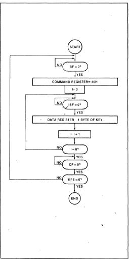
Figure 4. Flowchart for Entering a New Key
