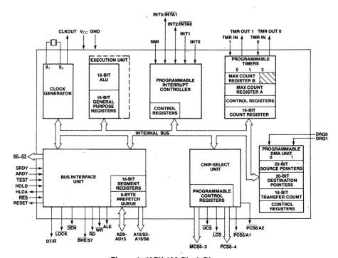
Figure 1. iAPX 186 Block Diagram
