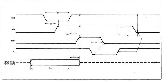
Figure 9. MODE 1 (Strobed Input)
