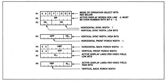
Figure 15. Optional Reset Parameters
