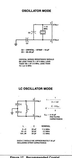
Figure 17. Recommended Crystal and L-C Connections
