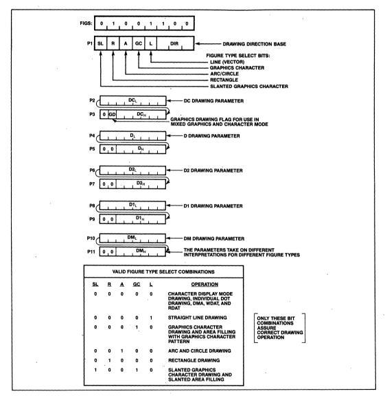
Figure 25. Figure Drawing Parameters Specify
