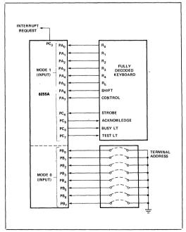
Figure 21. Keyboard and Terminal Address Interface
