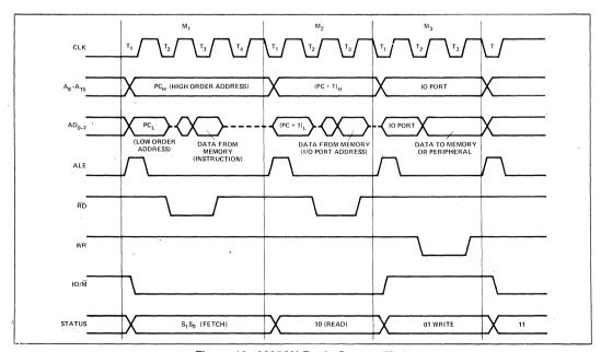
Figure 10. 8085AH Basic System Timing
