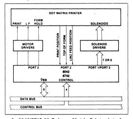
Figure 6. 8042/8742 80-Column Matrix Printer Interface
