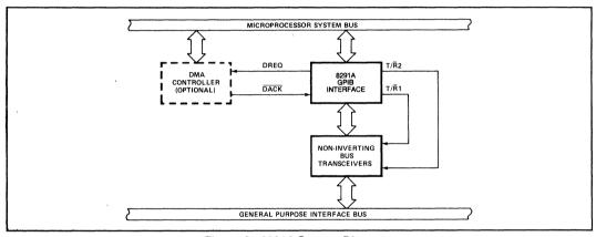
Figure 3. 8291A System Diagram
