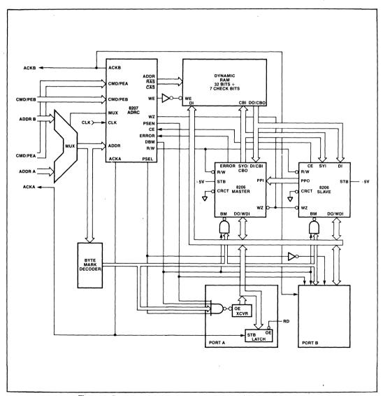
Figure 5. Dual Port RAM Subsystem with 8206/8207 (32-bit bus)
