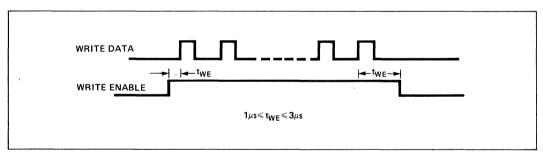
Figure 10. Write Enable Timing
