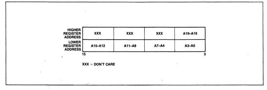
Figure 18a. DMA Memory Pointer Register Format
