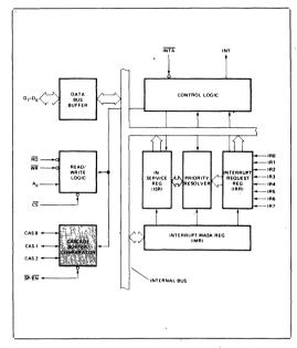
Figure 4c. 8259A Block Diagram
