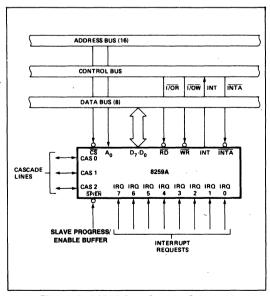
Figure 5. 8259A Interface to Standard System Bus
