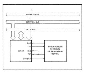
Figure 15. Synchronous Interface to Terminal or Peripheral Device
