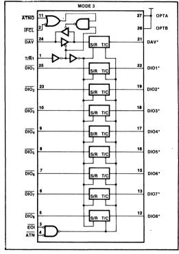
Figure 8. Talker/Listener/Controller Data Configuration
