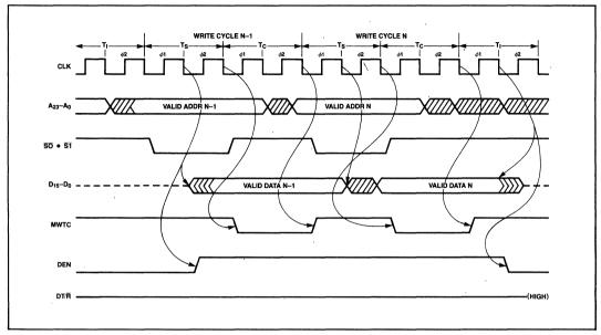
Figure 28. Back to Back Write-Write Cycles
