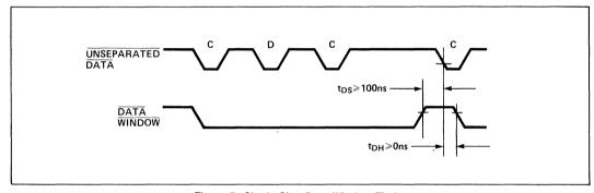
Figure 7. Single-Shot Data Window Timing
