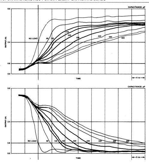
Use the Test Load as the base capacitance for estimating timing shifts for system critical timing parameters.
