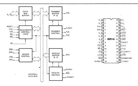
Figure 1. Block Diagram
