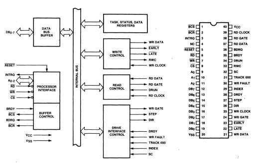
Figure 1. 82062 Internal Block Diagram
