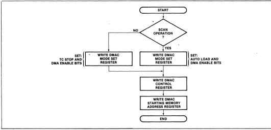
Figure 24. User DMA Channel Initialization Flowchart
