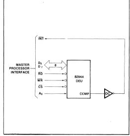
Figure 13. Single Interrupt Interface
