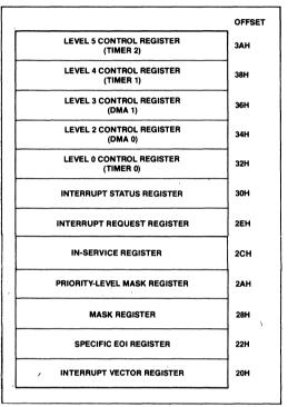
Figure 33. Interrupt Controller Registers (iRMX 86 Mode)
