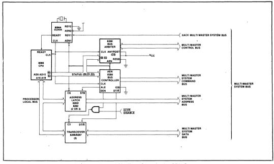
Figure 7. Typical Medium Complexity CPU System
