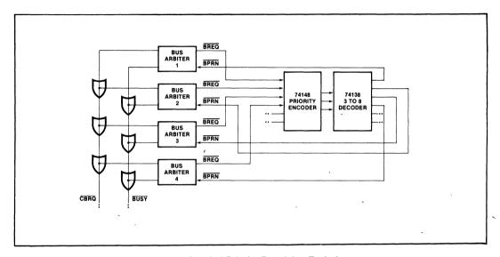
Figure 4. Parallel Priority Resolving Technique
