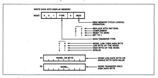
Figure 23. Drawing Control Commands
