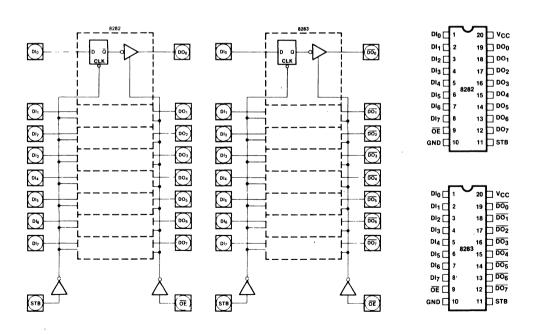
Figure 1. Logic Diagrams
