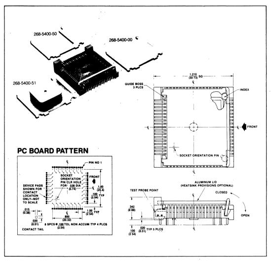
Figure 42. Textool 68 Lead Chip Carrier Socket
