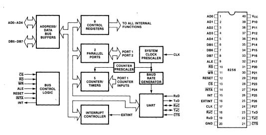
Figure 1. MUART Block Diagram
