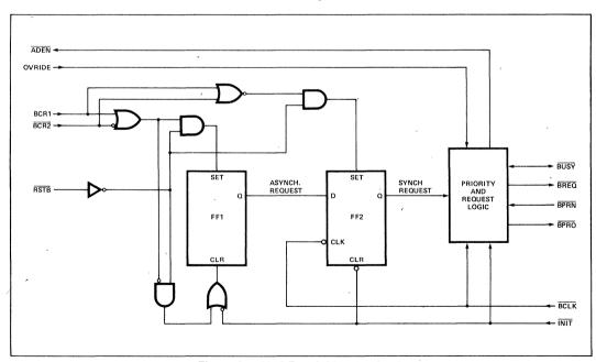
Figure 3a. 8218 Bus Arbitration Logic
