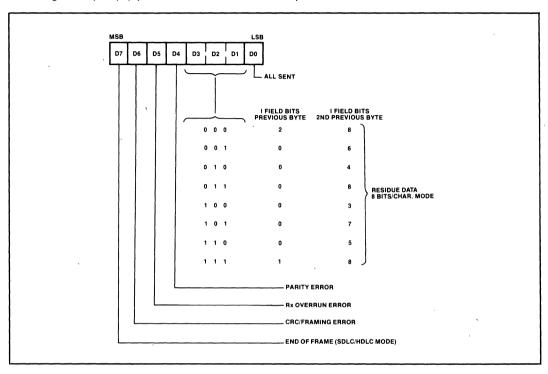
D5 Receive Overrun Error—this bit indicates that the receive FIFO has been overloaded by the receiver. The last character in the FIFO is overwritten and flagged with this error. Once the overwritten character is read, this error condition is latched until reset by the Error Reset command. If the MPSC is in the status affects vector mode, the overrun causes a special Receive Condition Vector.
