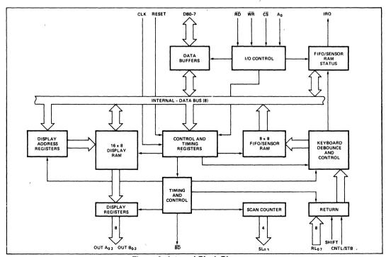
Figure 3. Internal Block Diagram
