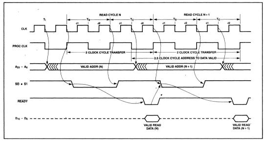
Figure 23. Basic Bus Cycle
