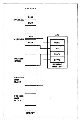
Figure 6. Segmented Memory Helps Structure Software
