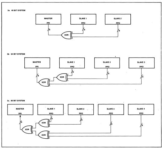
Figure 3. External Logic For Multi-Chip Systems
