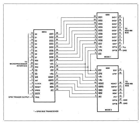
Figure 6. 8291A and 8293 System Configuration
