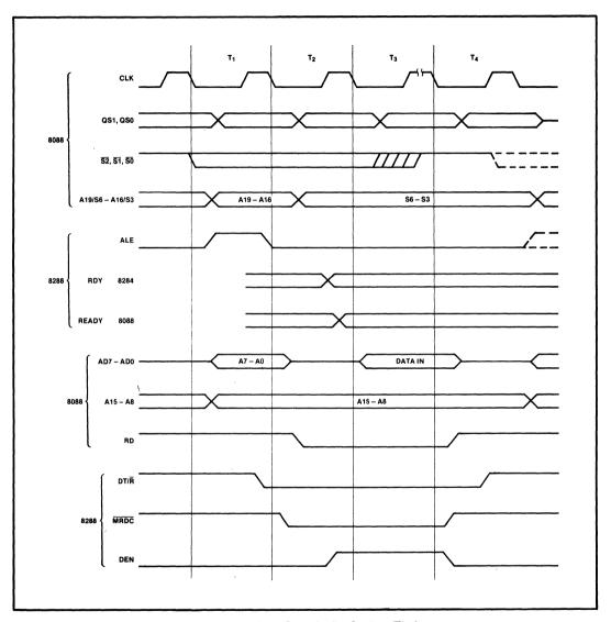
Figure 10. Medium Complexity System Timing
