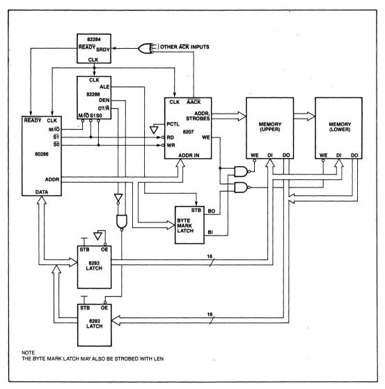
Figure 17. 80286 Hook-up to 8207 Non-ECC Synchronous System-Single Port.
