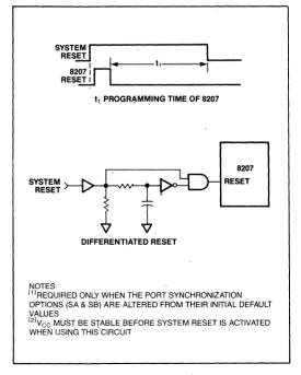
Figure 7. 8207 Differentiated Reset Circuit
