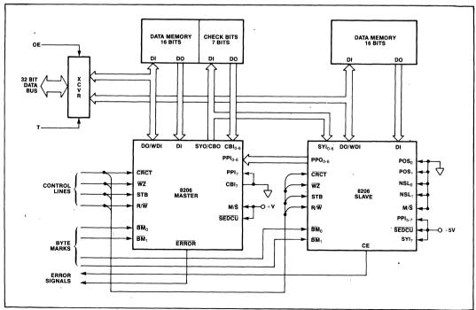
Figure 4. 32-Bit 8206 System Interface
