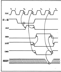
Figure 6. Idle-Read-Idle Bus Cycles with MB = 0
