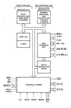
Figure 1. iAPX 86/10 CPU Block Diagram
