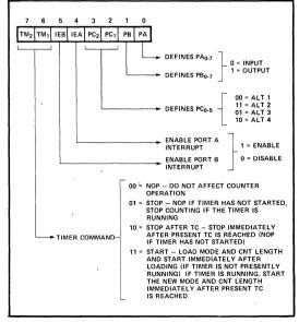
Figure 5. Command Register Bit Assignment
