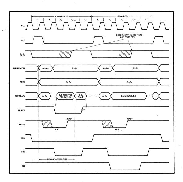
Figure 8. Basic System Timing
