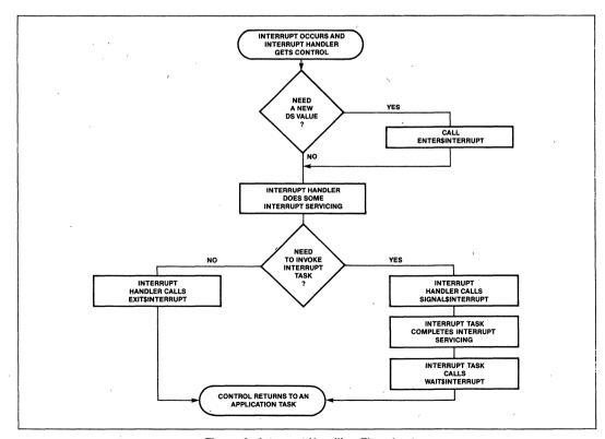
Figure 6. Interrupt Handling Flowchart
