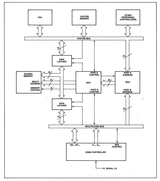
Figure 12. Dual-Port RAM-Based System
