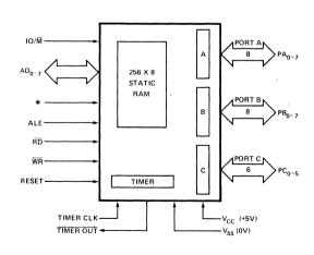
Figure 1. Block Diagram
