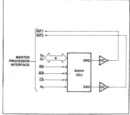
Figure 14. Dual Interrupt Interface
