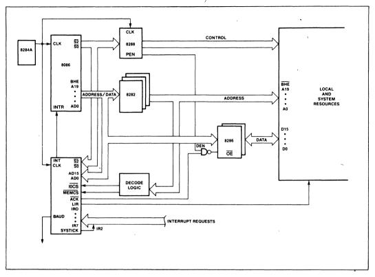
Figure 8. Typical OSP Configuration
