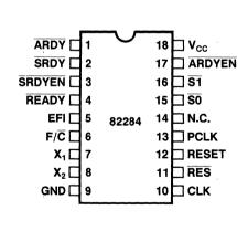
Figure 2. 82284 Pin Configuration
