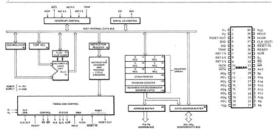
Figure 1. 8085AH CPU Functional Block Diagram
