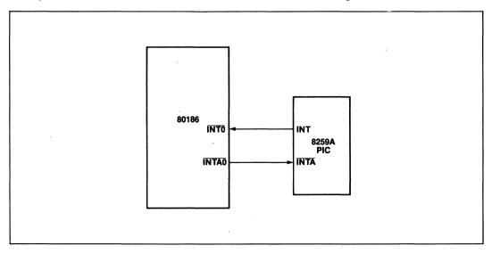
Figure 22. Cascade Mode Interrupt Connection
