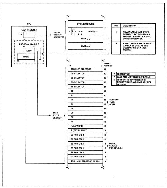
Figure 20. Task State Segment and TSS Registers
