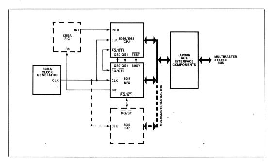
Figure 4. NDP System Configuration
