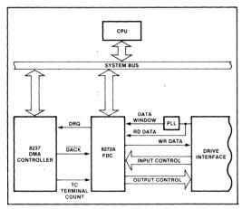
Figure 3. 8272A System Block Diagram
