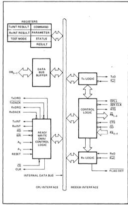
Figure 5. 8273 Block Diagram Showing Control Logic Functions
