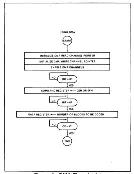
Figure 9. DMA Flowchart
