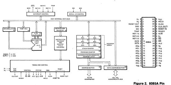
Figure 1. 8085A CPU Functional Block Diagram
