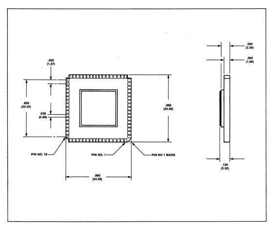
Figure 41. 80186 JEDEC Type A Package
