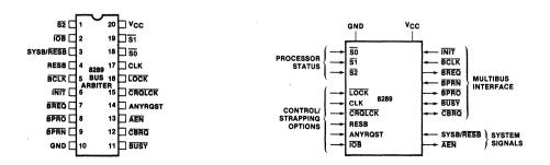
Figure 2. Pin Diagram
