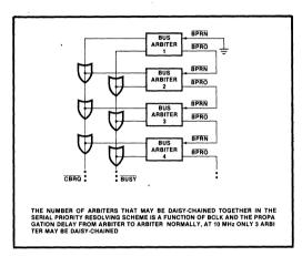
Figure 6. Serial Priority Resolving
