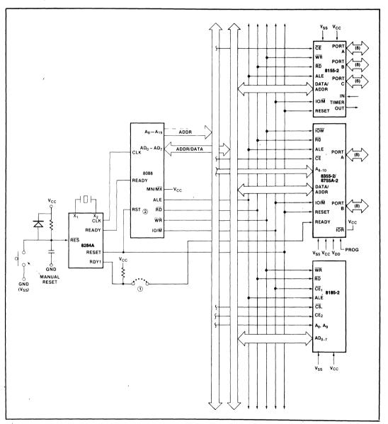
Figure 4. iAPX 88 Five Chip System Configuration
