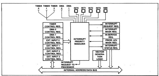
Figure 21. Interrupt Controller Block Diagram
