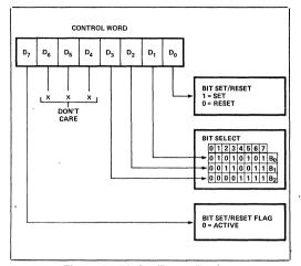
Figure 7. Bit Set/Reset Format
