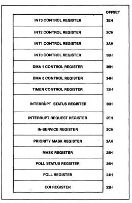
Figure 23. Interrupt Controller Registers (Non-iRMX 86 Mode)
