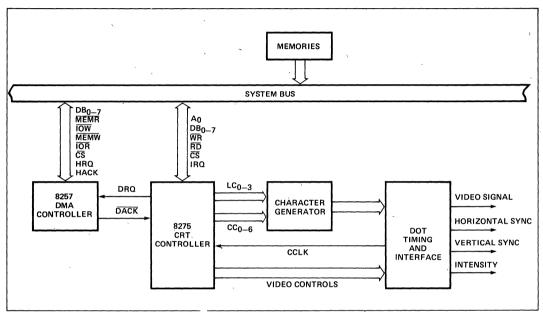
Figure 4. 8275 Systems Block Diagram Showing Systems Operation
