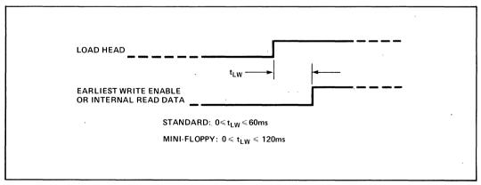
Figure 14. Head Load to Read/Write Timing
