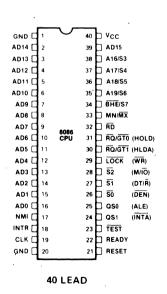
Figure 2. iAPX 86/10 Pin Configuration
