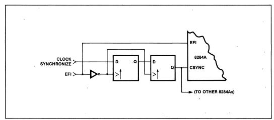
Figure 3. CSYNC Synchronization
