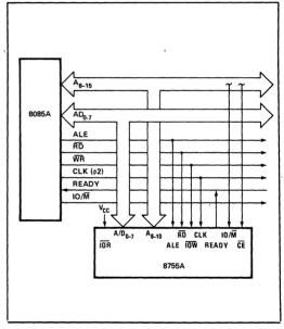
Figure 3. 8755A in 8085A System (Memory-Mapped I/O)
