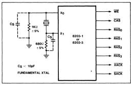
Figure 3. Crystal Operation for the 8203-1 and 8203-3
