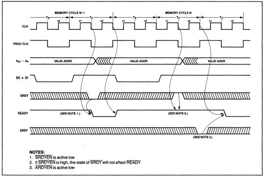
Figure 25. Synchronous and Asynchronous Ready
