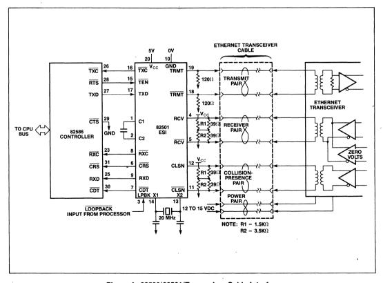
Figure 4. 82586/82501/Transceiver Cable Interface
