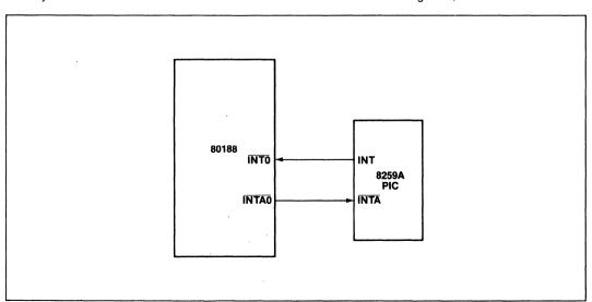
Figure 22. Cascade Mode Interrupt Connection
