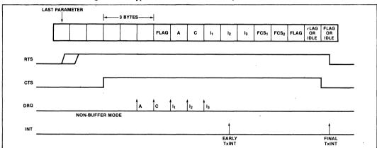
Figure 16b. Typical Frame Transmission, Non-Buffered Mode
