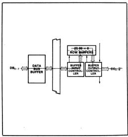
Figure 6. Second Row Buffer Filled, First Row Displayed
