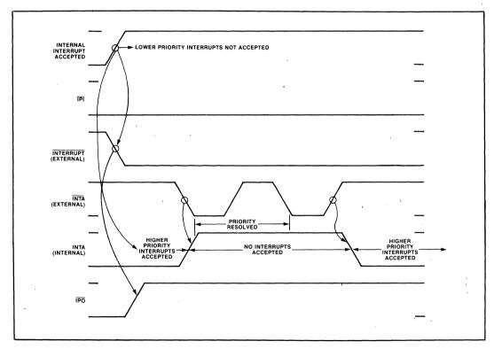
The MPSC's internal INTA is set on the leading (falling) edge of the first external INTA pulse, and reset on the trailing (rising) edge of the second external INTA pulse. After an interrupt is accepted internally,
