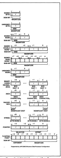
Figure 7. iAPX 286 Supported Data Types
