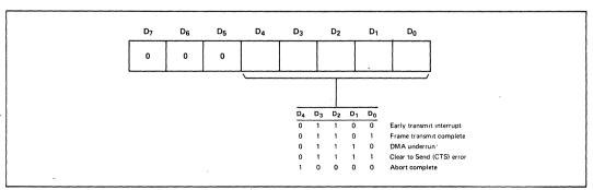
Figure 11. Tx Interrupt Result Byte Format
