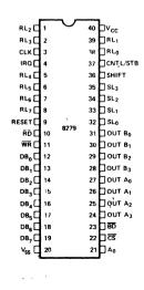
Figure 2. Pin Configuration
