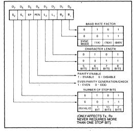
Figure 8. Mode Instruction Format, Asynchronous Mode
