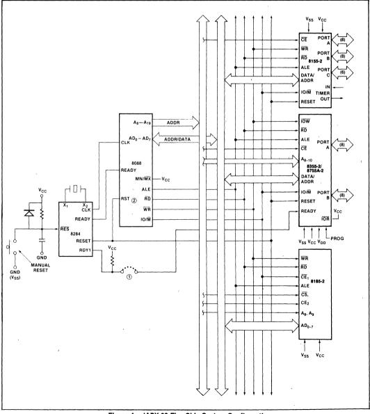
Figure 4a. iAPX 88 Five Chip System Configuration
