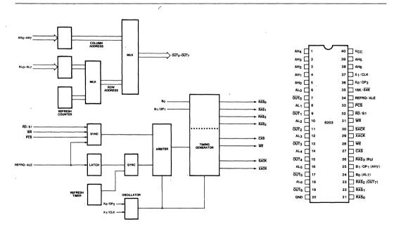
Figure 1. 8203 Block Diagram
