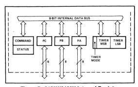
Figure 3. 8155H/8156H Internal Registers
