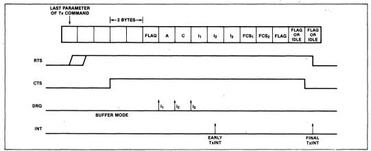
Figure 16a. Typical Frame Transmission, Buffered Mode
