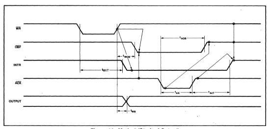
Figure 11. Mode 1 (Strobed Output)
