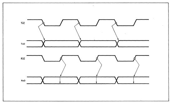
Figure 6. Transmit/Receive Timing
