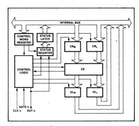
Figure 5. Internal Block Diagram of a Counter
