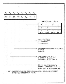
Figure 10. Mode Instruction Format, Synchronous Mode
