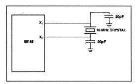
Figure 8. Recommended iAPX 186 Crystal Configuration
