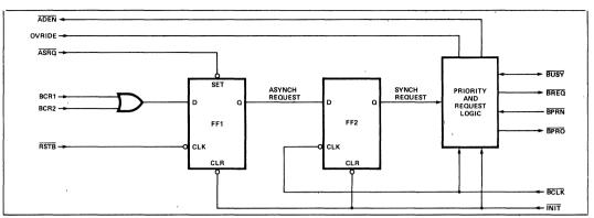
Figure 3b. 8219 Bus Arbitration Logic
