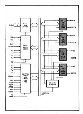
Figure 3. 8257 Block Diagram Showing DMA Channels
