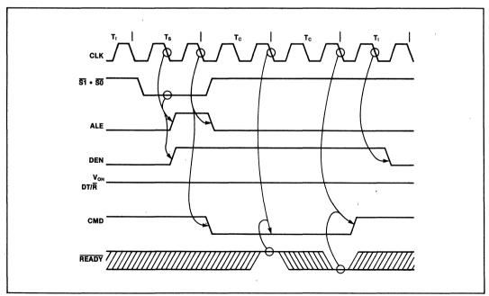
Figure 7. Idle-Write-Idle Bus Cycles with MB = 0
