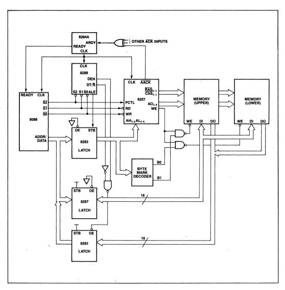
Figure 16. 8086 Hook-up to 8207 Non-ECC Synchronous System-Single Port.
