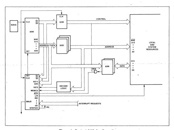
Figure 6. Typical OSP Configuration
