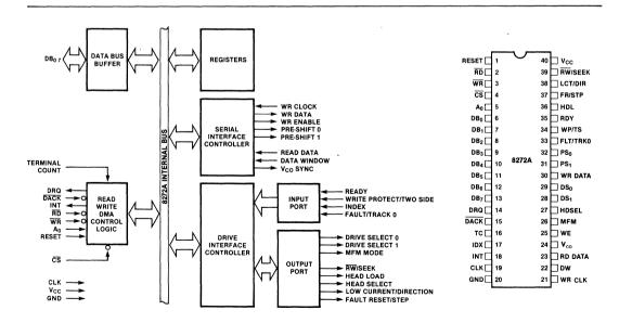
Figure 1. 8272A Internal Block Diagram
