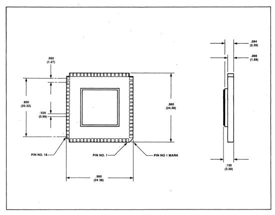
Figure 18. 8207 JEDEC Type A Package
