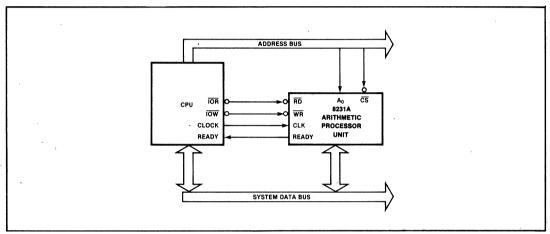
Figure 3. Minimum Configuration Example
