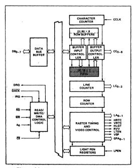
Figure 24. Block Diagram Showing FIFO Activation
