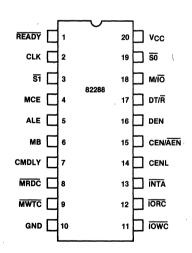
Figure 2. 82288 Pin Diagram
