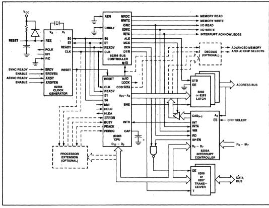
Figure 31. Basic iAPX 286 System Configuration
