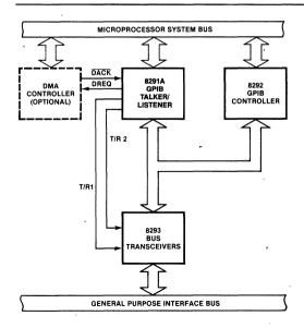
Figure 1. 8291A, 8292, 8293 Block Diagram
