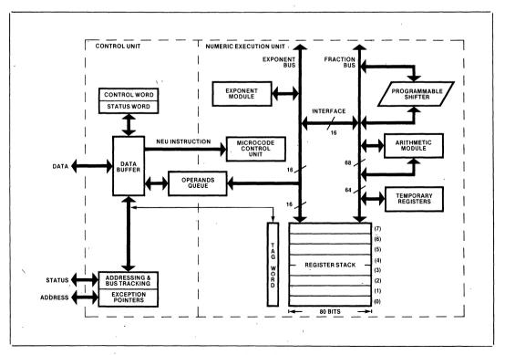
Figure 5. 8087 Block Diagram
