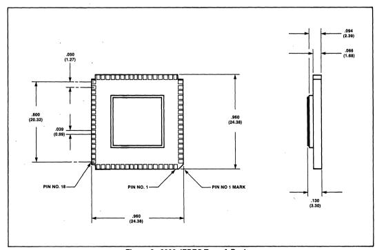
Figure 6. 8206 JEDEC Type A Package
