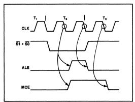
Figure 11. MCE Operation for an INTA Bus Cycle
