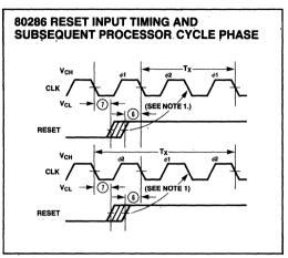
**NOTE 1:** When RESET meets the setup time shown, the next CLK will start or repeat  $\phi$ 1 of a processor cycle.
