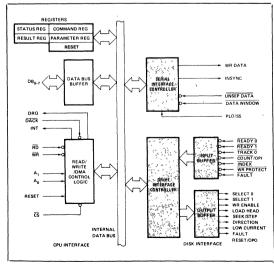
Figure 4. 8271 Block Diagram Showing Disk Interface
