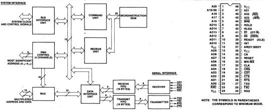
Figure 1. 82586 Functional Block Diagram Figure 2. 82586 Pinout
