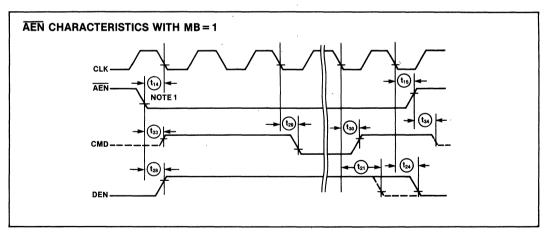
NOTE 1: ĀEN is an asynchronous input. ĀEN setup and hold time is specified to guarantee the response shown in the waveforms.
