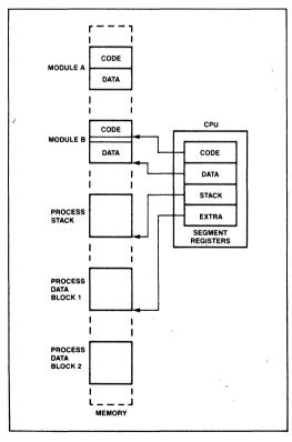
Figure 6. Segmented Memory Helps Structure Software
