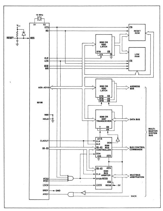
Figure 40. Typical iAPX 186 Multi-Master Bus Interface
