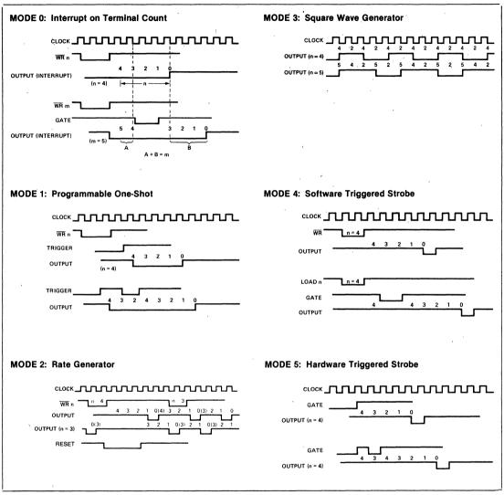
Figure 7. 8253 Timing Diagrams
