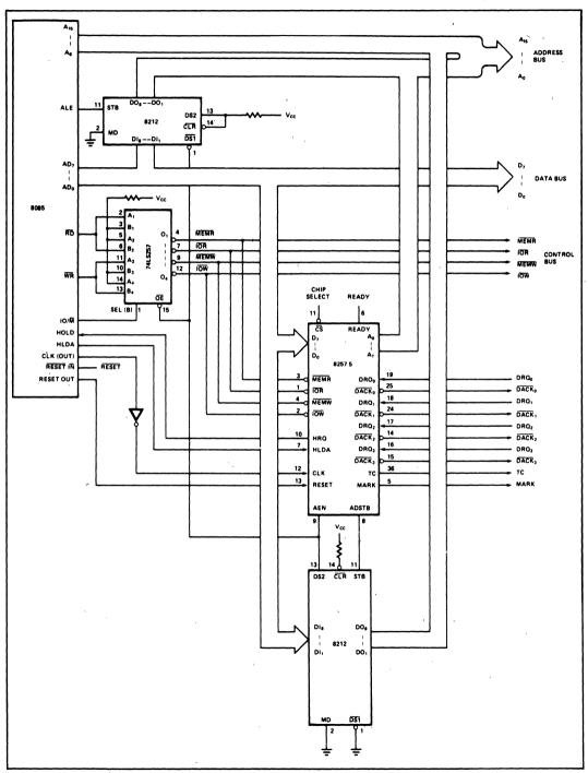
Figure 13. Detailed System Interface Schematic
