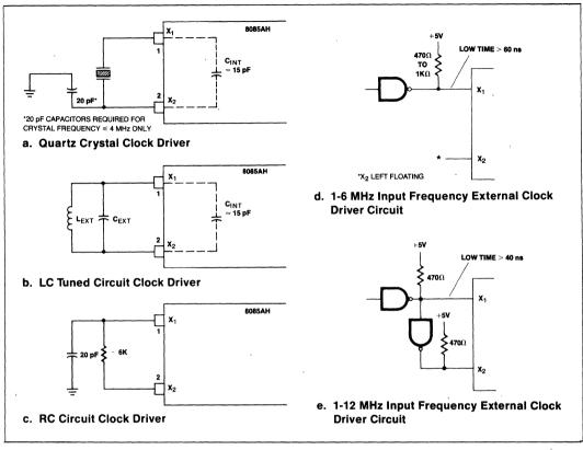
Figure 5. Clock Driver Circuits
