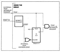
Figure 4. TRAP and RESET IN Circuit
