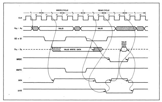
Figure 27. Back to Back Write-Read Cycles
