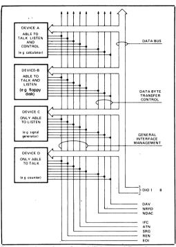
Figure 4. Interface Capabilities and Bus Structure
