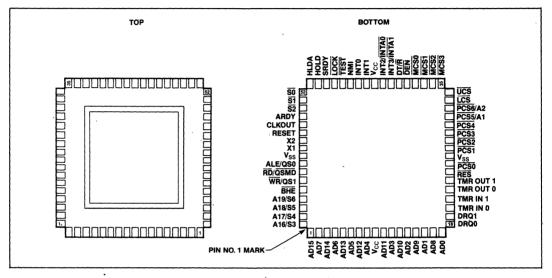
Figure 2. 80186 Pinout Diagram
