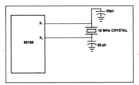
Figure 8. Recommended iAPX 188 Crystal Configuration
