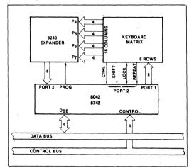
Figure 5. 8042/8742-8243 Keyboard Scanner
