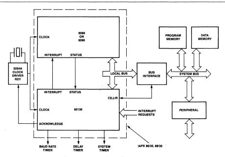
Figure 1. iAPX 86/30, 88/30 Block Diagram
