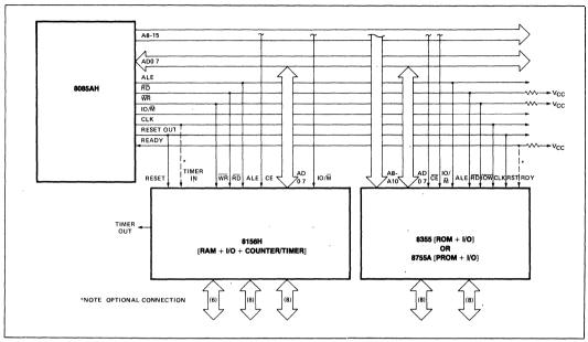
Figure 8. MCS-85® Minimum System (Memory Mapped I/O)
