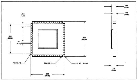
Figure 34. 80286 JEDEC Type A Package
