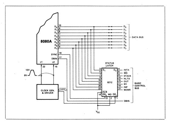
Note: The mode signal is tied high so that the output on the latch is active and enabled all the time.
