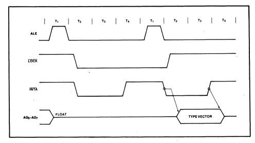
Figure 9. Interrupt Acknowledge Sequence
