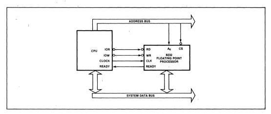
Figure 3. Minimum Configuration Example
