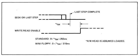
Figure 13. Head Load Settling Timing
