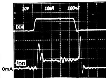
Figure 2.  $I_{DD}$  transient current during I/O cycles.
