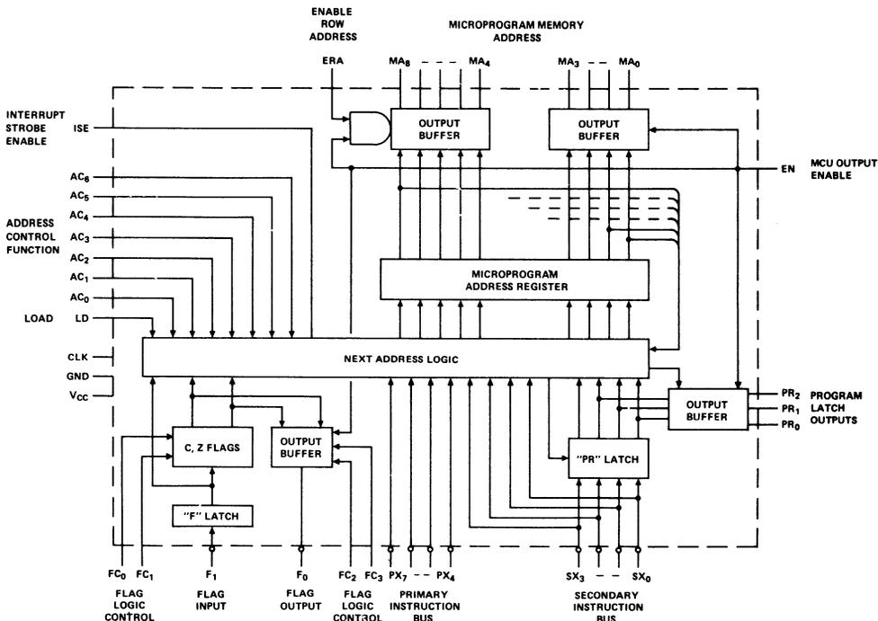
Figure 2. 3001 Block Diagram
