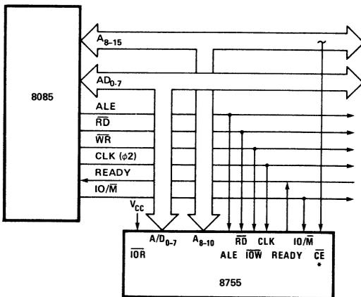
\*USE  $\overline{CE}$  FOR FIRST 8755 IN SYSTEM, AND CE FOR OTHERS. BY CONNECTING CE OF EACH 8755 CHIP TO EACH OF  $A_{11}$  THROUGH  $A_{15}$ , THE MINIMUM SYSTEM CAN USE 5-8755's (10K BYTES) WITHOUT REQUIRING CE DECODER.
