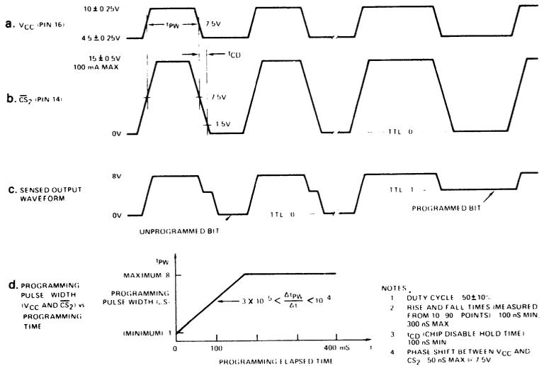
Figure 5. Pulses During Programming.
