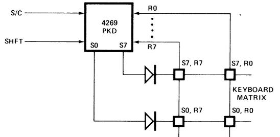
NOTE THAT ISOLATION DIODES MUST BE PLACED IN THE SCAN LINES AS SHOWN IF THE SCAN LINES ARE ALSO USED TO STROBE A DISPLAY. IF THE KEYBOARD USED HAS A DIODE AT EACH KEY, THEN THE SCAN LINE ISOLATION DIODES ARE NOT REQUIRED.
