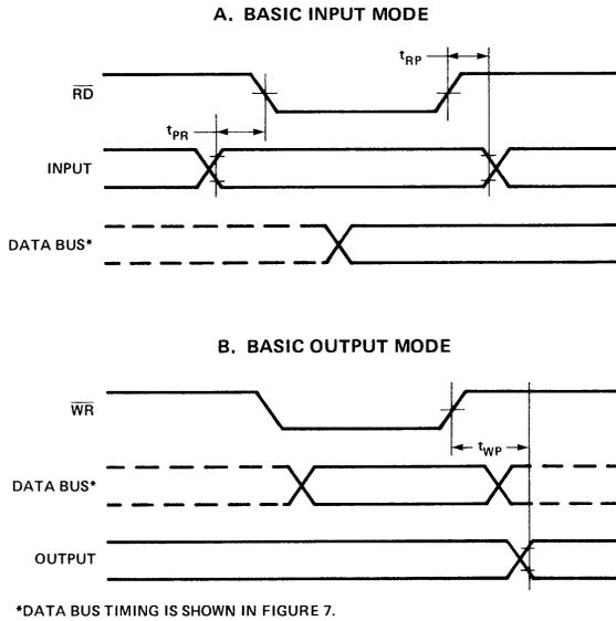
**FIGURE 9. STROBED I/O TIMING WAVEFORM.**
