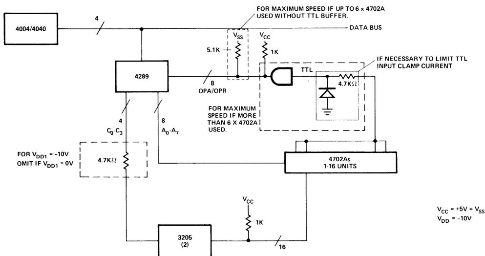
Figure 4. 4289 and 4702A Block Diagram.
