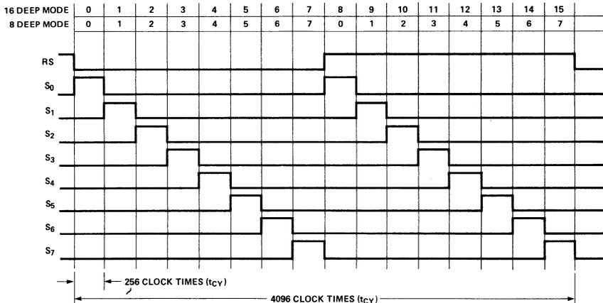
Figure 11. Individually Scanned Display Mode Timing After Execution of 0 or 16 WRM Instruction (or 8 WRMs for 8 Nibbles Deep Mode).
