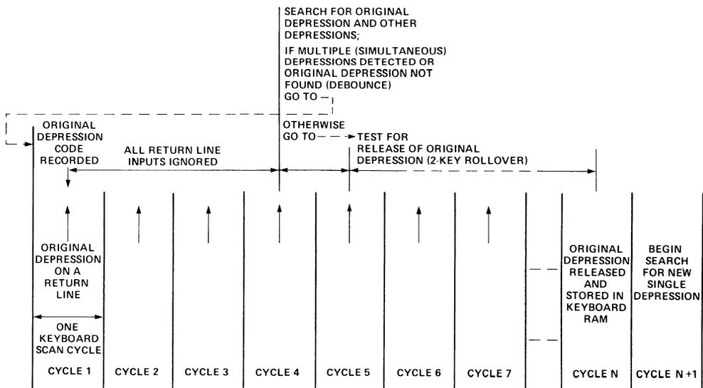
Figure 3. Keyboard Debounce and 2-Key Rollover Timing.
