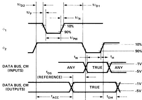
Figure 10. Timing Detail.
