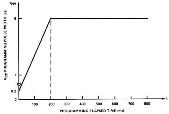
Figure 3.  $V_{CC}$  Pulse Width vs. Programming Time.
