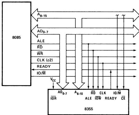
**FIGURE 2. 8355 IN 8085 SYSTEM (MEMORY-MAPPED I/O).**
