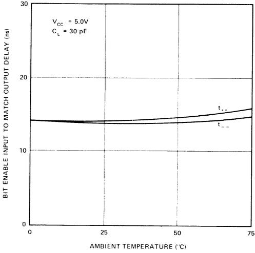
**DATA INPUT TO MATCH OUTPUT DELAY VS. TEMPERATURE**
