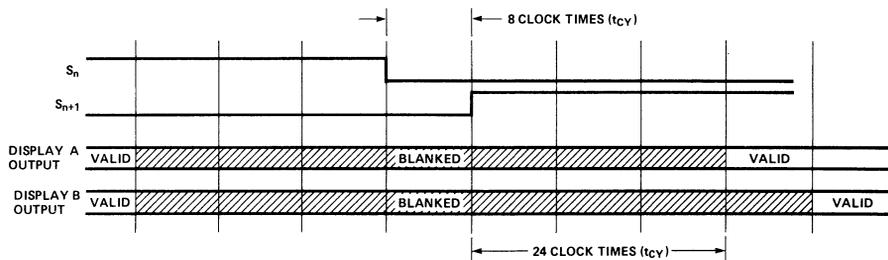
Figure 12. Individually Scanned Display Mode.
