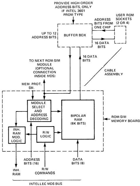
Fig. 1. Data Flow of ROM-SIM Module
