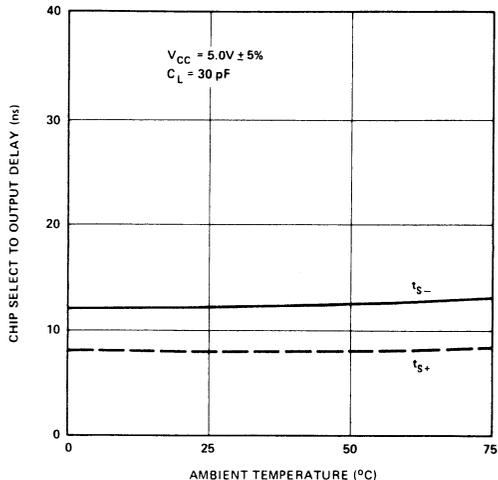
ADDRESS & CHIP SELECT TO OUTPUT DELAY
