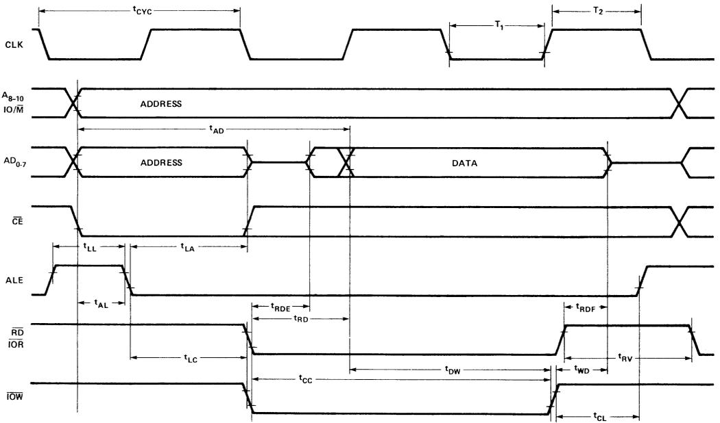
FIGURE 4. PROM READ AND I/O WRITE TIMING.
