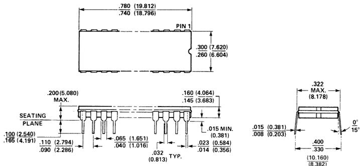
18-LEAD HERMETIC DUAL IN-LINE PACKAGE TYPE D
