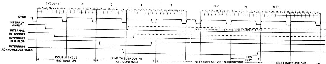
Figure 5. Interrupt Timing.
