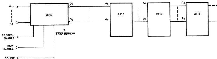
Figure 1. Typical Connection of 3242 and 2116 Memories.
