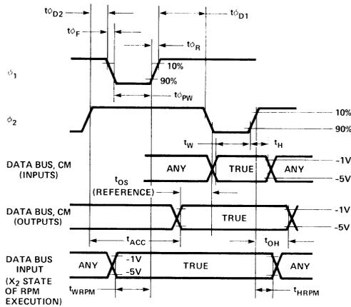
Figure 2. Timing Detail.
