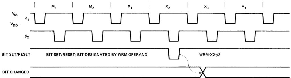
Figure 8. Bit Set/Reset Operation Timing.
