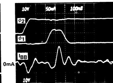
Figure 3.  $I_{BB}$  transient current during a shift cycle.
