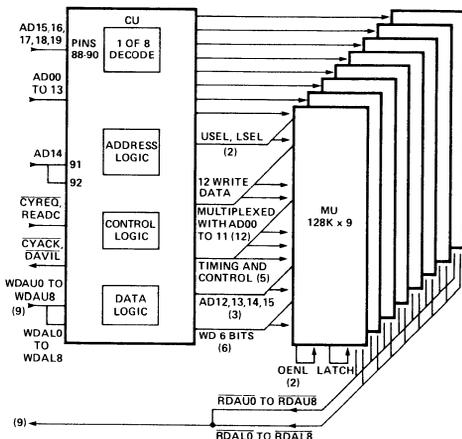
**in-1600 Series Block Diagram (Word Length Less Than 9-Bits)**
