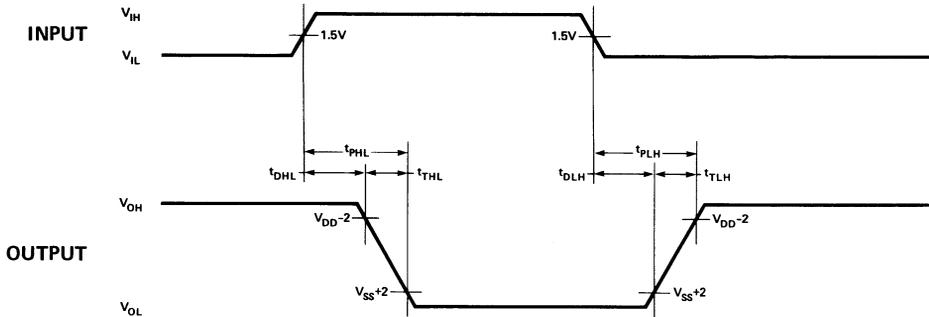
**B. 5244 OUTPUT CROSS-COUPLED VOLTAGE (DRIVING FOUR 2416'S)**
