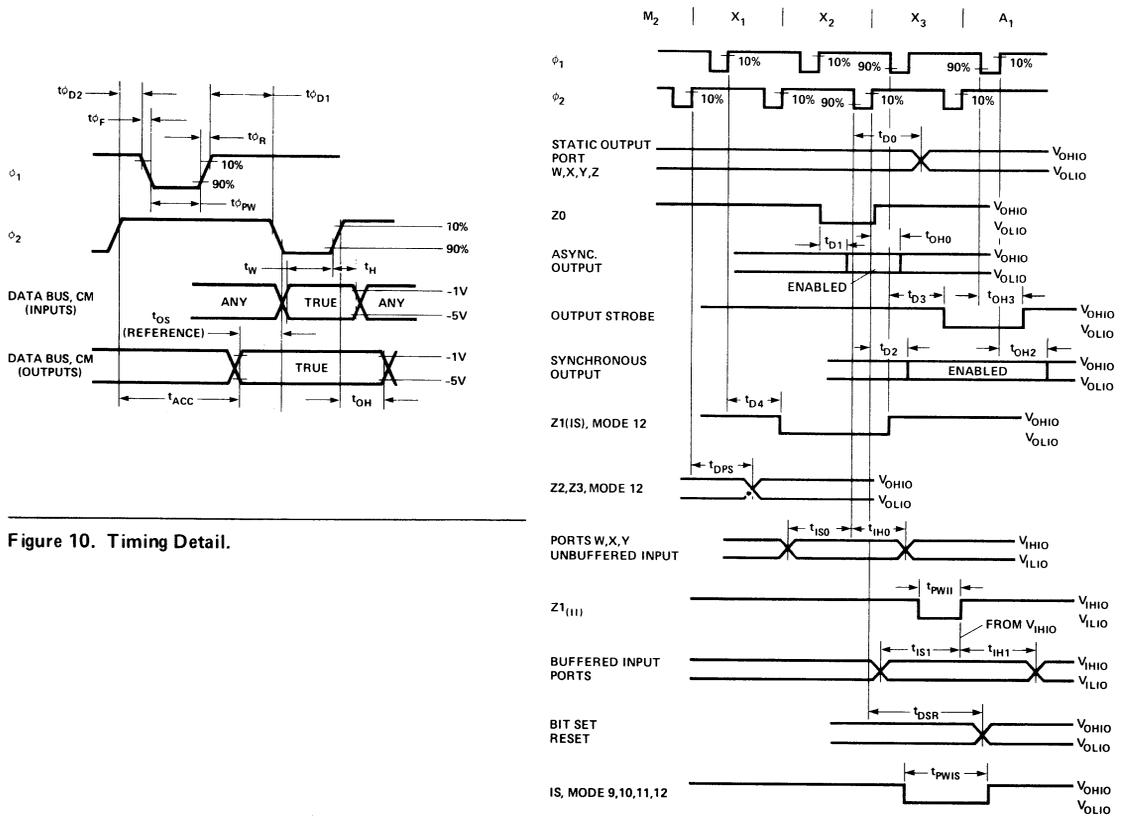
Figure 10. Timing Detail.
