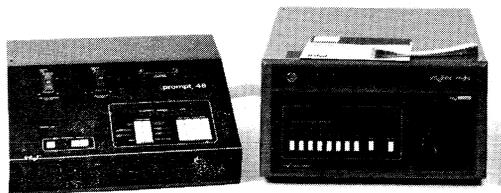
A Specialized PROM Programmer Kit, the PROMPT-SPP, allows PROMPT 48 to serve as an economical 8748 Specialized PROM Programmer peripheral in Intellec Microcomputer Development Systems. The PROMPT-SPP cable plugs directly into the rear panel of the Intellec Microcomputer Development System.
