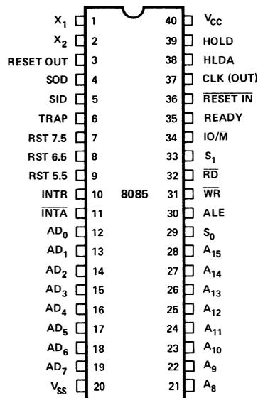
Figure 1. 8085 PINOUT DIAGRAM
