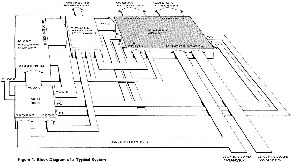
Figure 1. Block Diagram of a Typical System
