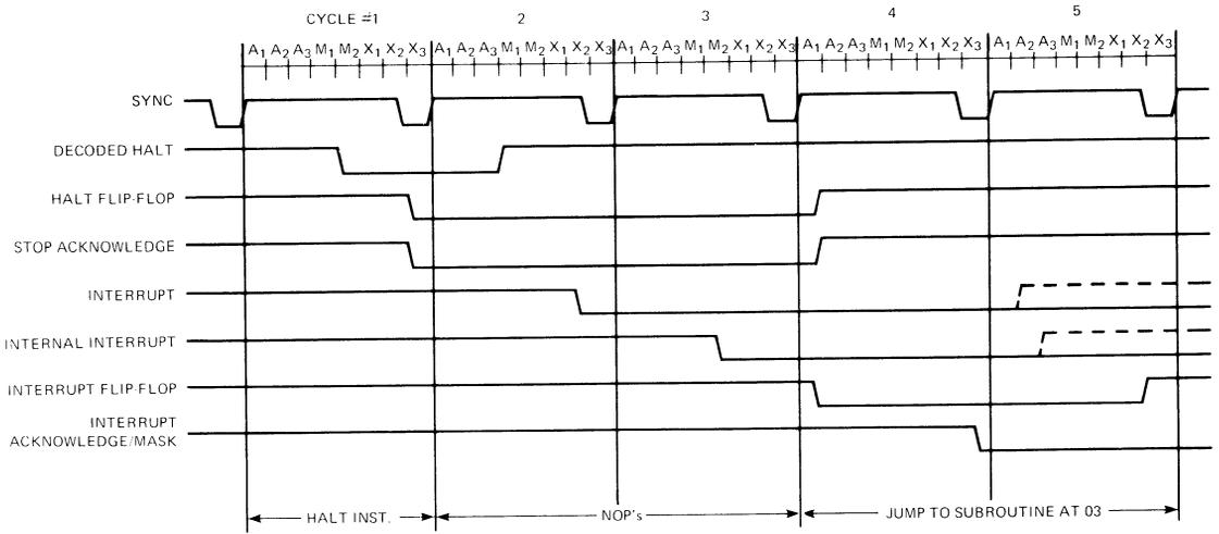
Figure 6. Halt Timing (Exit Using Interrupt).
