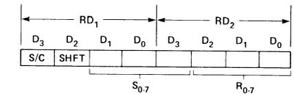
Figure 6. Key Encoding.
