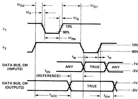
Figure 2. Timing Detail
