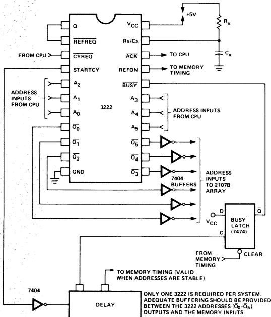
F. USE OF 3222 FOR REFRESH TIMING AND CONTROL IN A 2104A SYSTEM
