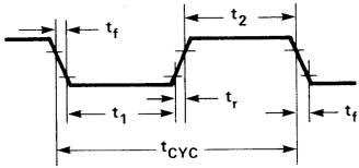
FIGURE 3. CLOCK TIMING WAVEFORM
