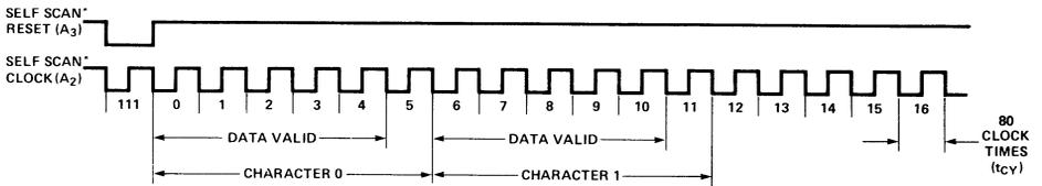
Figure 17. Gas Discharge (Self-Scan®) Mode Timing – 18 Character Mode.
