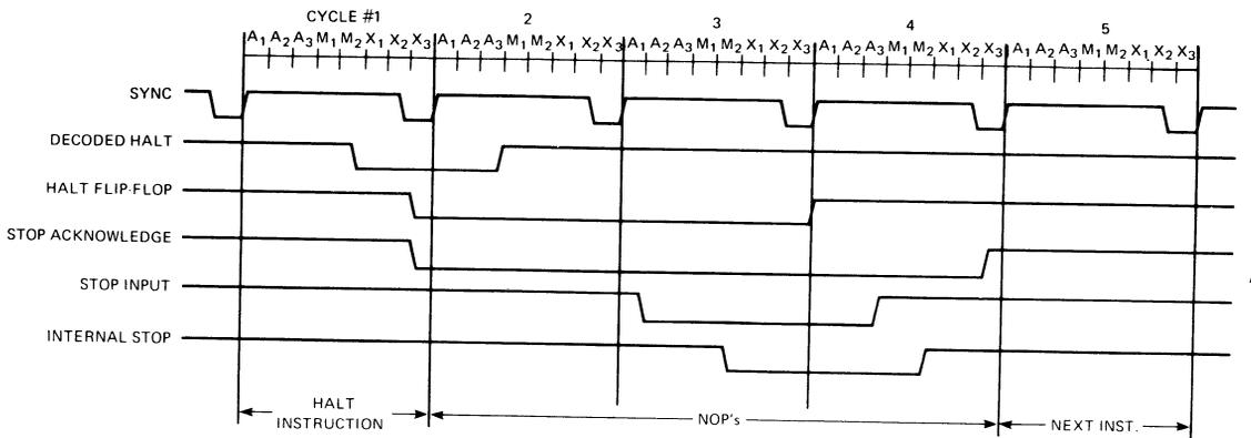
Figure 4. Halt Timing (Exit Using Stop Input).
