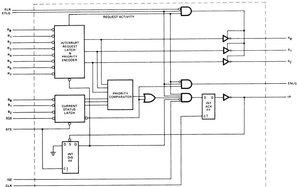
Figure 1. 3214 Block Diagram.
