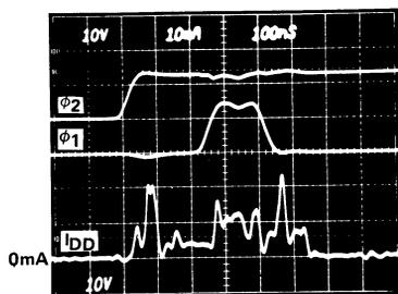
Figure 1.  $I_{DD}$  transient current during shift cycles.
