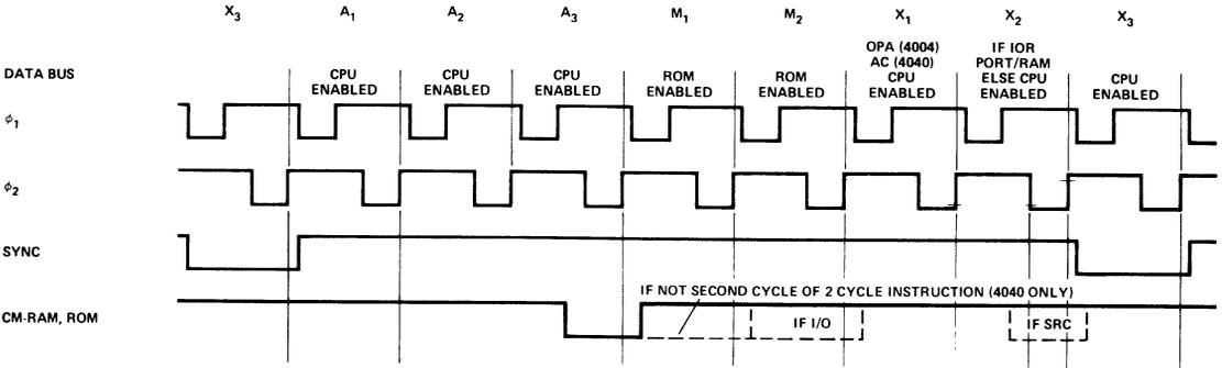
Figure 9. Timing Diagram.
