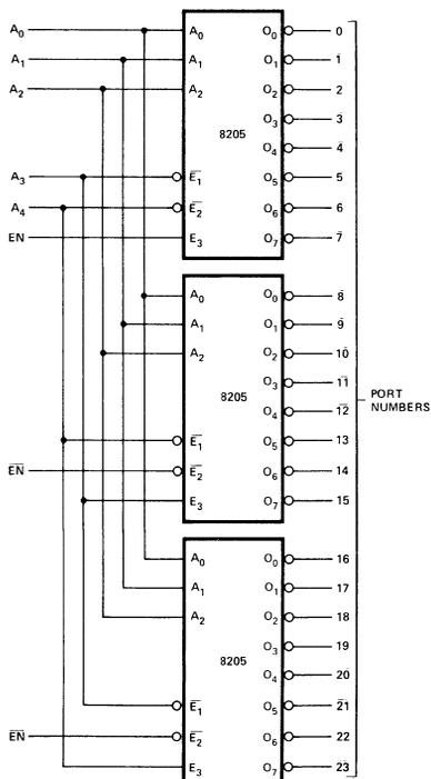
ray of 8205s can be used to create a simple interface to a 24K memory system.
