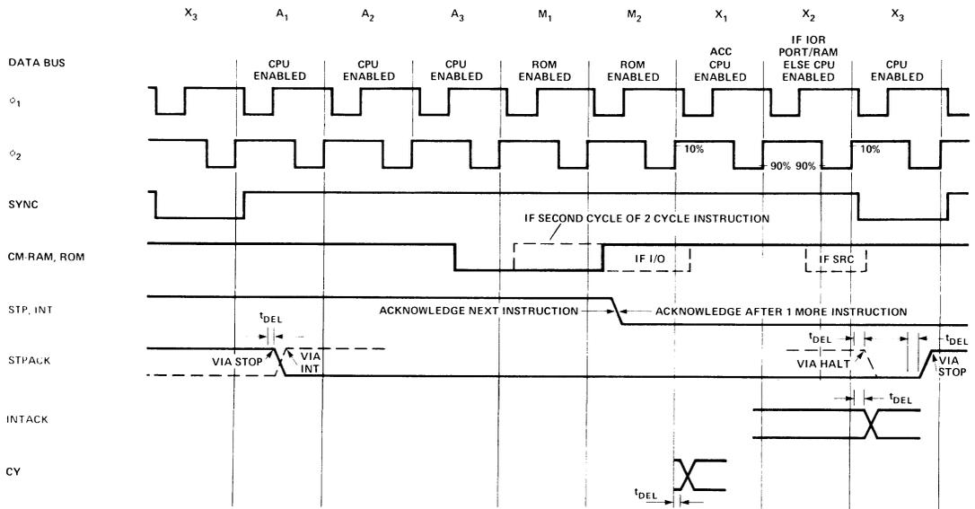
Figure 1. Timing Diagram.
