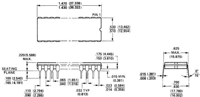
40-LEAD HERMETIC DUAL IN-LINE PACKAGE TYPE D
