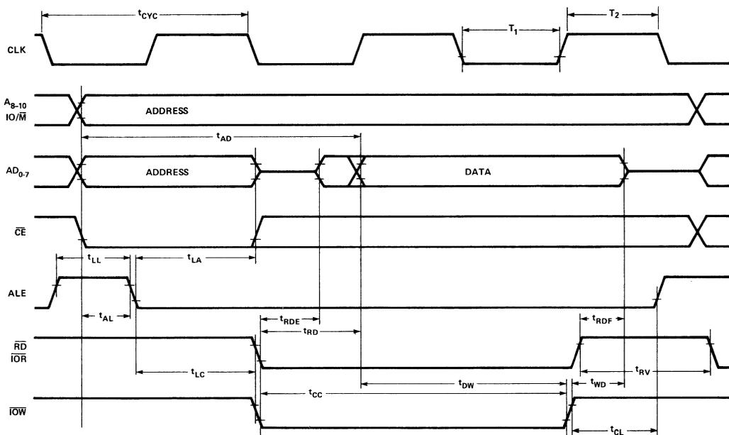
FIGURE 5. ROM READ AND I/O READ AND WRITE.
