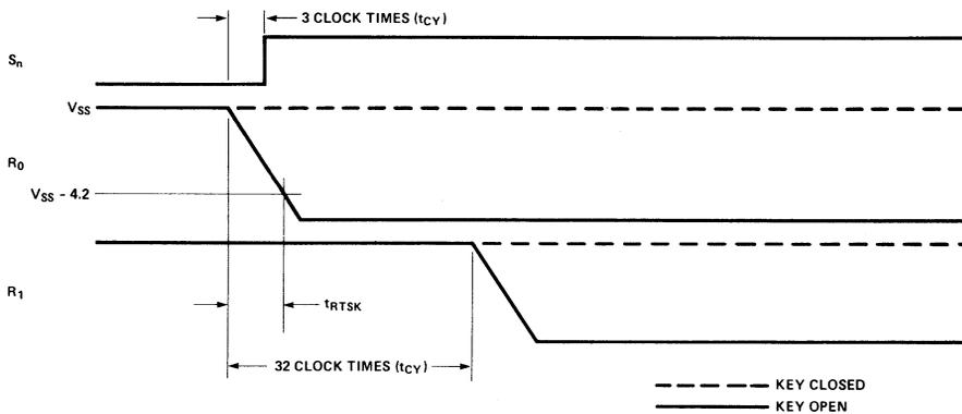
Figure 14. Detailed Timing - Scanned Keyboard Mode.
