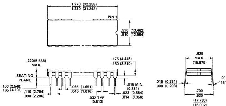
28-LEAD HERMETIC DUAL IN-LINE PACKAGE TYPE D
