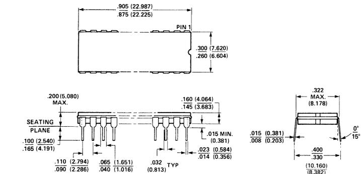
22-LEAD HERMETIC DUAL IN-LINE PACKAGE TYPE D
