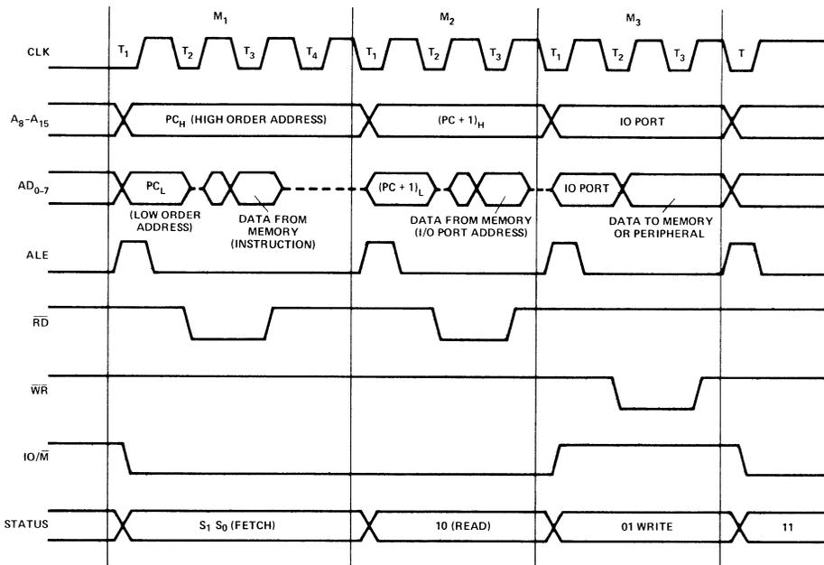
FIGURE 2. 8085 BASIC SYSTEM TIMING.
