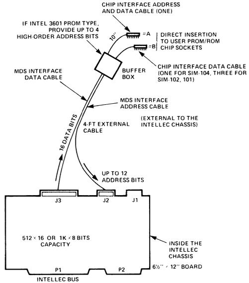
Fig. 2. Cable Connection of ROM-SIM Module
