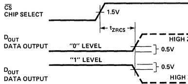
(All t<sub>ZXXX</sub> parameters are measured at a delta of 0.5V from the logic level and using Load 1.)
