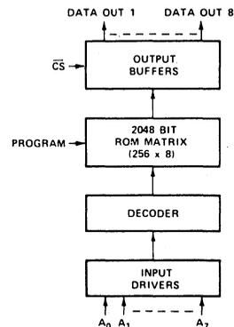
NOTE: In the read mode a logic 1 at the address inputs and data outputs is a high and logic 0 is a low.
