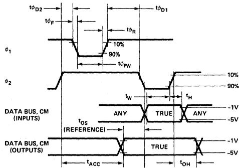
Figure 2. Timing Detail
