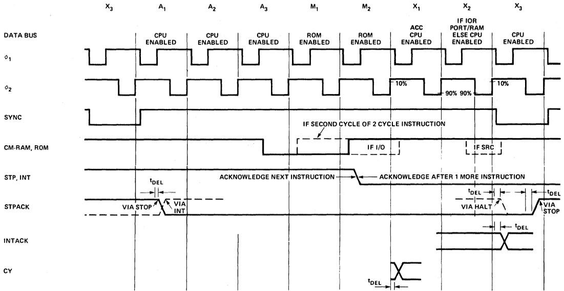
Figure 1. Timing Diagram.
