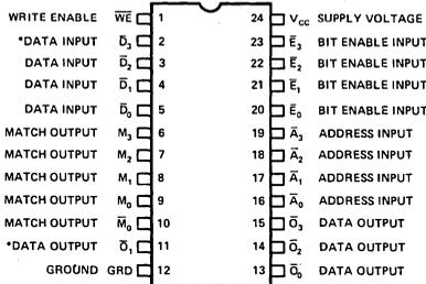
\*DATA IN and DATA OUT are of the same logic levels. For a chip that is not selected, the data output is at a high level.
