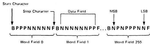
3. Between word fields, comments not containing B's or F's may be inserted. Carriage return and line feed characters should be inserted (as a "comment") just before each word field (or at least between every four word fields). When these carriage returns, etc., are inserted, the tape may be easily listed on the teletype for purposes of error checking. It may be helpful to insert the word number (as a comment) at least every four word fields.
