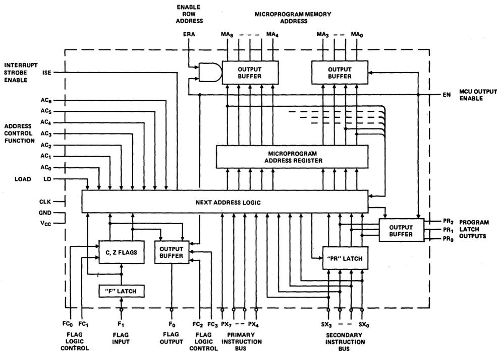
Figure 2. 3001 Block Diagram
