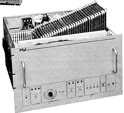
The **in-Jumbochassis** is designed for memory systems that may be mounted in a 24" cabinet. With integral power supplies and fan assemblies, it measures only 14" H x 24" W x 24" D. Forty-three card slots are available to house thousands of combinations of standardized Intel memory cards. For example, a 128K x 18 or 256K x 9 in-10 system, or a 512K x 18 or 1024K x 9 in-40 system can be housed with seven I/O slots left over for address and data buffers or for other custom logic.
