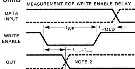
NOTE 2: Output Data is valid after  $t_{+-}, t_{+-}$
