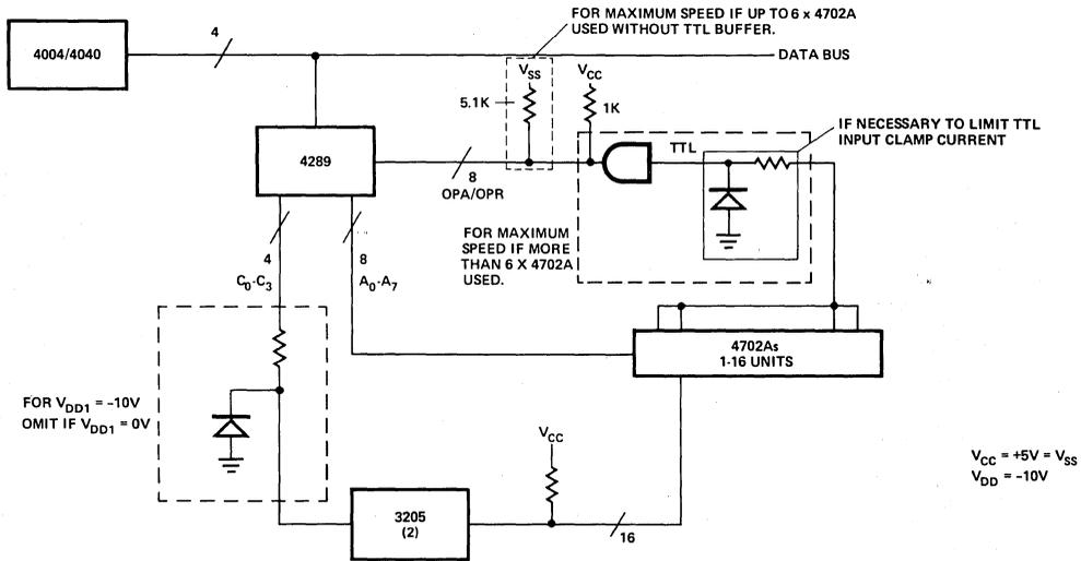
Figure 4. 4289 and 4702A Block Diagram.
