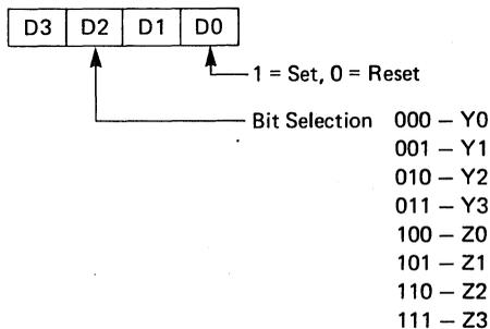
Care should be taken when bit setting and resetting control bits of Port Z as these bits will also be changing as a function of their synchronous or asynchronous control functions.
