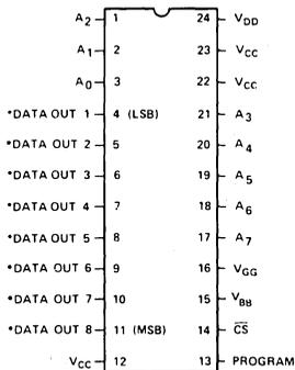
\*THIS PIN IS THE DATA INPUT LEAD DURING PROGRAMMING
