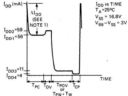
Note 1.  $\Delta I_{DD}$  is due to charging of internal device node capacitance at precharge
