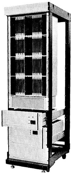
**in-CAB-HB** Memory Cabinet can accommodate up to 96 MU-10/MU-40 series cards. This memory cabinet is 72" high, 19" wide and 30" deep. It is designed to be free-standing and contains room for cooling fans, power supplies and interface cabling. The memory size can vary from 32K x 144 to 256K x 18 bits. All power supplies are mounted on slides for easy access.
