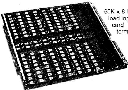
65K x 8 Memory System with a 32 bit parallel load input and an 8 bit wide serial output. The card is used for CRT refresh in an intelligent terminal.
