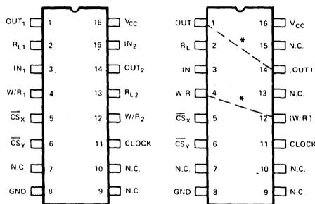
\* DASH LINES INDICATE NECESSARY EXTERNAL PRINTED CIRCUIT BOARD CONNECTIONS FOR PROPER OPERATION OF THE 2405. (SEE APPLICATION SECTION)
