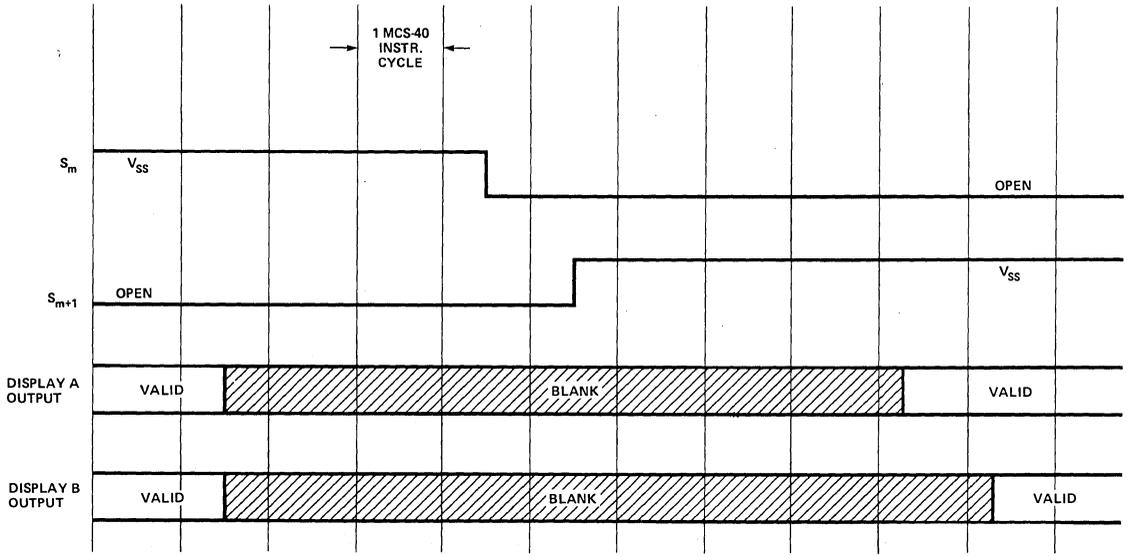
Figure 11. Data Blanking Detail - Individual Display Mode.
