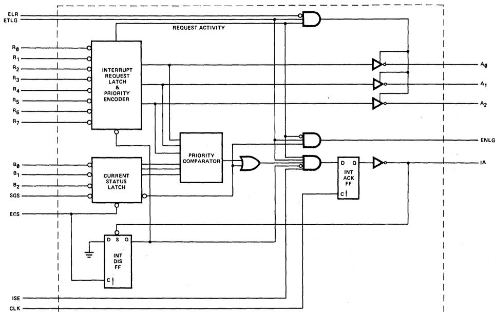
Figure 1. 3214 Block Diagram.
