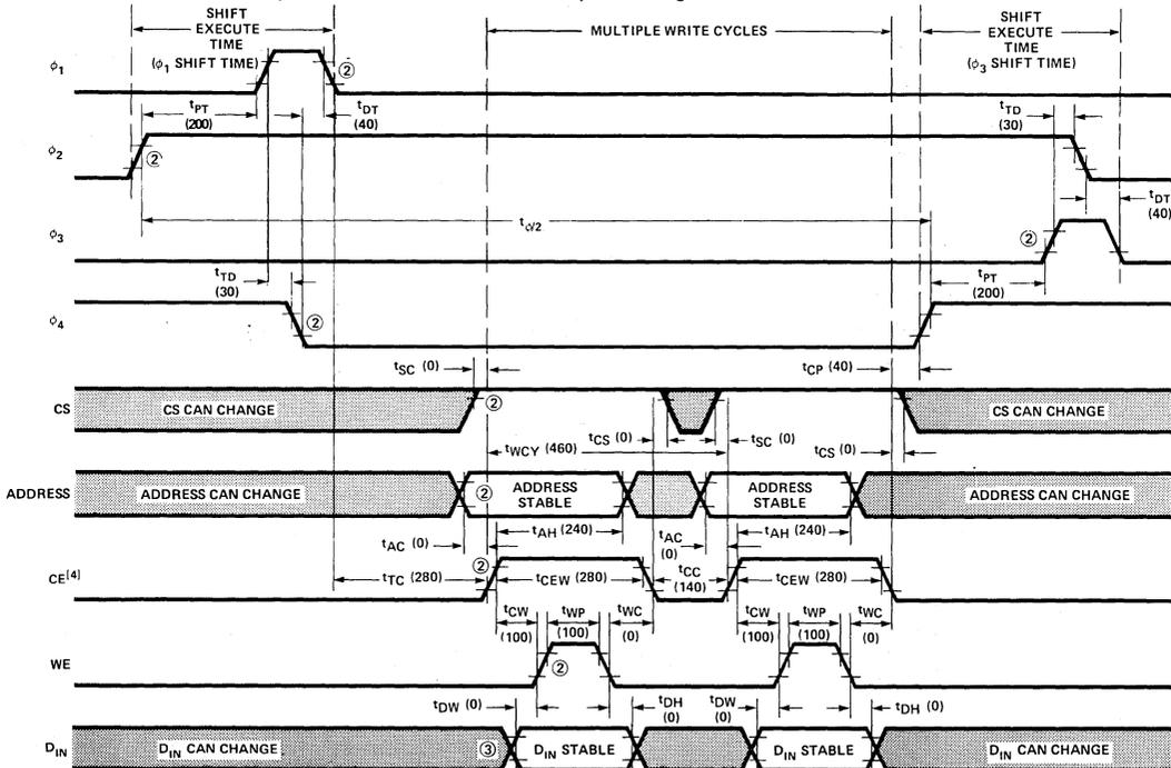
Notes: 2. +2.0V and V<sub>DD</sub>-2.0V are the reference low and high level respectively for measuring the timing of φ<sub>1</sub> . . . φ<sub>4</sub>, CE, CS, WE, and addresses.
