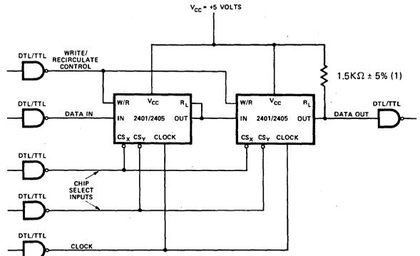
NOTE (1): The 2401/2405 is directly compatible device to device. An external 1.5K $\Omega$   $\pm$  5% load resistor is recommended for driving one TTL load with the 2401/2405 output.
