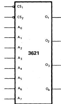
NOTE 1. DURING PROGRAMMING, THE PROGRAM PULSE MAY BE APPLIED TO EITHER CS<sub>1</sub> OR CS<sub>2</sub> FOR THE 3621 FAMILY. THE PROGRAM PULSE IS APPLIED TO CS<sub>2</sub> FOR THE 3601 FAMILY.
