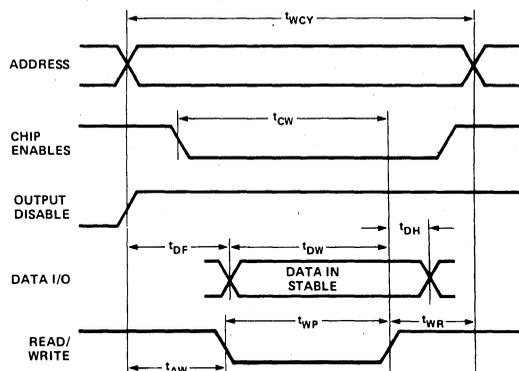
NOTE: 1.  $t_{DF}$  is with respect to the trailing edge of  $\overline{CE1}$ ,  $\overline{CE2}$ , or OD, whichever occurs first.
