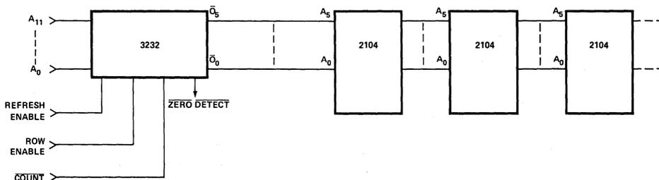
Figure 1. Typical Connection of 3232 and 2104 Memories.
