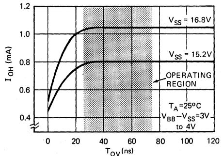
**AC Characteristics**  $T_A = 0^\circ\text{C to } 70^\circ\text{C}$ ,  $V_{SS} = 16 \pm 5\%$ ,  $(V_{BB} - V_{SS}) = 3.0\text{V to } 4.0\text{V}$ ,  $V_{DD} = 0\text{V}$
