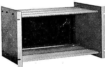
The **in-Unichassis** Memory Chassis is designed to accommodate up to 33 memory and control cards for mounting in a 19" relay rack. This chassis features the use of a full PC back plane with internal power and ground. The chassis can be wired for a number of memory sizes and configurations, and also be used in multiples for even larger memory configurations. It is 10.5" high, 12" deep, and can be used with in-CAB memory cabinet.
