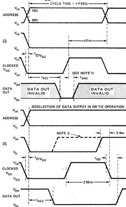
NOTE 1: The output will remain valid for  $t_{OHC}$  as long as clocked  $V_{GG}$  is at  $V_{CC}$ . An address change may occur as soon as the output is sensed (clocked  $V_{GG}$  may still be at  $V_{CC}$ ). Data becomes invalid for the old address when clocked  $V_{GG}$  is returned to  $V_{GG}$ .
