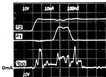
Figure 1.  $I_{DD}$  transient current during shift cycles.
