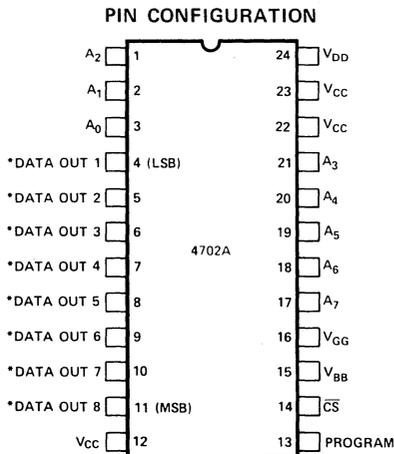
\*THIS PIN IS THE DATA INPUT LEAD DURING PROGRAMMING.
