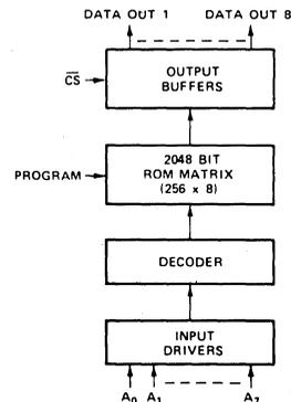
NOTE: In the read mode a logic 1 at the address inputs and data outputs is a high and logic 0 is a low.
