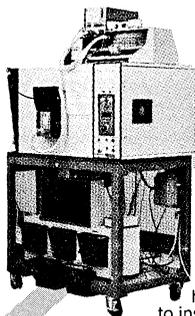
**Continuity at high temperature** to insure that no terminals will open or short at high temperatures. (Monitored by QA)
