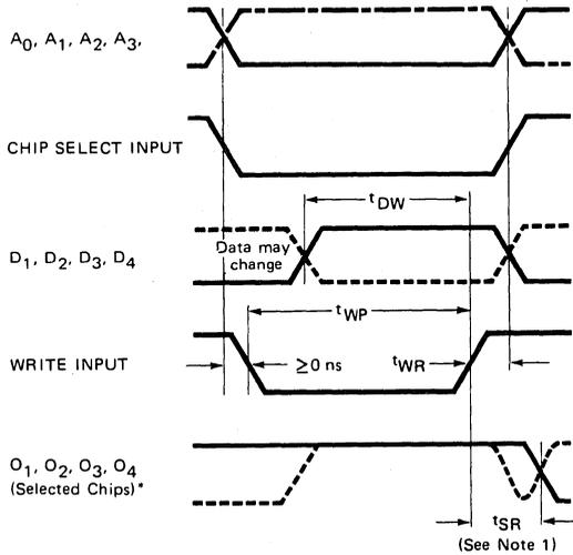
\*Outputs of unselected chips remain high during write cycle.
