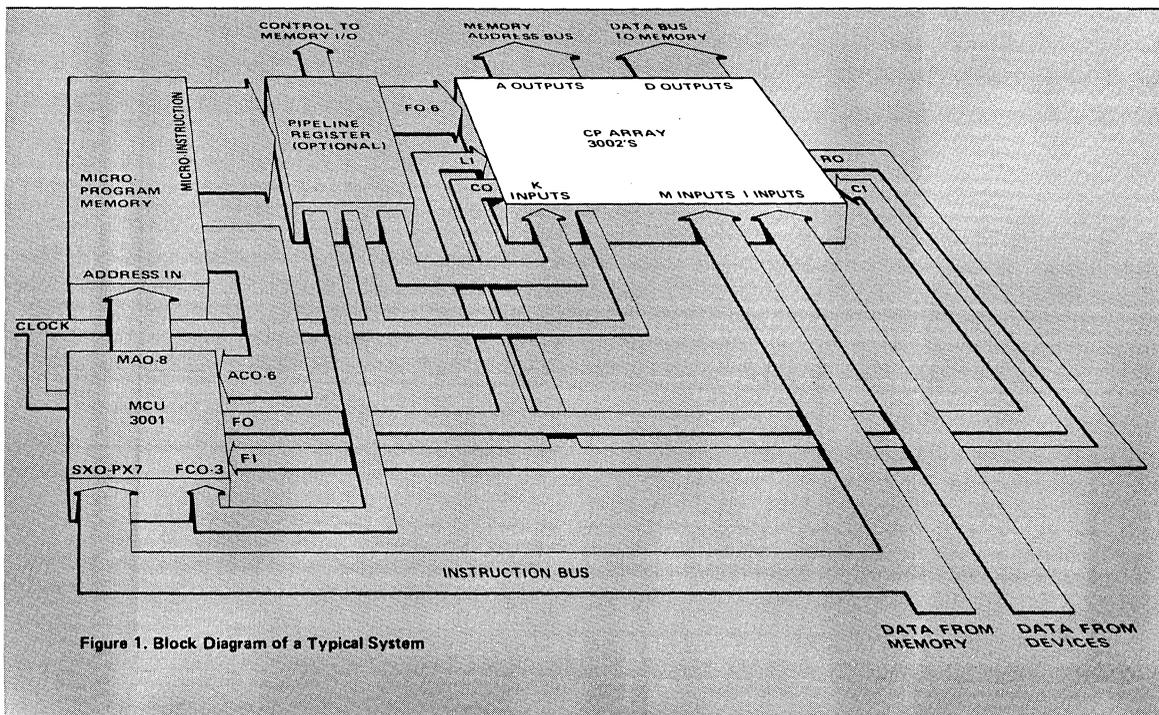
Figure 1. Block Diagram of a Typical System
