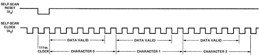
Figure 13. Gas Discharge (Self-Scan) Mode Timing - 18 Character Mode.
