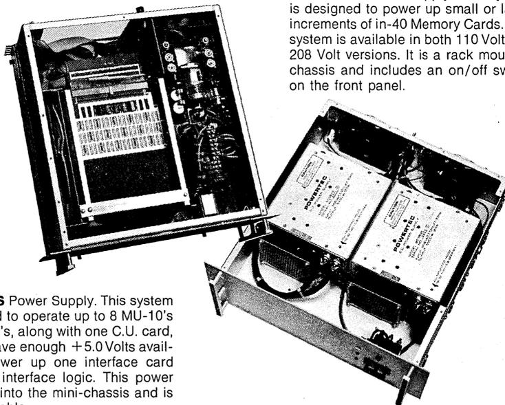
The **in-MPS** Power Supply. This system is designed to operate up to 8 MU-10's or 8 MU-40's, along with one C.U. card, and also have enough +5.0 Volts available to power up one interface card containing interface logic. This power supply fits into the mini-chassis and is rack mountable.
