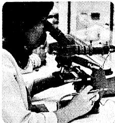
**Optical inspection** criteria based on MIL-STD-883 Method 2010.1B to insure that all devices are free from internal defects which could lead to failure in normal applications. (Monitored by QA)
