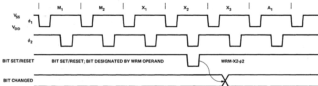
Figure 8. Bit Set/Reset Operation Timing.
