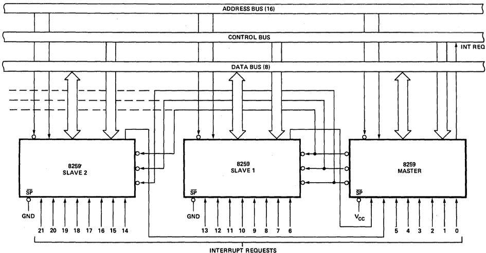
Cascading the 8259 22 Level Controller (Expandable to 64 levels).
