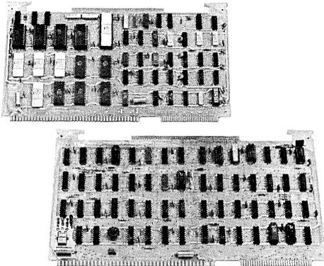
DOS Channel and Interface Controller Boards
