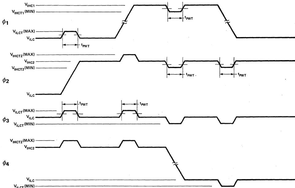
**A.C. Characteristics**  $T_A = 0^\circ\text{C to } 70^\circ\text{C}$ ,  $V_{DD} = 12\text{V} \pm 5\%$ ,  $V_{BB} = -5\text{V} \pm 5\%$ ,  $V_{SS} = 0\text{V}$ , unless otherwise specified.
