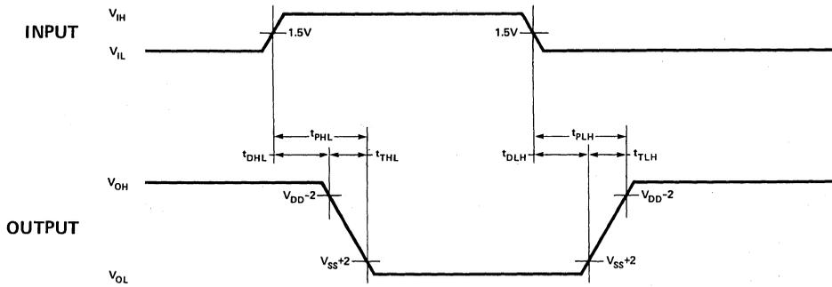
**B. 5244 OUTPUT CROSS-COUPLED VOLTAGE (DRIVING FOUR 2416'S)**
