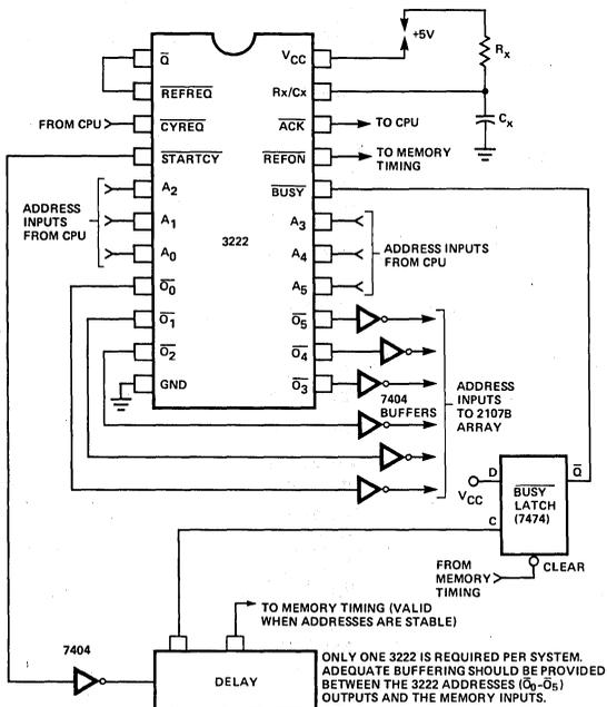
**F. USE OF 3222 FOR REFRESH TIMING AND CONTROL IN A 2104 SYSTEM**
