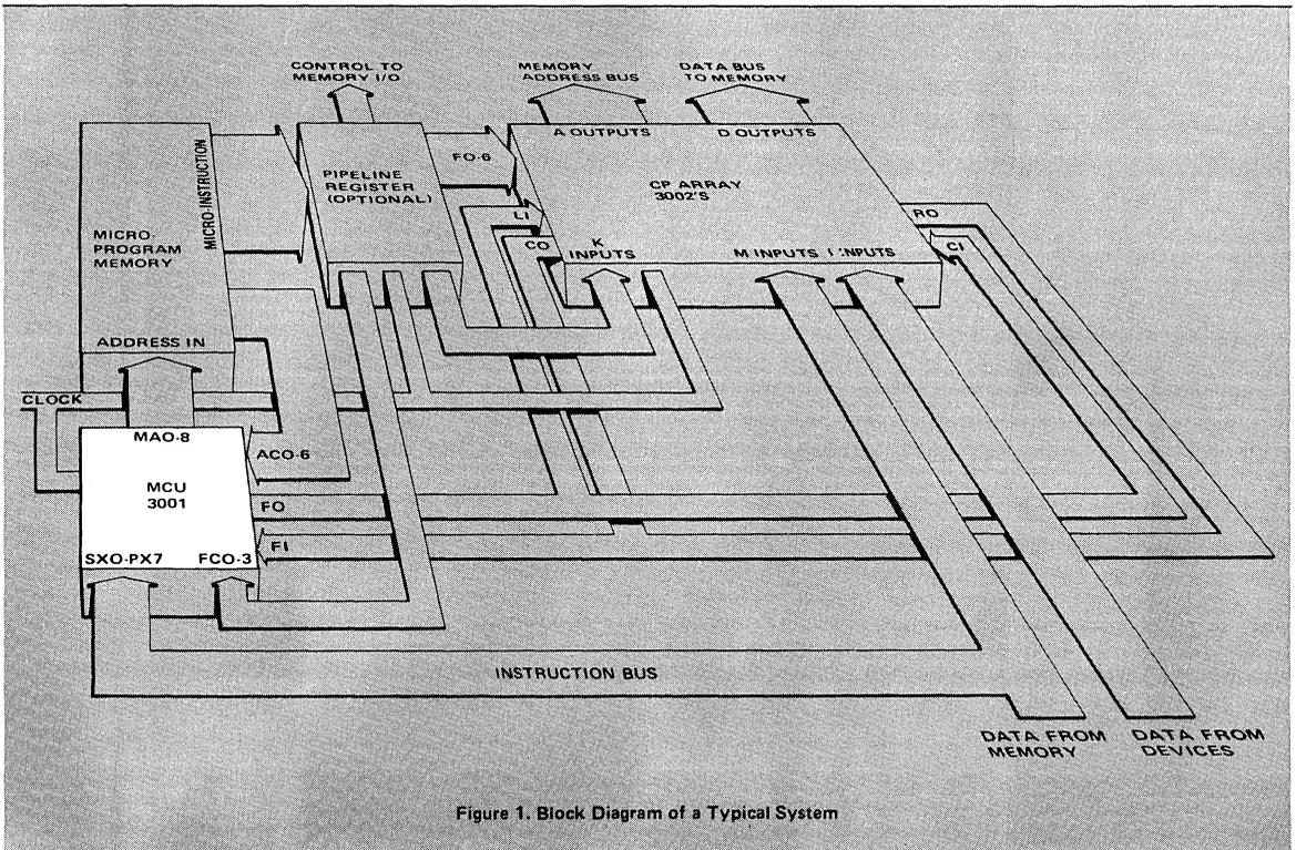
Figure 1. Block Diagram of a Typical System
