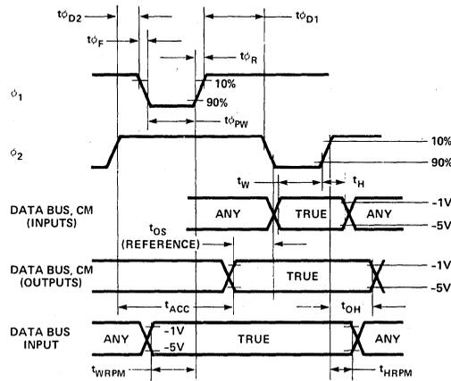
Figure 2. Timing Detail.
