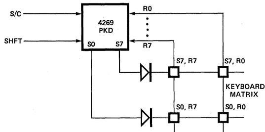
Figure 4. Hardware Configuration.
