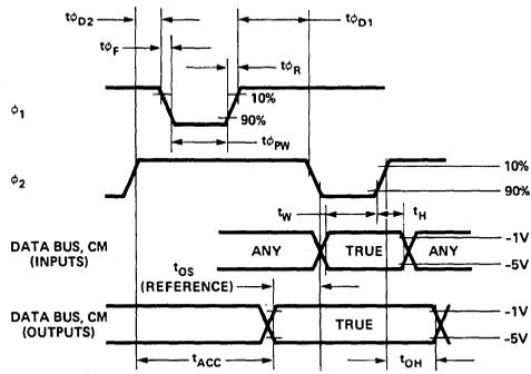
Figure 2. Timing Detail.
