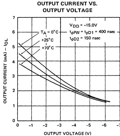
A.C. Characteristics  $T_A = 0^\circ\text{C to } 70^\circ\text{C}$ ,  $V_{SS} - V_{DD} = 15\text{V} \pm 5\%$
