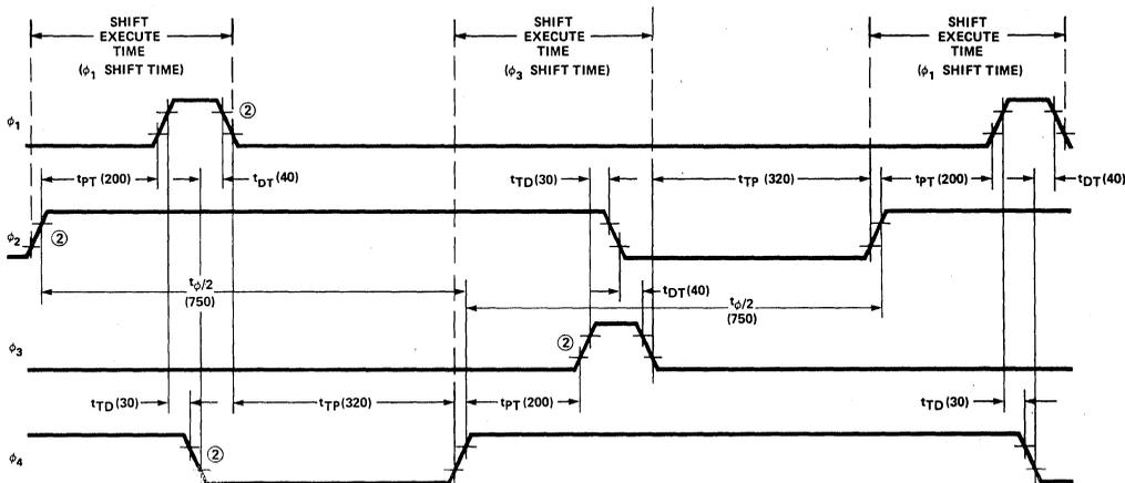
Note: 2. +2.0V and  $V_{DD}-2.0\text{V}$  are the reference low and high level respectively for measuring the timing of  $\phi_1, \phi_2, \phi_3$  and  $\phi_4$ .
