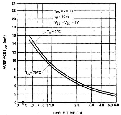
**A.C. Characteristics**  $T_A = 0^\circ\text{C}$  to  $70^\circ\text{C}$ ,  $V_{SS} = 16\text{V} \pm 5\%$ ,  $(V_{BB} - V_{SS}) = 3.0\text{V}$  to  $4.0\text{V}$ ,  $V_{DD} = 0\text{V}$
