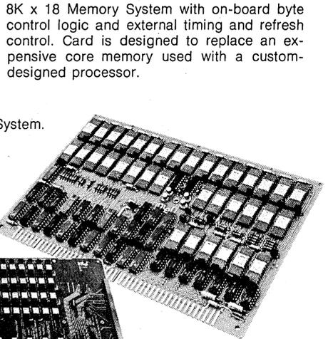
8K x 18 Memory System with on-board byte control logic and external timing and refresh control. Card is designed to replace an expensive core memory used with a custom-designed processor.
