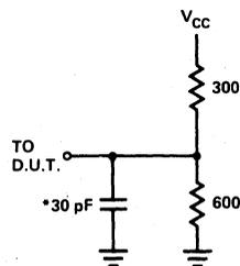
\* INCLUDING JIG &amp; PROBE CAPACITANCE
