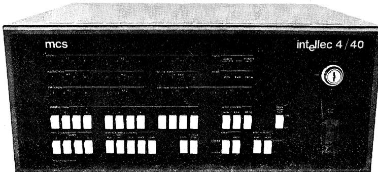
The Intellec® 4/MOD 40 (imm 4-44A) is a complete, self-contained microcomputer development system designed specifically to support the development and implementation of 4040 and 4004 CPU based microcomputer systems. Its modular design provides the flexibility to adapt to any size user system and the resident software facilitates program development.
