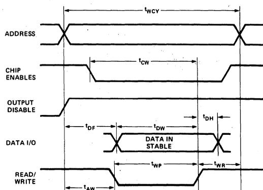
NOTE: 1.  $t_{DF}$  is with respect to the trailing edge of  $\overline{CE1}$ ,  $\overline{CE2}$ , or OD, whichever occurs first.
