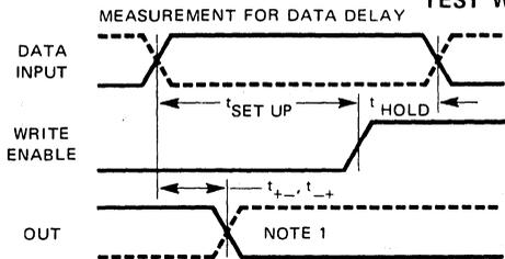
NOTE 1: Output Data is valid after  $t_{+-}, t_{+-}$
