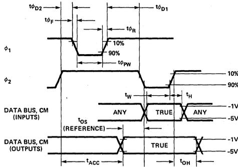
Figure 2. Timing Detail.
