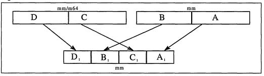
Figure 5-2. Interleaved Pack with Saturation Example
