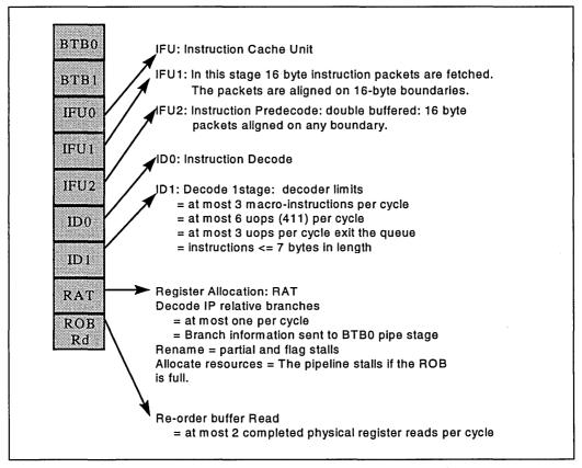
Figure 2-3. Out-Of-Order Core and Retirement Pipeline
