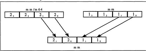
Figure 5-3. Result of Non-Interleaved Unpack in MMO
