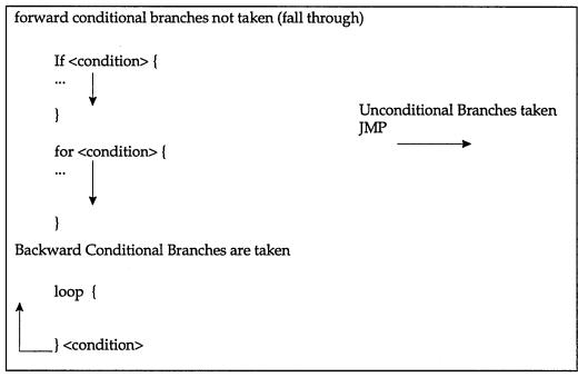
Figure 3-2. Dynamic Execution (P6-Family) Static Branch Prediction Algorithm
