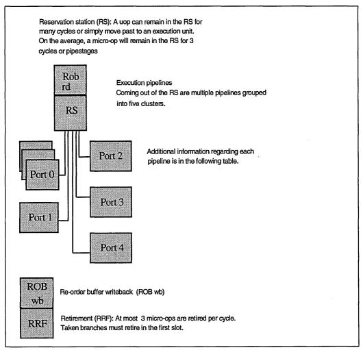
Figure 2-4. Out-Of-Order Core and Retirement Pipeline
