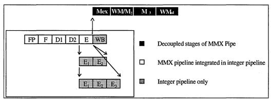
Figure 2-1. MMX<sup>™</sup> Pipeline Structure
