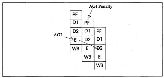
Figure 3-1. Pipeline Example of AGI Stall
