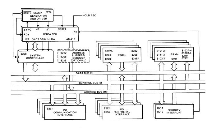
Figure 3-6. Microcomputer System
