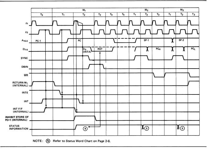
Figure 2-8. Interrupt Timing
