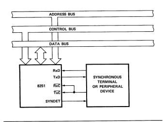
Synchronous Interface to Terminal or Peripheral Device
