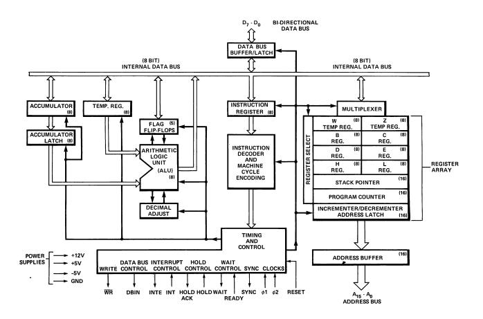
Figure 2-2. 8080 CPU Functional Block Diagram
