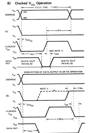
NOTE 1: The output will remain valid for  $t_{OHC}$  as long as clocked  $V_{GG}$  is at  $V_{CC}$ . An address change may occur as soon as the output is sensed (clocked  $V_{GG}$  may still be at  $V_{CC}$ ). Data becomes invalid for the old address when clocked  $V_{GG}$  is returned to  $V_{GG}$ .
