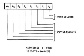
Figure 3-11. Isolated I/O - (Linear Select) (8255)
