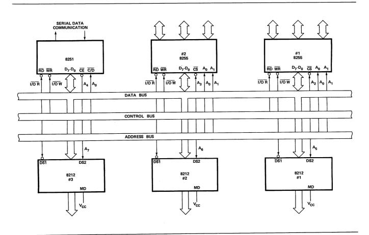
Figure 3-16. Typical I/O Interface.
