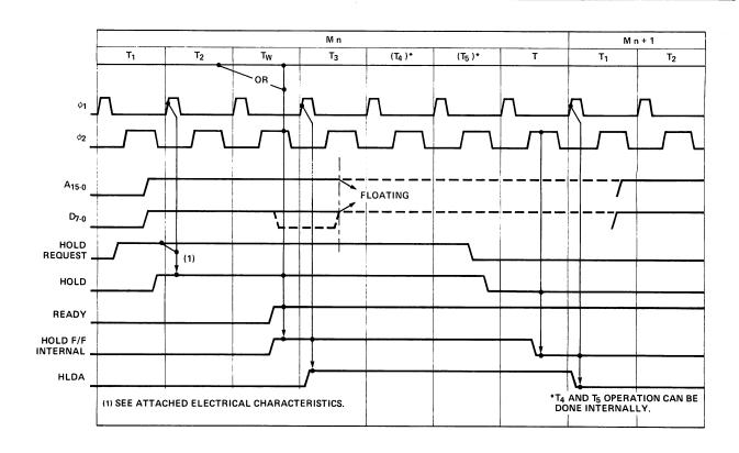
Figure 2-9. HOLD Operation (Read Mode)
