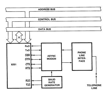
Asynchronous Interface to Telephone Lines
