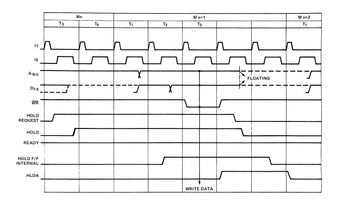
Figure 2-10. HOLD Operation (Write Mode)
