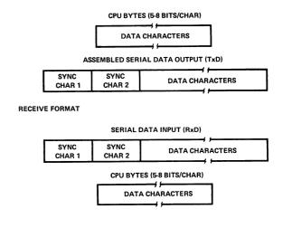
Synchronous Mode, Transmission Format
