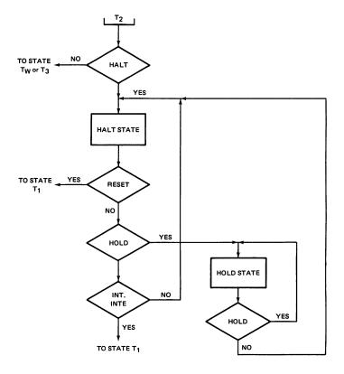
Figure 2-12. HALT Sequence Flow Chart.
