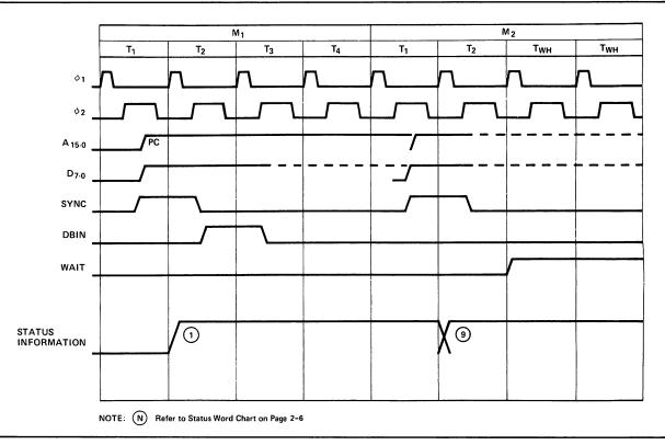
Figure 2-11. HALT Timing
