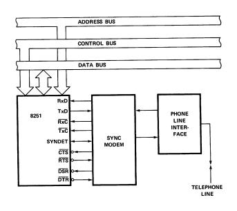
**Synchronous Interface to Telephone Lines**
