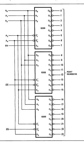
ray of 8205s can be used to create a simple interface to a 24K memory system.
