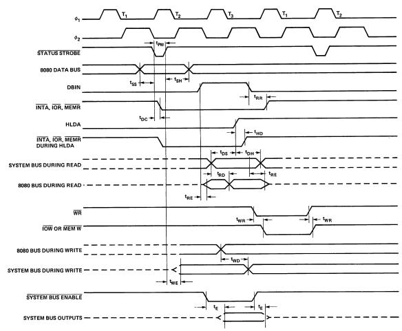
VOLTAGE MEASUREMENT POINTS: D<sub>0</sub>-D<sub>7</sub> (when outputs) Logic "0" = 0.8V, Logic "1" = 3.0V. All other signals measured at 1.5V
