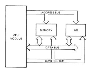
Figure 3-1. Typical Computer System Block Diagram
