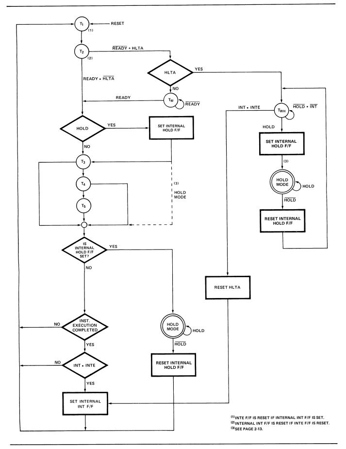
Figure 2-4. CPU State Transition Diagram
