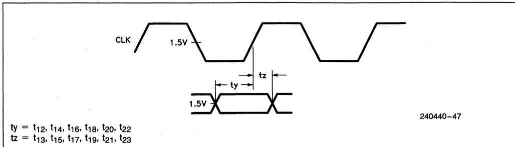
**Figure 12.3. Input Waveforms**
