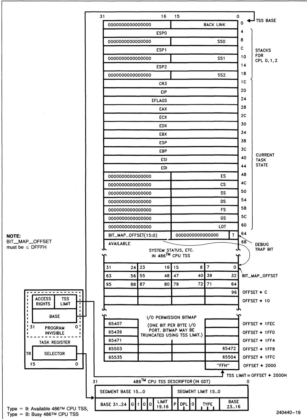
Figure 4.15a. i486™ Microprocessor TSS and TSS Registers
