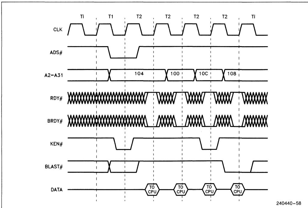
**Figure 7.15. Burst Cycle Showing Order of Addresses**
