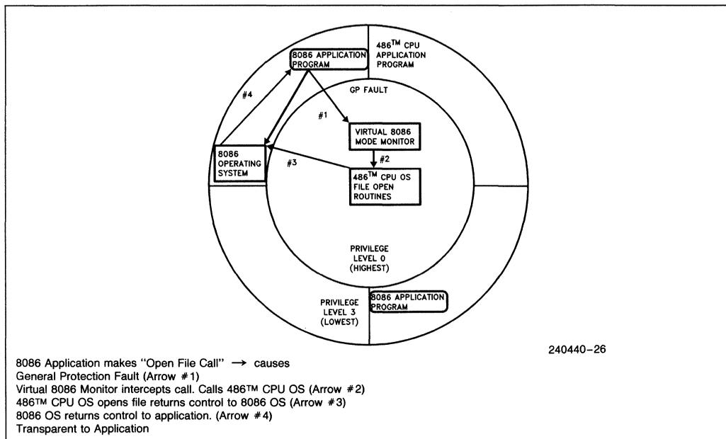
**Figure 4.25. Virtual 8086 Environment Interrupt and Call Handling**
