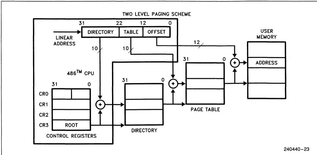
Figure 4.19. Paging Mechanism
