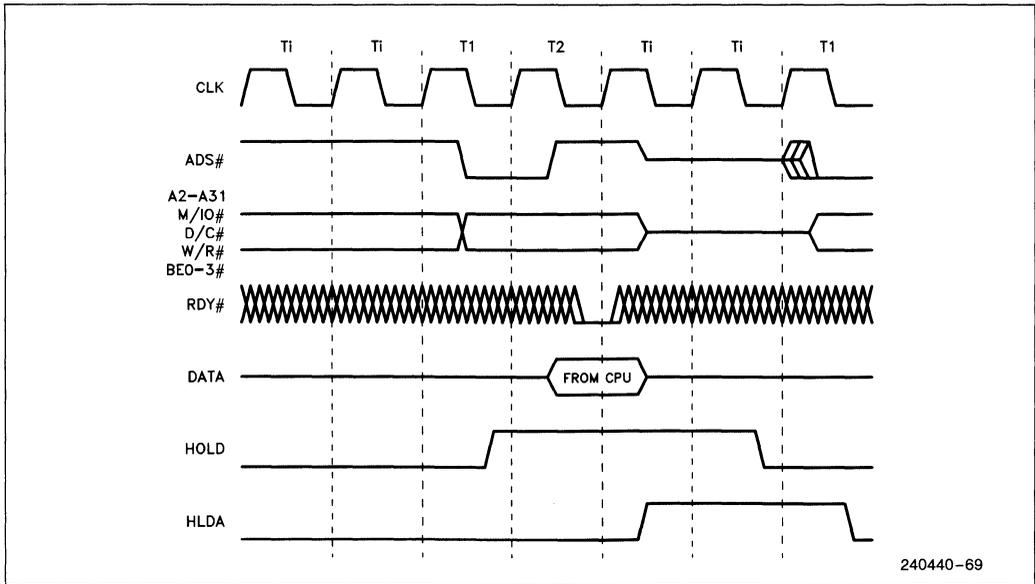
**Figure 7.26. HOLD/HLDA Cycles**
