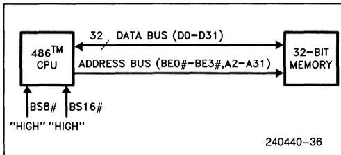
Figure 7.3. i486™ Microprocessor with 32-Bit Memory
