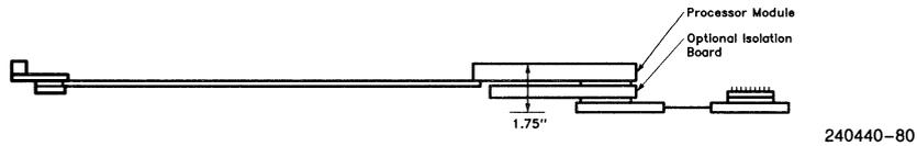
Figure 12.4c. ICD-486™ Probe Dimensions
