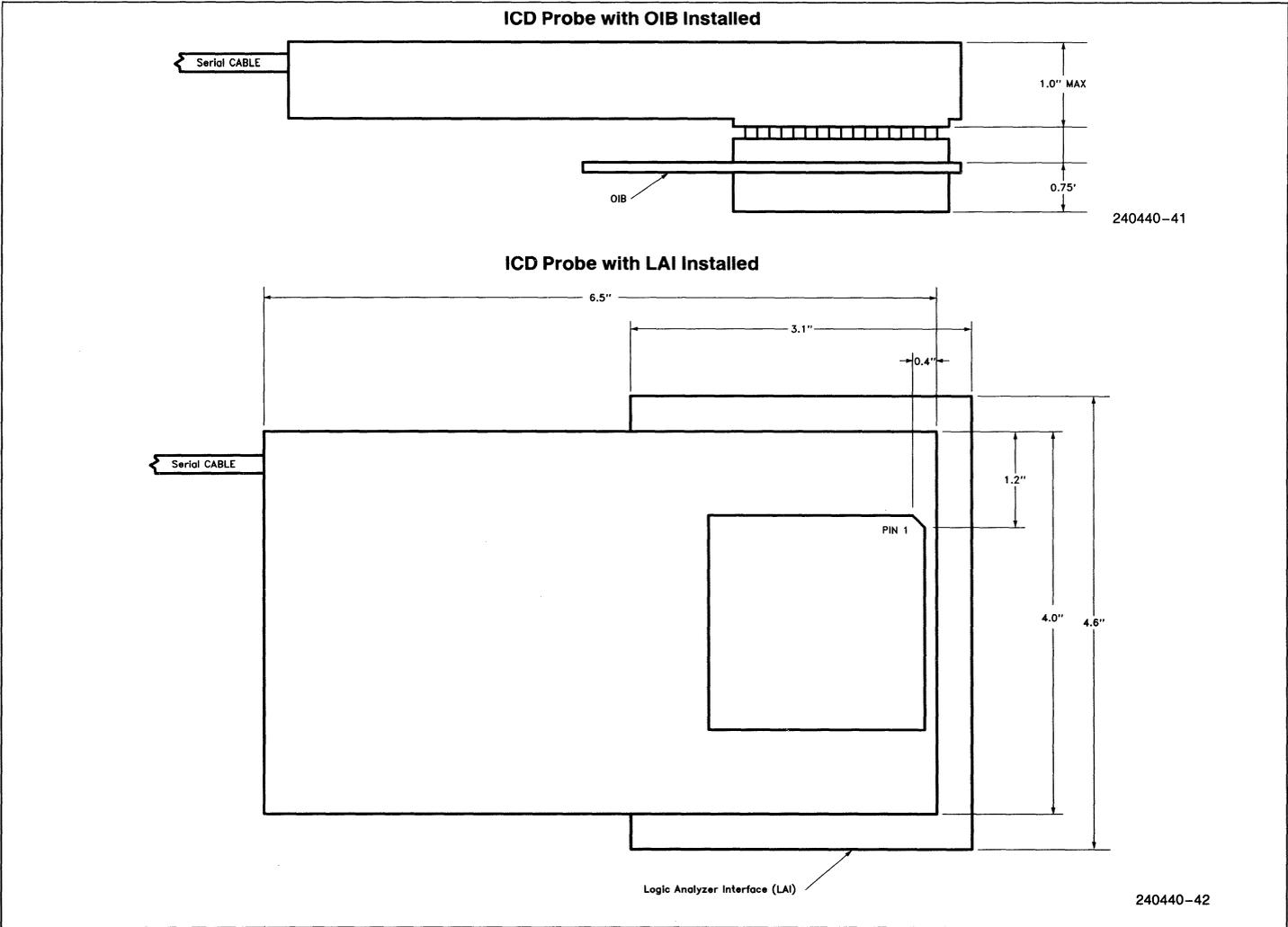
Figure 12.4b. ICD-486™ Probe Dimensions
