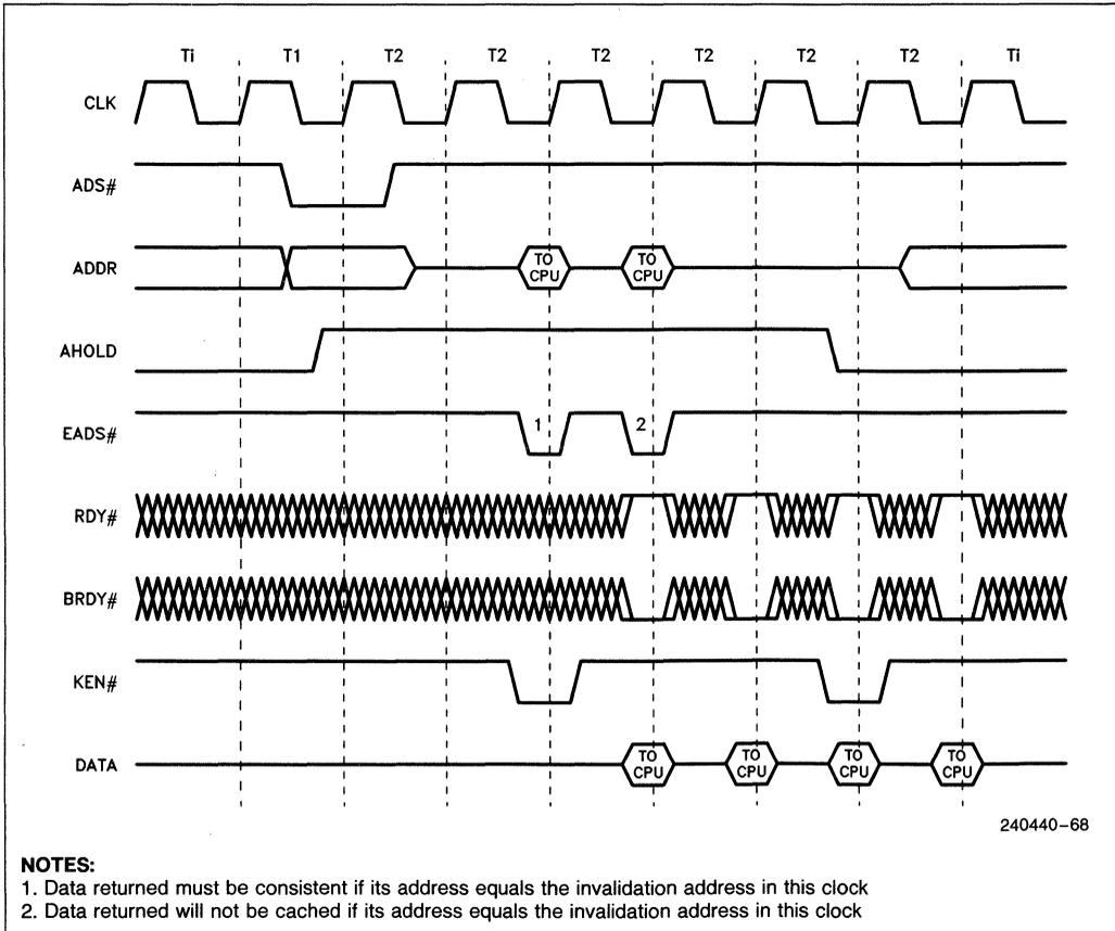
**Figure 7.25. Cache Invalidation Cycle Concurrent with Line Fill**
