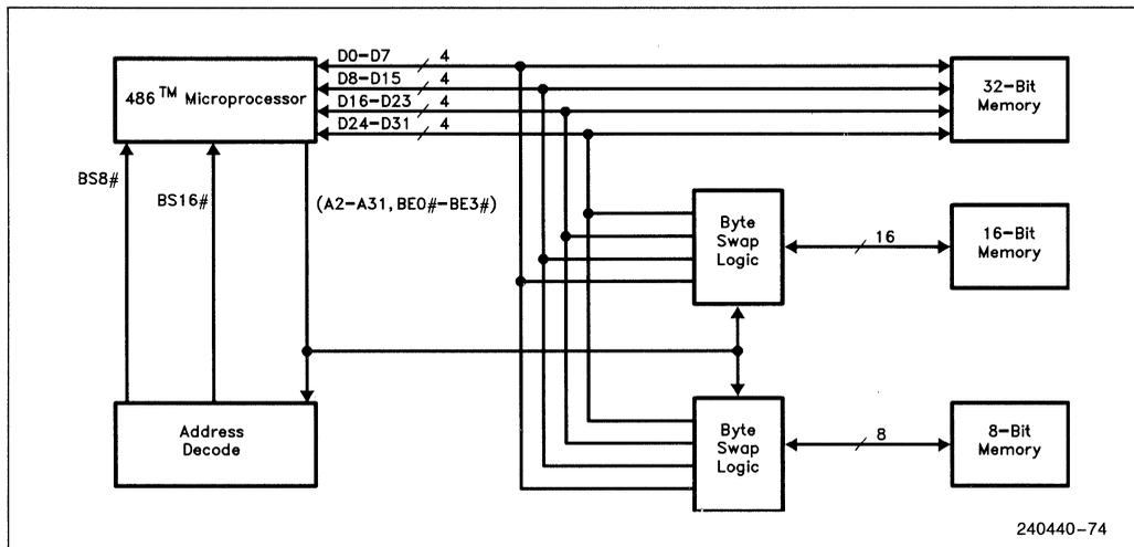
**Figure 7.6. Data Bus Interface to 16- and 8-bit Memories**
