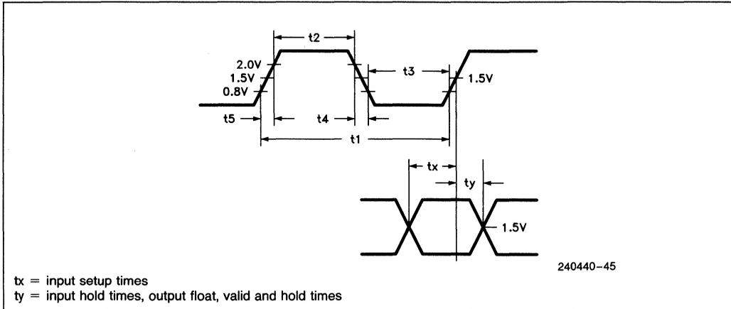
**Figure 12.1. CLK Waveforms**
