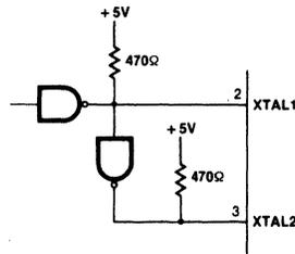
BOTH XTAL1 AND XTAL2 SHOULD BE DRIVEN. RESISTORS TO  $V_{CC}$  ARE NEEDED TO ENSURE  $V_{IH} = 3.8V$  IF TTL CIRCUITRY IS USED.
