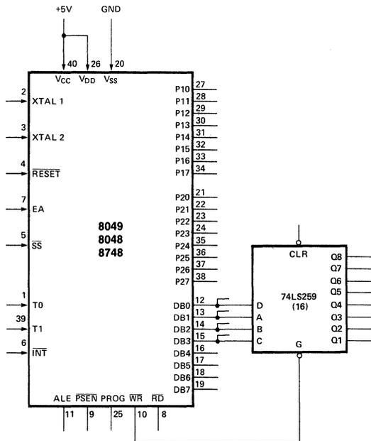
Individual bits of the 74LS259 eight-bit addressable latch can be set or reset using the OUTL instruction. During the OUTL operation bit zero of the accumulator is written into the bit of the latch specified by bits 1 through 3 of the accumulator. In this configuration DB0-DB7 will be momentarily disturbed while the external latch is loaded.
