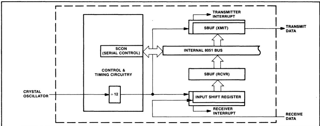
Figure 2.6.A Serial Port—Synchronous Mode 0
