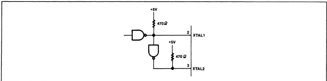
XTAL 1 MUST BE HIGH 35-65% OF THE PERIOD AND XTAL 2 MUST BE HIGH 35-65% OF THE PERIOD. RISE AND FALL TIMES MUST NOT EXCEED 20ns.
