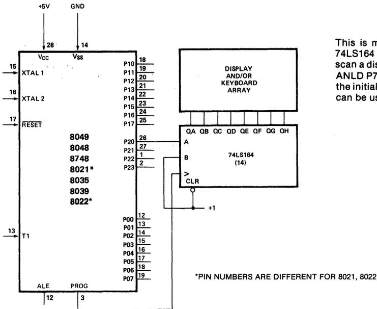
This is most useful when the outputs of the 74LS164 eight-bit shift register will be used to scan a display and/or keyboard. In this case an ANLD P7, A with A = 0FFH can be used to load the initial "1" and an ANLD P6, A with A = 0FEH can be used to move it down the shift register.
