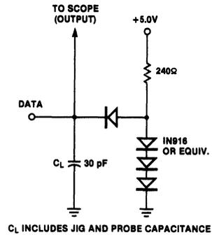
Figure 12. Bus Input to Data Output (Receiver)
