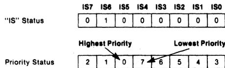
The Rotate command mode A is issued in OCW2 where:  $R=1$ ,  $EOI=1$ ,  $SEOI=0$ . Internal status is updated by an End of Interrupt (EOI or AEOI) command. If  $R=1$ ,  $EOI=0$ ,  $SEOI=0$ , a "Rotate-A" flip-flop is set. This is useful in AEOI, and described under Automatic End of Interrupt.
