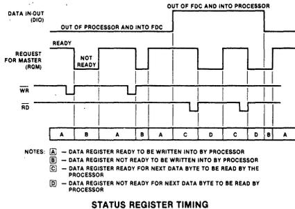
The 8272 is capable of executing 15 different commands. Each command is initiated by a multi-byte transfer from the processor, and the result after execution of the command may also be a multi-byte transfer back to the processor. Because of this multi-byte interchange of information between the 8272 and the processor, it is convenient to consider each command as consisting of three phases:
