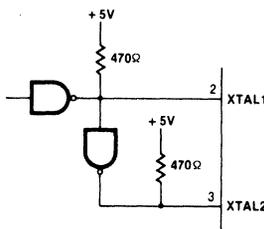
FOR XTAL 1 AND XTAL 2 DEFINE "HIGH" AS VOLTAGES ABOVE 1.6V AND "LOW" AS VOLTAGES BELOW 1.6V. THE DUTY CYCLE REQUIREMENTS FOR EXTERNALLY DRIVING XTAL 1 AND XTAL 2 USING THE CIRCUIT SHOWN ABOVE ARE AS FOLLOWS:
