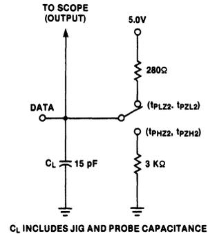
Figure 14. Send/Receive Input to Data Output (Receiver)
