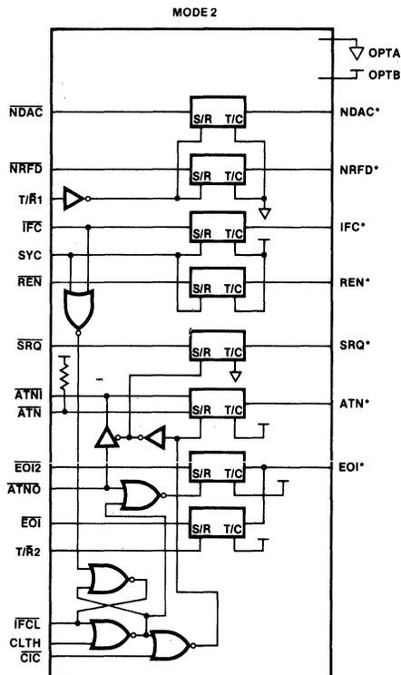
Figure 5. Talker/Listener/Controller Control Configuration
