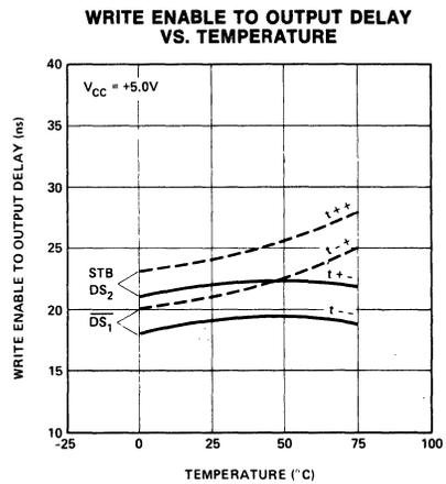
**A.C. CHARACTERISTICS**  $T_A = 0^\circ\text{C}$  to  $+70^\circ\text{C}$ ,  $V_{CC} = +5V \pm 5\%$
