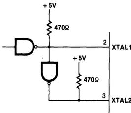
FOR XTAL 1 AND XTAL 2 DEFINE "HIGH" AS VOLTAGES ABOVE 1.8V AND "LOW" AS VOLTAGES BELOW 1.8V. THE DUTY CYCLE REQUIREMENTS FOR EXTERNALLY DRIVING XTAL 1 AND XTAL 2 USING THE CIRCUIT SHOWN ABOVE ARE AS FOLLOWS:
