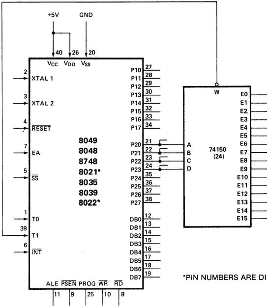
Normal I/O port is used to select an address for the 16-to-1 multiplexer. The output of the multiplexer is brought into a test input. Eight inputs could be added with a 74LS151 8-to-1 multiplexer using the same structure.
