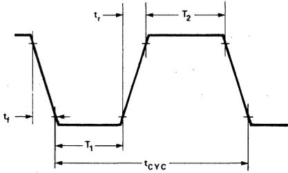
Figure 2. Clock Specification for 8755A
