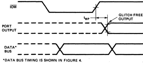
Figure 3. I/O Port Timing
