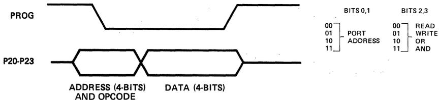
A high to low transition of the PROG line indicates that address is present while a low to high transition indicates the presence of data. Additional 8243's may be added to the four bit bus and chip selected using additional output lines from the 8048/8748.
