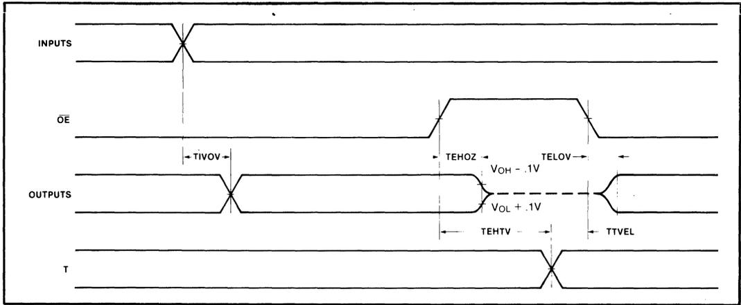
NOTE: 1. All timing measurements are made at 1.5V unless otherwise noted.
