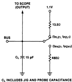
Figure 13. Send/Receive Input to Bus Output (Driver)
