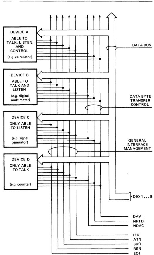
Figure 1. Interface Capabilities and Bus Structure.
