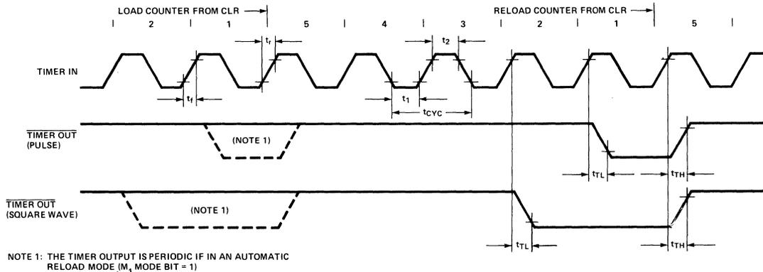
Figure 15. Timer Output Waveform Countdown from 5 to 1
