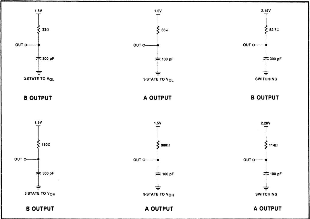
Figure 5. Test Load Circuits
