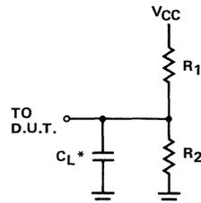
\*INCLUDING JIG & PROBE CAPACITANCE
