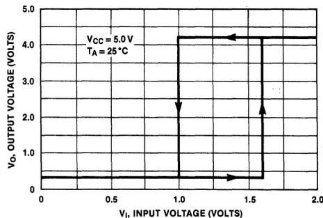
Figure 10. Typical Receiver Hysteresis Characteristics
