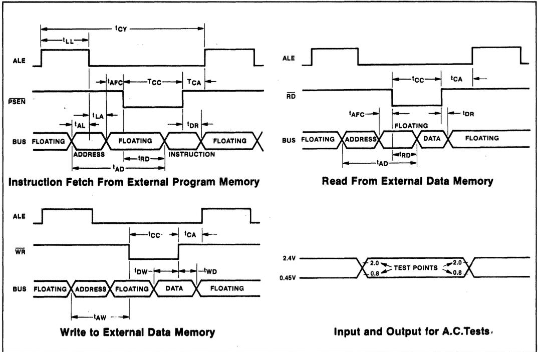
A.C. CHARACTERISTICS  $T_A = 0^\circ\text{C}$  to  $70^\circ\text{C}$   $V_{CC} = V_{DD} = 5V \pm 10\%$ ,  $V_{SS} = 0V$
