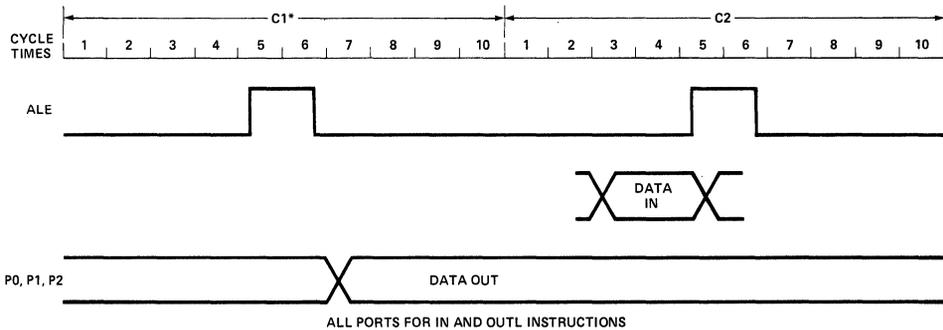
FIGURE 2. 8021 TIMING DIAGRAM
