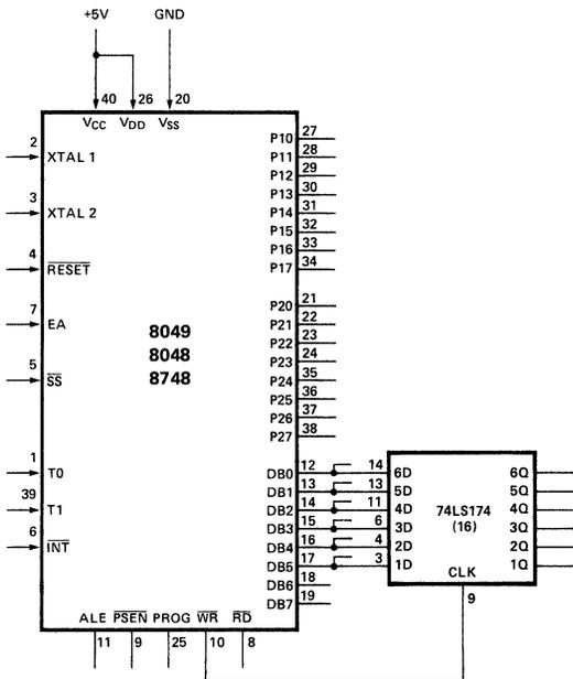
The latch can be loaded with the OUTL instruction. After the latch is loaded the BUS output state can be modified with the ANL BUS, # DATA and the ORL BUS, # DATA. The OUTL generates a WR strobe; ANL and ORL do not. In this configuration DB<sub>0</sub>-DB<sub>7</sub> will be momentarily disturbed while the external latch is loaded.
