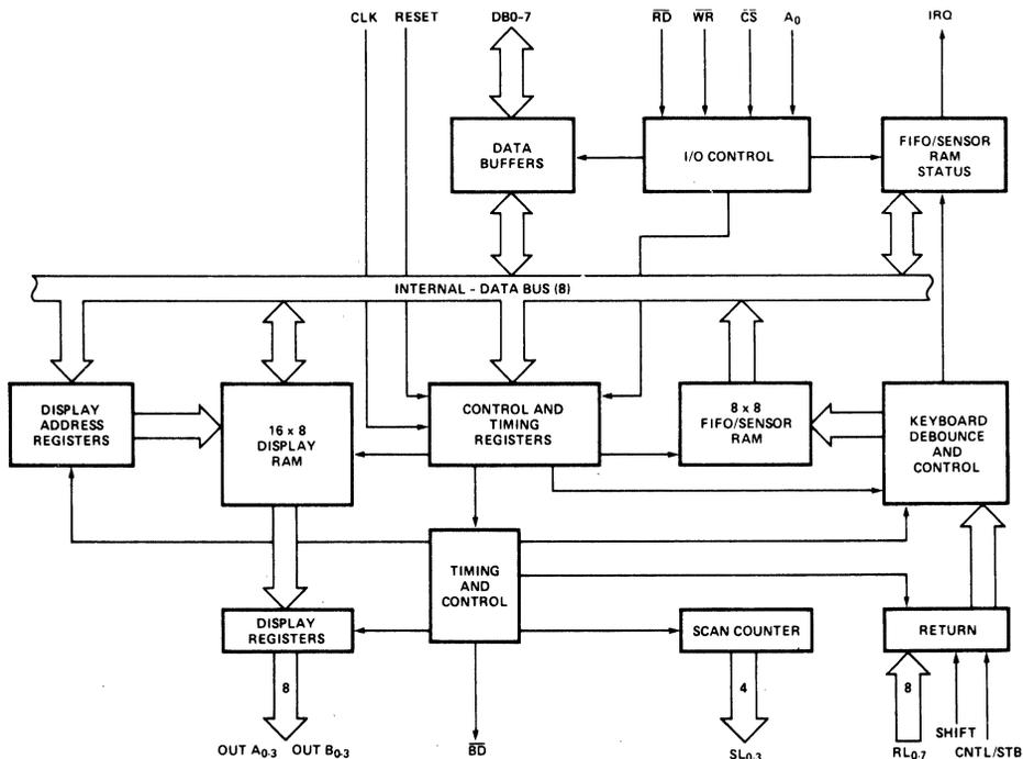
The command is then decoded and the appropriate function is set. The timing control contains the basic timing counter chain. The first counter is a  $\div N$  prescaler that can be programmed to yield an internal frequency of 100 kHz which gives a 5.1 ms keyboard scan time and a 10.3 ms debounce time. The other counters divide down the basic internal frequency to provide the proper key scan, row scan, keyboard matrix scan, and display scan times.
