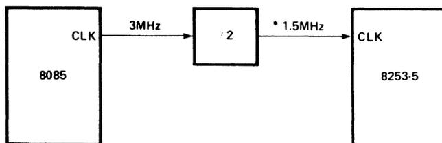
\*If an 8085 clock output is to drive an 8253-5 clock input, it must be reduced to 2 MHz or less.
