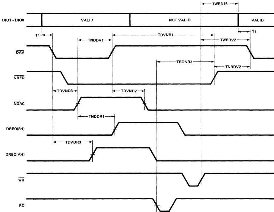
Figure C-1. 3-Wire Handshake Timing at 8291.
