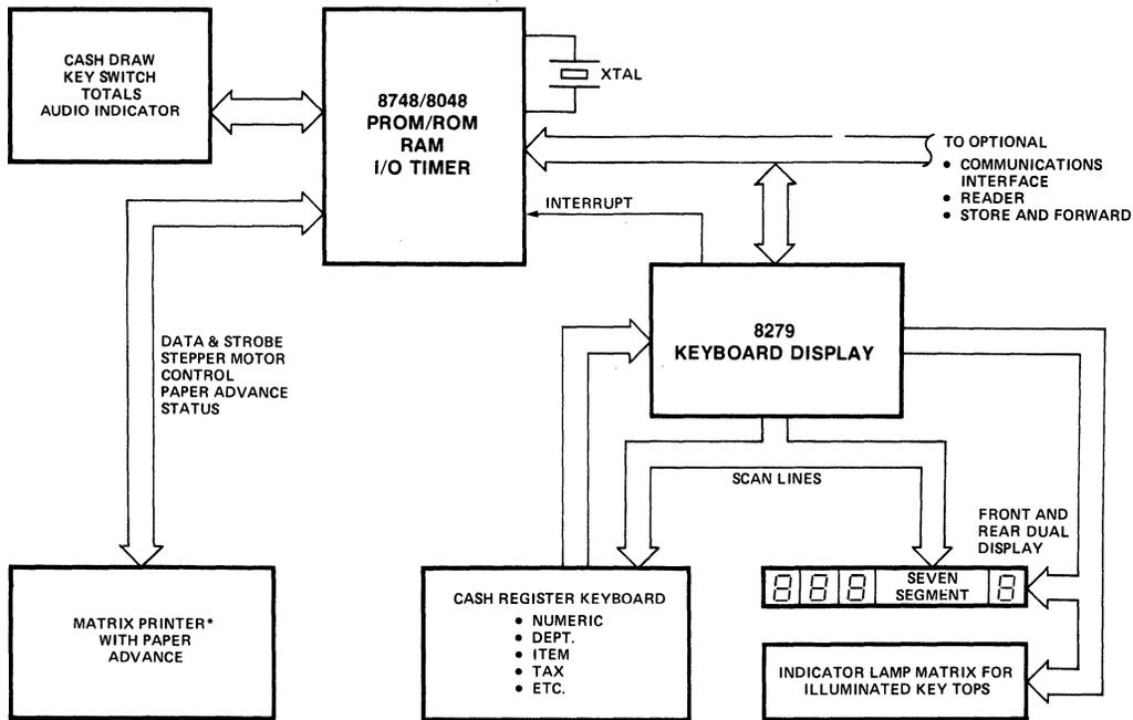
\*DRUM PRINTER MAY BE USED. DRUM PRINTER REQUIRES MORE OUTPUTS WHICH CAN BE OBTAINED FROM AN EXPANDER DEVICE.
