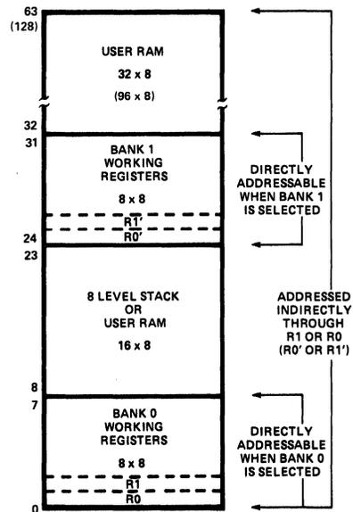
IN ADDITION R0 OR R1 (R0' OR R1') MAY BE USED TO ADDRESS 256 WORDS OF EXTERNAL RAM.
