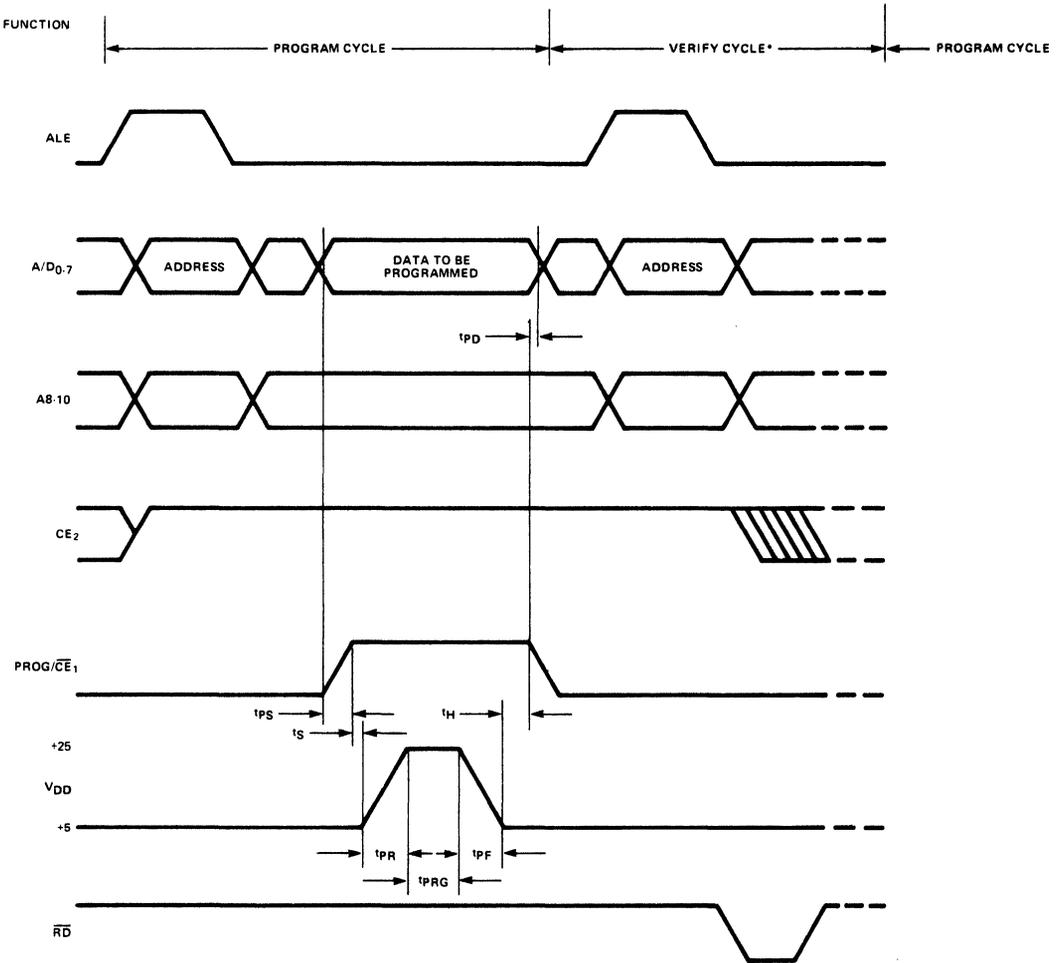
\*VERIFY CYCLE IS A REGULAR MEMORY READ CYCLE (WITH V<sub>DD</sub> = +5V FOR 8755A)
