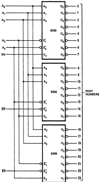
Figure 2. I/O Port Decoder
