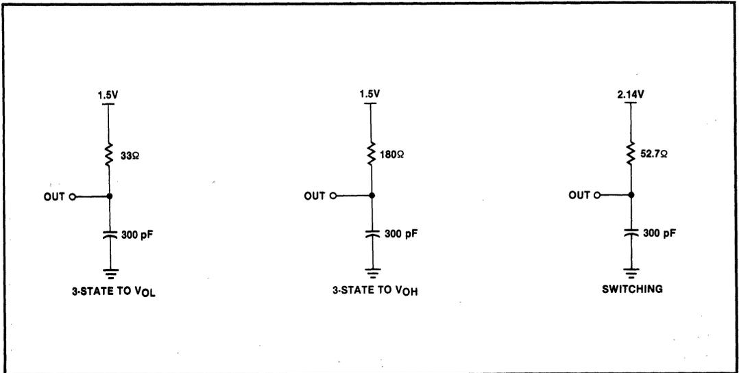
Figure 5. Output Test Load Circuits
