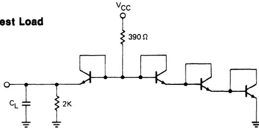
All Transistors 2N2369 or Equivalent.  $C_L = 30$  pF
