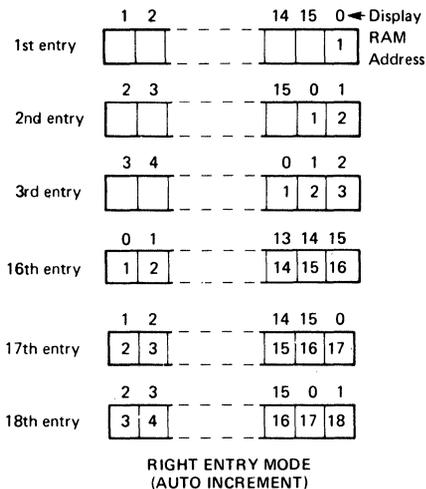
Note that now the display position and register address do not correspond. Consequently, entering a character to an arbitrary position in the Auto Increment mode may have unexpected results. Entry starting at Display RAM address 0 with sequential entry is recommended.
