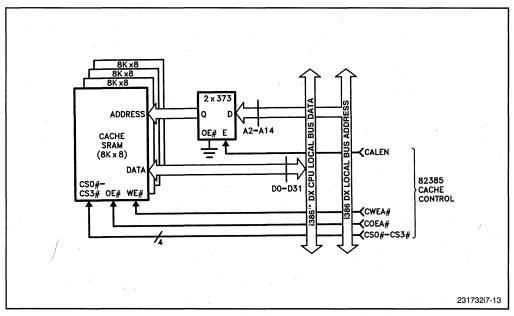
Figure 7-13. Direct Mapped Cache without Data Buffers
