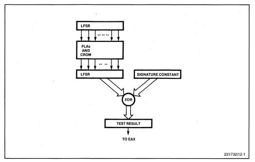
Figure 12-1. Intel386™ DX Microprocessor Self-Test
