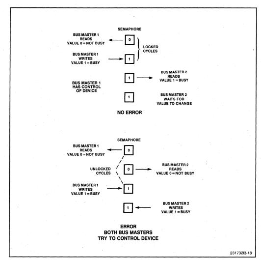
Figure 3-18. Error Condition Caused by Unlocked Cycles
