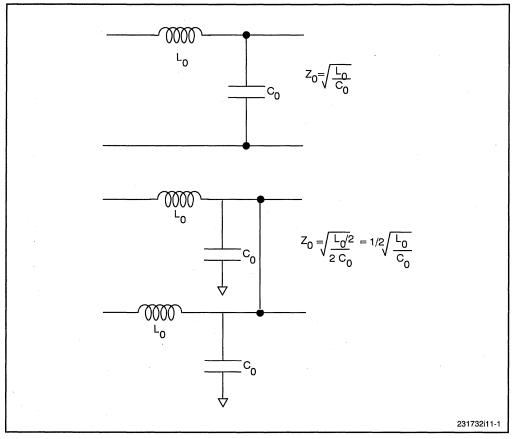
Figure 11-1. Reduction in Impedance
