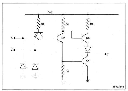
Figure 11-4. Circuit without Decoupling
