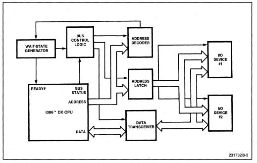
Figure 8-3. Basic I/O Interface Block Diagram
