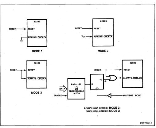
Figure 9-8. Operating Mode Configurations
