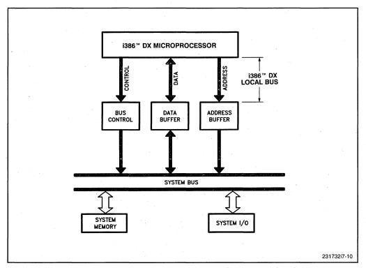
Figure 7-10. Intel386™ DX Microprocessor System Bus Structure
