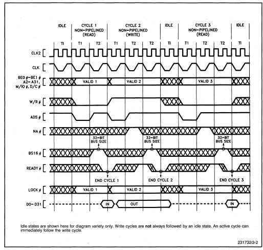
Figure 3-2. Intel386<sup>™</sup> DX CPU Bus States Timing Example
