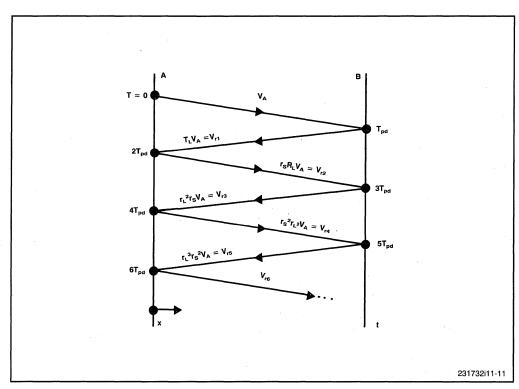
Figure 11-11. Lattice Diagram
