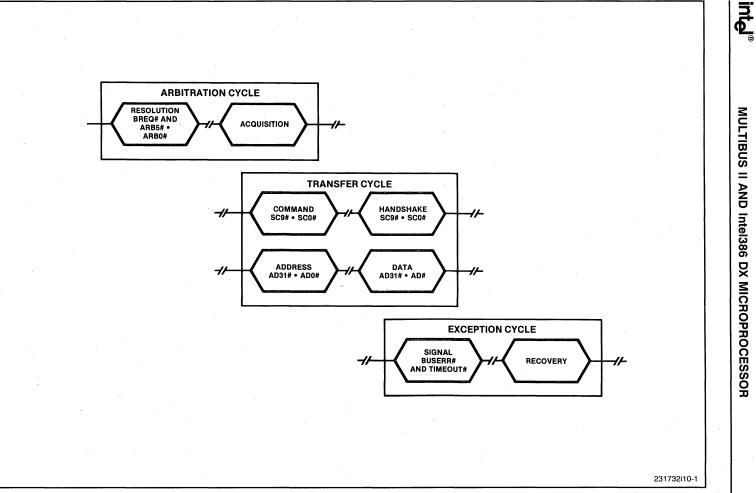
Figure 10-1. iPSB Bus Cycle Timing
