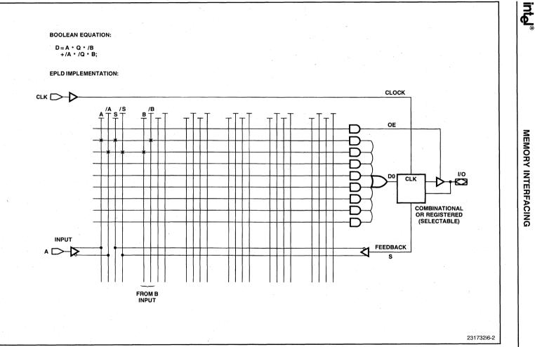
Figure 6-2. PLD Equation and Device Implementation
