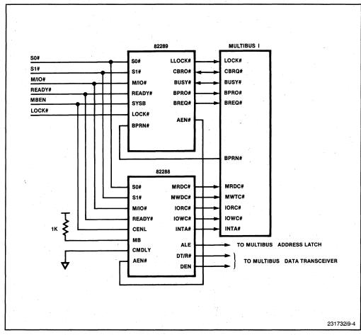
Figure 9-4. MULTIBUS Arbiter and Bus Controller
