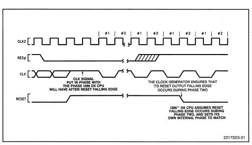
Figure 3-21. RESET, CLK, and CLK2 Timing
