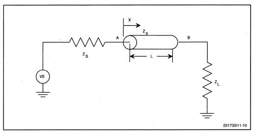
Figure 11-10. Loaded Transmission Line
