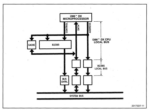
Figure 7-11. Intel386<sup>™</sup> DX Microprocessor/82385 System Bus Structure
