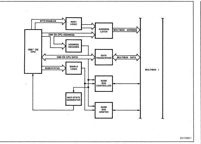
Figure 9-1. Intel386<sup>™</sup> DX Microprocessor/MULTIBUS I Interface
