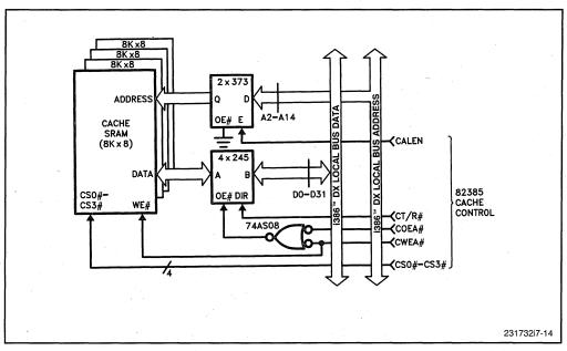
Figure 7-14. Direct Mapped Cache with Data Buffers
