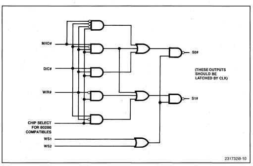
Figure 8-10. S0#/S1# Generator Logic
