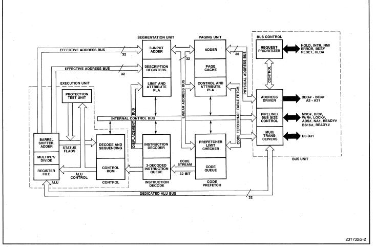
Figure 2-2. Intel386<sup>™</sup> DX Microprocessor Functional Units
