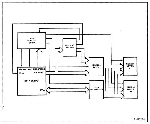
Figure 6-1. Basic Memory Interface Block Diagram
