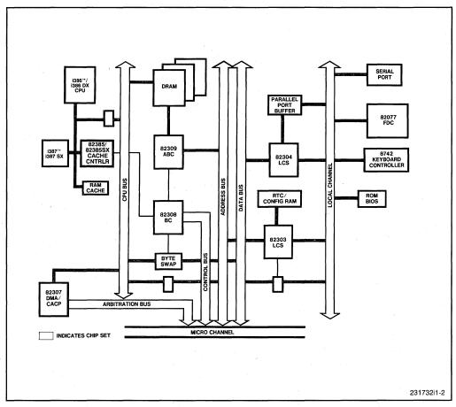
Figure 1-2. Micro Channel-Compatible Solution with 82311 Chip Set
