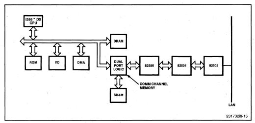
Figure 8-15. Decoupled Dual-Port Memory Interface
