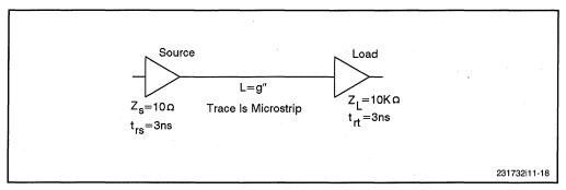
Figure 11-18. Impedance Mismatch Example
