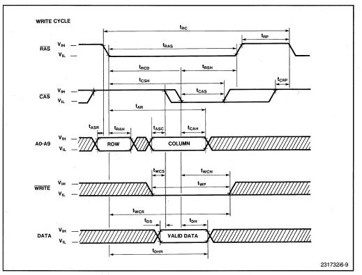
Figure 6-9. Timing Waveforms (Write Cycle)
