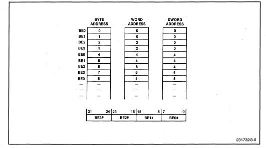
Figure 3-6. Address, Data Bus, and Byte Enables for 32-Bit Bus
