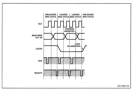
Figure 3-19. LOCK# Signal during Address Pipelining
