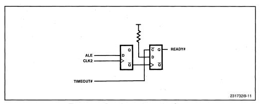
Figure 9-11. Bus-Timeout Protection Circuit
