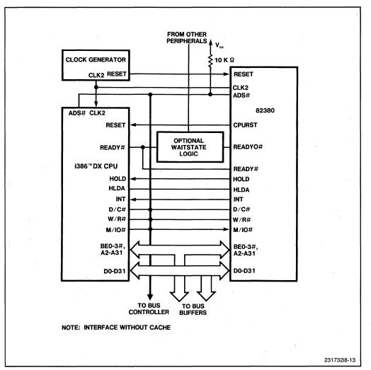
Figure 8-13. Intel386<sup>™</sup> DX Microprocessor/82380 Interface
