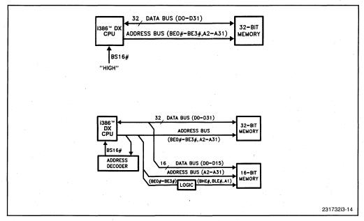
Figure 3-14. 32-Bit and 16-Bit Data Addressing
