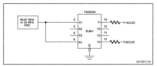
Figure 11-24. Typical Intel386<sup>™</sup> DX Microprocessor Clock Circuit
