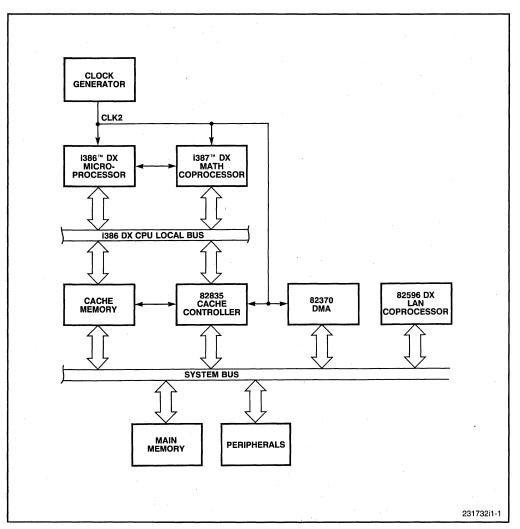
Figure 1-1. Intel386<sup>™</sup> DX Microprocessor System Block Diagram
