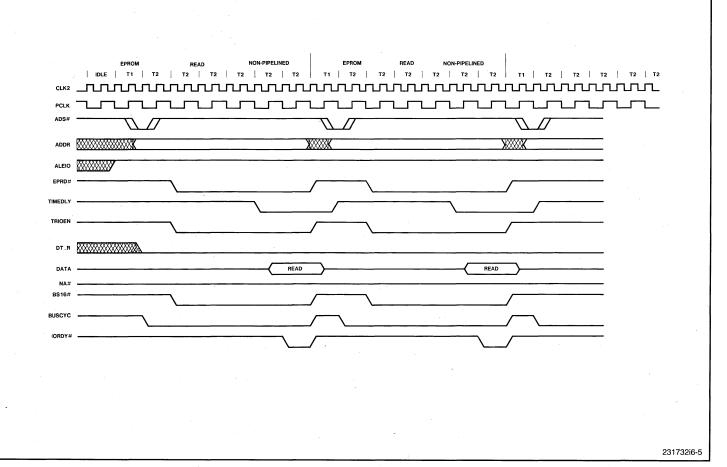
Figure 6-5. 250 Nanosecond EPROM Timing Diagram
