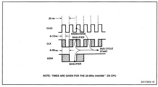
Figure 3-15. Using CLK to Determine Bus Cycle Start
