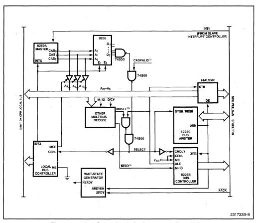
Figure 9-9. Bus-Select Logic for Interrupt Acknowledge
