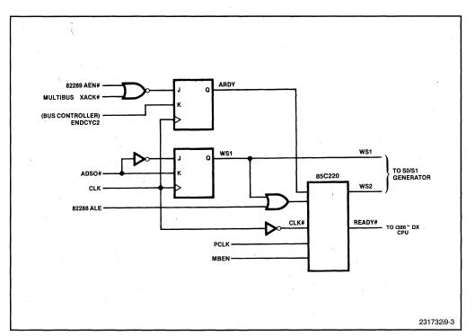
Figure 9-3. Wait-State Generator Logic
