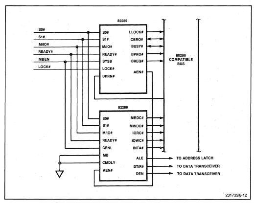
Figure 8-12. 82288 and 82289 Connections
