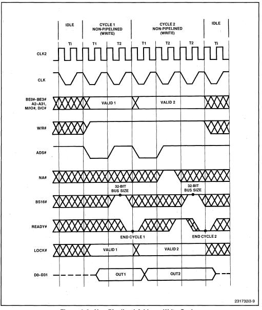
Figure 3-9. Non-Pipelined Address Write Cycles
