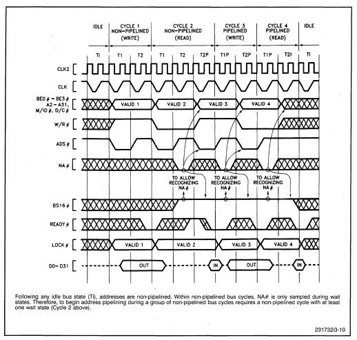
Figure 3-10. Pipelined Address Cycles
