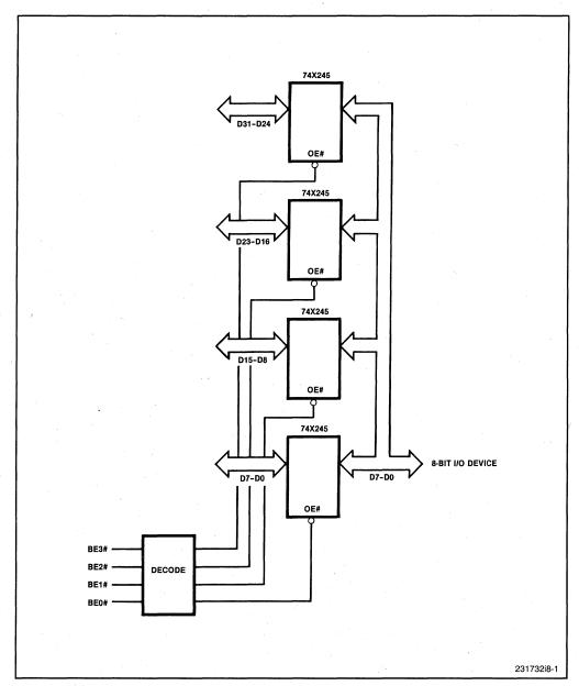
Figure 8-1. 32-Bit to 8-Bit Bus Conversion
