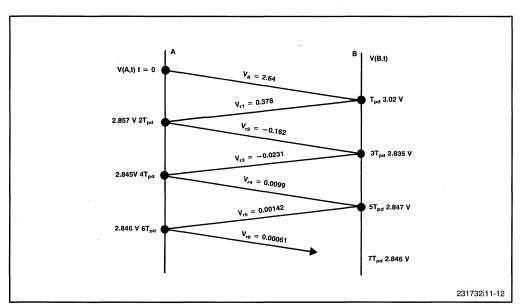
Figure 11-12. Lattice Diagram Example
