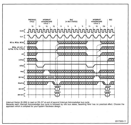
Figure 3-11. Interrupt Acknowledge Bus Cycles
