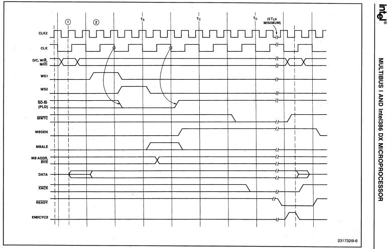
Figure 9-6. MULTIBUS I Write Cycle Timing
