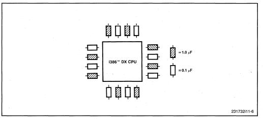
Figure 11-6. Decoupling with Leaded Capacitors
