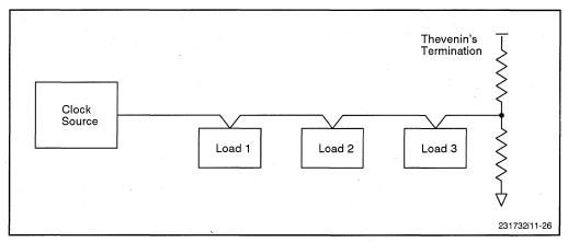
Figure 11-26. Clock Routing
