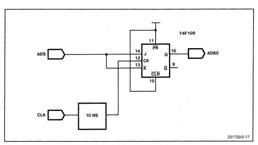
Figure 3-17. ADS# Synchronizer
