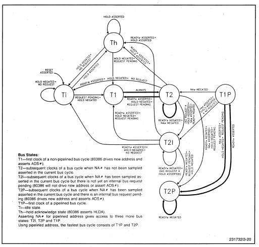
Figure 3-20. Bus State Diagram with HOLD State
