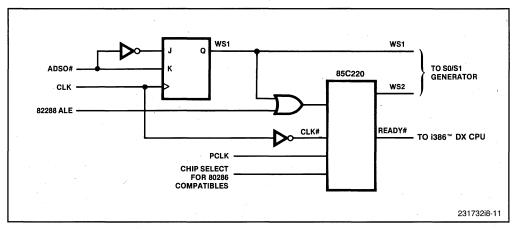
Figure 8-11. Wait-State Generator Logic
