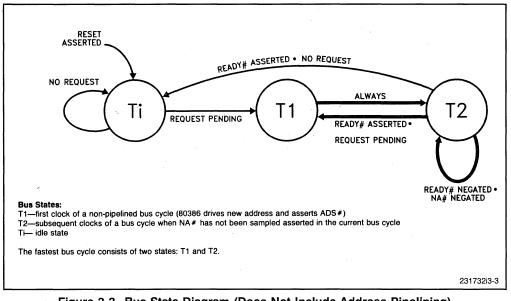
Figure 3-3. Bus State Diagram (Does Not Include Address Pipelining)
