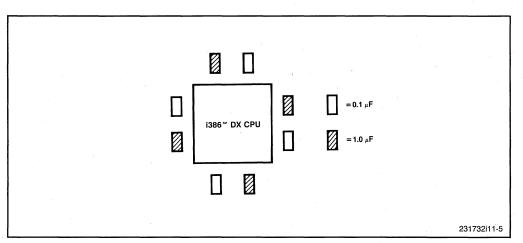
Figure 11-5. Decoupling with Surface Mount Capacitors
