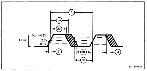
Figure 11-25. CLK2 Timing Diagram
