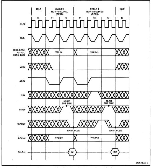
Figure 3-8. Non-Pipelined Address Read Cycles
